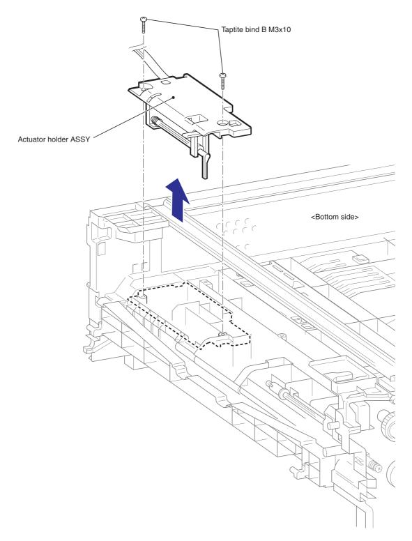
(2) Remove the two Taptite bind B M3x10 screws, and then remove the Actuator holder ASSY from the Main body.
