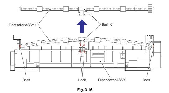
(3) Remove the Bush C, the Bush R and the Bush L from the Eject roller ASSY 1.
