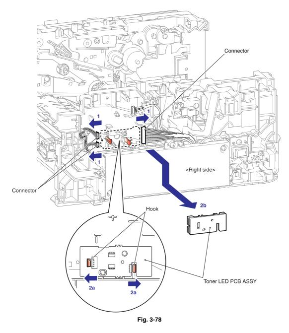
(3) Release the Hook to remove the LED holder from the Toner LED PCB ASSY.
