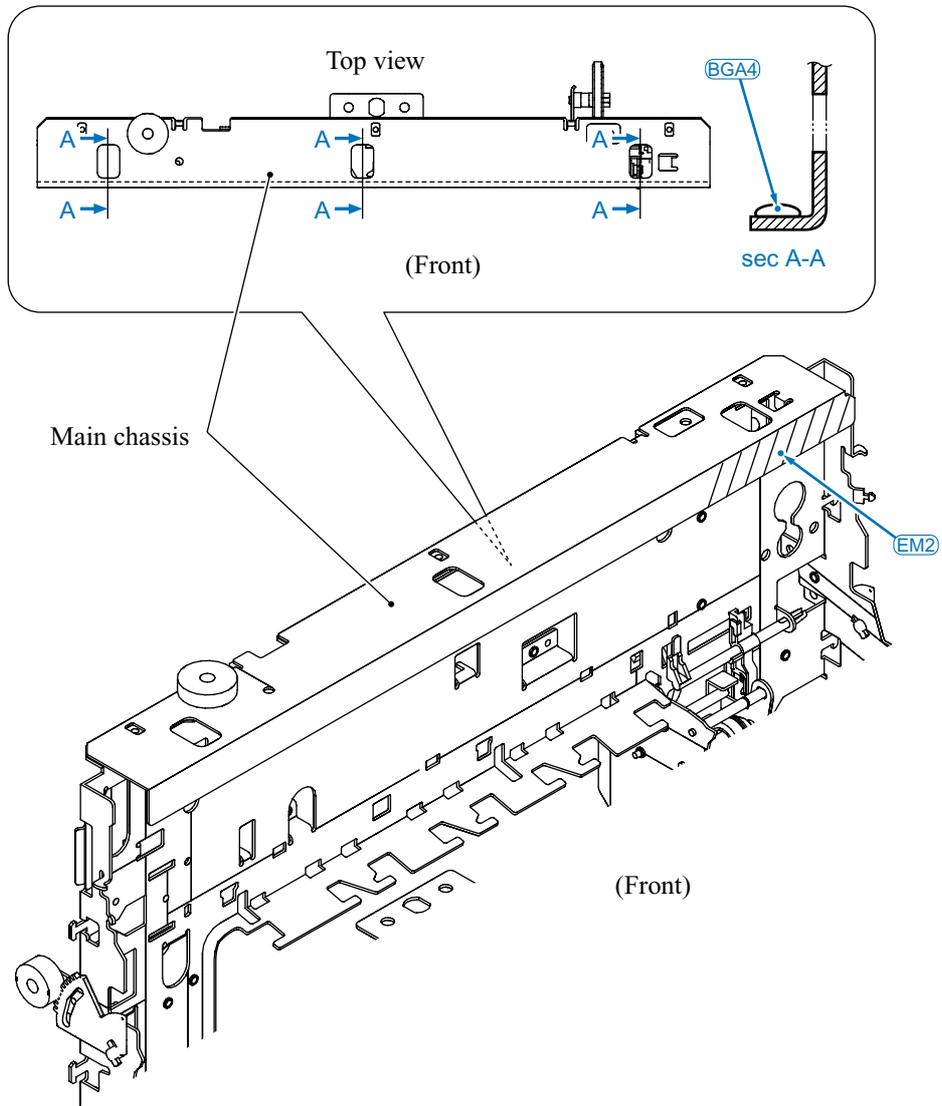
**[ 9 ] Purge shaft and slideway of the purge lever on the main chassis**
