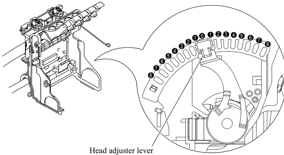
(12) To install a new (or removed) print head unit, remove the head nozzle seal.
