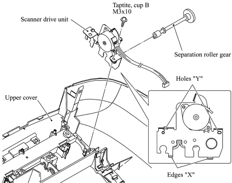
(7) Remove the screw and release the scanner motor from the scanner drive unit.
