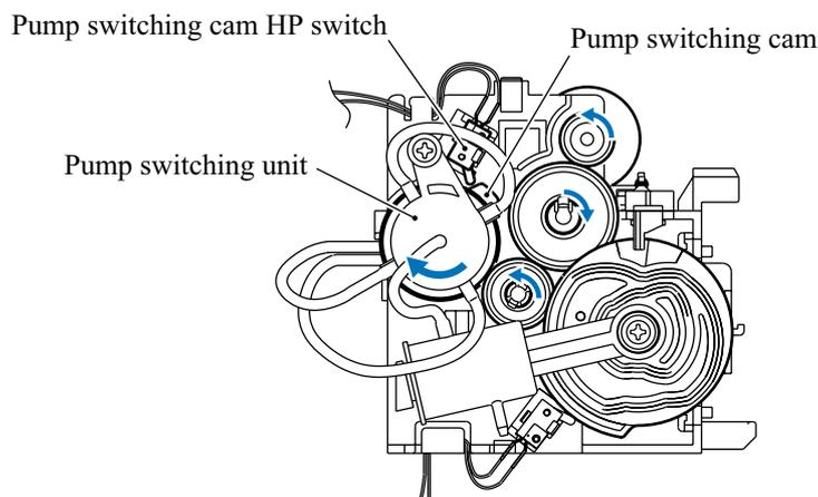
When the paper feed motor rotates clockwise
