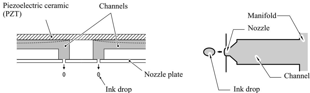
As the carriage holding the print head unit travels at the printing speed, the controller sends print command pulses to the piezoelectric actuator driver circuit embedded in the print head unit.
