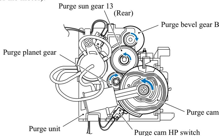
When the paper feed motor rotates counterclockwise
