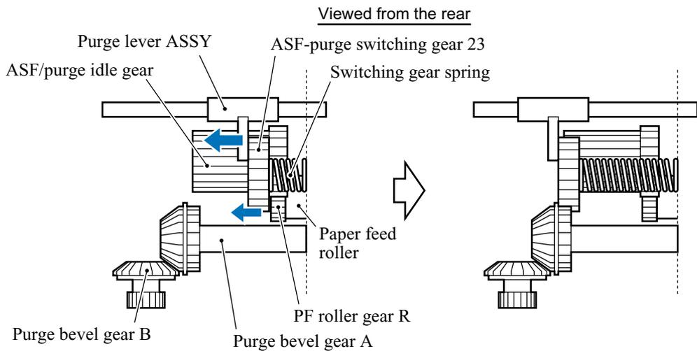
During printing: The ASF-purge switching gear 23 is not engaged with purge bevel gear A (but engaged with gear 25 in the ASF gear train).
