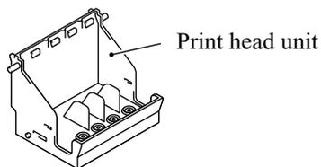
**NOTE:** Be sure to put a head nozzle seal and filter seal on the print head unit as shown below. Leaving the print head unit without those seals will dry up its printing ends and filters, resulting in a damaged head.
