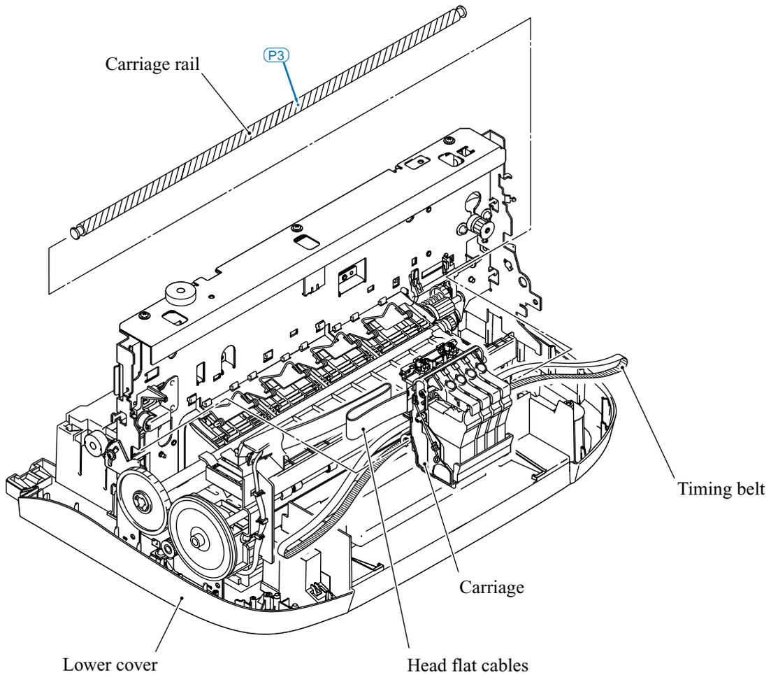
[ 8 ] Main chassis (slideway of the carriage guide)
