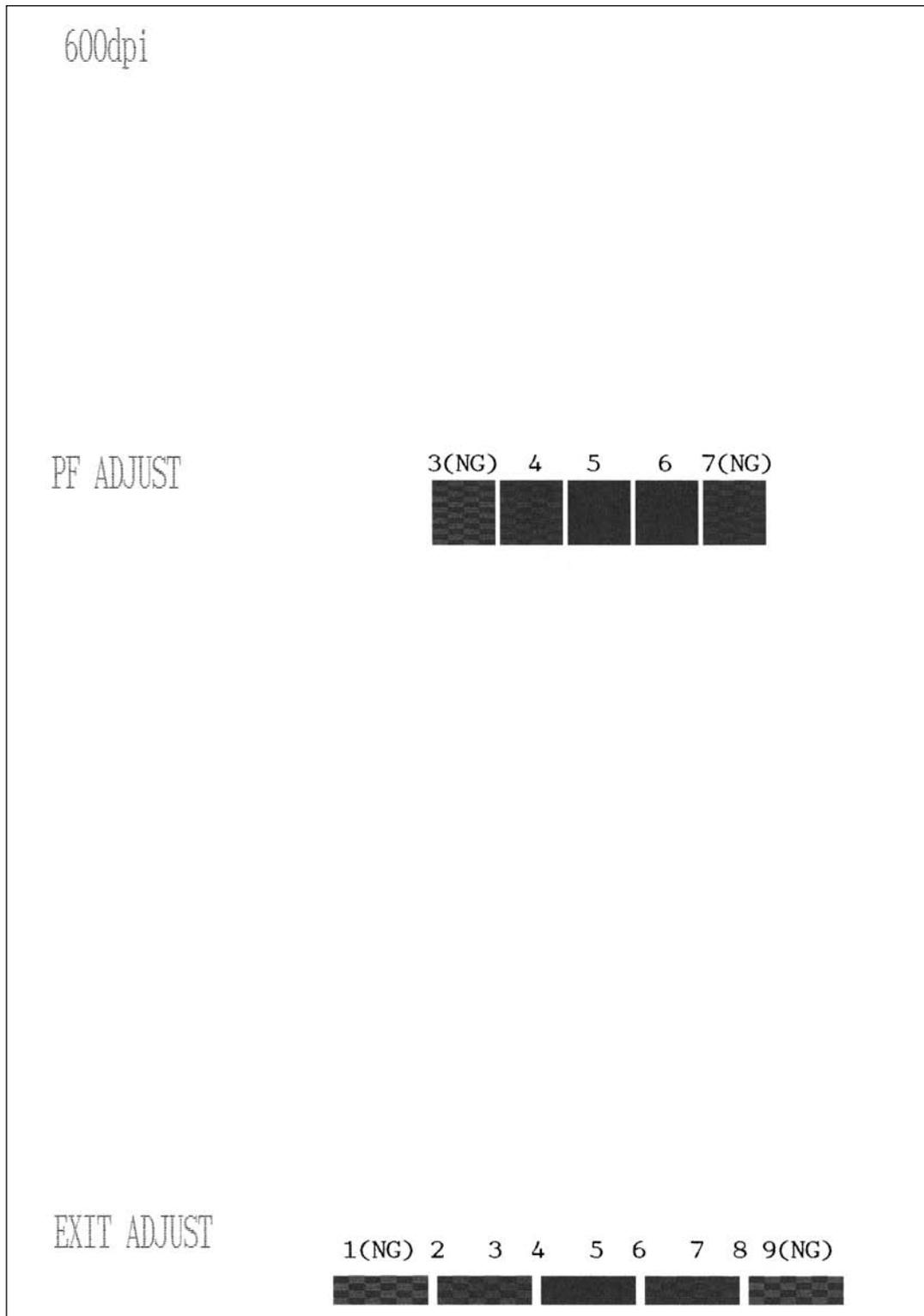
**Paper Feeding Check Patterns for the Paper Feed Roller and Paper Ejection Roller**
