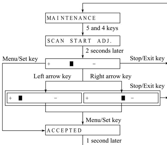
**NOTE:** The relationship between the scanning start/end positions and their correction values is shown below.
