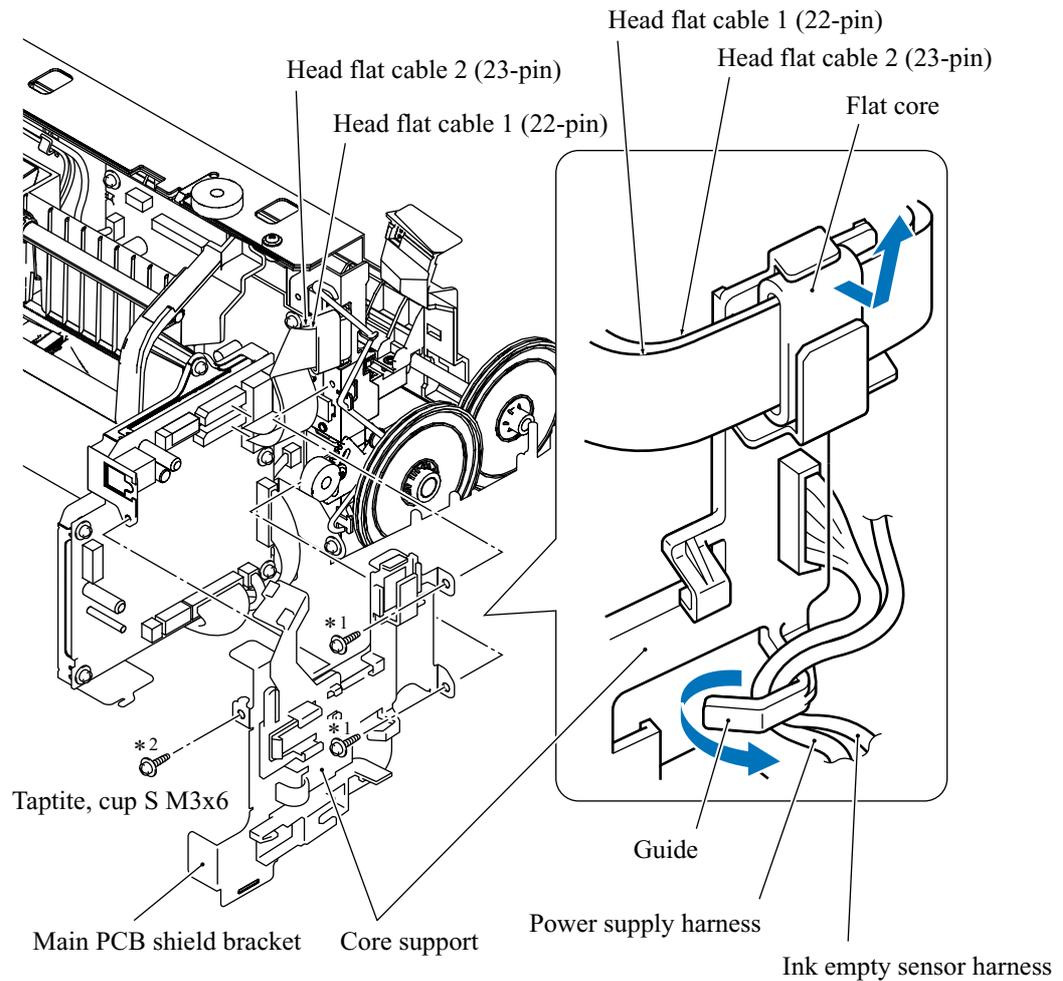
\*<sup>1</sup> Tightening torque:  $0.78 \pm 0.10 \text{ N}\cdot\text{m}$
