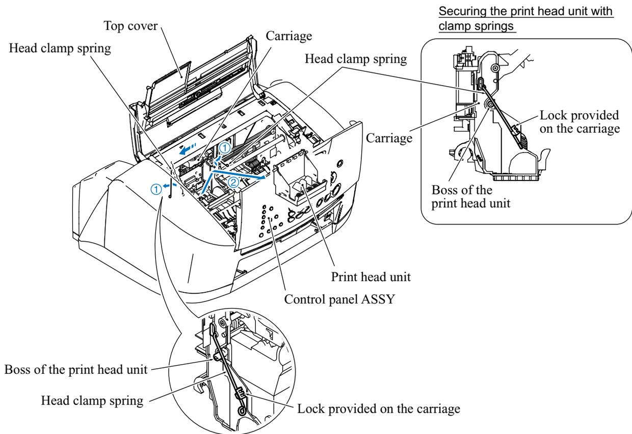
**NOTE:** Do not touch the printing ends (nozzles) of the print head unit or the ink orifices of the ink cartridges; doing so will not only stain your hands with ink but result in an ink jet-out failure. Once you touch them, clean them with a dedicated cleaning stick and liquid.
