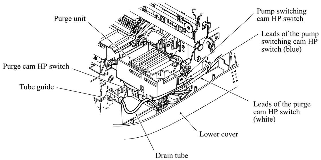
**Harness routing D: Head flat cables and power supply harness, and ink empty sensor harness**
