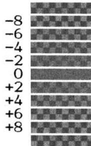
**Head Positioning Test Pattern**
