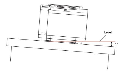
ii) Is the printer inclined because the table surface the printer is installed on is not strong enough?
