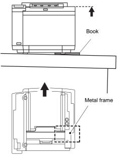
ii) When the gap is less than 3 mm; (the OPC belt has moved to the left.) Place something 1 cm thick such as a book under the left hand side of the printer as shown in the figure on the right.
