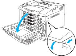
3) Pull out the all toner cartridges from the printer.
