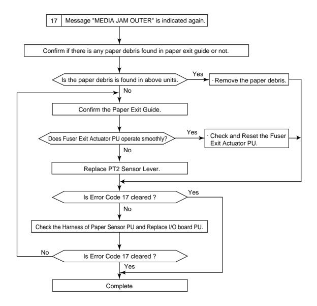
PT2 Sensor : Fuser Exit Sensor
