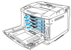
4) Install the orange protective cover to the each toner cartridge as shown in the illustration.
