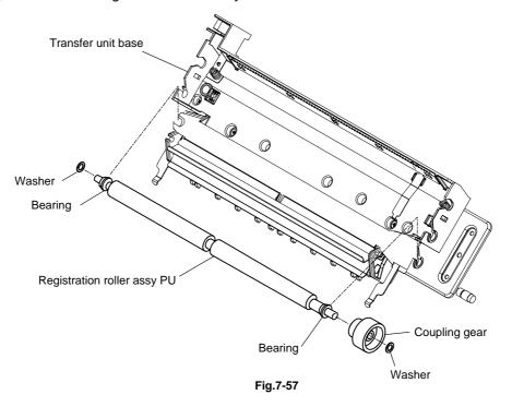
NOTE: Adjustments is required when the Registration Roller is changed. Please refer to Section5 in this chapter.
