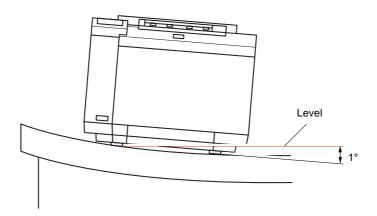
iii) Is the printer inclined because it is installed across two or more tables?
