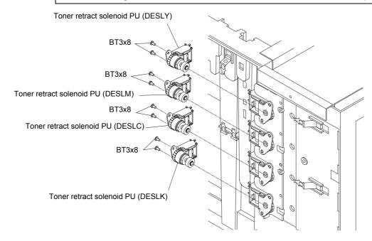
Toner retract solenoid PU (DESLY/DESLM/DESLC/DESLK)
