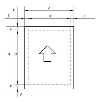
The effective printing area means the area within which the printing of all the data received without any omissions can be guaranteed. (Refer to Table 2-1 for details.)
