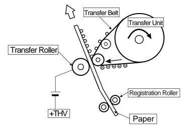
THV: Power Supply for Transfer Roller Bias.
