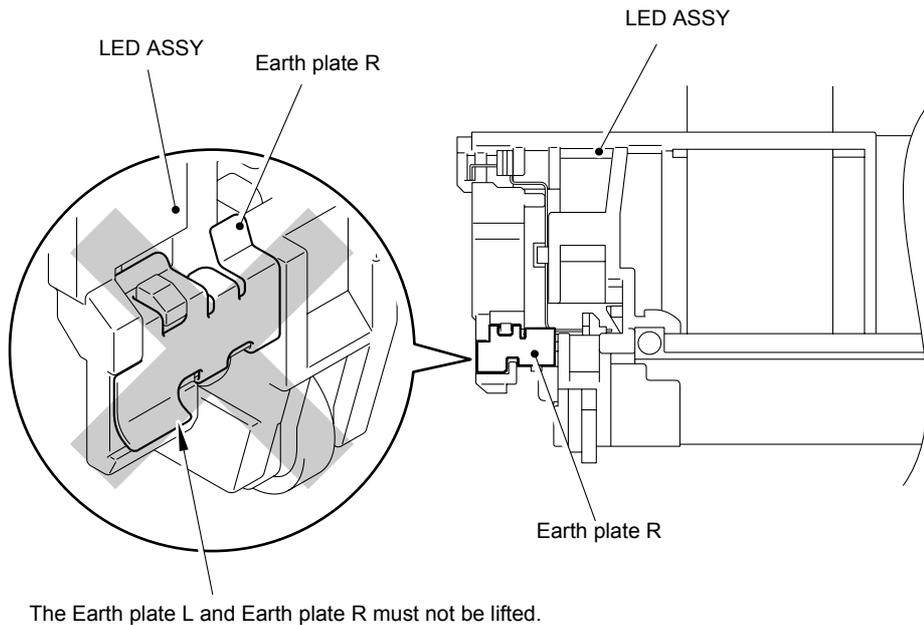
The Earth plate L and Earth plate R must not be lifted.
