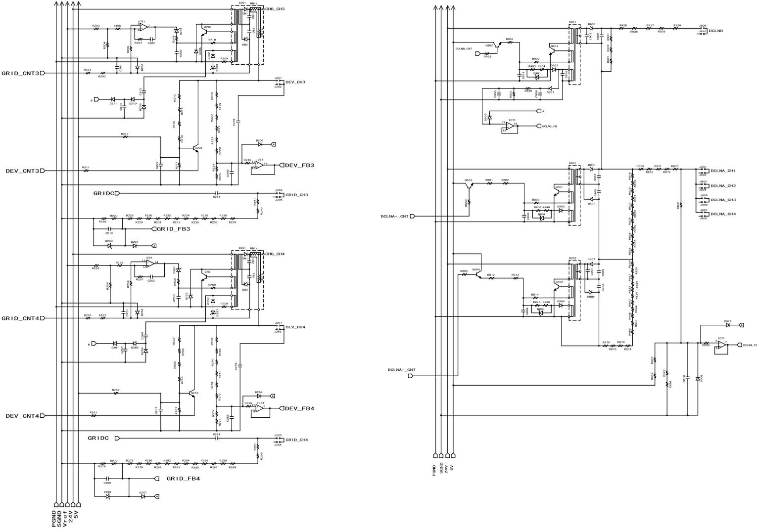
High-voltage Power Supply PCB Circuit Diagram MURATA: MPH3316 (3/3)
