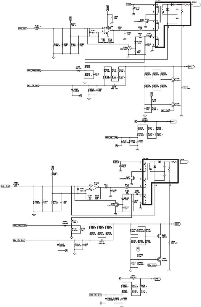
■ High-voltage Power Supply PCB Circuit Diagram SYS HITEK: SPH-8N35 (3/3)
