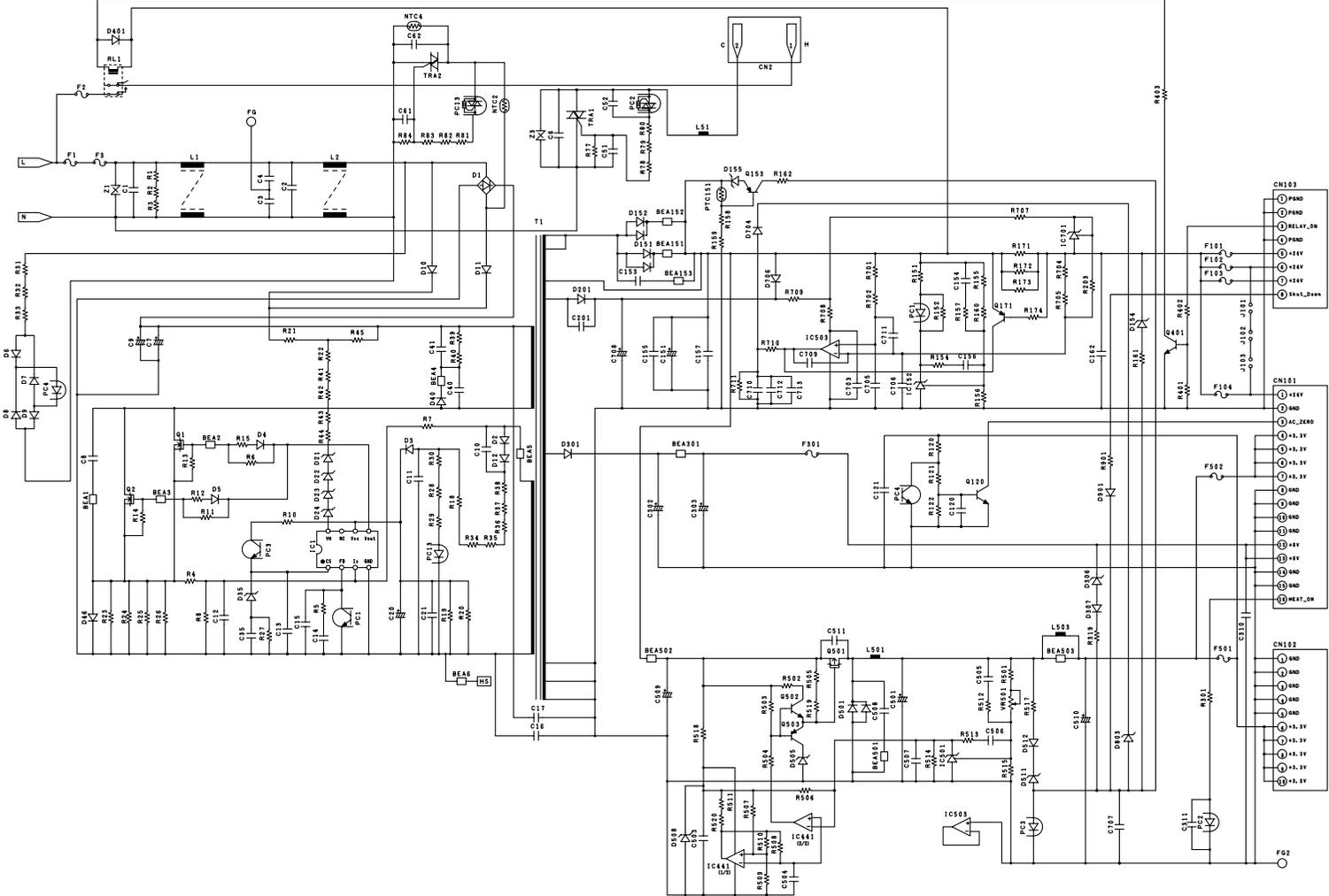
■ Low-voltage Power Supply PCB Circuit Diagram (200V)
