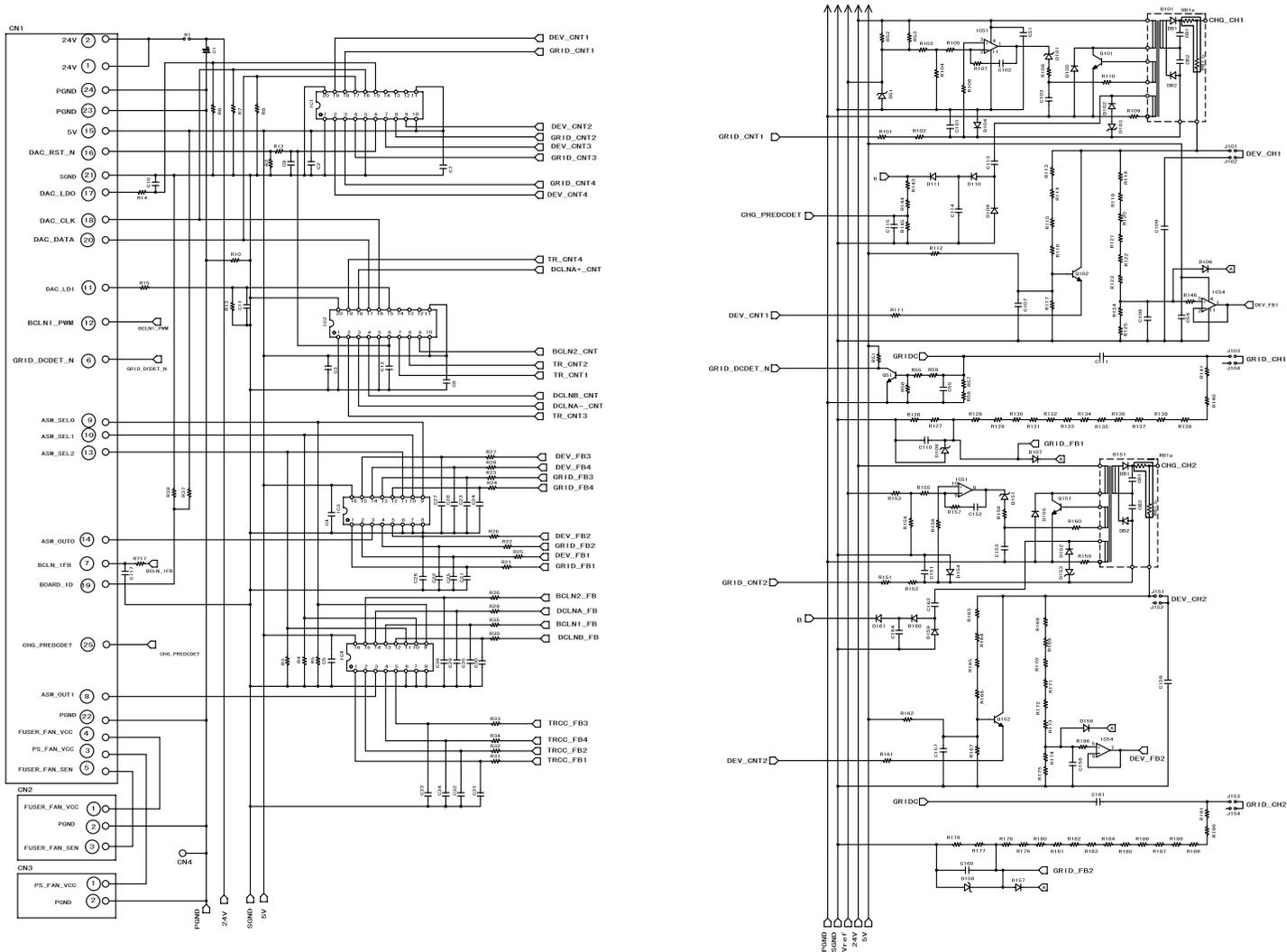
■ High-voltage Power Supply PCB Circuit Diagram MURATA: MPH3316 (2/3)
