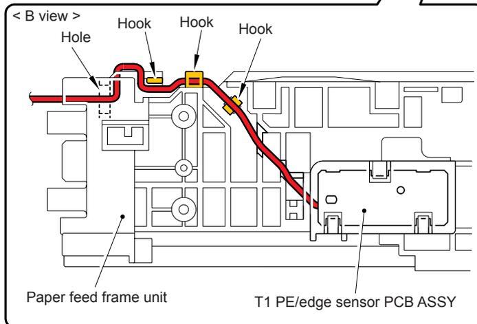
T1 PE/edge sensor PCB ASSY
