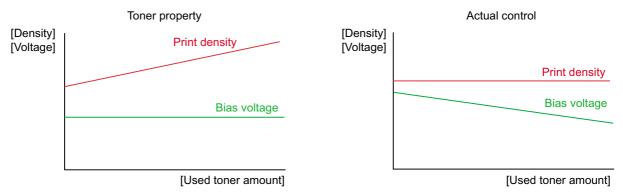
To obtain a print result of a constant density all the time, the printer counts the number of print pages immediately after the toner cartridge is replaced and changes the bias voltage according to the accumulated number of prints with the toner cartridge.
