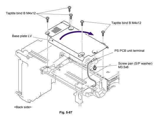
(4) Remove the two bind B M4x12 Taptite screws, and then remove the LV insulation sheet.
