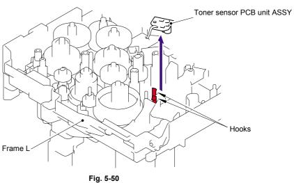
(2) Remove the PT sensor holder from the Toner sensor PCB ASSY AL.
