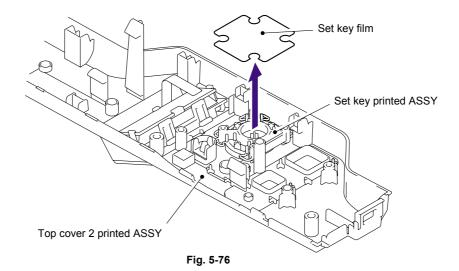
(5) Remove the Set key printed ASSY from the Top cover 2 printed ASSY.
