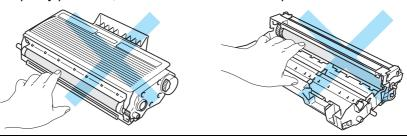
(4) Put the toner cartridge back into the drum unit until you hear it lock into place. If you put the cartridge in properly, the blue lock lever will lift automatically.
