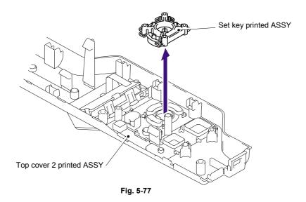
(6) Remove the Key top from the Set key printed ASSY.
