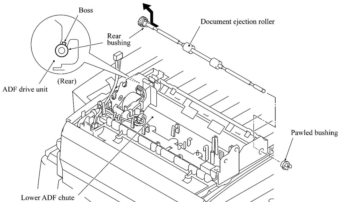
**Reassembling Note:** When fitting the rear bushing of the document ejection roller into the cutout of the ADF drive unit, orient the boss as illustrated on the previous page.
