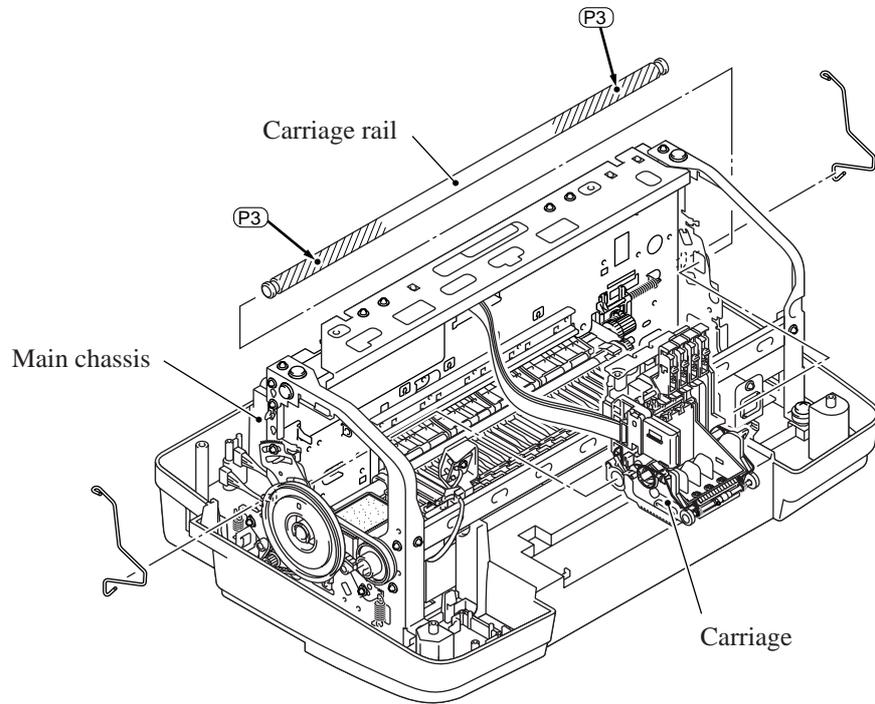
**[ 10 ] Main chassis (slideway of the carriage guide)**
