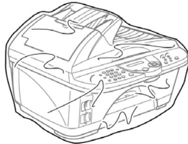
(8) Place the machine in the original box with the original packaging material.
