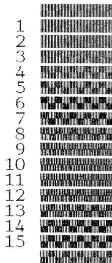
**Head Positioning Test Pattern**
