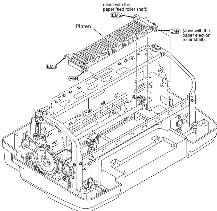
[ 8 ] Paper feed roller, paper ejection roller, and PF roller pulley L
