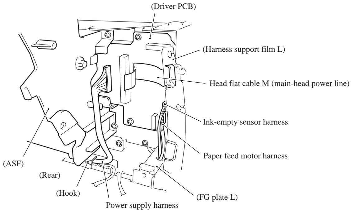
**Harness routing E: Head flat cables, carriage motor harness, speaker harness, power supply harness, NCU harness, ink empty sensor harness, paper feed motor harness, and purge switch harness**
