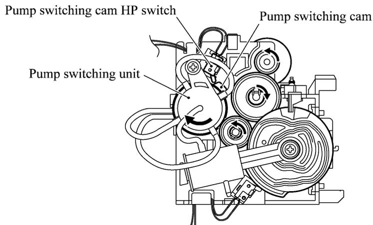
When the paper feed motor rotates clockwise
