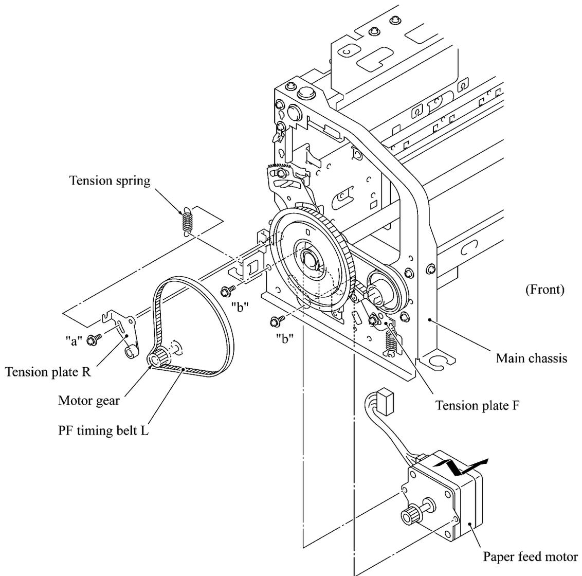
"a" and "b": Screw, pan (s/p washer) M3x6
