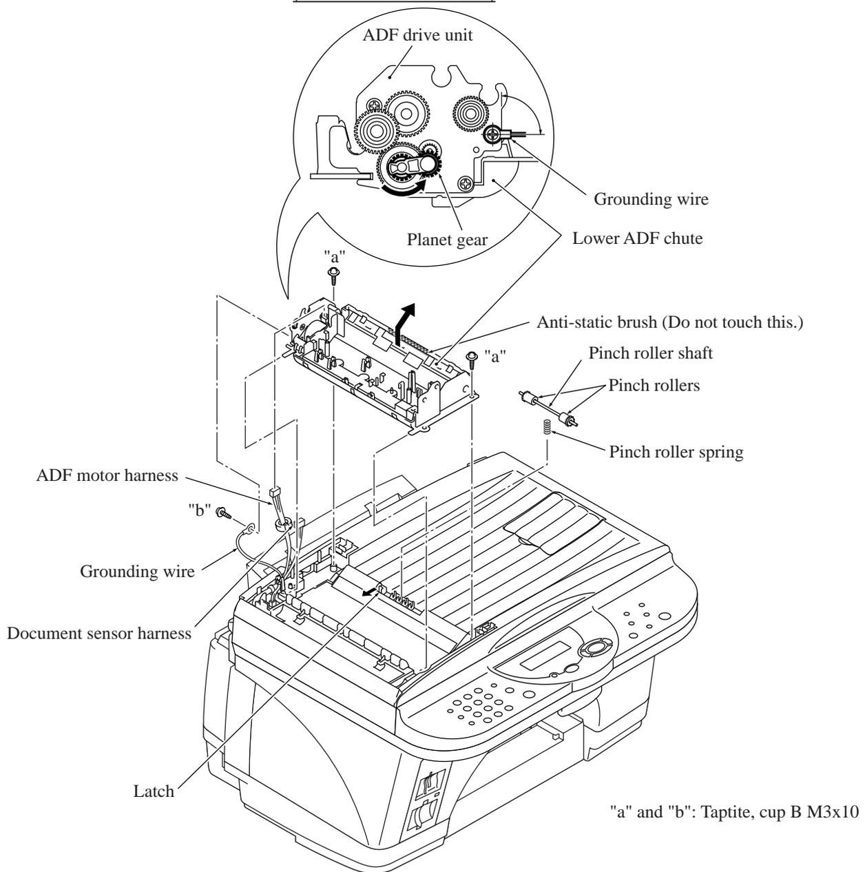
(15) Remove the two screws from the ADF drive unit and release the ADF motor.
