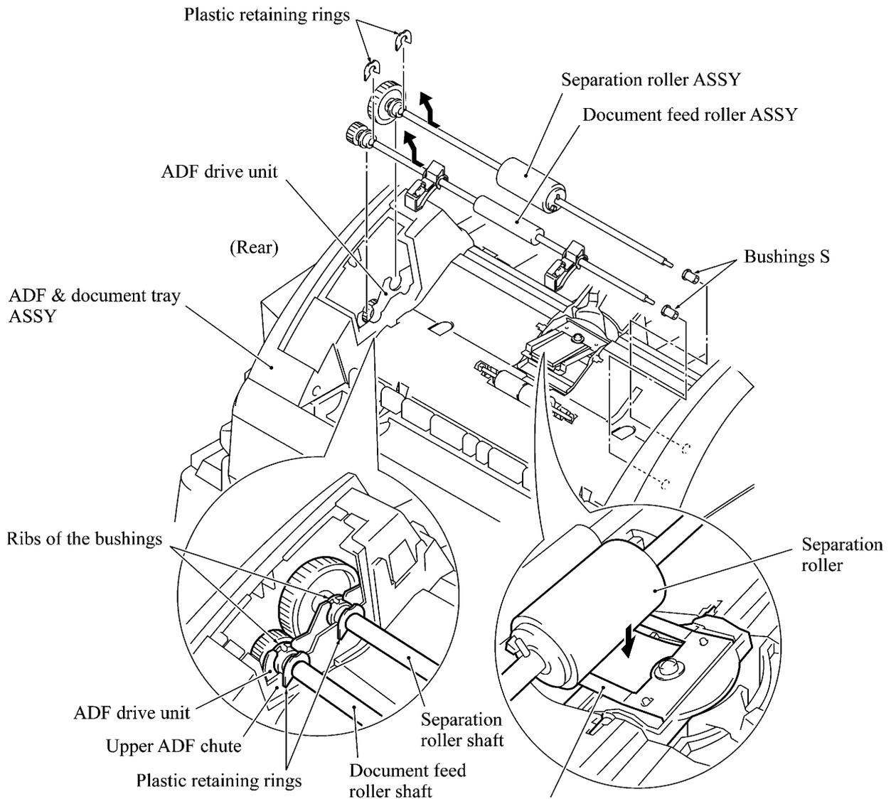
Fitting the bushings into the cutouts provided in the ADF drive unit and setting the plastic retaining rings inside the upper ADF chute
