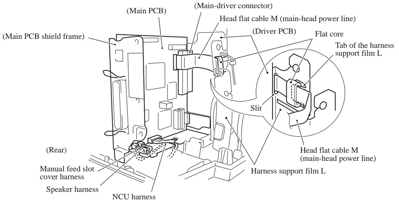
**Harness routing D: Power supply harness, ink-empty harness, paper feed motor harness, and head flat cable M (main-head power line)**
