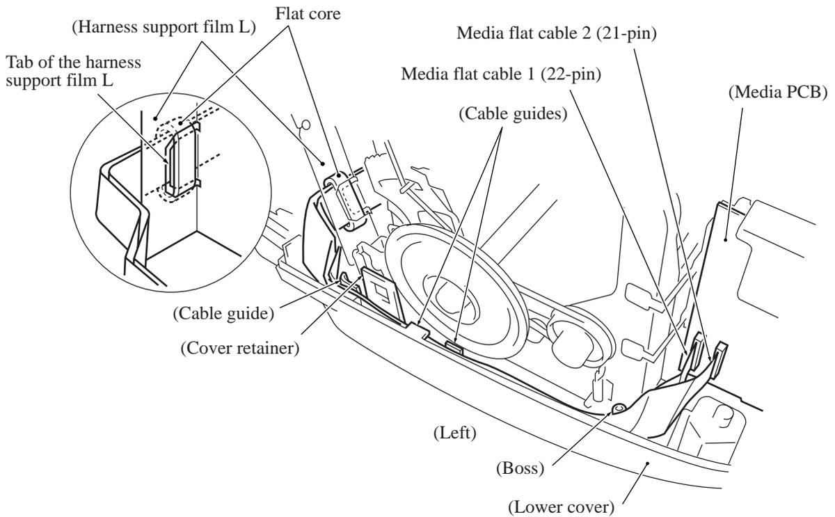
**Harness routing C: Head flat cable M (main-head power line), NCU harness, speaker harness, and manual feed slot cover sensor harness**
