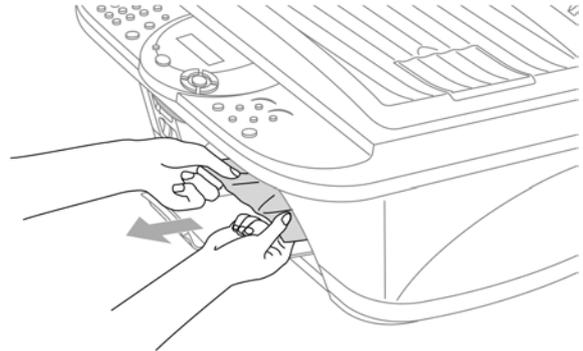
(4) Paper is jammed inside the back of the MFC.
