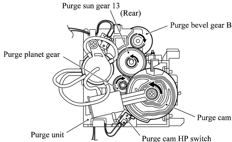
When the paper feed motor rotates counterclockwise
