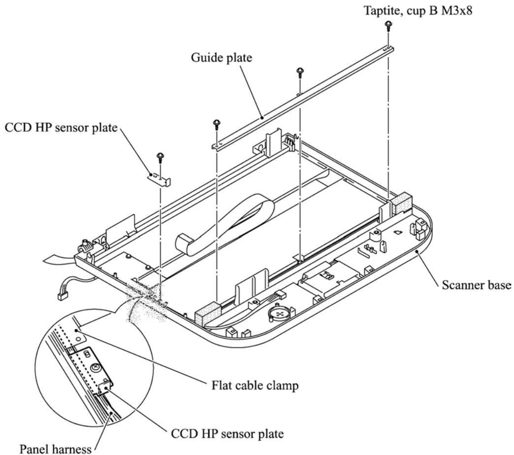
(10) Remove the two screws and take off the flat cable clamp. (See the next page.)
