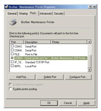
In this example, the port number assigned to the Brother Maintenance USB Printer is USB001.
