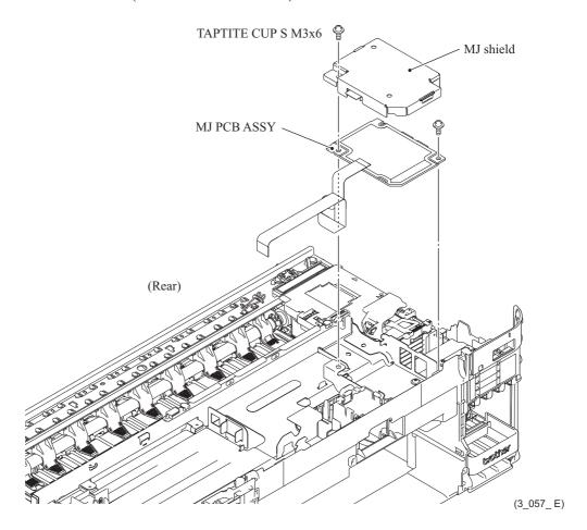
**Assembling Note:** Make sure that two insulation films are sandwiched between the MJ shield and the MJ PCB.
