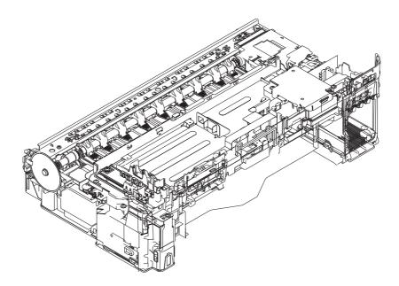
**Assembling Note:** When tightening the right front screw on the main PCB, secure the FG wire together.
