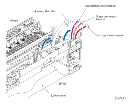
**Assembling Note:** When routing the carriage motor harness, set the ferrite core into the square hole with the cable tie positioned on the top of the ferrite core.
