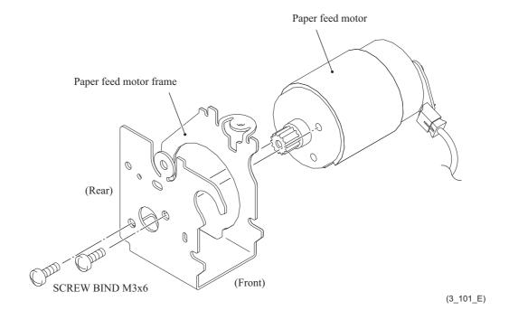
Assembling Note: Mount the paper feed motor on its frame as shown above.
