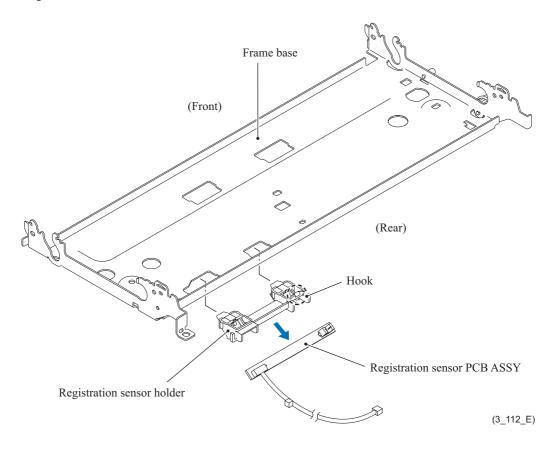
**Assembling Note:** Set the registration sensor PCB ASSY to its holder while pressing the sensor section of registration sensor PCB ASSY.
