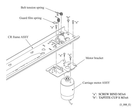
**Assembling Note:** Tighten screw "C" (TAPTITE CUP S M3x6) temporarily. After setting the head/carriage unit and the CR timing belt, tighten screw "C" firmly.
