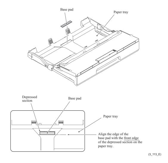
**Assembling Note:** When attaching a new base pad to the paper tray, align the front edge of the pad with that of the depressed section on the paper tray and center the pad widthways as shown above.
