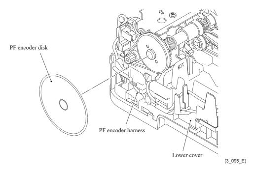
**Note:** Once removed, the PF encoder disk should be replaced with a new one.
