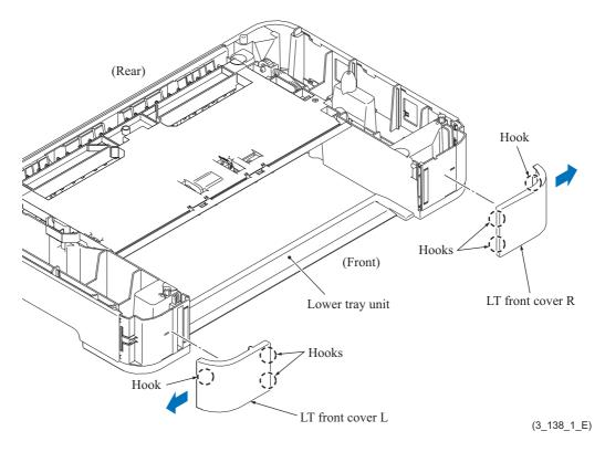
(6) While pulling the LT side cover L to the rear, pull it outwards to release the hooks and remove the LT side cover L.
