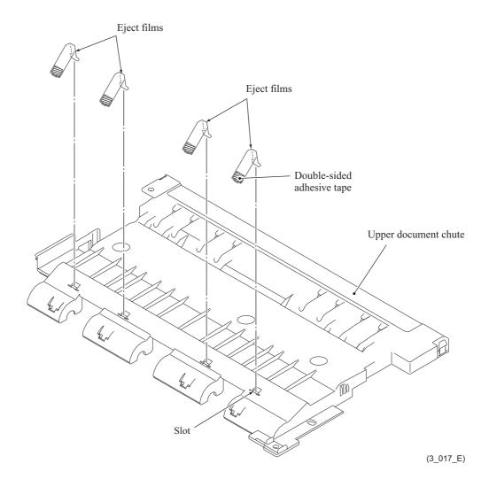
Assembling Note: Once removed, the eject films should be replaced with new ones.
