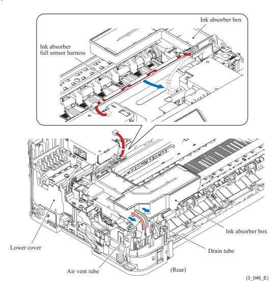
**Note:** Pinch the end of each tube with a clip in order to prevent drained ink from leaking and the machine from getting stained with leaked ink.
