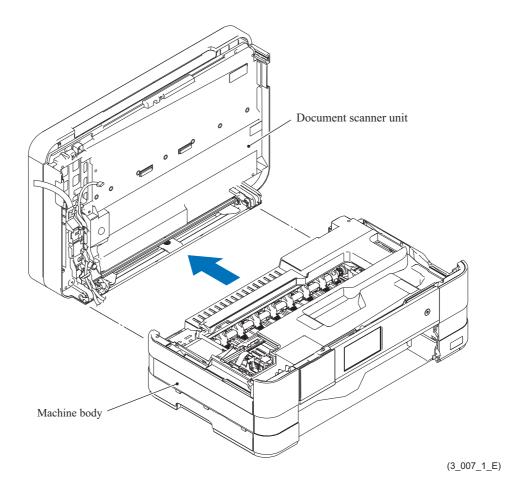
**Assembling Note:** Before routing the document detection/document scanning position sensor harness and the ADF motor harness through the harness holder, put a 20-mm-thick pad on the scanner glass of the document scanner cover. Otherwise, when you scan a thick book on the scanner glass, the ADF unit cannot be closed due to those tense harnesses.
