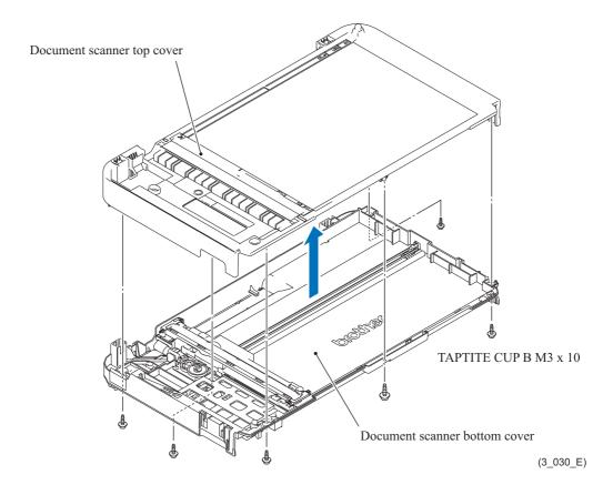
**Assembling Note:** When mounting the document scanner top cover, tighten the left front screw first.
