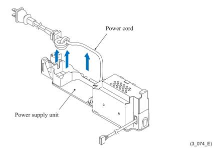
$\underline{\text{For 200 V}}$  Remove the screw (SCREW PAN (WASHER) M4x8D) and remove the power inlet from the power cord holder.
