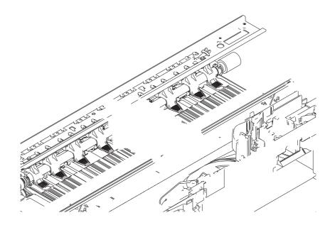
(8) Release the lock spring and hook to remove the carriage PCB ASSY.
