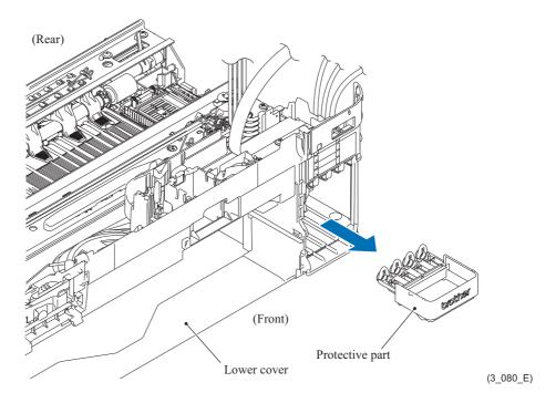
**Note:** To prevent the ink remaining in the ink supply tubes from leaking from the ink supply needle side, keep the head joint side at the same height as the ink supply needles in the ink refill ASSY and perform steps (5) and (6).
