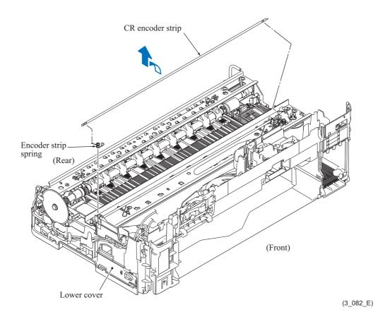
**Assembling Note:** Set the CR encoder strip so that the  $\triangle$ -marked end is to the right (carriage motor side) and the mark  $\triangle$  points upwards.
