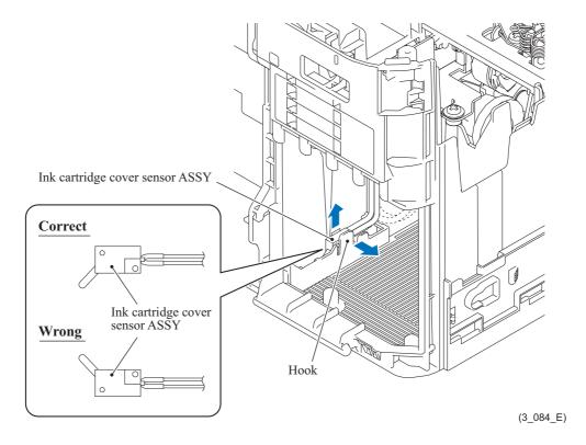
**Assembling Note:** When mounting the ink cartridge cover sensor ASSY, be careful with the mounting direction.
