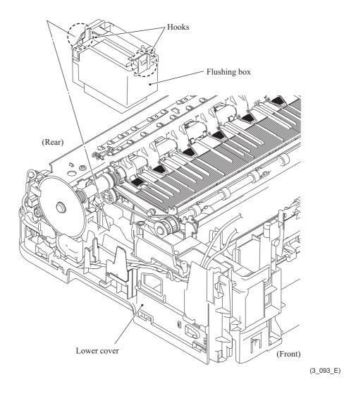
**Assembling Note:** If you replace the flushing box (without replacing the main PCB), reset the flushing count, using the procedure given in Chapter 4, Section 1.14 "Reset purge and flushing counts."
