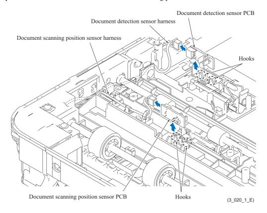
**Assembling Note:** Mount the document detection sensor PCB and the document scanning position sensor PCB to the holders by pressing the sensor section of each PCB.
