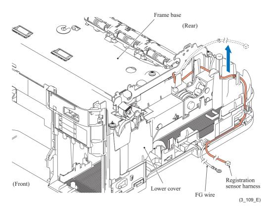
**Assembling Note:** In wiring of the registration sensor harness, set the cable tie on the left side of the rib of the lower cover.
