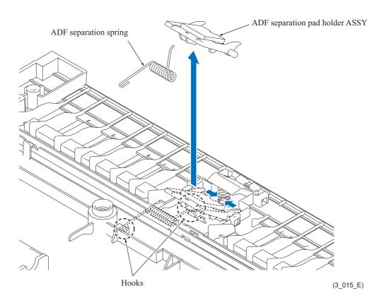
**Assembling Note:** Mount the ADF separation spring and the ADF separation pad holder ASSY to the ADF unit, then hook the other end of the spring on the ADF unit.
