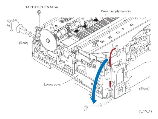
(3) Release the hook and remove the power supply unit from the bottom of the lower cover.
