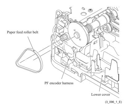
**Assembling Note:** When setting the paper feed roller belt, first fit it over the motor gear and then over the paper feed roller shaft.
