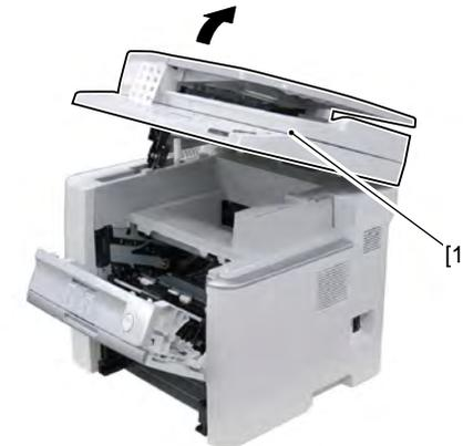
3. Remove the claw [1] and remove the reader shaft retainer [2].
