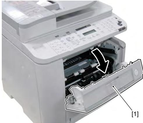
2. Open the pickup roller cover [1], move the roller holder [2] in the direction of the arrow and remove the manual pickup roller [3].
