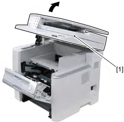
5. Remove the reader support shaft [1] and open the reader unit [2].
