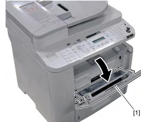
2. Lower the manual guide [1], insert the precision flat-screwdriver into the clearance [2] of the separation pad and displace it in the direction of the arrow.
