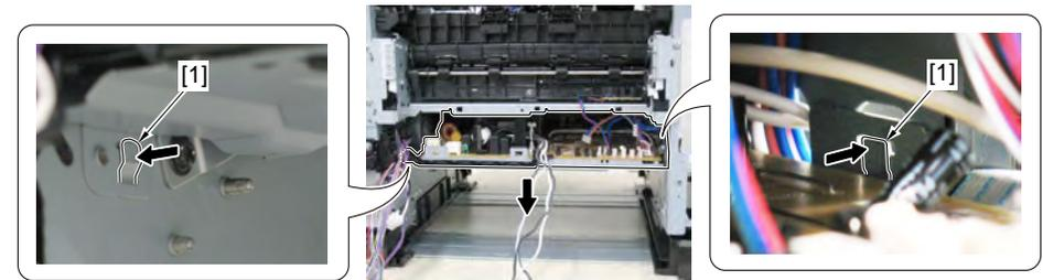
22. While pulling out the flat cable [1] and the harness [2] from the hole of the host machine, remove the engine controller unit [3].
