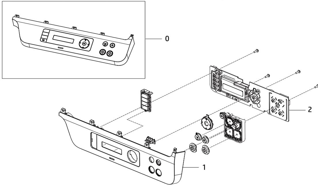
Table 2-5 Control panel assembly (HP Color Laser MFP 178nw,178nwg)
