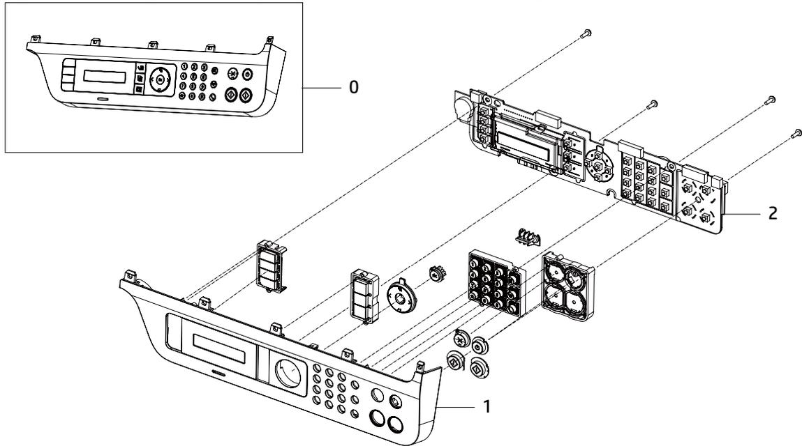
Table 2-6 Control panel assembly (HP Color Laser MFP 179fnw,179fwg)
