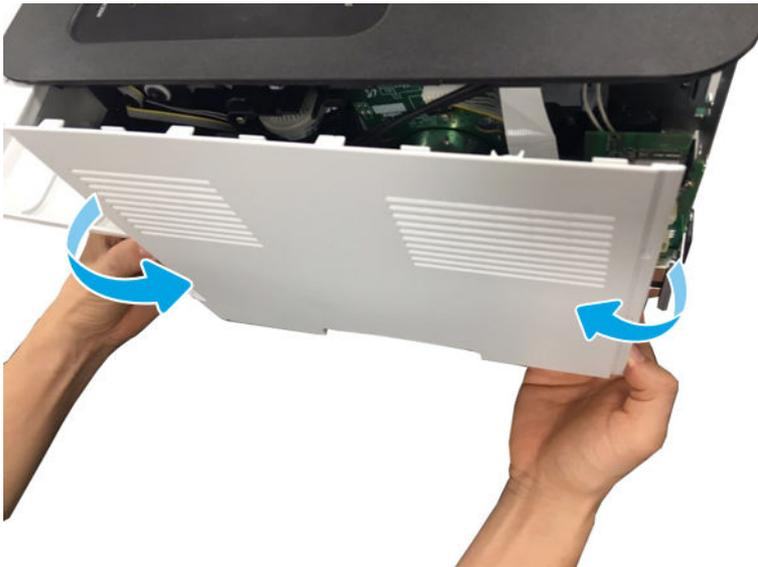
3. Remove the Flabled scanner assembly unit.
