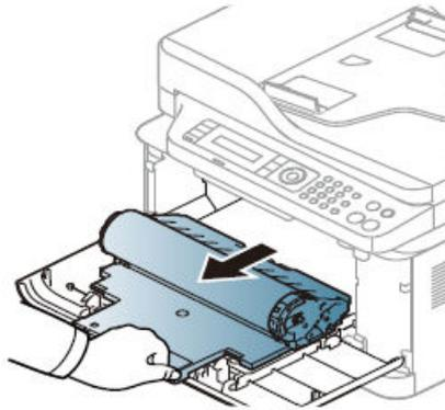
2. Unpack a replacement imaging unit and then insert imaging unit.
