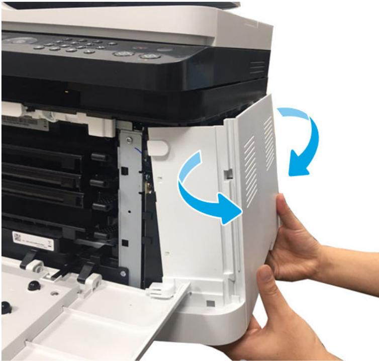
3. Remove the Flabed scanner assembly unit.
