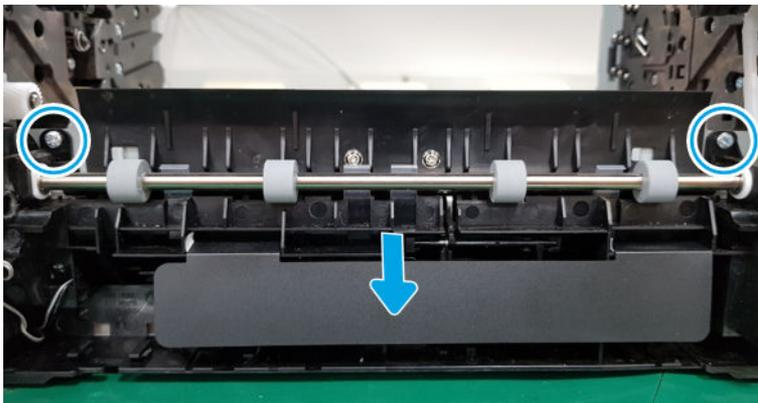
7. Remove Regi clutch and Pick up solenoid.
