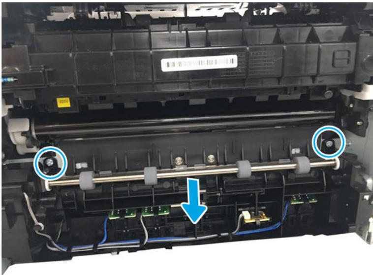
8. Remove Regi clutch and Pick up solenoid.
