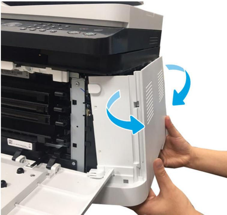
3. Remove the Flaped scanner assembly.
