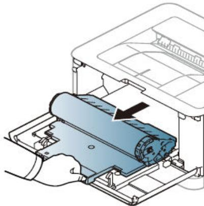
2. Unpack a replacement imaging unit and then insert imaging unit.
