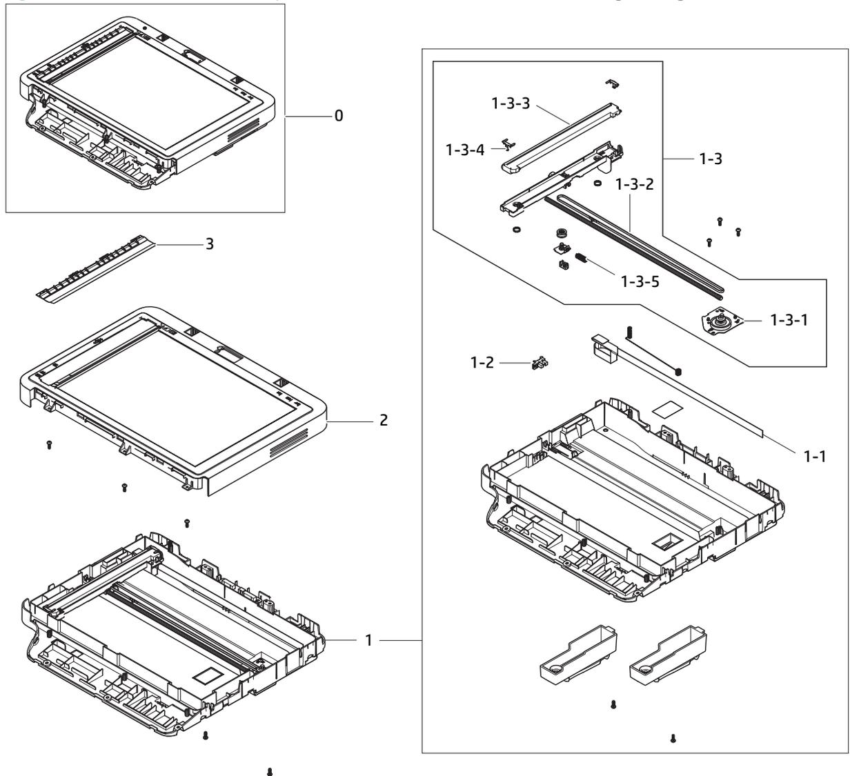
Table 2-8 Flatbed scanner assembly (HP Color Laser MFP 178nw, 179fnw,178nwg,179fwg)
