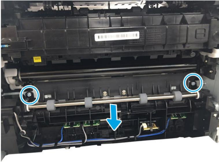
8. Remove the Empty sensor PCA and Paper size sensor PCA.
