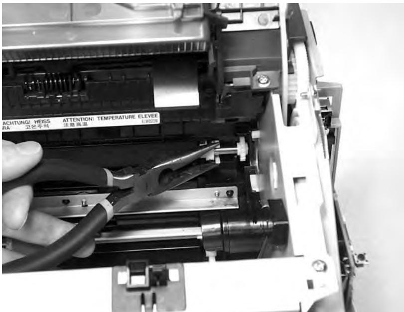
Figure 5-22 Remove the transfer roller (3 of 3)
