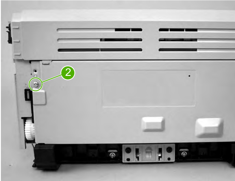
Figure 5-12 Remove the rear panel and top-cover assembly (4 of 6; HP LJ 1020 printer shown)
