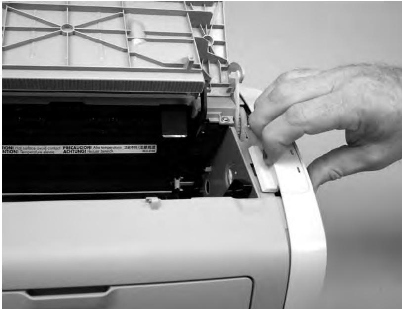
Figure 5-7 Remove the right-side cover (3 of 4; HP LJ 1020 printer shown)
