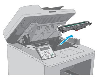
6. Remove any jammed paper from the toner-cartridge area. Use both hands to remove jammed paper to avoid tearing the paper.
