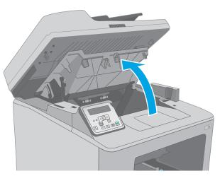
**3.** Remove the toner cartridge from the printer.
