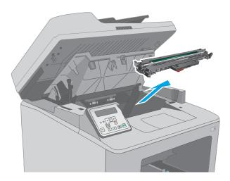
Remove any jammed paper from the toner-cartridge area. Use both hands to remove jammed paper to avoid tearing the paper.
