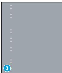
Position a metric ruler on the page with the "zero" ruler mark at one occurrence of the defect (callout 1). 2.
