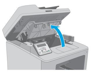
4. Remove the toner cartridge from the printer.
