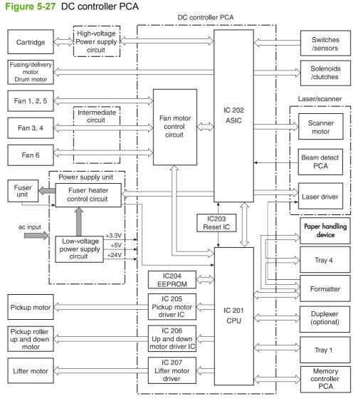
The DC controller PCA manages the operational sequences of the product. The following table lists the DC controller components and their functions.
