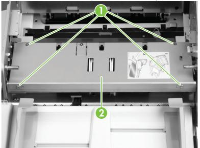
Figure 6-105 Remove the separation belt assembly (1 of 6)
