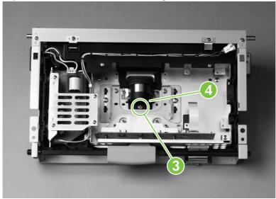
Figure 6-62 Remove the ADF shading filter (2 of 2)
