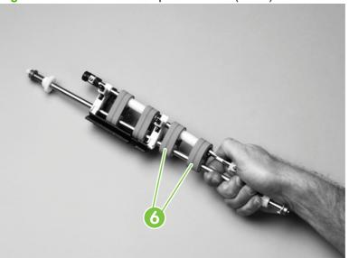
Figure 6-113 Remove the separation belts (3 of 3)
