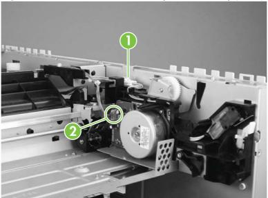
Figure 6-197 Remove the fuser delivery-drive assembly (1 of 3)
