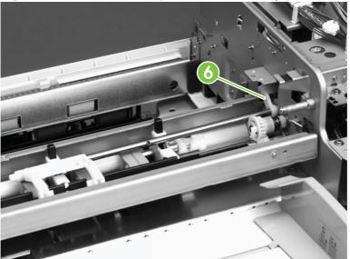
Figure 6-108 Remove the separation belt assembly (4 of 6)
