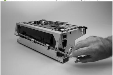
Figure 6-54 Remove the ADF optical assembly (9 of 13)
