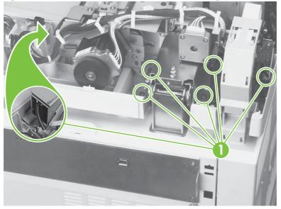
Figure 6-27 Remove the ADF base cover assembly (1 of 7)
