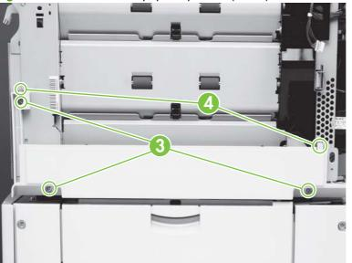
Figure 6-163 Remove the paper-input unit (3 of 5)
