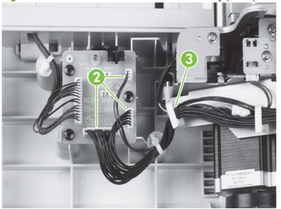
Figure 6-28 Remove the ADF base cover assembly (2 of 7)
