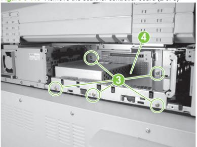
Figure 6-119 Remove the scanner controller board (2 of 5)
