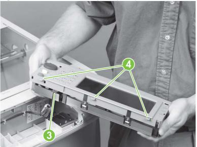
Figure 6-5 Remove the control panel (3 of 3)
