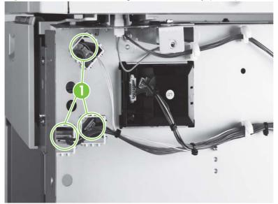
Figure 6-205 Remove the registration assembly (1 of 2)
