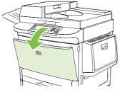
6. Check for paper in the duplex printing accessory area, and remove any paper by pulling it out of the product. Be careful not to tear the paper.
