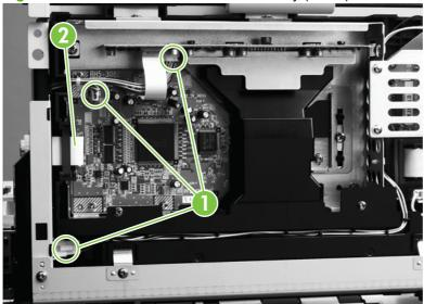
Figure 6-38 Remove the ADF main assembly (1 of 8)
