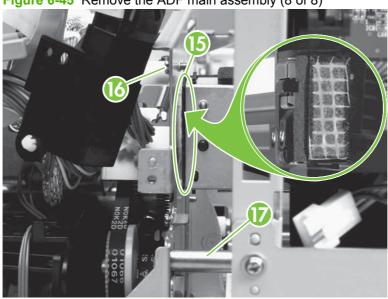
Figure 6-45 Remove the ADF main assembly (8 of 8)
