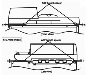
4. If the gap is not within specifications, loosen the fixing nut and turn the two ADF height adjust screws. Turn the screws clockwise (CW) to increase the gap, or counterclockwise (CCW) to decrease the gap.
