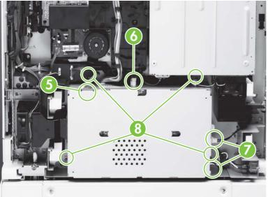
Figure 6-177 Remove the low-voltage power supply (3 of 3)
