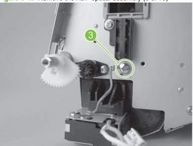
Figure 6-48 Remove the ADF optical assembly (3 of 13)
