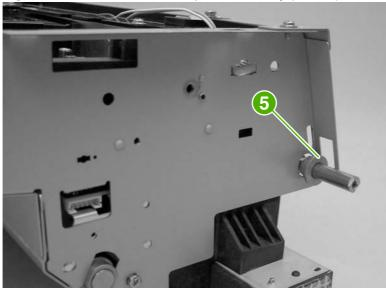
Figure 6-53 Remove the ADF optical assembly (8 of 13)
