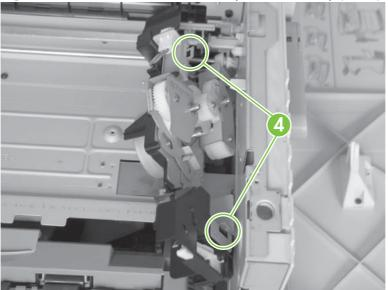
Figure 6-199 Remove the fuser delivery-drive assembly (3 of 3)
