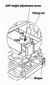
**NOTE:** Each rotation of the screw increases or decreases the gap by 0.7 mm (0.03 inch).
