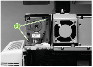
Figure 6-78 Remove the flatbed motor (2 of 3)
