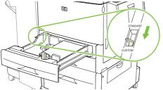
8. Close the tray. The product control panel might show the tray media type and size. If the configuration is not correct, touch Modify on the control panel. If the configuration is correct, touch OK.
