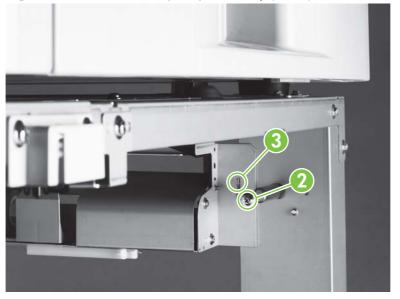
4. Lift the pickup assembly off the hook (callout 3) to remove it.
