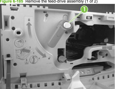
Figure 6-185 Remove the feed-drive assembly (1 of 2)
