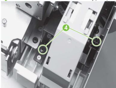
Figure 6-29 Remove the ADF base cover assembly (3 of 7)
