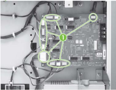
Figure 6-209 Remove the controller board (1 of 2)
