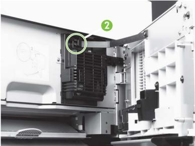
Figure 6-189 Remove the cartridge fan (2 of 4)
