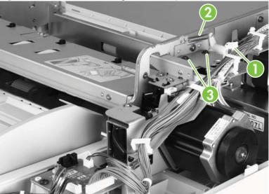
Figure 6-71 Remove the weight solenoid (2 of 2)
