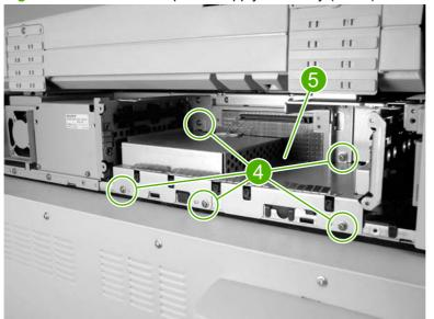
Figure 6-82 Remove the power supply assembly (3 of 6)
