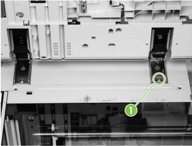
Figure 7-13 The bracket fixing screw
