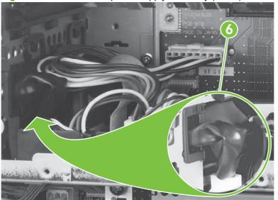
Figure 6-83 Remove the power supply assembly (4 of 6)
