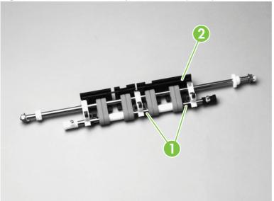
Figure 6-111 Remove the separation belts (1 of 3)
