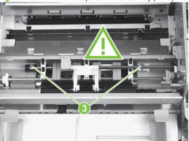
Figure 6-106 Remove the separation belt assembly (2 of 6)
