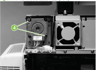
Figure 6-79 Remove the flatbed motor (3 of 3)
