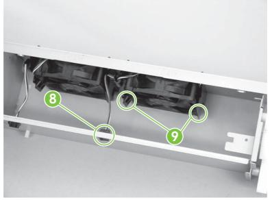
Figure 6-137 Remove the delivery fan assembly (5 of 5)
