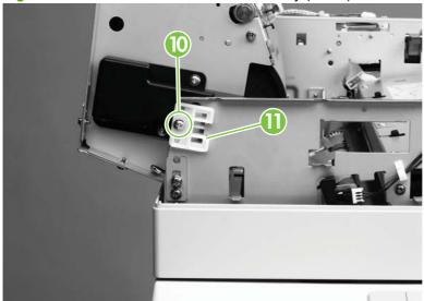
Figure 6-42 Remove the ADF main assembly (5 of 8)
