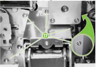
Figure 6-97 Remove the lower registration roller assembly (7 of 11)
