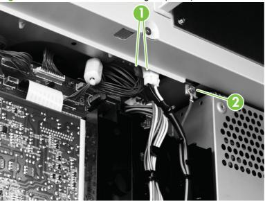
Figure 6-124 Remove the scan engine (1 of 7)
