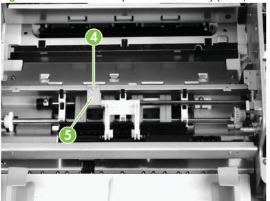
Figure 6-107 Remove the separation belt assembly (3 of 6)
