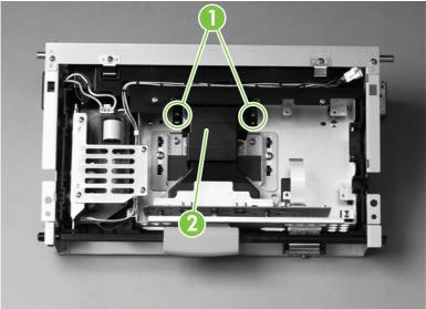
Figure 6-61 Remove the ADF shading filter (1 of 2)
