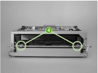
9. Slide the springs to the center of the shaft until they stop.
