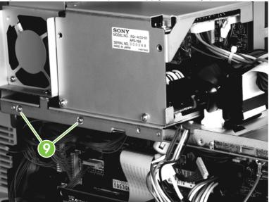
Figure 6-85 Remove the power supply assembly (6 of 6)
