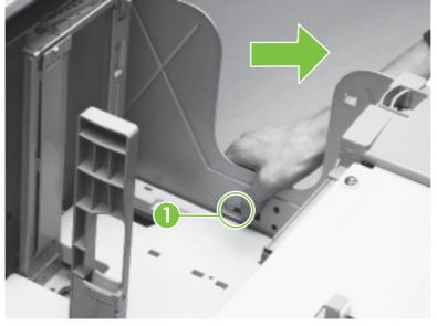
3. Continue to press the two release buttons while pulling the tray out to remove it.
