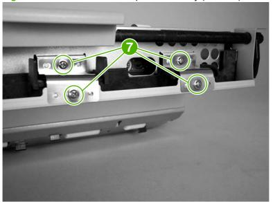
Figure 6-56 Remove the ADF optical assembly (11 of 13)
