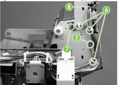
Figure 6-40 Remove the ADF main assembly (3 of 8)
