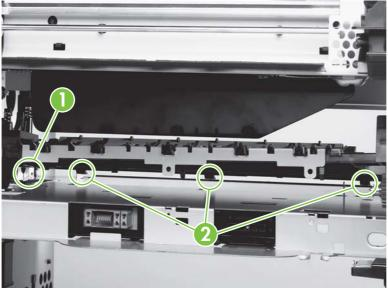
2. Rotate the transfer guide assembly upward, and slide the three back tabs (callout 2) into place.
