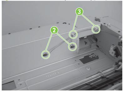
Figure 6-134 Remove the delivery fan assembly (2 of 5)
