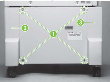
Callout 1 shows the screws to remove for removal of the center back cover.
