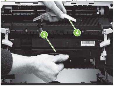
Figure 6-173 Remove the fuser assembly (2 of 2)
