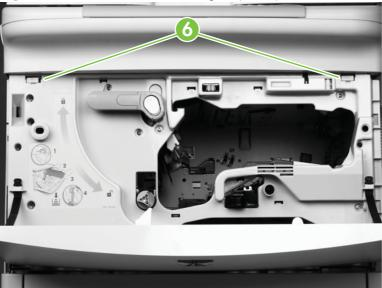
Figure 6-128 Remove the scan engine (5 of 7)
