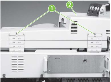
Figure 6-11 Remove the ADF back cover (1 of 2)
