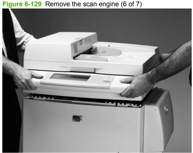
NOTE: As you remove the scan engine assembly, two black plastic spacer rings (see figure) fall into the top of the print engine under the rear alignment holes. These rings cannot be reinstalled, but removing them is recommended to ensure that they do not interfere with printing operations.
