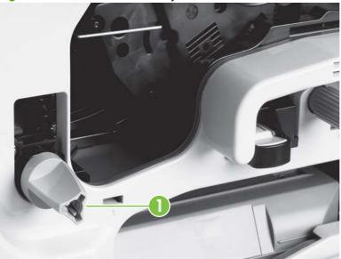
Figure 6-157 Remove the fuser-jam-removal knob
