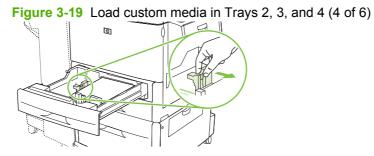
7. Adjust the front (X) paper guide by pressing the tab on the guide, and slide the guide until it gently touches the paper.
