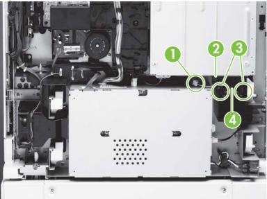
Figure 6-192 Remove the controller fan
