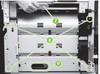
Figure 6-165 Remove the paper-input unit (5 of 5)
