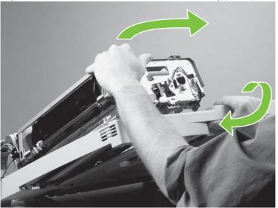
Figure 6-33 Remove the ADF base cover assembly (7 of 7)
