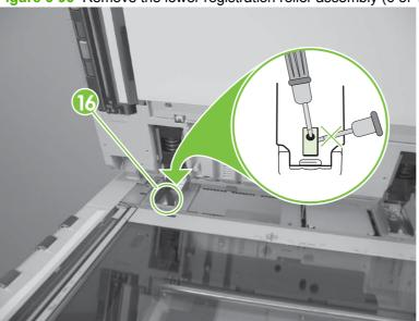
Figure 6-96 Remove the lower registration roller assembly (6 of 11)
