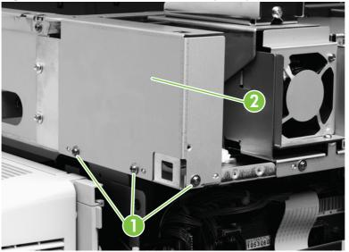
Figure 6-77 Remove the flatbed motor (1 of 3)
