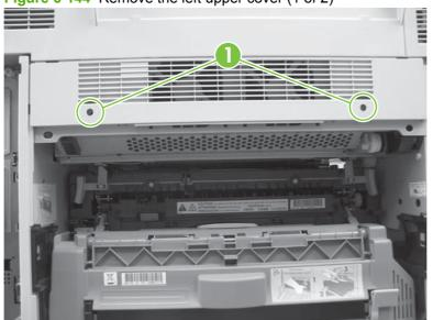
Figure 6-144 Remove the left upper cover (1 of 2)
