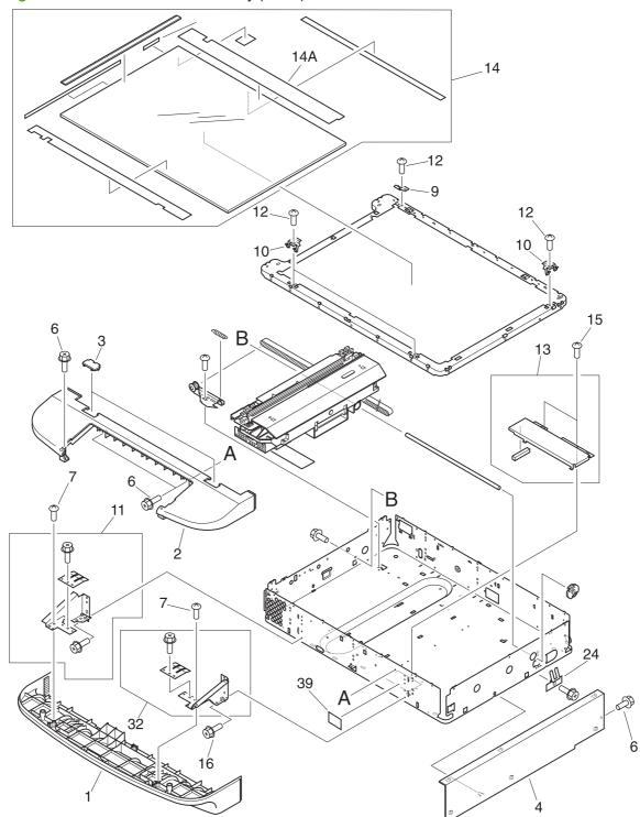
Figure 8-7 Flatbed scanner assembly (2 of 3)
