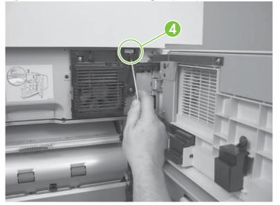
Figure 6-126 Remove the scan engine (3 of 7)
