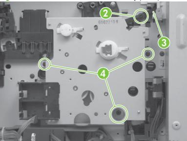
Figure 6-186 Remove the feed-drive assembly (2 of 2)
