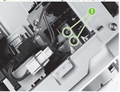
Figure 6-151 Remove the cartridge release lever (2 of 3)
