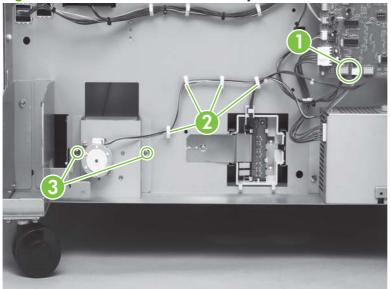
3. Carefully unwind the cable from the cable guides (callout 2).
