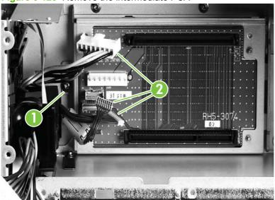
Figure 6-123 Remove the intermediate PCA
