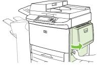
2. Check for media in the right door area, and remove any media from this area. Carefully check to be sure you have removed all pieces of torn media.
