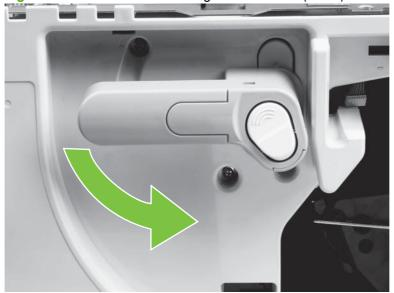
Figure 6-150 Remove the cartridge release lever (1 of 3)
