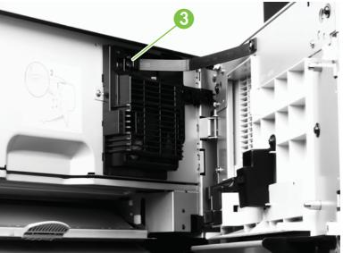
Figure 6-125 Remove the scan engine (2 of 7)
