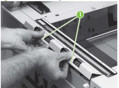
Figure 6-14 Remove the delivery roller cover
