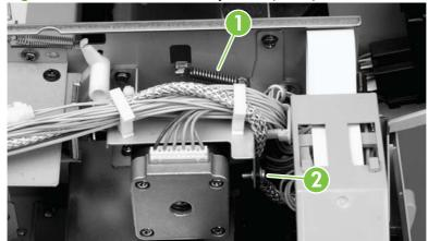
3. Remove one cable clamp screw (callout 2) and the cable clamp.
