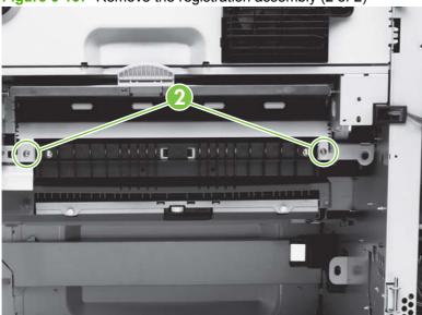
Figure 6-167 Remove the registration assembly (2 of 2)
