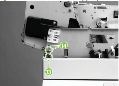
**Figure 6-44** Remove the ADF main assembly (7 of 8)
