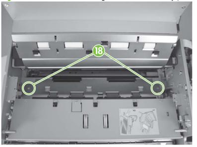
Figure 6-98 Remove the lower registration roller assembly (8 of 11)
