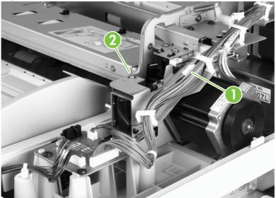
Figure 6-72 Remove the shutter solenoid
