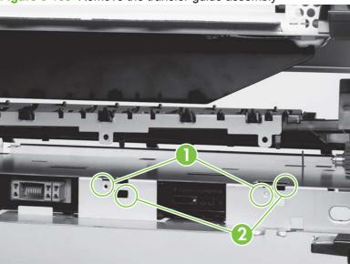
Figure 6-168 Remove the transfer-guide assembly
