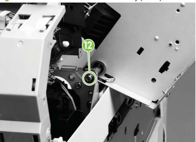
Figure 6-43 Remove the ADF main assembly (6 of 8)
