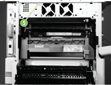
Figure 6-127 Remove the scan engine (4 of 7)
