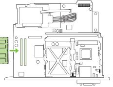
Figure 4-28 Install DDR memory DIMMs (6 of 8)
