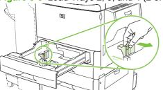
3. Adjust the front (X) paper guide by pressing the tab on the guide, and set the guide to the correct paper size.
