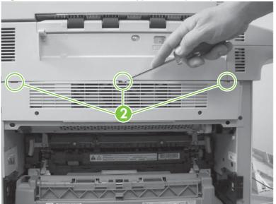
**Figure 6-145** Remove the left upper cover (2 of 2)
