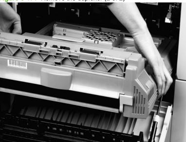
Figure 6-171 Remove the duplexer (2 of 2)
