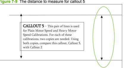
7. Record the difference in line spacing in a copy of the following table.
