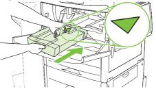
5. Rotate the green handle into the locked position.
