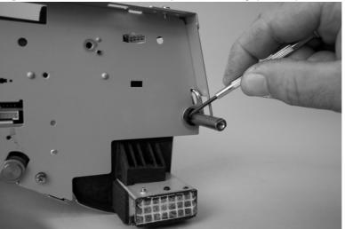
8. Remove the two spring retention screws (callout 4).
