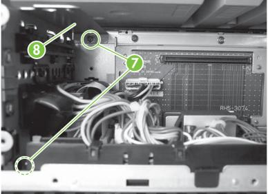
Figure 6-84 Remove the power supply assembly (5 of 6)
