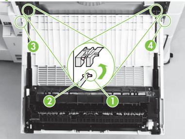
Figure 6-146 Remove the left door and diverter
