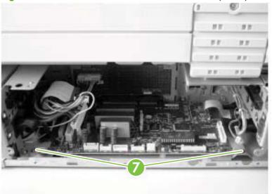
Figure 6-121 Remove the scanner controller board (4 of 5)
