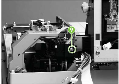
**12.** Slide the flatbed cable cover away from the optical unit to remove it.
