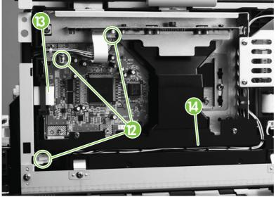
Figure 6-94 Remove the lower registration roller assembly (4 of 11)
