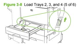
6. Close the tray. The product control panel might show the tray media type and size. If the configuration is not correct, touch Modify on the control panel. If the configuration is correct, touch OK.
