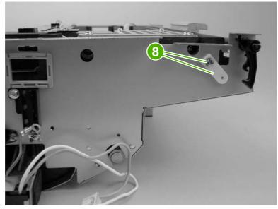
15. Remove the ADF optical assembly from the sheet metal chassis.
