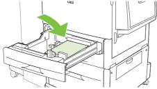
5. Adjust the left paper guide by pressing the tab on the guide, and slide the guide until it gently touches the paper.
