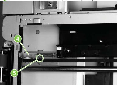
Figure 6-65 Remove the flatbed optical unit (3 of 6)
