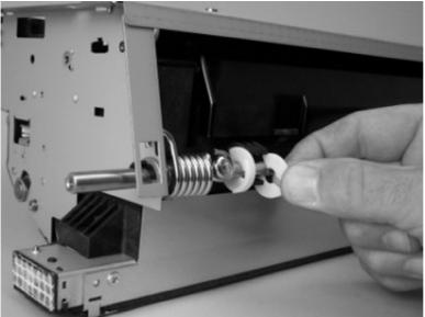
7. Remove the black E-ring from the shaft. Use a small screwdriver to pry it out.
