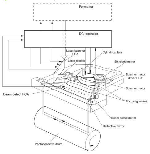
Figure 5-30 Laser/scanner system
