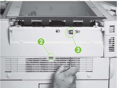
Figure 6-24 Remove the flatbed left cover (2 of 2)
