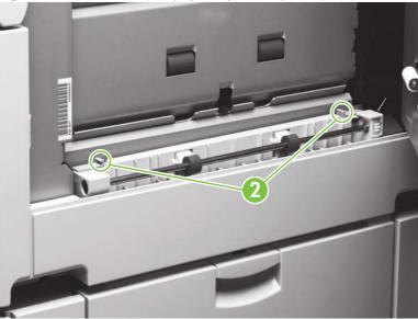
Figure 6-162 Remove the paper-input unit (2 of 5)
