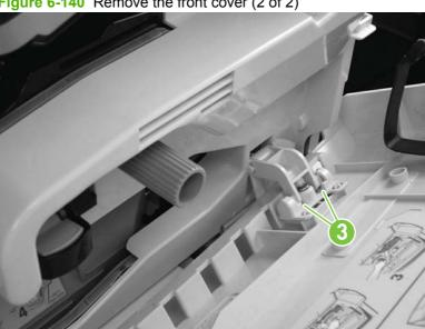
Figure 6-140 Remove the front cover (2 of 2)
