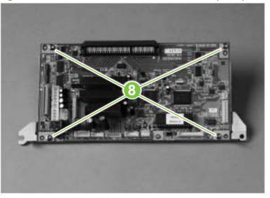
Figure 6-122 Remove the scanner controller board (5 of 5)
