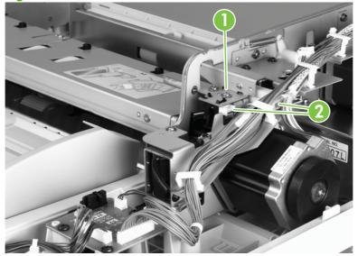
Figure 6-69 Remove the feeder cover detection switch
