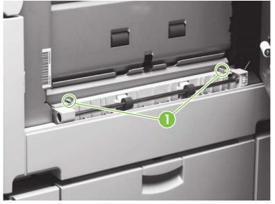
Figure 6-216 Remove the paper-connecting unit
