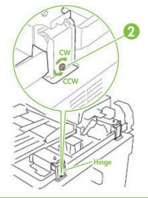
**NOTE:** The skew adjusts 0.7 mm (0.03 inch) with each rotation of the ADF skew adjusting screw.
