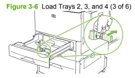
4. Load (orient) the paper according to size.
