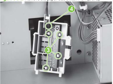
Figure 6-212 Remove the paper-size switch PCA (2 of 2)
