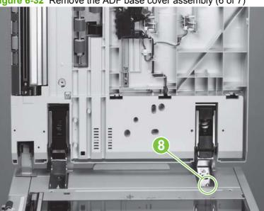
Figure 6-32 Remove the ADF base cover assembly (6 of 7)
