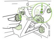
**4.** Turn the small green knob at the top of the stapler unit clockwise until the staple cartridge moves to the left of the stapler unit.
