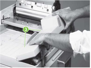
Figure 6-12 Remove the ADF back cover (2 of 2)
