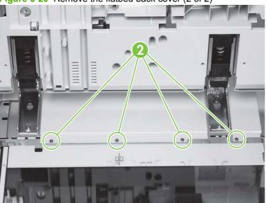
Figure 6-20 Remove the flatbed back cover (2 of 2)
