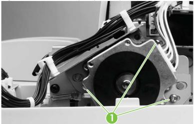
3. Slide the motor to the right to relieve the belt tension, and then tighten the three motor mount screws.
