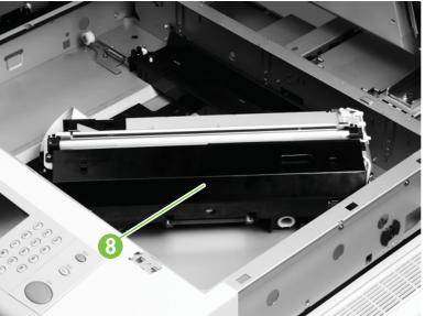
Figure 6-68 Remove the flatbed optical unit (6 of 6)
