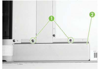
Figure 6-63 Remove the flatbed optical unit (1 of 6)
