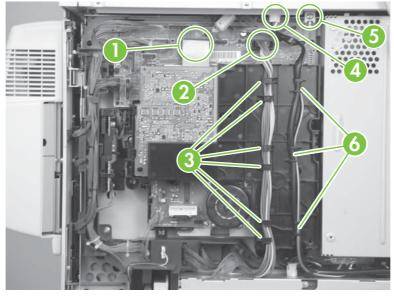
Figure 6-178 Remove the high-voltage power supply (1 of 2)
