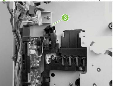
Figure 6-183 Reinstall the toner-sensor contact assembly
