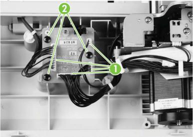
Figure 6-114 Remove the ADF intermediate PCA
