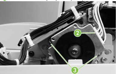
Figure 6-74 Remove the pickup motor (2 of 2)
