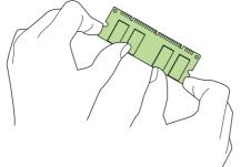
7. Press the DIMM straight into the slot (press firmly). Make sure the locks on each side of the DIMM snap inward into place. (To remove a DIMM, the locks must be released.)
