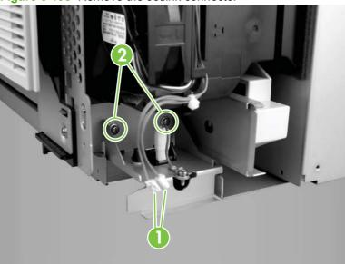
Figure 6-193 Remove the Jetlink connector
