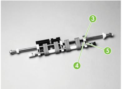
Figure 6-112 Remove the separation belts (2 of 3)
