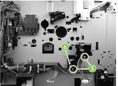
Figure 6-196 Remove the duplexer connector holder assembly (3 of 3)
