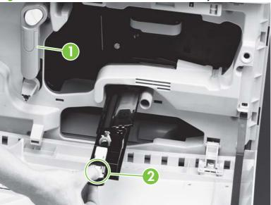
Figure 6-154 Remove the transfer-roller assembly
