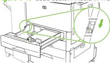
6. Adjust the left (Y) paper guide by pressing the tab on the guide, and slide the guide until it gently touches the paper.
