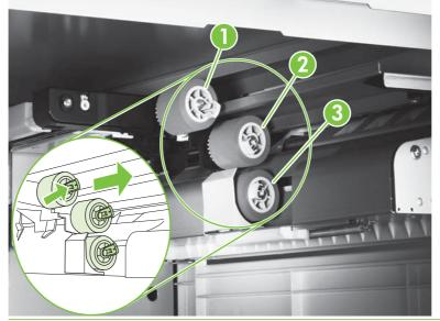
Figure 6-204 Remove the Tray 4 rollers
