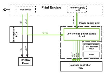
NOTE: When the control panel backlight is off, the +5V line is being signaled off at the control panel assembly by the control panel controller board. SPON is the scanner power-on signal sent to the scan engine power supply when the product is powered on by pressing the power switch on the print engine. See Low-voltage power supply on page 131.
