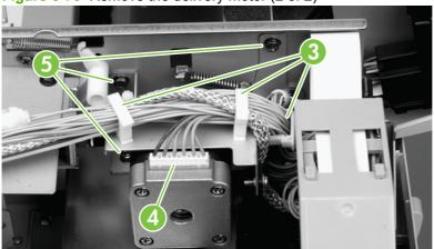
Figure 6-76 Remove the delivery motor (2 of 2)
