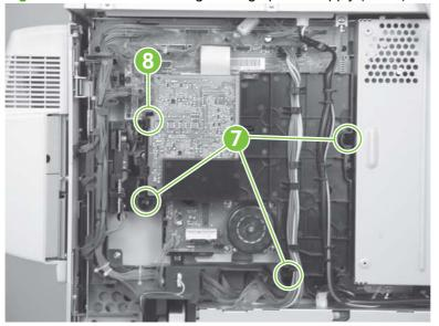
Figure 6-179 Remove the high-voltage power supply (2 of 2)
