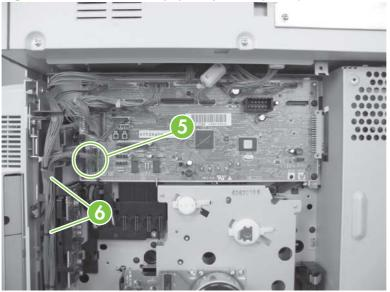
Figure 6-164 Remove the paper-input unit (4 of 5)
