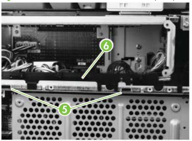
**Figure 6-120** Remove the scanner controller board (3 of 5)
