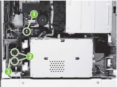
Figure 6-187 Remove the power-supply fan
