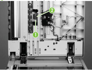
Figure 6-88 Remove the pickup roller (D roller)
