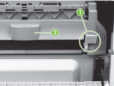
Figure 6-170 Remove the duplexer (1 of 2)
