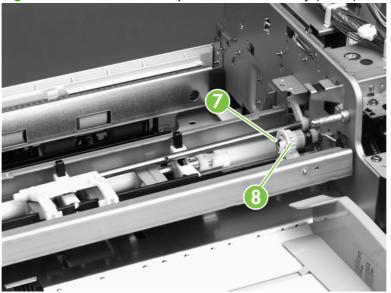
Figure 6-109 Remove the separation belt assembly (5 of 6)
