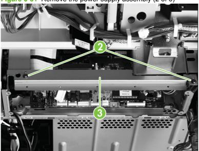
Figure 6-81 Remove the power supply assembly (2 of 6)
