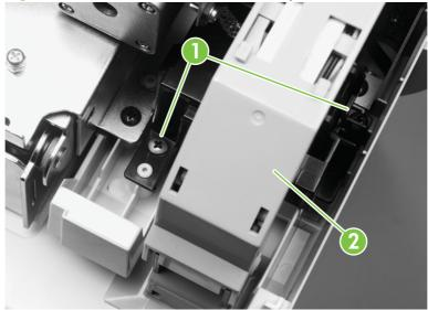
Figure 6-86 Remove the ADF fan assembly
