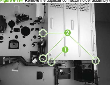
Figure 6-194 Remove the duplexer connector holder assembly (1 of 3)
