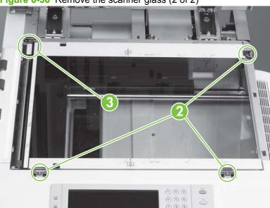
Figure 6-36 Remove the scanner glass (2 of 2)
