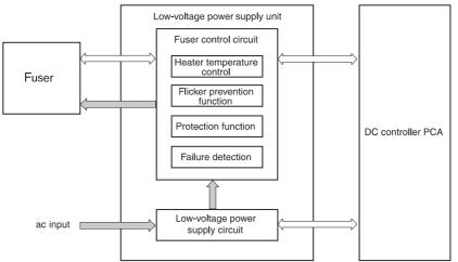
Figure 5-29 Low-voltage power supply
