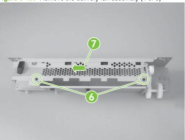
Figure 6-136 Remove the delivery fan assembly (4 of 5)
