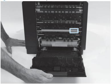
Run the product so that it performs a wipe, and then see if the web has advanced. If it has not, replace the print mechanism.
