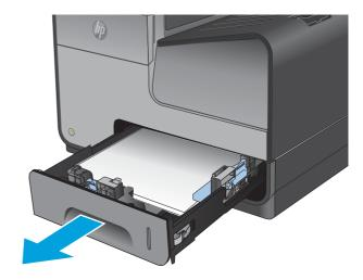
Remove the jammed sheet by pulling it to the right and then out of the product.
