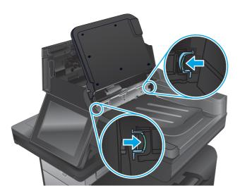
Flow models only: Remove the e-Duplex assembly by pulling it out.
