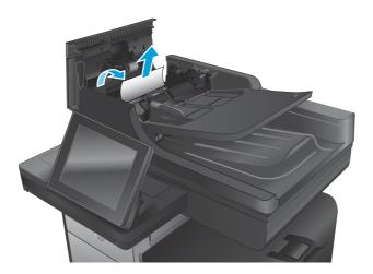
Press on the door next to the document-feeder rollers to make sure it is closed completely.
