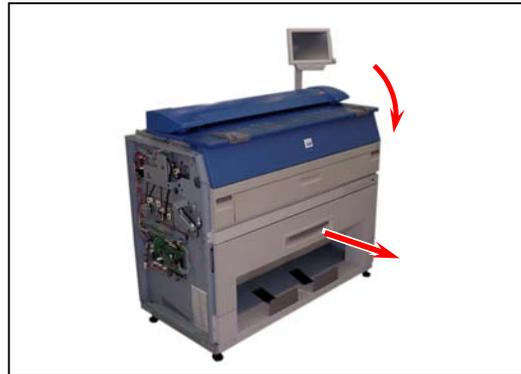
12. Remove 7 screws (12) to remove Cover 14 (13).
