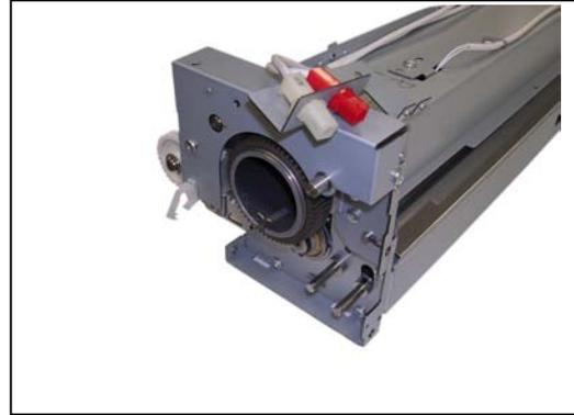
21. Remove 2 screws (38) to remove Bracket 7 Assy (39).
