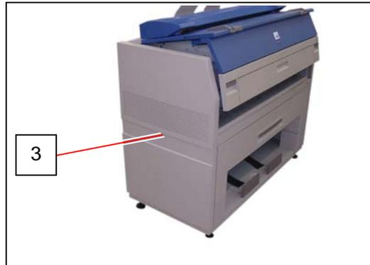
3. Remove 4 pieces of 4x6 screw (4), loosen 4 pieces of 4x6 screw (5), and then remove the Cover 15 (6).
