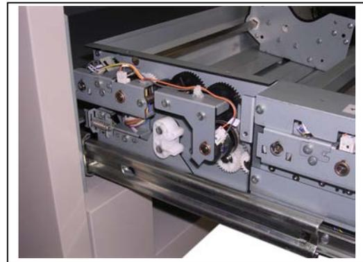
14. Remove 1 Bind Head Screw (16) and 1 Pan Head Screw (17) to remove Gear Bracket 2 Assy (18).
