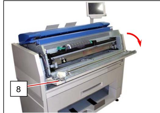
8. Disconnect the connector (9). Holding both Side Plates (10), remove the **Developer Unit** (11) from the machine.
