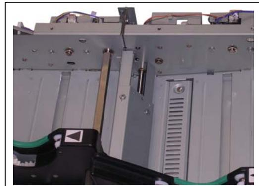
22. Remove 8 screws (35) to remove Guide Plate (36) from the joint of the decks.
