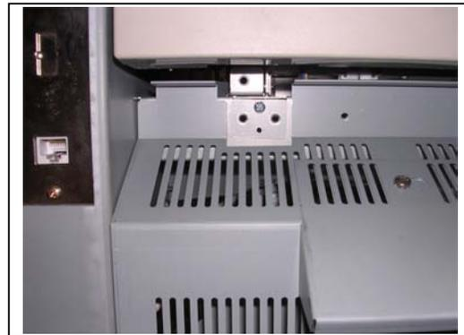
11. With Engine Unit open, remove **Fuser Unit** (15).
