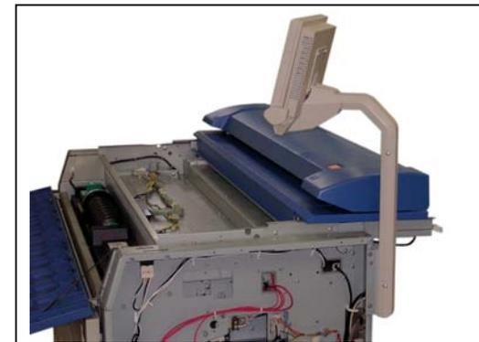
13. There are 2 pieces of Stopper (16) at both sides, which lock the LED Head Frame.
