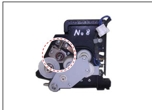
43. Make sure that the 6 screws (48) (55) (34) (52) are installed loose. If not, loosen them.
