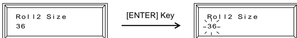
5. Pressing the [ < ] and [ > ] Keys, select the size of the roll paper installed on the concerning Roll Deck.
