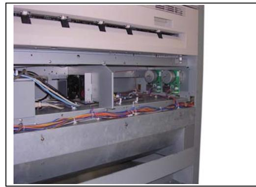
3. Disconnect the connector (6), remove 1 screw (7), and then remove the Bracket Blower (8). Remove 3 screws (9) to replace **Blower** (10) with the new one.
