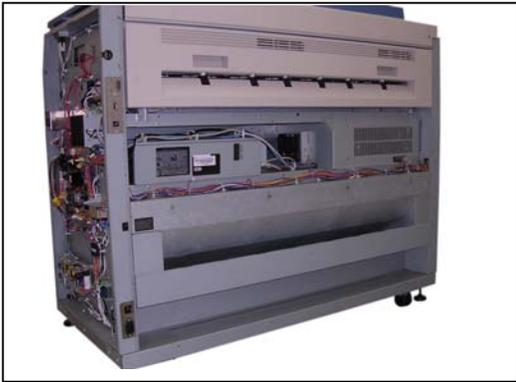
4. Remove 5 screws (7) to remove Case 5 (8).
