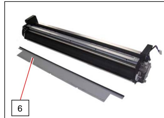
6. Remove 4 pieces of 4x6 screw (7) to remove Scraper Assembly (8).
