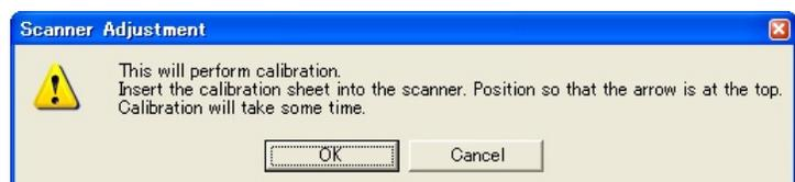
5. Set Shading Sheet in the KIP 3100 accessory to the scanner noting the arrow direction.
