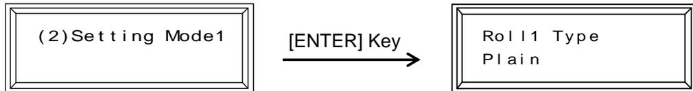
3. There are 2 setting items “Roll Type” and “Roll Size” in the Setting Mode, which you can specify for each Roll Deck 1 and 2 respectively. To specify the type of roll paper, indicate either “Roll 1 Type” or “Roll 2 Type” pressing the [ < ] key and [ > ] key.
