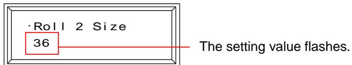
2. Indicate the same size with the roll paper in the Roll Deck 2 pressing [←] key or [→] key.
