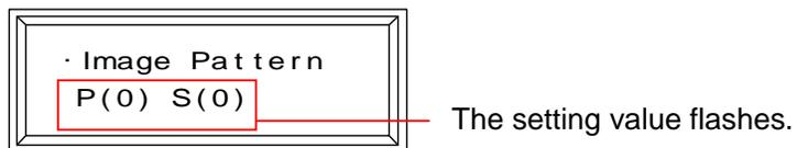
2. "P(X)" of the setting value means the Test Pattern Number
