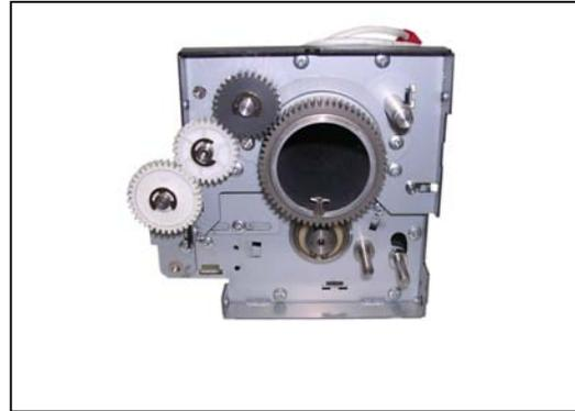
22. Remove 2 screws (40) on the media exit side.
