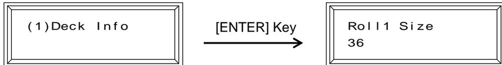
3. If you press [ < ] and [ > ] Keys, you can indicate either "Roll 1 Size" or "Roll 2 Size" on the LCD.
