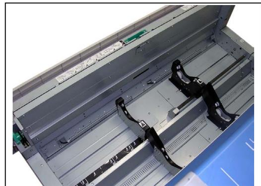
4. Remove 7 screws (5) to remove Cover 22 (6).
