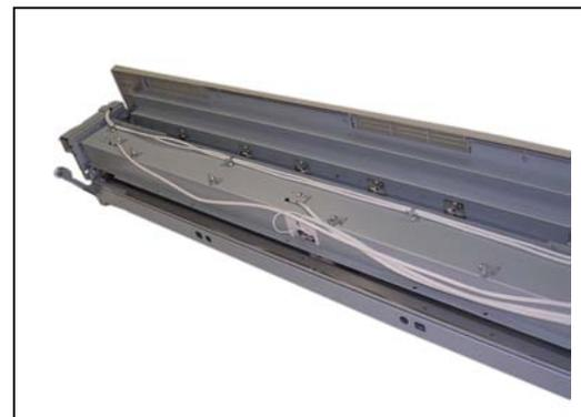
4. Remove each 1 screw (7) to release Thermistor Assy (8: TH1, short harness) and Thermistor 3 Assy (9: TH3, long harness).
