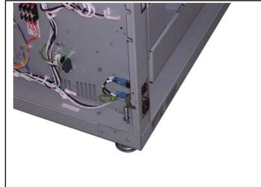
38. Cut off the portion on the rear of Cover 3 (11) for Dehumidify Heater Switch.
