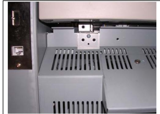
8. Open Paper Exit Assy (11). Loosen 1 screw (12) fixing Fuser Unit inside the machine.
