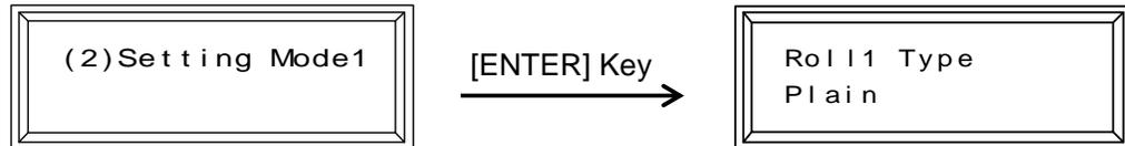
3. There are 2 setting items "Roll Type" and "Roll Size" in the Setting Mode, which you can specify for each Roll Deck 1 and 2 respectively. To specify the size of roll paper, indicate either "Roll 1 Size" or "Roll 2 Size" pressing the [ < ] key and [ > ] key.
