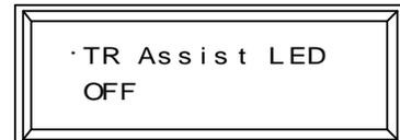
2. Switch between "ON" and "OFF" pressing the [ENTER] Key.
