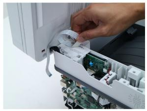
**8** Disconnect the four cables, and then remove the screw securing the two ground cables.
