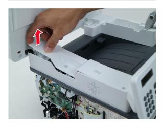
**7** Disconnect the FFC cable, and then remove it from the frame.
