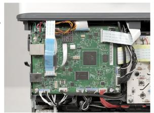
**7** Remove the controller board.
