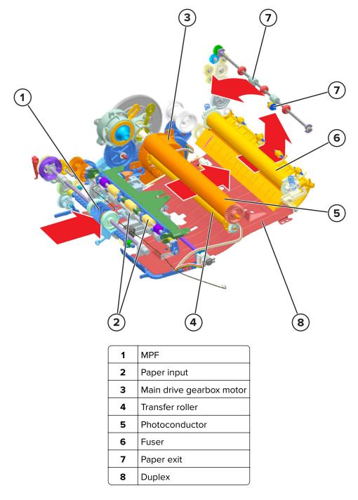
The gearbox provides mechanical power to the printer. Its motor transfer power through a number of gears to the following parts: MPF, paper input, transfer roll, photoconductor drum, fuser, paper exit, and duplex.
