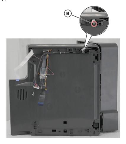
**6** Release the cable from the clamps, and then remove it.
