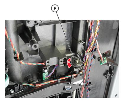
**15** Pull out the shaft, and then remove the pick roller assembly.
