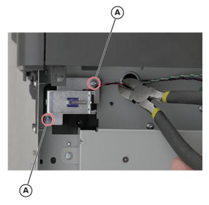
7 Disconnect connector JDUPSOL1 from the controller board, and then pull the cable out of the printer.
