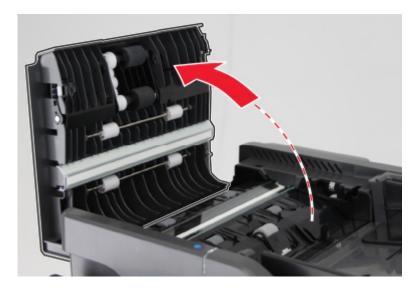
**2** Pull and then release the latch on the right side of the door. Do the same to release the latch on the other side.
