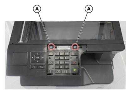
**4** Carefully disengage the assembly from the rear cover.
