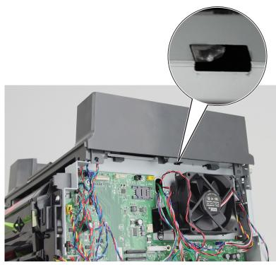
**8** Slide the cover to the front, and then pull up to remove.
