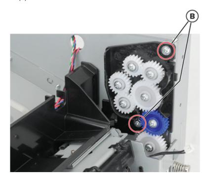
**7** Remove the redrive gear assembly.
