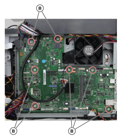
**8** Remove the controller board.
