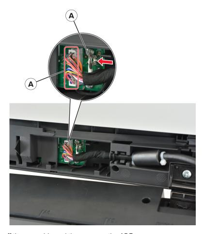
**5** Release the cables off the assembly, and then remove the ADF.
