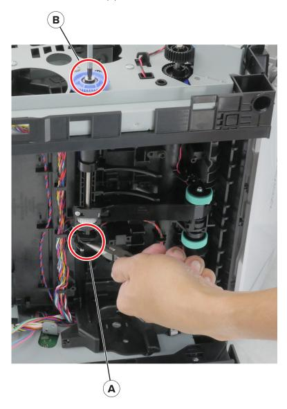
**8** Pull out the pick roller assembly clutch, and then cut the cable to remove it.
