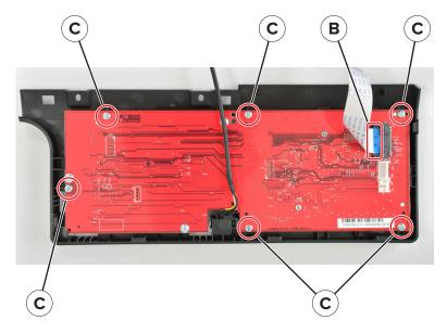
4 Remove the control panel assembly.
