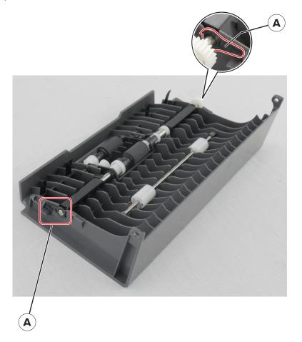
**3** Rotate the latches as shown, and then pull up to remove the roller.
