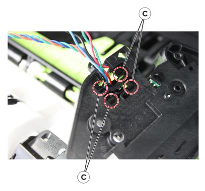
**7** Remove the toner cartridge smart chip contact.
