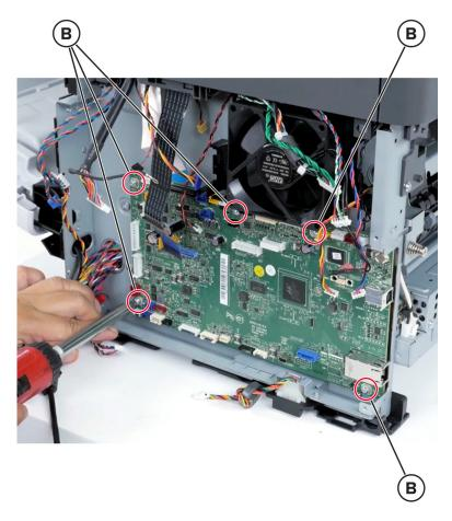
**7** Remove the controller board.
