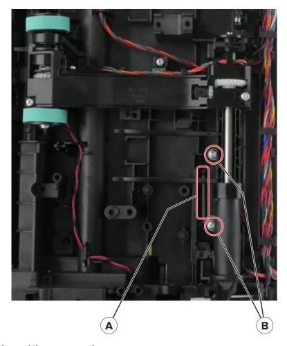
**6** Disconnect the cable, and then remove the sensor.
