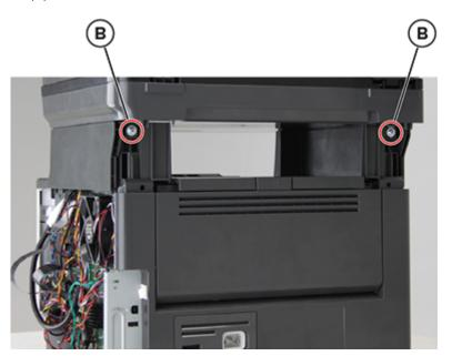
**6** Remove the flatbed scanner assembly.
