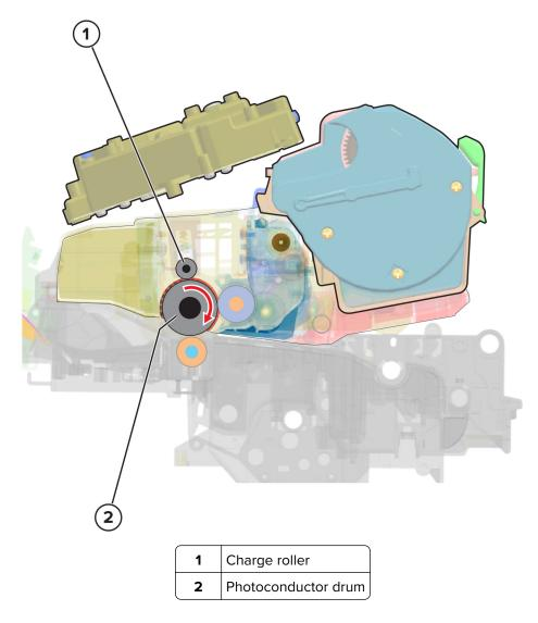
A uniform negative electrical charge is applied by the charge roller to the surface of the photoconductor drum. The photoconductive properties of the surface material allow it to hold the charge as long as it is not exposed to light.
