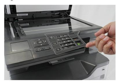
**Installation note:** When installing the cover, put in place the two latches (A) first.
