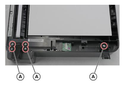
**Installation note:** When installing the left hinge, make sure that the extension (A) is facing to the left.
