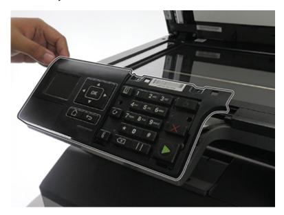
**5** Remove the screw (B), and then disconnect the cable (C).
