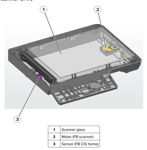
The flatbed scanner has a scanner lamp that is used to illuminate the surface of the document. The reflections produced are processed to create the scan image.
