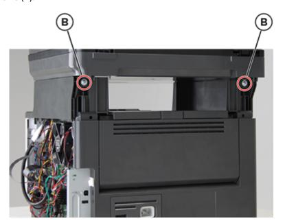
**6** Remove the flatbed scanner assembly.
