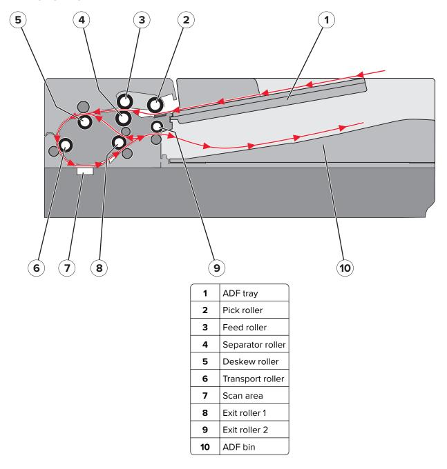
After the sensor (ADF paper present) detects paper in the ADF tray, the pick roller drops and advances the paper into the ADF.
