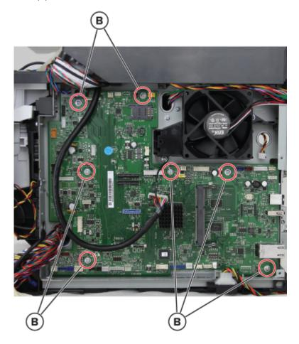
**7** Remove the controller board.
