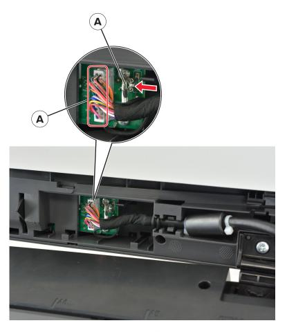
4 Close the ADF, and then remove the scanner assembly. See <u>"Scanner assembly removal" on page 273</u>.
