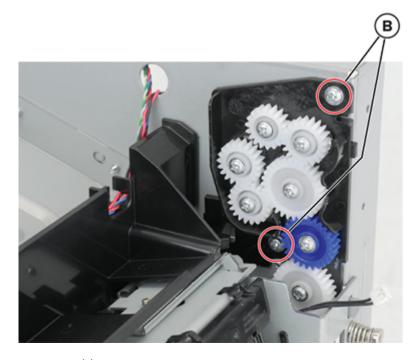
**7** Remove the redrive gear assembly.
