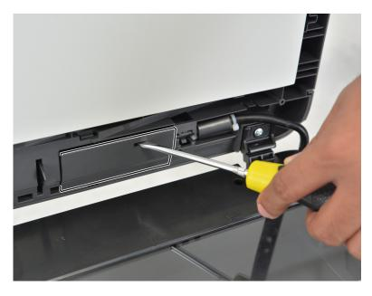
4 Disconnect the two cables (A).
