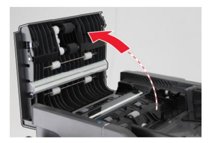
**2** Pull and then release the latch on the right side of the door. Do the same to release the latch on the other side.
