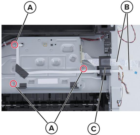
**Installation note:** When installing the printhead, tighten the screws in the following the order:
