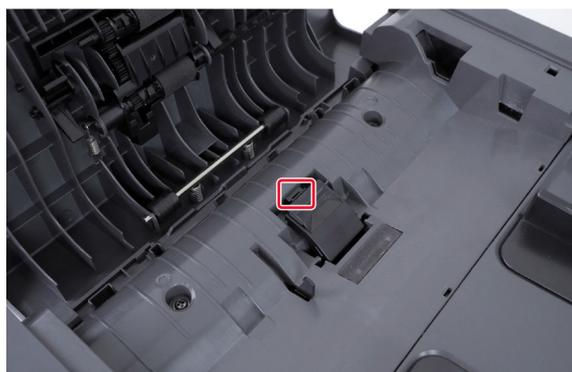
**Installation note:** Do not lose the spring under the ADF separator pad.
