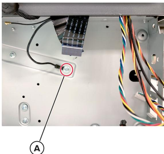
**Installation note:** Secure the fax card ground wire to location A on the frame (see above).
