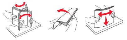
**4** Load the paper stack toward the back of the tray as shown with the recommended print side facedown.
