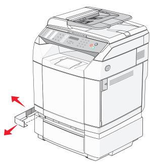
**5** Loosen the right thumbscrew, and remove the right bracket.
