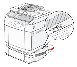
4 Remove the left side cover by starting at the back of the printer and gently pulling each of the four slots off of its matching tab as you work your way to the front of the printer.
