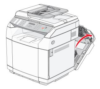
3 Pull the fuser pressure release levers to release tension on the paper.
