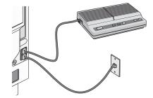
**Note:** Once this plug is removed, any country- or region-specific equipment that you connect to the printer by the adapter, as shown, will not function properly.
