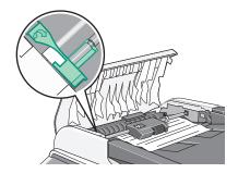
Warning: Do not pull the jammed paper out from the bottom of the ADF.
