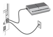
Warning: Do not touch cables or the printer in the area shown while actively sending or receiving a fax.
