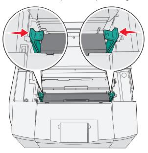
Grasp the handle, and pull the photodeveloper cartridge straight up and out.
