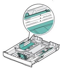
**3** Squeeze the width guide tabs together as shown, and slide the width guide to the correct position for the paper size being loaded.
