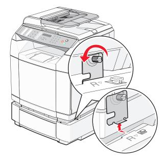
**6** Loosen the left thumbscrew, and remove the left bracket.
