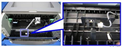
2. Relay sensor [A] ( x 1, hooks)
