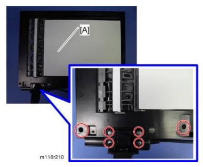
4. At the bottom of the ARDF unit [A] ( \* x 6).
