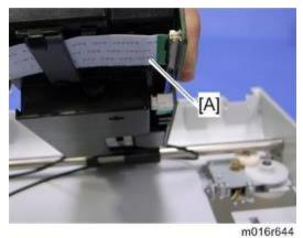
5. Remove the flat cable [A] from the scanner carriage unit.
