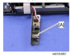
3. ARDF feed sensor [A] (hooks, 🗐 x 1)
