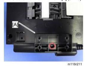
5. At the bottom of the ARDF unit [A] (  $\mbox{\it P}$  x 1).
