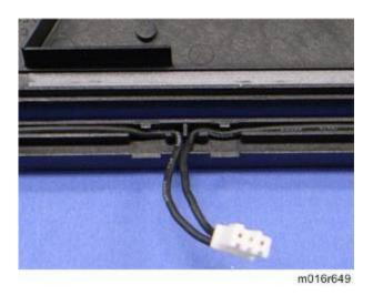
Place the lamp cord wires as shown above. Otherwise, the top cover could pinch the lamp cords and damage them when reinstalling the top cover on the scanner carriage unit.
