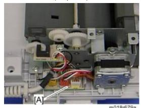
3. ADF drive board [A] (no screws, all plugs ( )s and hooks)
