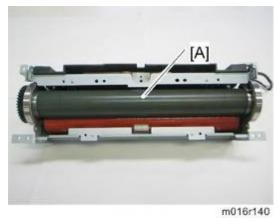
3. Hot roller [A] (C-ring x 2, gear x 1, bushing x 2)
