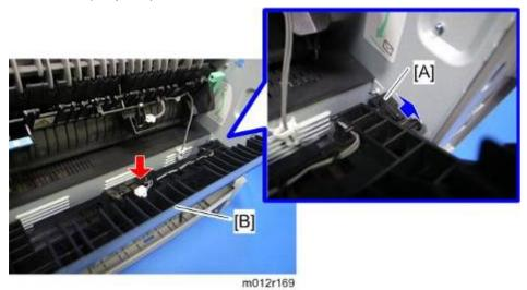
4. Release the lock [A], and then remove the entrance guide [B] ( 1).
