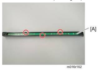
3. Remove the quenching lamp [A] from the case (hook x 3).
