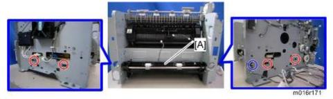
22. For M119 only: Duplex cover [A] ( x 4, C x 1, gear x 1)
