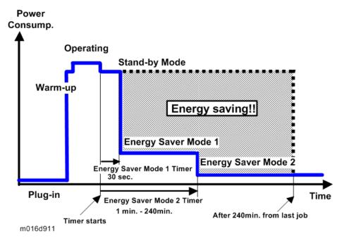
The backlight of the screen is turned off and "Energy Saver Mode1" appears on the screen, and then the fusing lamp is turned off and "Energy Saver Mode2" appears on the screen.
