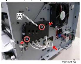
2. Charge terminal case [A] with the harness ( x 2, v 1, hooks)
