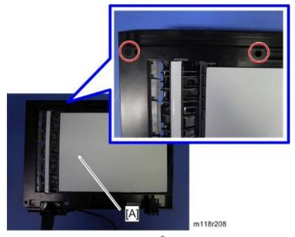
4. At the bottom of the ARDF unit [A] ( x 2).
