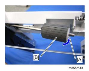
4. Release the hook [A] and then move the paper feed roller [B] to the right.
