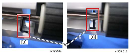
2. Reinstall the paper feed roller shaft correctly.
