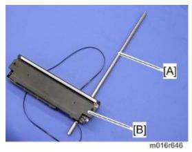
7. Carriage bar [A] and scanner carriage unit [B]
