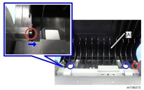
4. ARDF top cover [A] from the left side (two tabs, two hooks)
