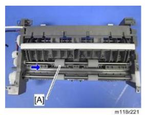
5. ARDF transport roller [A] (Bush POM x 2, Gear POM x 1).
