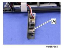
4. ADF feed sensor [A] (hooks, 🔎 x 1)
