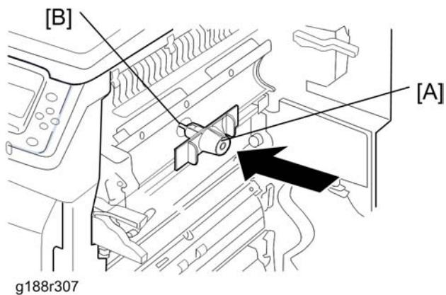
3. Insert the special cleaning tool [A] into the hole [B] of the printer.
