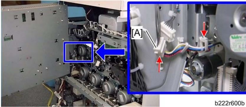
7. Disconnect the connector [A] (⚙️ x 1)
