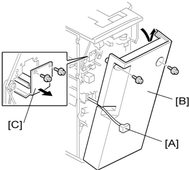
1. If the finisher is connected to the mainframe, disconnect the power connector [A] and move the finisher away from the mainframe.
