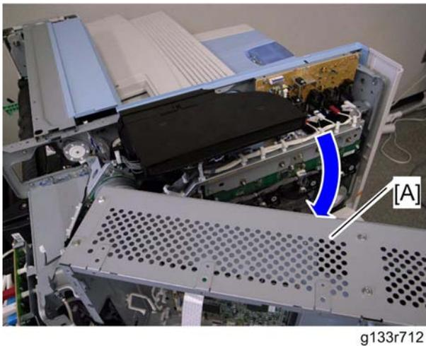
8. Open the controller box [A] as shown.
