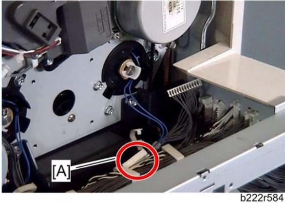
5. Disconnect the connector [A] (☞ x 1).
