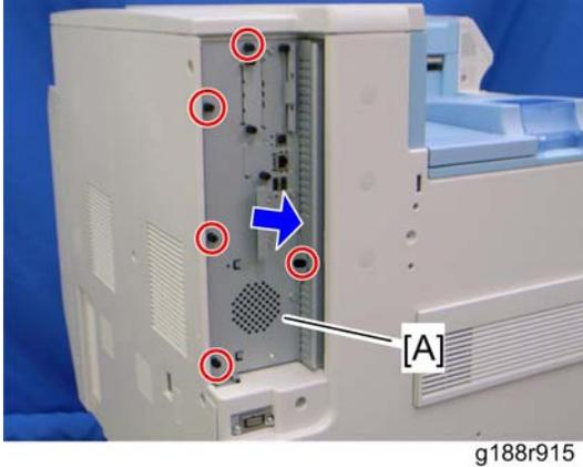
1. Controller unit [A] (knob screw x 5)
