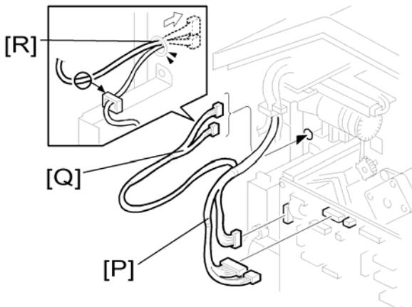
14. Connect the harnesses [P] to the main PCB.
