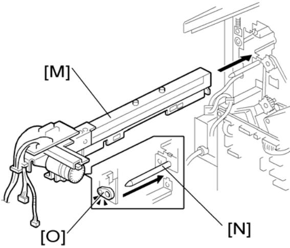
12. Install the punch unit [M] along the punch unit stay from the rear side.
