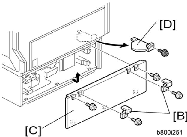
4. Remove the two securing brackets [B] (🔩 x 1 each), and then the rear cover [C] of the optional paper feed unit (🔩 x 2).
