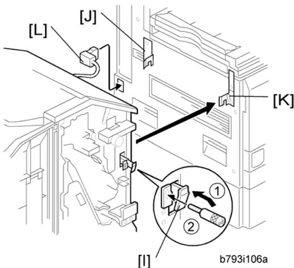
8. Pull the lock lever [I] (Long knob screw x 1).
