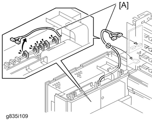
16. Release the harness [A] from the printer (🔌 x 5).
