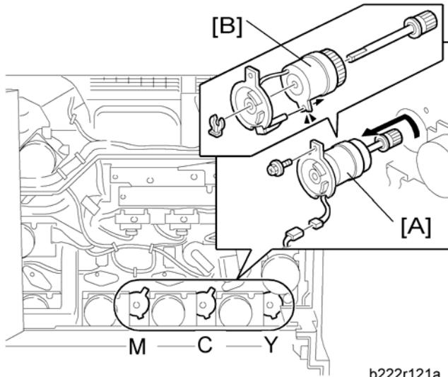
6. Turn the development clutch unit [A] counter-clockwise and then pull it out (🔩 x 1).
