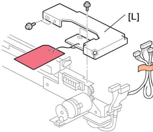
11. Remove the bracket [L] from the punch unit (⚙ x 1).
