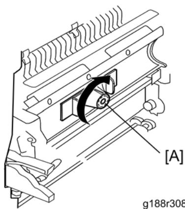
4. Rotate the special cleaning tool [A] 10 times while pushing in to clean the lens inside of the printer.
