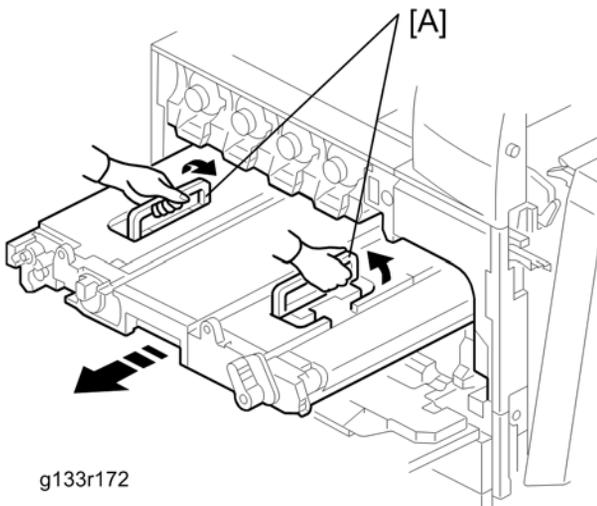
6. Grasp the handles [A], and then pull out the image transfer belt unit fully.
