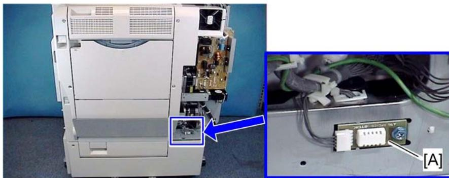
3. Temperature and humidity sensor [A] (🔧 x 1, 📦 x 1)
