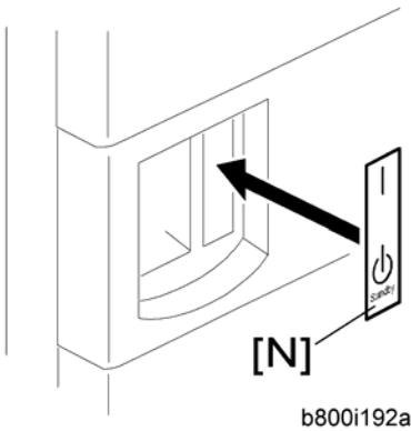
14. Attach the on/standby decal [N] to the right-hand side of the main power switch.
