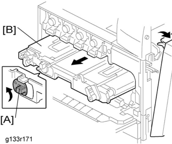
4. Turn the image transfer belt unit lock lever [A] counterclockwise.
