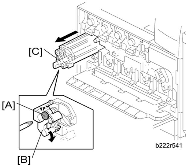
6. Loosen the screw [A].
