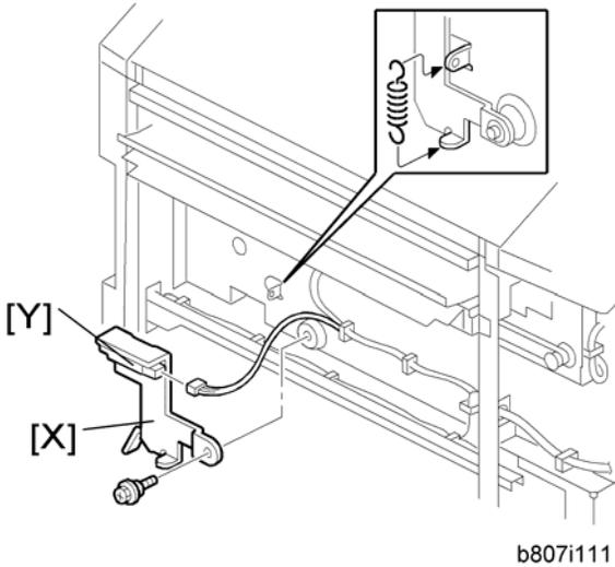
22. Install the hopper full sensor arm [X] (⚙️ x 1, spring x 1).
