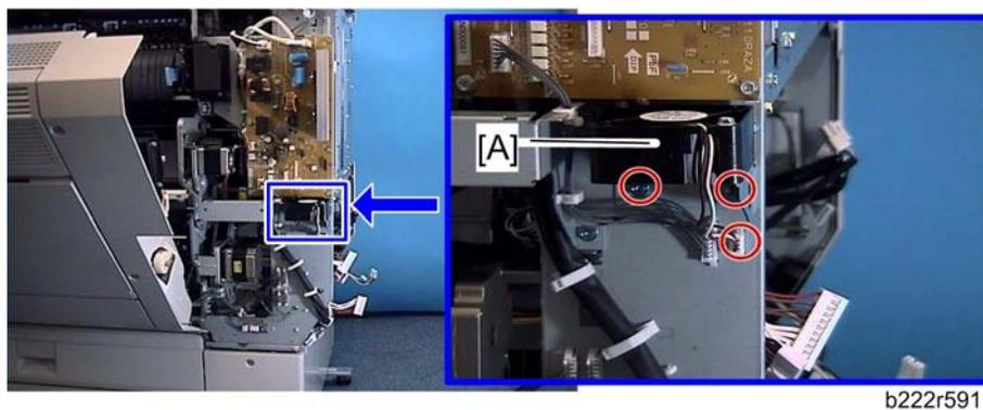
3. IH inverter fan bracket [A] (🔧 x 2, 📏 x 1)
