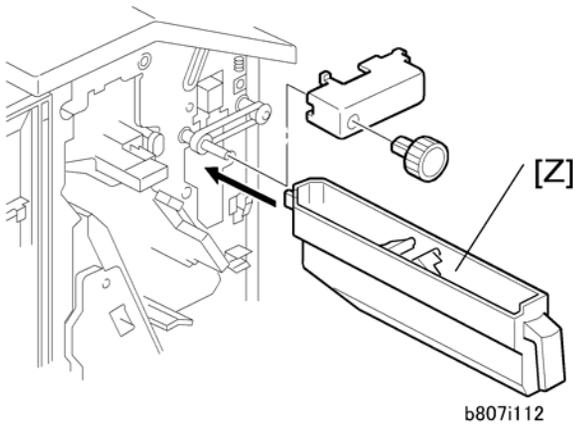
24. Install the hopper [Z] from the front side.
