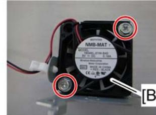
2. HDD fan bracket [A] (🔩 x 2)
