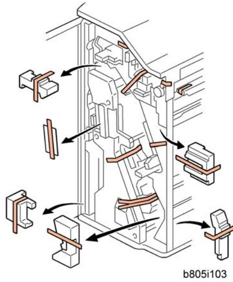
1. Unpack the finisher and remove all tapes and packing materials from the finisher.
