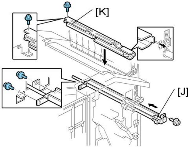
9. Install the punch unit stay [J] from the front side (⚙ x 3).
