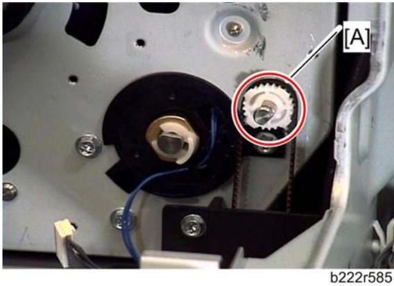
6. Remove the pulley and bushing [A].
