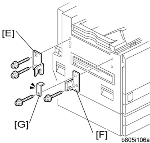
7. Attach the rear joint bracket [E] (⚙ x 2; M4 x 14).
