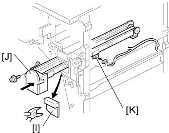
12. At the front, use a pair of wire cutters to remove the part [I] of the cover.
