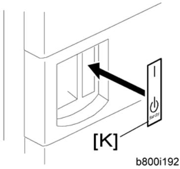
12. Attach the on/standby decal [K] to the right-hand side of the main power switch.
