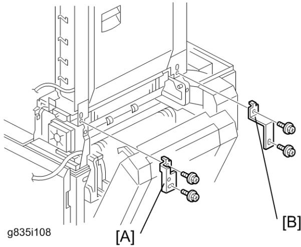
15. Attach the front hold bracket [A] and rear hold bracket [B] (🔩 x 2 each).
