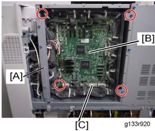
4. Remove the controller box stay [A] (⚙️ x 4).
