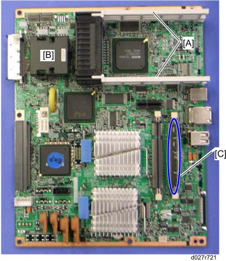
3. Interface rails [A], NV-RAM [B], RAM-DIMM [C]
