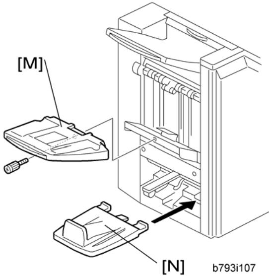
13. Install the upper output tray [M] (Short knob screw x 1).
