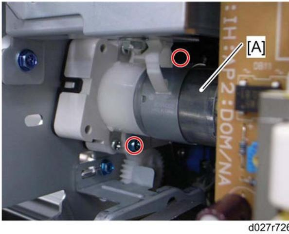
8. Paper transfer contact motor [A] (⚙️ x 2)
