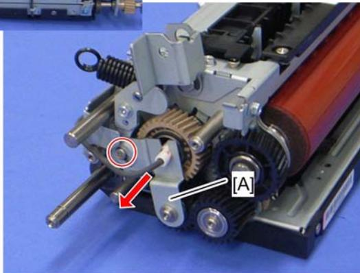
5. Rear terminal of the fusing lamp (☛ x 1, ☛ x 3)
