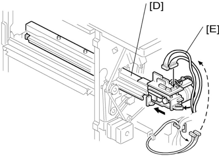
4. Move the punch unit [D] along its rails into the finisher. Make sure that the pin engages correctly at the front and rear.
