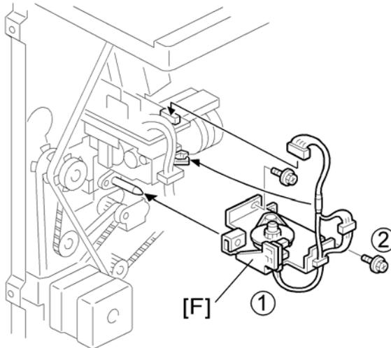
6. Attach the slide drive unit [F] to the finisher and connect it to the punch unit (🔌 x 2, 📡 x 1). Push in the slide drive unit at (1) when you attach the screw (2).
