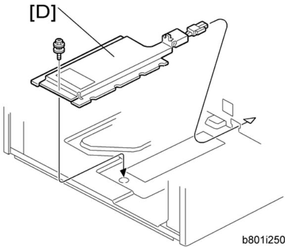
5. Install the tray heater [D] in the optional LCT (1 x 1).
