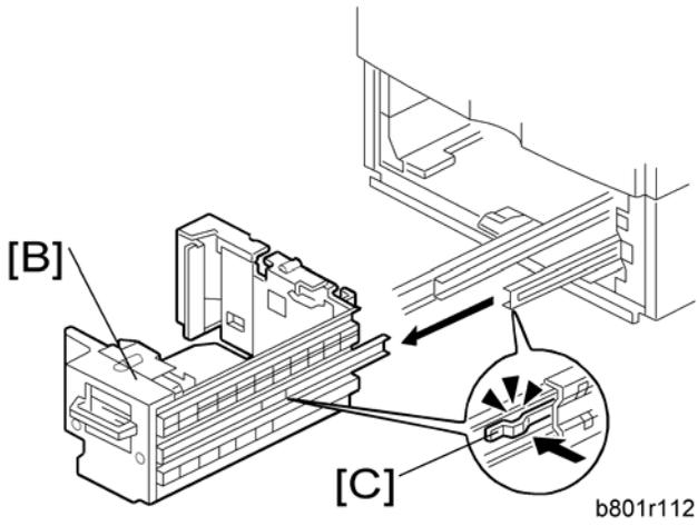
4. Remove the right tray [B] while pressing down the stopper [C].
