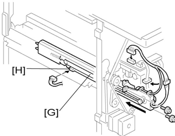
8. Put the side-to-side detection unit [G] in the machine. Make sure that the two pins are engaged correctly at the front.
