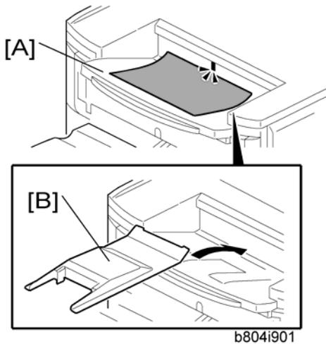
1. If a stack problem occurs several times on the upper output tray [A], put the support tray [B] on the tray as shown.
