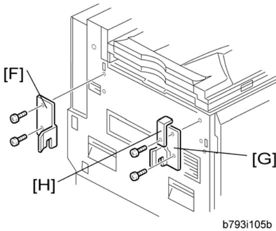
6. Attach the rear joint bracket [F] (⚓ x 2, M4 x 14).
