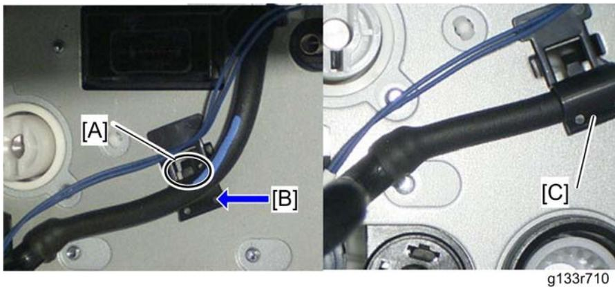
6. Pass the harness of the toner pump unit behind the hook [A], while pressing at [B].
