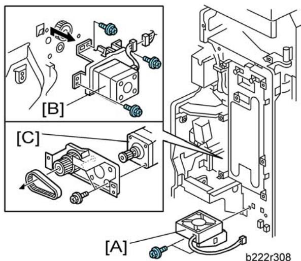
5. Fusing power supply board fan bracket [A] (☞ x 2, ☞ x 1)
