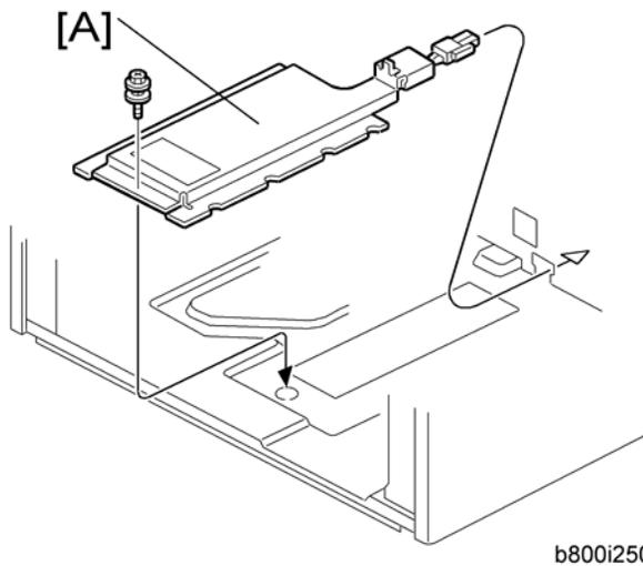
3. Install the tray heater [A] in the optional paper feed unit (⚙ x 1).
