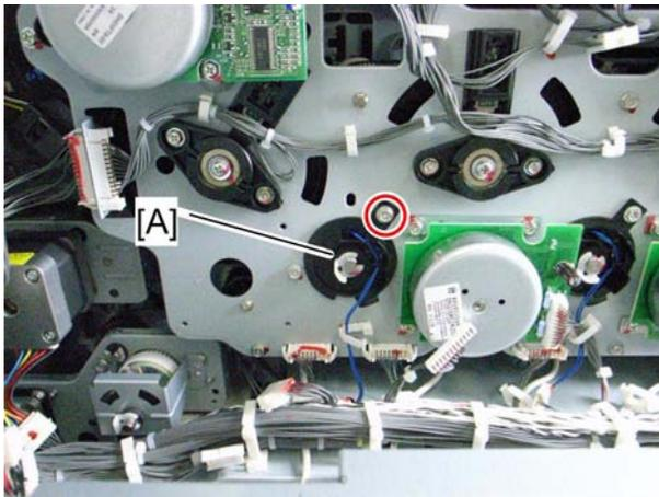
5. Turn the development clutch unit [A] counter-clockwise and then pull it out (🔩 x 1).
