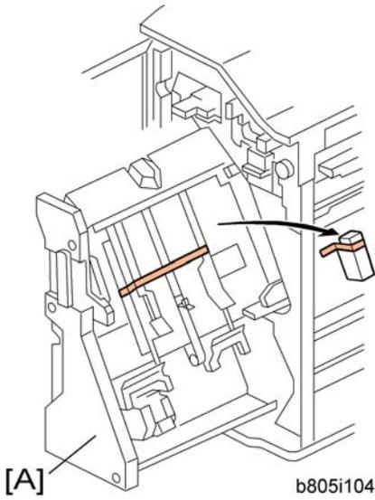
3. Pull out the jogger unit [A], and then remove all tapes and retainers.
