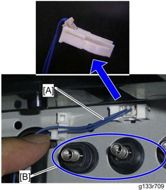
4. Connect the harness [A] to the connector of the machine.
