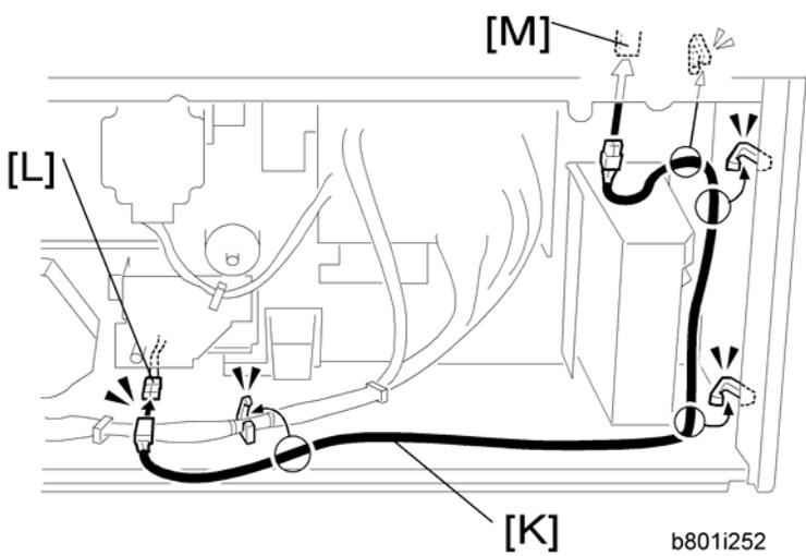
10. Connect the harness [K] to the connector [L] of the tray heater.
