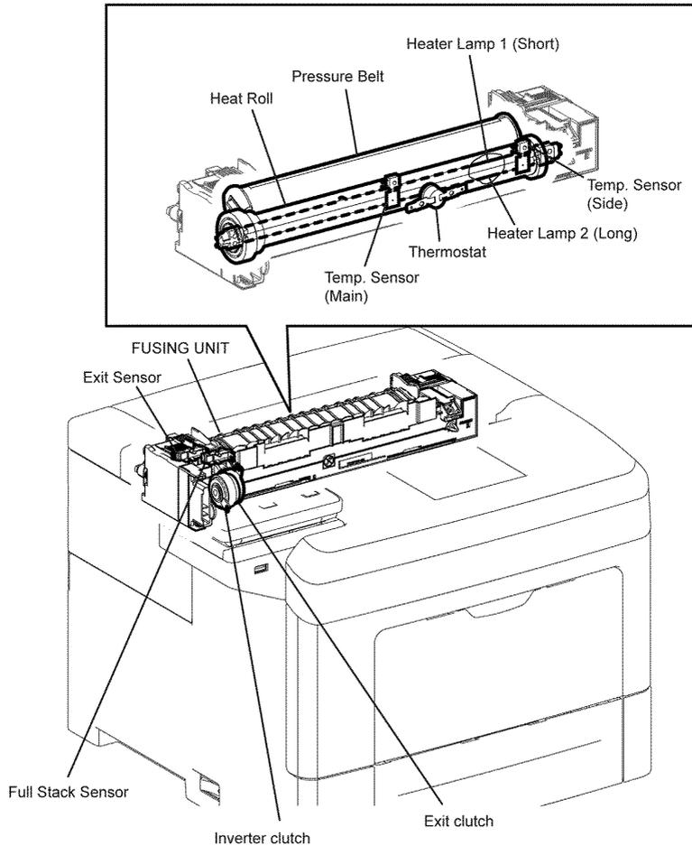
Figure 6 Fusing/exit
