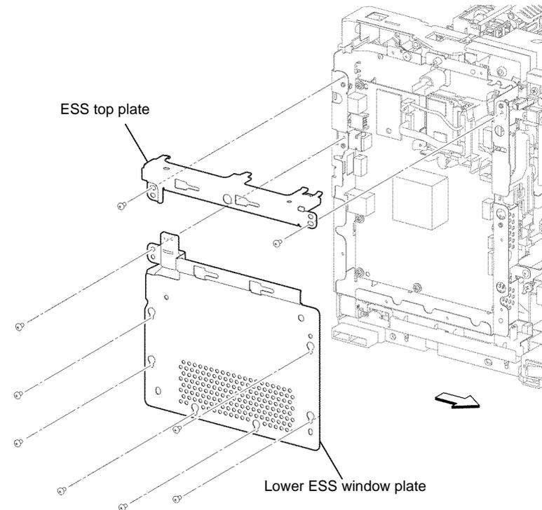
Figure 2 ESS top and lower plate removal
