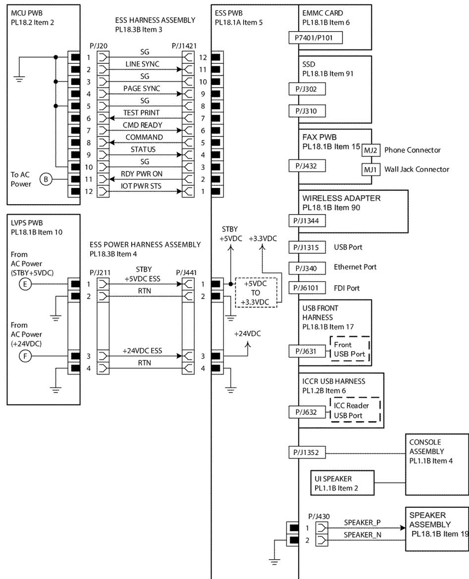
Figure 10 Wiring Diagram 10
