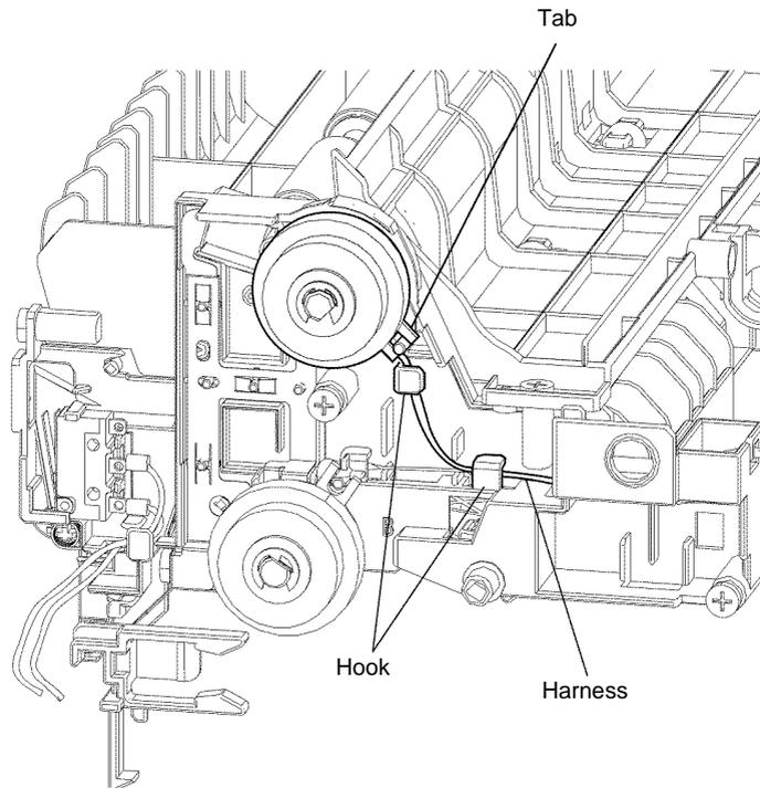
Figure 5 Registration clutch installation
