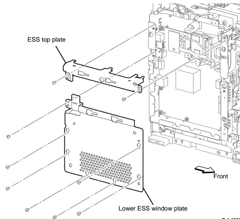
**Figure 1 ESS top and lower plate removal**
