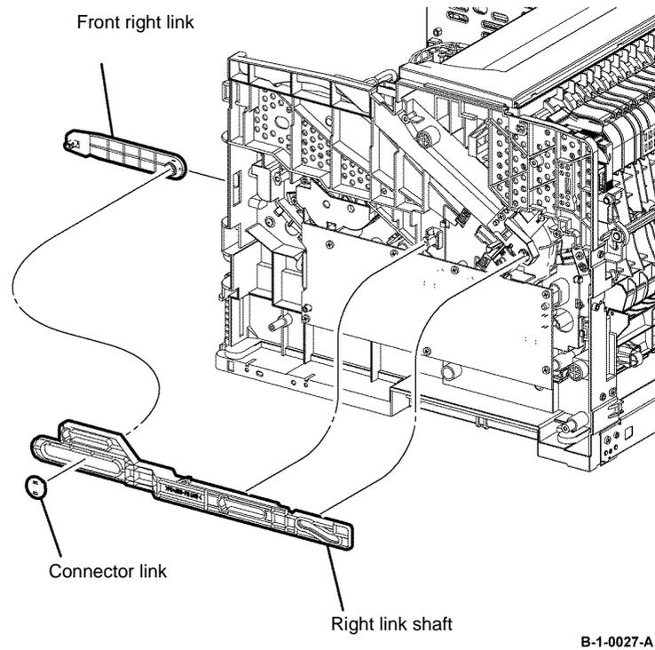
Figure 2 Right link shaft removal
