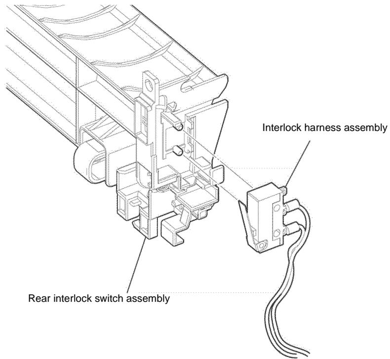
**Figure 4 Interlock harness assembly removal**
