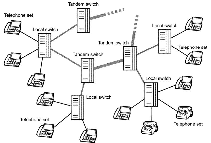
Figure 2 Switching equipment network
