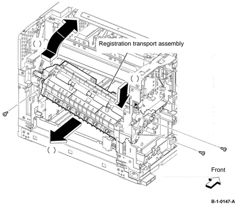
Figure 6 Registration transport assembly removal
