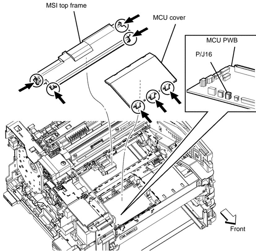
**Figure 2 T24 inverter clutch harness assembly release**
