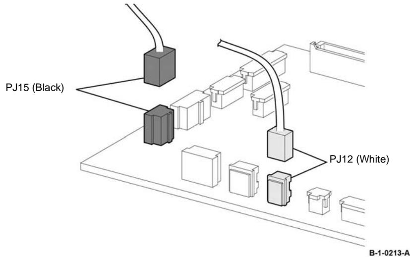
Figure 3 MCU PWB Installation
