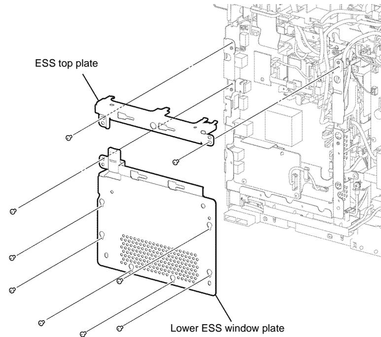
Figure 2 ESS top and lower plate removal
