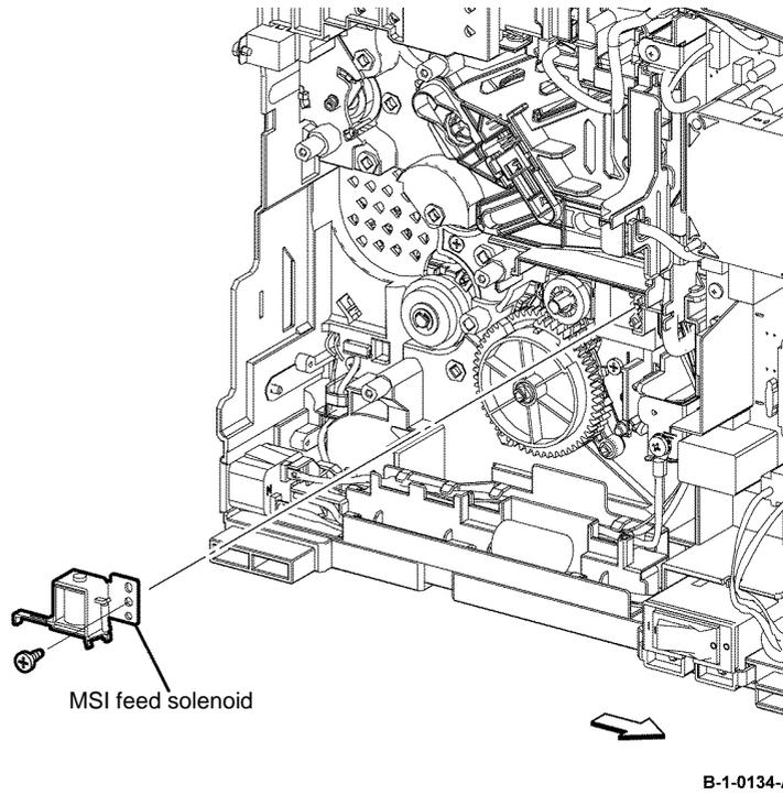
**Figure 2 MSI feed solenoid removal**
