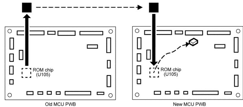
**Figure 4 U105 ROM chip installation**
