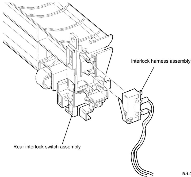
**Figure 4 Interlock harness assembly removal**
