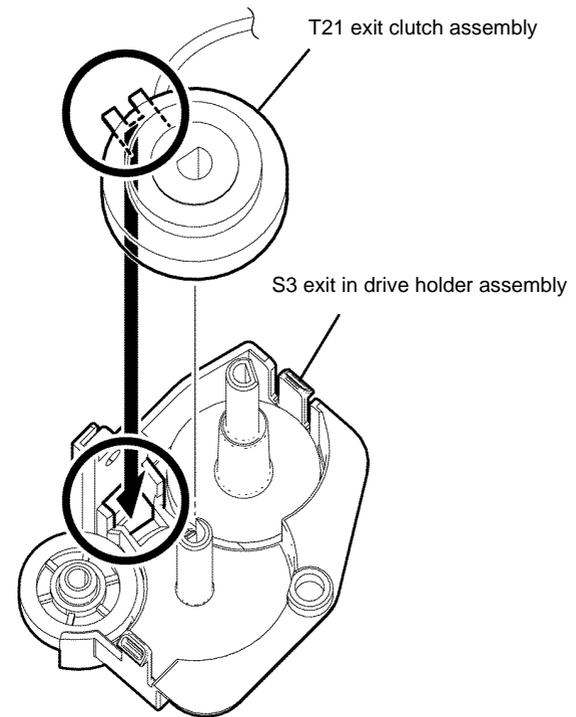
**Figure 5 T21 exit clutch assembly installation**
