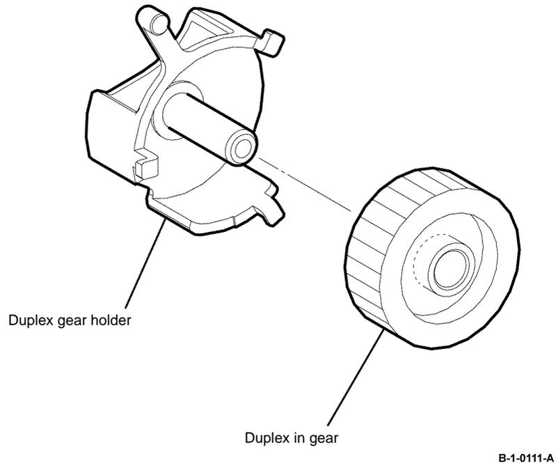
**Figure 2 Duplex in gear removal**
