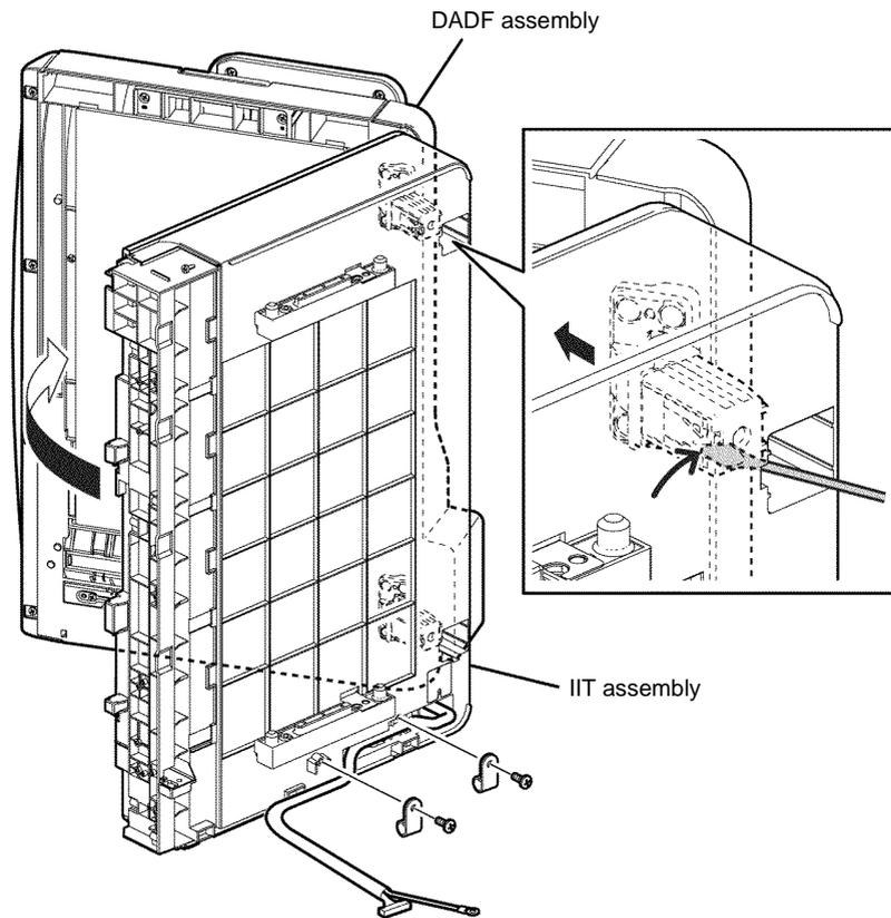
Figure 4 DADF, IIT assembly separation
