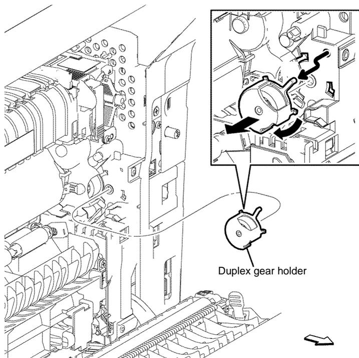
Figure 1 Duplex gear holder removal
