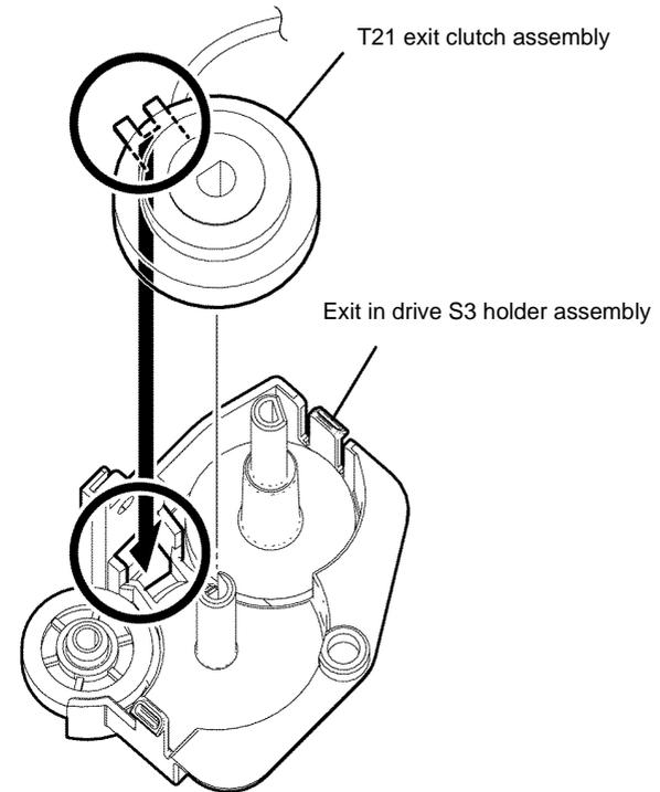
Figure 5 T21 exit clutch assembly installation
