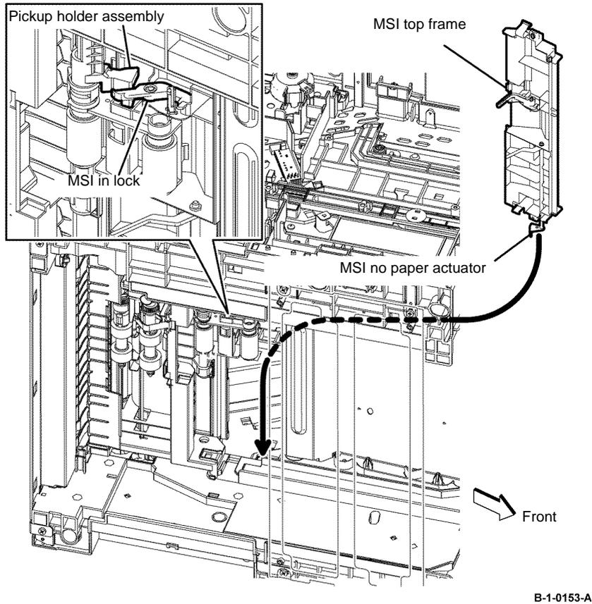
Figure 12 MSI top frame installation
