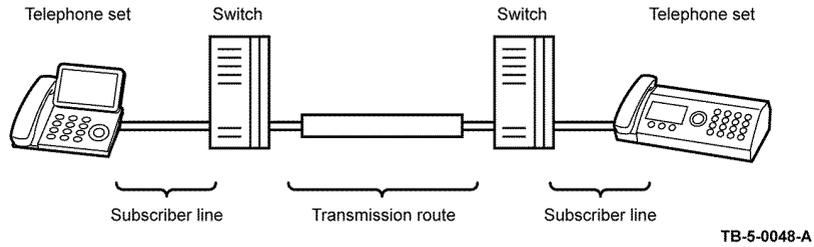
Figure 1 Analog telephone network
