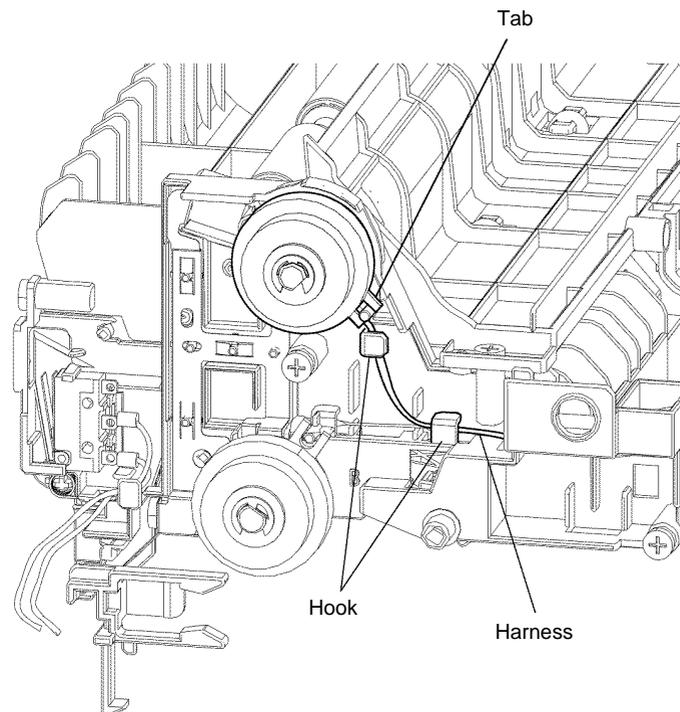
**Figure 5 Registration clutch installation**
