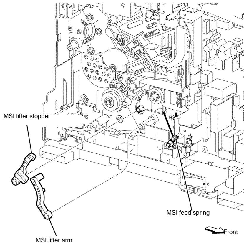
**Figure 3 MSI lifter arm and lifter stopper removal**
