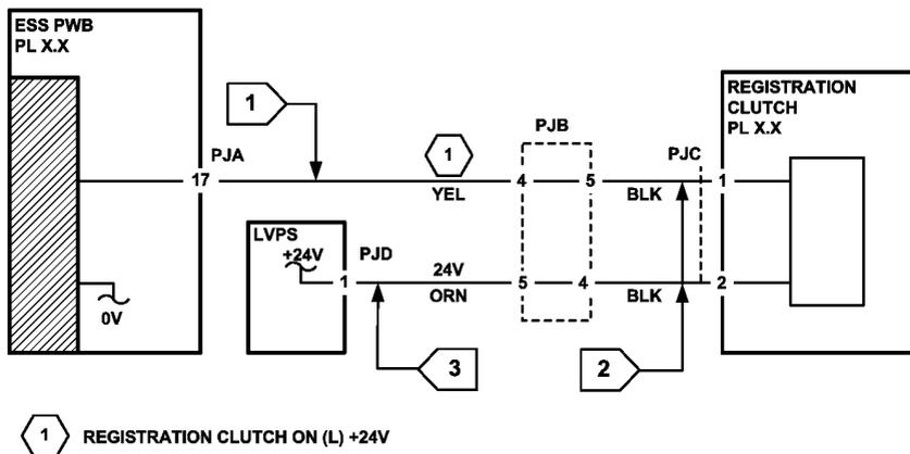
Figure 1 Wiring diagram
