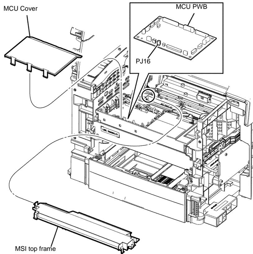
**Figure 2 T24 inverter clutch assembly harness release**
