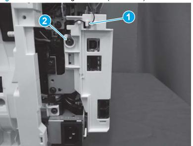
Figure 1-234 Install the ground wire (ISA models)
