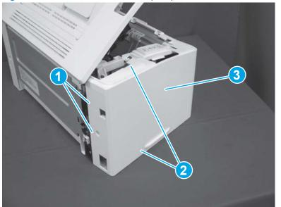
Figure 1-83 Remove the left cover (SFP)
