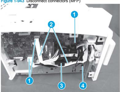
Figure 1-943 Disconnect connectors (MFP)
