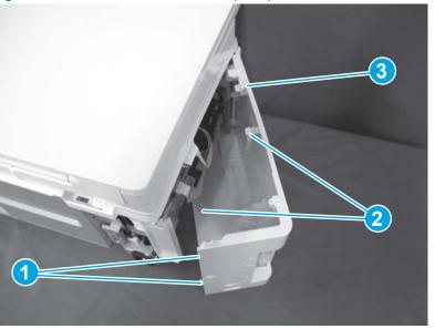
Figure 1-548 Remove the left cover (MFP)
