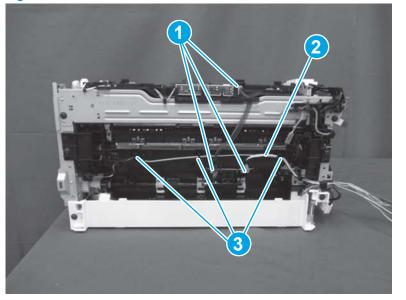
Figure 1-874 Disconnect three connectors
