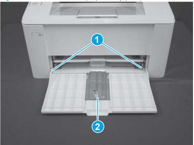
Figure 1-541 Install the multipurpose tray (SFP)
