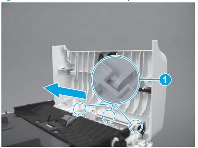
Figure 1-71 Install the document feeder top cover
