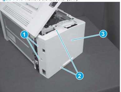
Figure 1-618 Remove the left cover (SFP)
