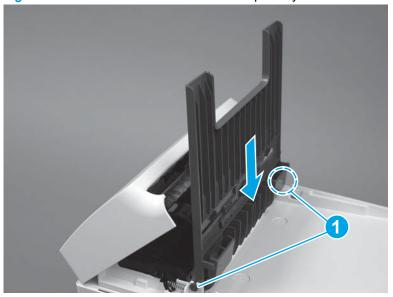
Figure 1-65 Install the document feeder input tray
