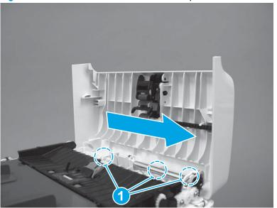
Figure 1-70 Remove the document feeder top cover
