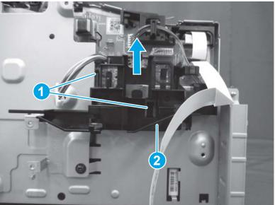
Figure 1-1065 Remove the guide (MFP)
