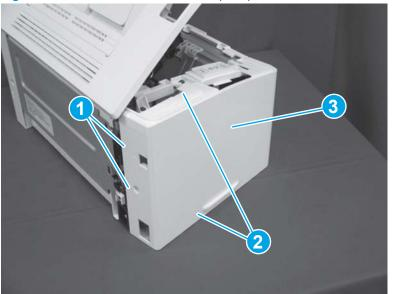
Figure 1-546 Remove the left cover (SFP)
