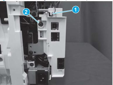
Figure 1-1019 Install the ground wire (ISA models)
