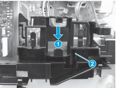
Figure 1-717 Install the guide (MFP)
