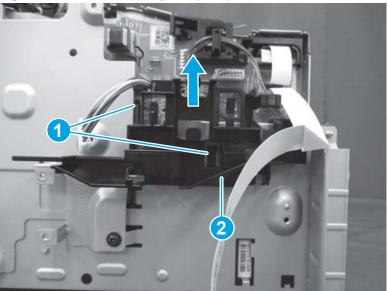
Figure 1-867 Remove the guide (MFP)
