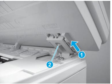
Figure 1-232 Engage the right hinge (M129/M134)
