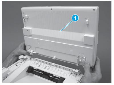
Figure 1-736 Install the ISA or IS (M129/M134)
