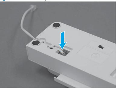
2. Connect the receiver cord to the back of the handset base and the bottom of the handset receiver.
