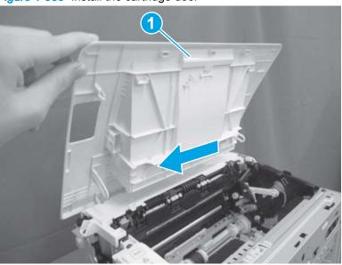
Figure 1-585 Install the cartridge door
