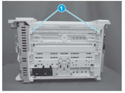
Figure 1-1009 Engage two tabs (MFP)
