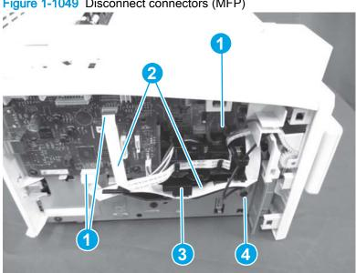
Figure 1-1049 Disconnect connectors (MFP)
