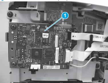
Figure 1-1086 Install the formatter (SFP)
