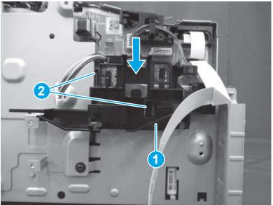
Figure 1-1098 Install the guide (MFP)
