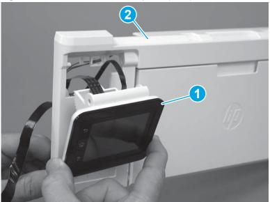
Figure 1-259 Remove the control panel (MFP)
