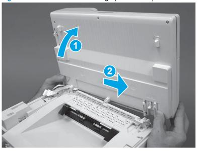
Figure 1-1041 Release the left hinge (M129/M134)
