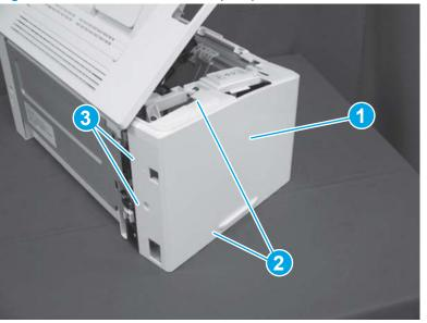
Figure 1-823 Install the left cover (SFP)
