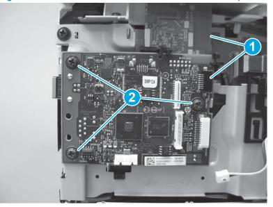
Figure 1-462 Install the formatter PCA and wireless PCA (M101/M106)
