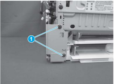
**c.** Remove three screws (callout 1), remove one ground screw (callout 2), and then remove the LVPS.
