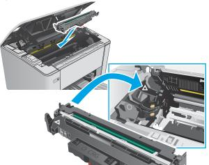
Figure 1-5 Install the image drum
