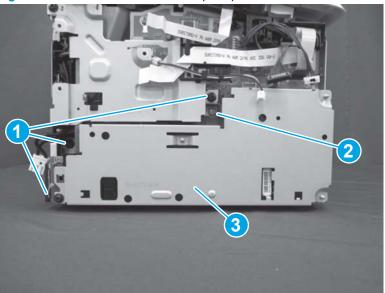
Figure 1-1063 Remove the LVPS (SFP)
