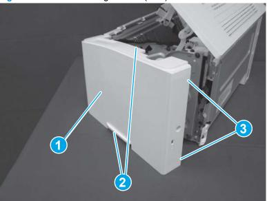
Figure 1-360 Install the right cover (SFP)
