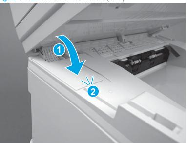
Figure 1-1123 Install the cable cover (MFP)
