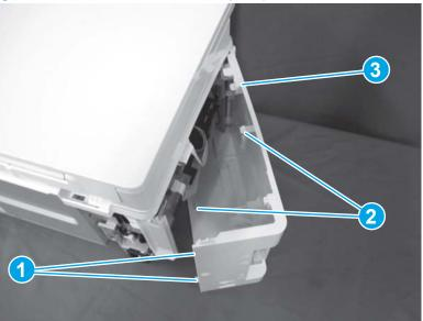
Figure 1-157 Remove the left cover (MFP)
