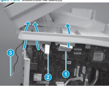
Figure 1-249 Disconnect flat cable(s)
