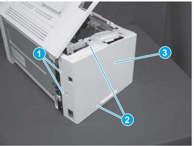
Figure 1-324 Remove the left cover (SFP)
