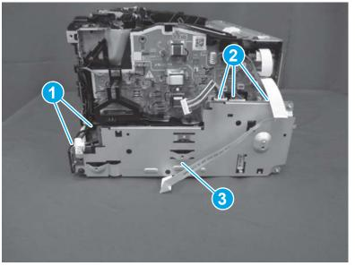
Figure 1-1068 Remove the LVPS (MFP)
