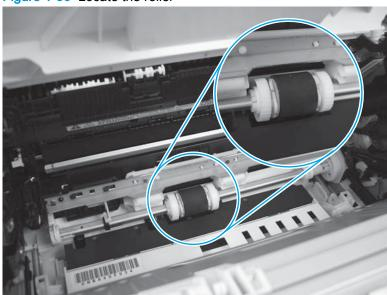
Figure 1-36 Locate the roller
