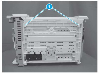
Figure 1-903 Engage two tabs (MFP)
