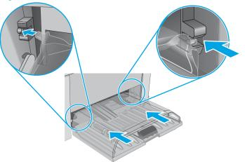
Figure 1-61 Install the dust cover
