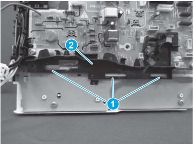
Figure 1-1077 Remove the guide (MFP)
