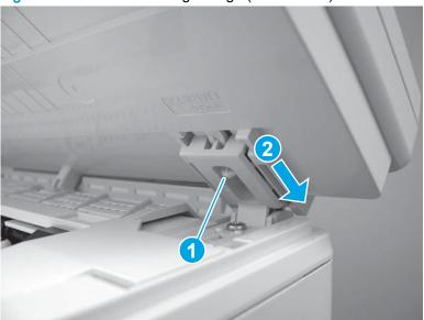
Figure 1-383 Release the right hinge (M129/M134)
