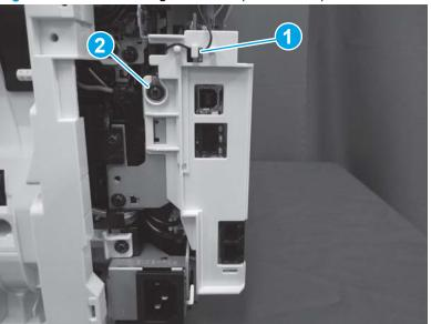
Figure 1-188 Install the ground wire (ISA models)
