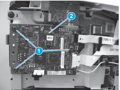
Figure 1-956 Remove the formatter PCA (SFP)
