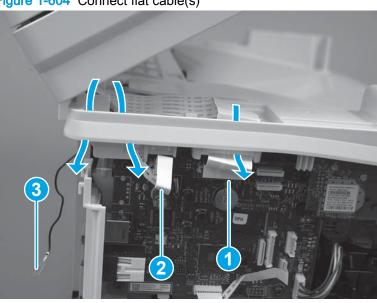
Figure 1-604 Connect flat cable(s)
