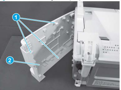
Figure 1-337 Remove the right cover (MFP)
