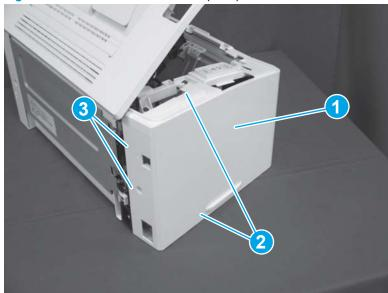
Figure 1-467 Install the left cover (SFP)
