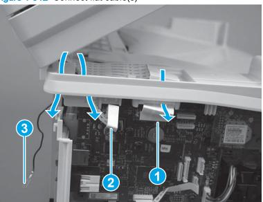
Figure 1-912 Connect flat cable(s)
