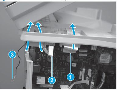
Figure 1-109 Disconnect flat cable(s)
