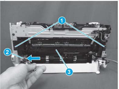
Figure 1-875 Remove the transfer assembly
