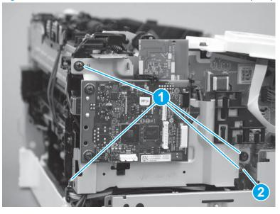
Figure 1-713 Install the formatter and sheet-metal bracket (SFP)
