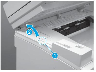
Figure 1-682 Remove the cable cover (MFP)
