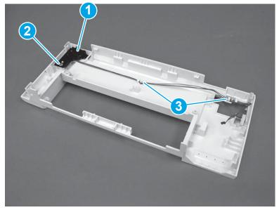
2. Install the control panel (callout 1) on the cover, install the hinge plate (callout 2), install one screw (callout 3), and then engage the wire harnesses in the retainer (callout 4).
