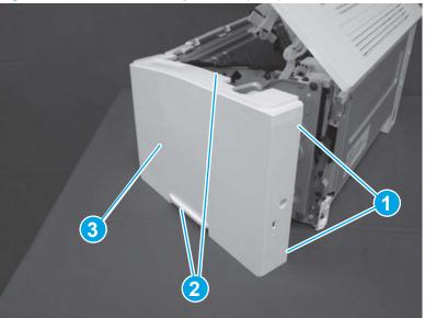
Figure 1-764 Remove the right cover (SFP)
