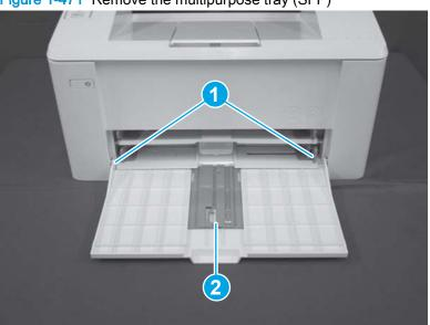
Figure 1-471 Remove the multipurpose tray (SFP)
