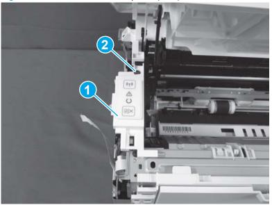
Figure 1-608 Install the control panel (SFP)
