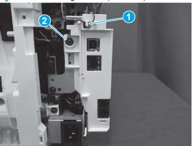
Figure 1-666 Install the ground wire (ISA models)
