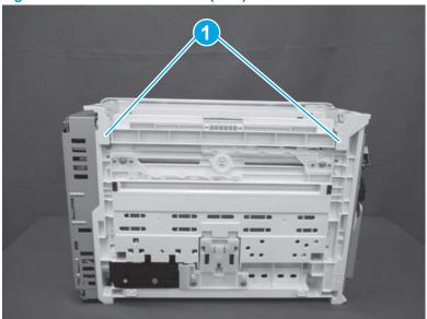
Figure 1-847 Release two tabs (SFP)
