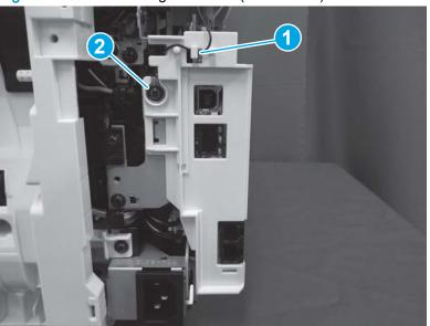
Figure 1-605 Install the ground wire (ISA models)
