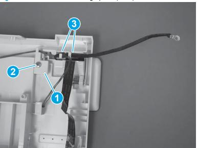
Figure 1-261 Remove the hinge plate (MFP)
