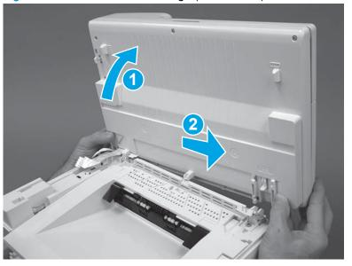
Figure 1-111 Release the left hinge (M129/M134)
