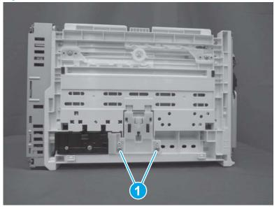
2. Remove the separation pad assembly.
