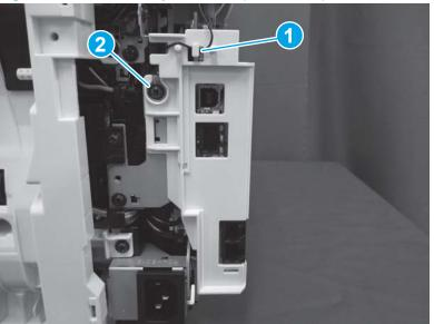
Figure 1-149 Install the ground wire (ISA models)
