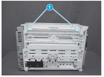
Figure 1-593 Engage two tabs (M101/M106)
