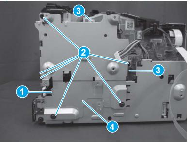
Figure 1-787 Remove the support plate (MFP)
