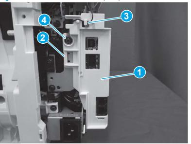
Figure 1-916 Install the USB cover (MFP)
