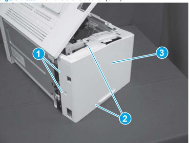
Figure 1-926 Remove the left cover (SFP)
