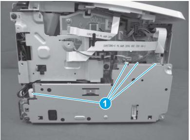
Figure 1-781 Disconnect four connectors (SFP)
