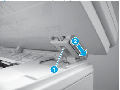
Figure 1-554 Release the right hinge (M129/M134)
