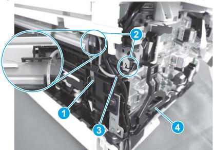
Figure 1-1070 Disconnect one connector and remove the support (SFP)
