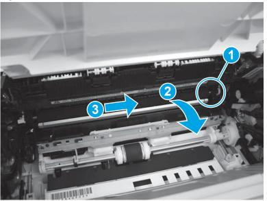
Figure 1-446 Remove the transfer roller
