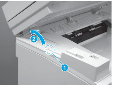
Figure 1-931 Remove the cable cover (MFP)
