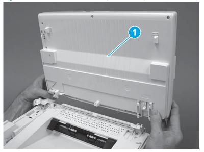
Figure 1-364 Install the ISA or IS (M129/M134)
