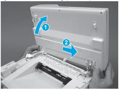
Figure 1-163 Release the left hinge (M129/M134)
