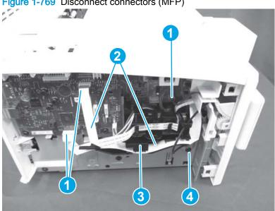
Figure 1-769 Disconnect connectors (MFP)
