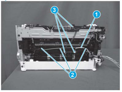
Figure 1-983 Connect three connectors
