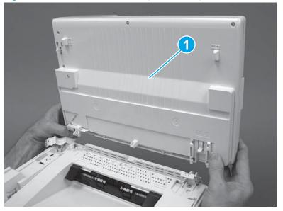
Figure 1-230 Install the ISA or IS (M129/M134)
