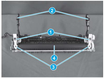
Figure 1-975 Remove the fuser film
