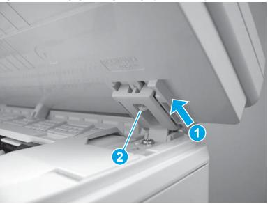
Figure 1-366 Engage the right hinge (M129/M134)
