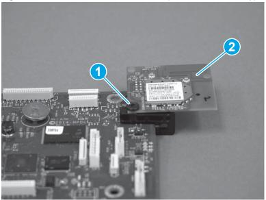
Figure 1-460 Remove the wireless PCA (wireless models only)
