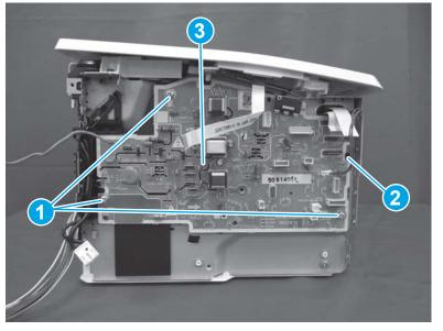
Figure 1-1074 Remove the ECU PCA (SFP)
