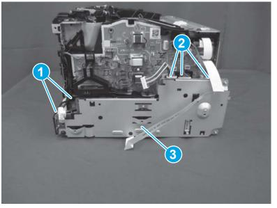
Figure 1-870 Remove the LVPS (MFP)
