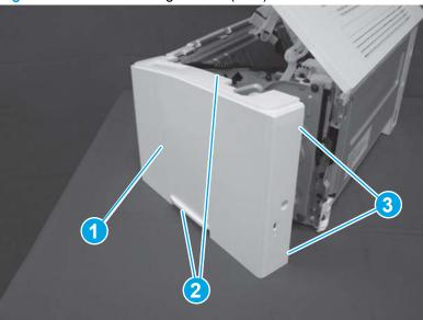
Figure 1-658 Install the right cover (SFP)
