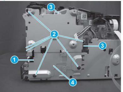
Figure 1-1067 Remove the support plate (MFP)
