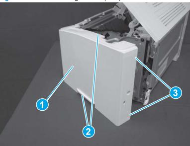
Figure 1-811 Install the right cover (SFP)
