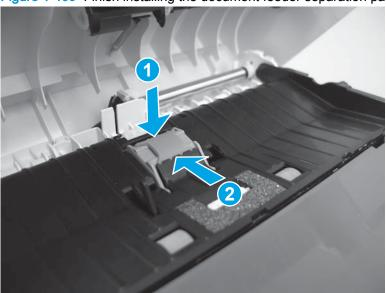
Figure 1-409 Finish installing the document feeder separation pad
