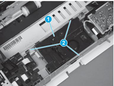
Figure 1-507 Install the laser scanner
