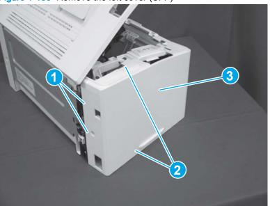
Figure 1-155 Remove the left cover (SFP)
