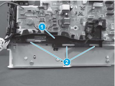
Figure 1-1089 Install the guide (MFP)
