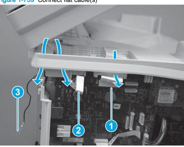
Figure 1-739 Connect flat cable(s)
