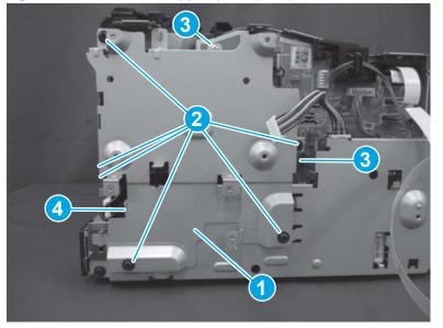
Figure 1-991 Install the support plate (MFP)
