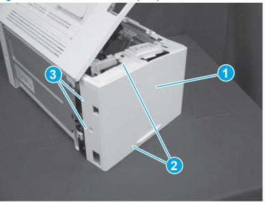
Figure 1-315 Install the left cover (SFP)
