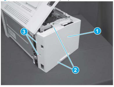
Figure 1-917 Install the left cover (SFP)
