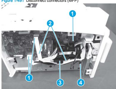
Figure 1-491 Disconnect connectors (MFP)
