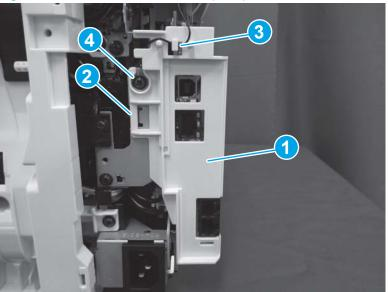
Figure 1-822 Install the USB cover (MFP)
