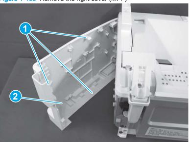
Figure 1-168 Remove the right cover (MFP)
