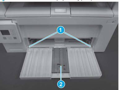
Figure 1-924 Remove the multipurpose tray (MFP)
