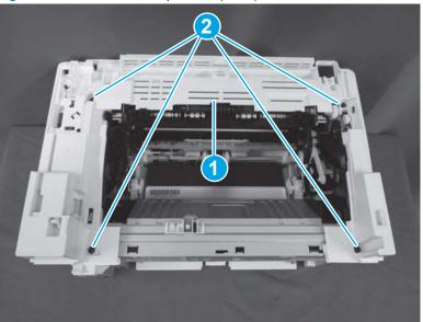
Figure 1-350 Install the top cover (MFP)
