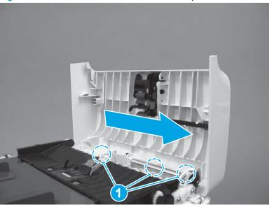
Figure 1-422 Remove the document feeder top cover
