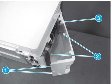
Figure 1-620 Remove the left cover (MFP)
