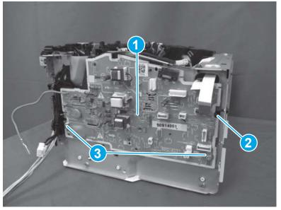
**b.** Slide the guide (callout 1) as shown below to install it, and then engage one boss (callout 2).
