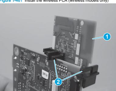
Figure 1-461 Install the wireless PCA (wireless models only)
