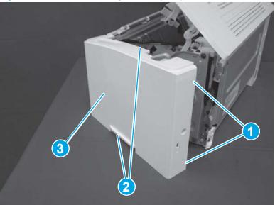
Figure 1-166 Remove the right cover (SFP)
