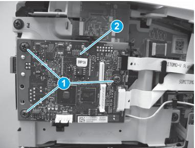
Step 13: Remove the low-voltage power supply (LVPS)
