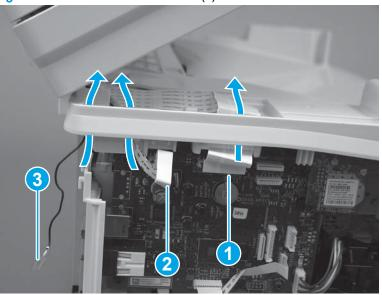
Figure 1-204 Disconnect flat cable(s)
