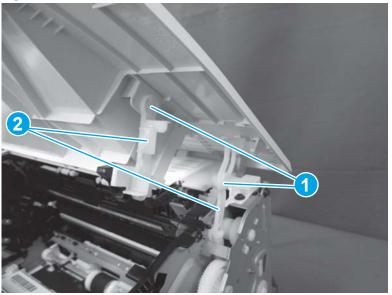
4. Fully open the door, and then slide it towards the right-side of the printer to remove the cartridge door (callout 1).
