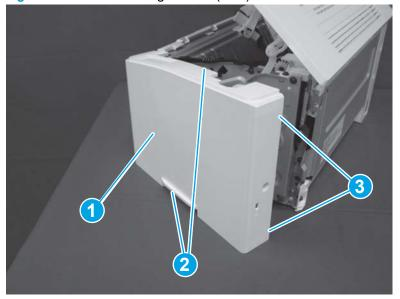
Figure 1-180 Install the right cover (SFP)
