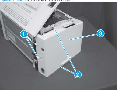
Figure 1-452 Remove the left cover (SFP)
