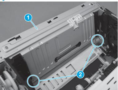
Figure 1-509 Install the laser scanner cover
