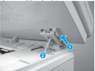
Figure 1-1120 Engage the right hinge (M129/M134)
