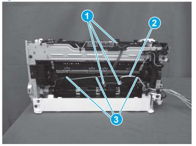
Figure 1-968 Disconnect three connectors
