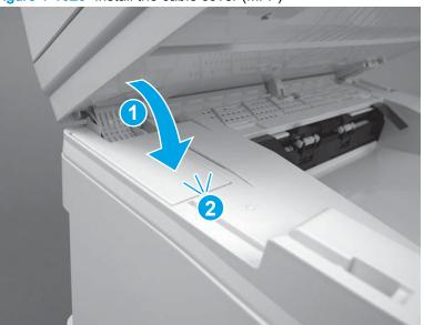
Figure 1-1020 Install the cable cover (MFP)
