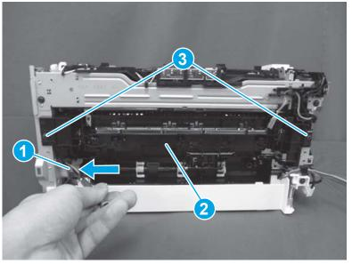
2. Install the wire harnesses (callout 1) in the guide (callout 2), and then connect three connectors (callout 3).
