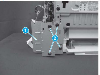
Figure 1-794 Install the plate (MFP)
