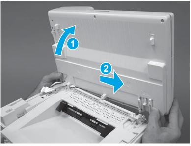
Figure 1-251 Release the left hinge (M129/M134)
