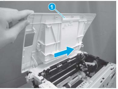
Figure 1-640 Remove the cartridge door
