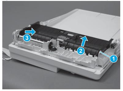
2. Release the wire harness from the guide (callout 1), release the flat cable two-sided tape (callout 2), and then thread the wire harness and flat cable through the opening in the hinge (callout 3) while removing the core assembly (callout 4).
