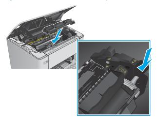
2. Rotate the replacement toner cartridge to the lock position.
