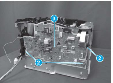
Figure 1-1079 Remove the ECU PCA (MFP)
