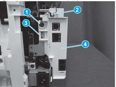
Figure 1-755 Remove the USB cover (MFP)
