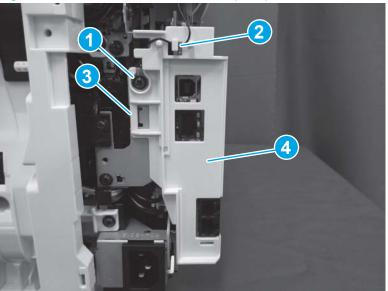
Figure 1-1035 Remove the USB cover (MFP)
