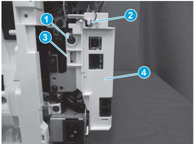
Figure 1-100 Remove the USB cover (MFP)
