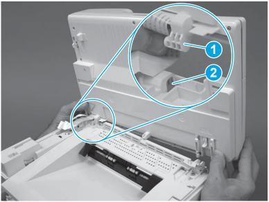
3. Push the right side of the ISA toward the front of the printer to engage the right hinge (callout 1). Make sure that the tab (callout 2) snaps into place.
