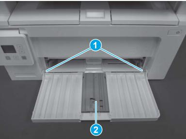
Figure 1-472 Remove the multipurpose tray (MFP)
