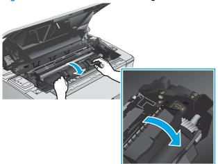
Figure 1-15 Unlock the toner cartridge
