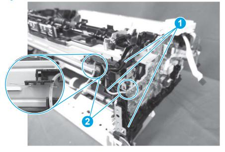
2. Release one boss (callout 1), release two tabs (callout 2), and then slide the guide (callout 3) upward to remove it.
