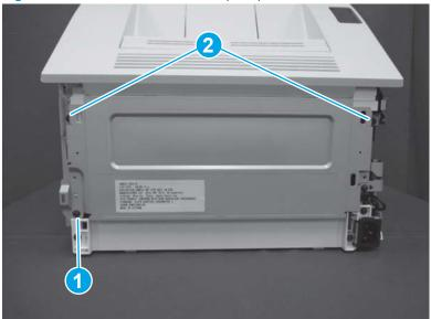
Figure 1-853 Remove one screw (SFP)
