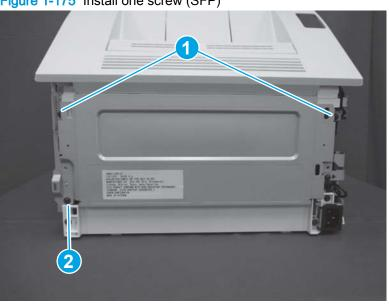
Figure 1-175 Install one screw (SFP)
