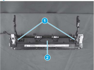
Figure 1-974 Remove the fuser cover
