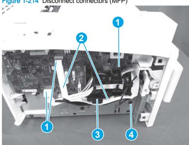
Figure 1-214 Disconnect connectors (MFP)
