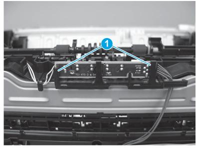
2. Release two tabs (callout 1), and then remove the delivery sensor (callout 2).
