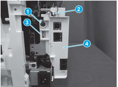
Figure 1-835 Remove the USB cover (MFP)
