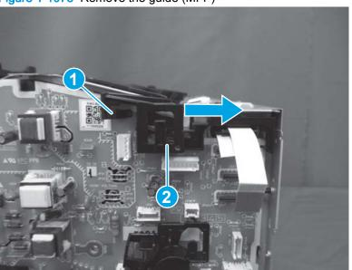
Figure 1-1078 Remove the guide (MFP)
