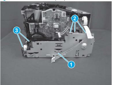
Figure 1-1095 Install the LVPS (MFP)
