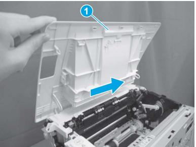
Figure 1-860 Remove the cartridge door
