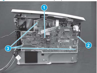
Figure 1-1080 Install the ECU PCA (SFP)
