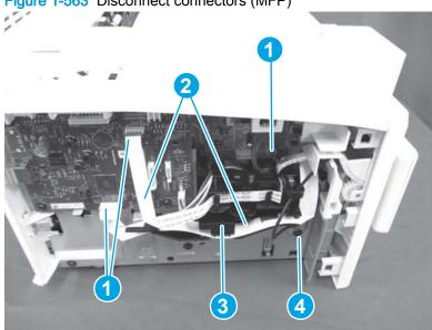
Figure 1-563 Disconnect connectors (MFP)
