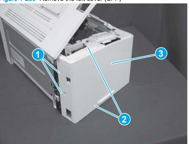
Figure 1-280 Remove the left cover (SFP)
