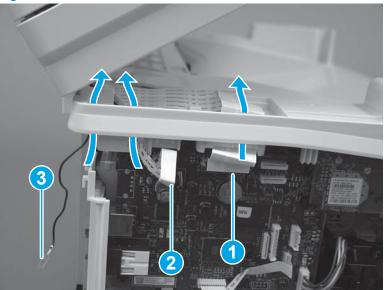
Figure 1-416 Disconnect flat cables
