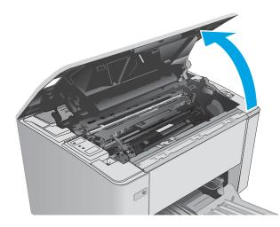
2. Remove the used toner cartridge from the printer.
