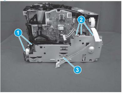
Figure 1-964 Remove the LVPS (MFP)
