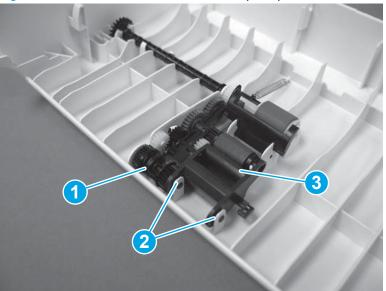
Figure 1-401 Install the document feeder pickup roller
