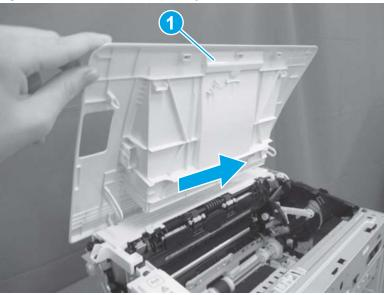
Figure 1-346 Remove the cartridge door
