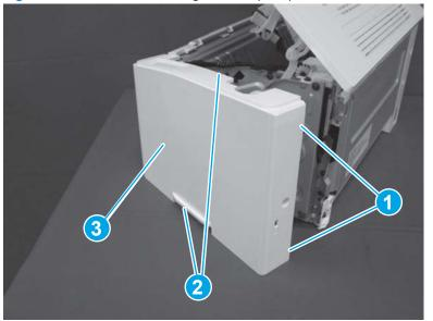
Figure 1-1115 Remove the right cover (SFP)
