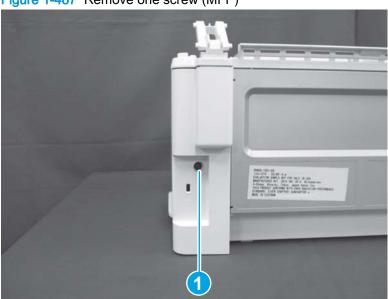
Figure 1-487 Remove one screw (MFP)
