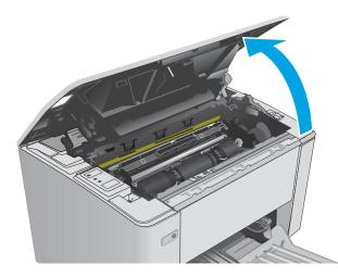
2. Remove the used imaging drum (including the used toner cartridge) from the printer.
