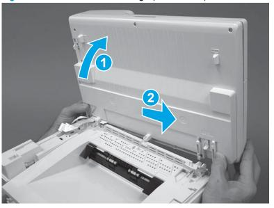
Figure 1-384 Release the left hinge (M129/M134)
