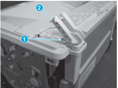
Figure 1-338 Remove the hinge assembly (MFP)
