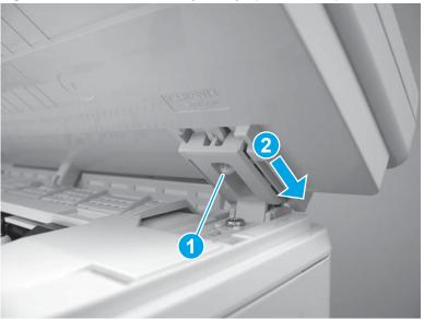
Figure 1-1040 Release the right hinge (M129/M134)
