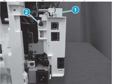
Figure 1-125 Install the ground wire (ISA models)
