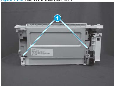
Figure 1-949 Remove two screws (MFP)
