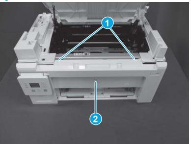
Figure 1-257 Remove the front cover
