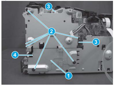
Figure 1-885 Install the support plate (MFP)
