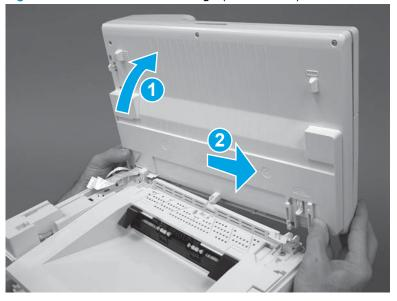
Figure 1-332 Release the left hinge (M129/M134)
