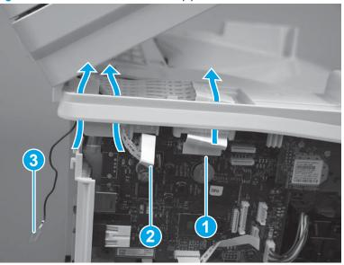
Figure 1-481 Disconnect flat cable(s)
