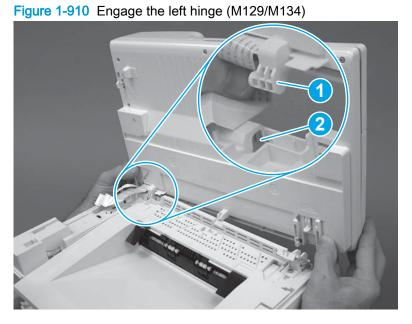
3. Push the right side of the ISA or IS toward the front of the printer to engage the right hinge (callout 1). Make sure that the tab (callout 2) snaps into place.
