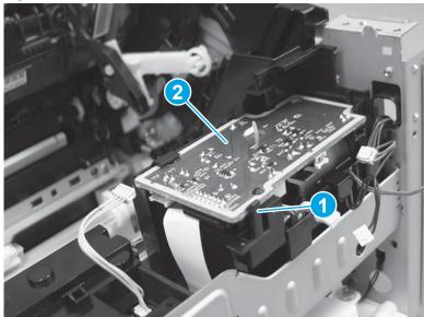
Figure 1-578 Remove the motor PCA
