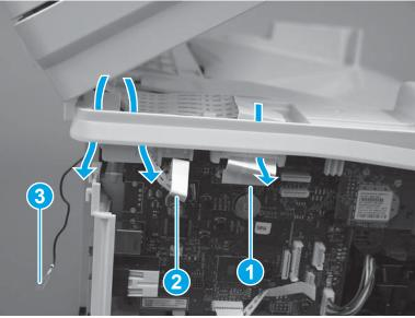
5. **ISA models only**: Install the ground wire in the retainer (callout 1), and then install one screw (callout 2).
