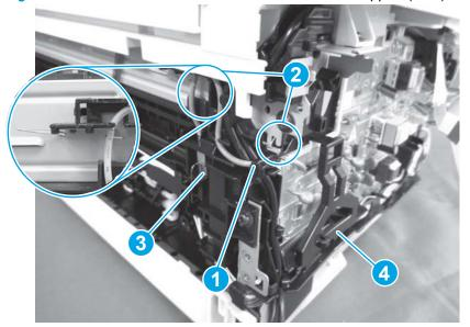
Figure 1-1084 Connect one connector and install the support (SFP)
