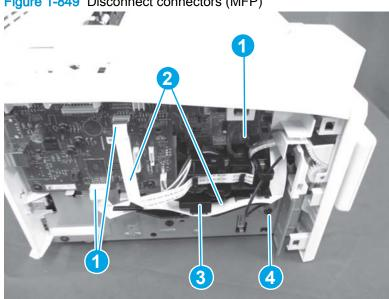
Figure 1-849 Disconnect connectors (MFP)
