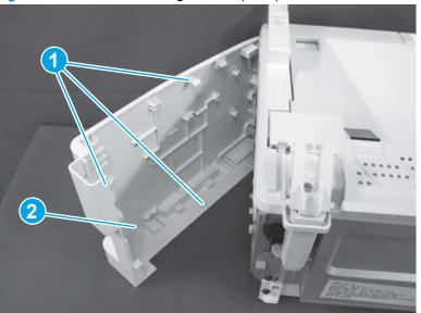
Figure 1-766 Remove the right cover (MFP)
