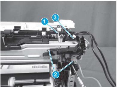
Figure 1-971 Remove the guide
