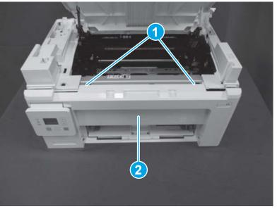
Figure 1-771 Remove the front cover (MFP)
