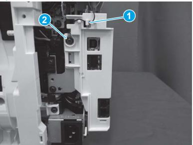
Figure 1-913 Install the ground wire (ISA models)
