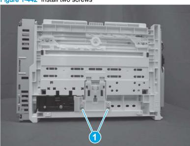
Figure 1-442 Install two screws
