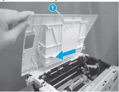
Figure 1-513 Install the cartridge door
