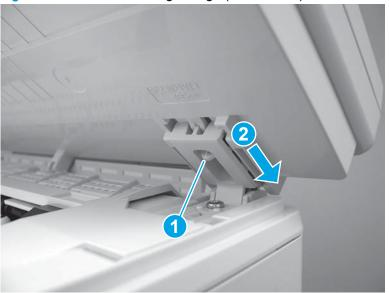
Figure 1-331 Release the right hinge (M129/M134)
