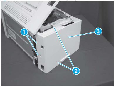
Figure 1-1032 Remove the left cover (SFP)
