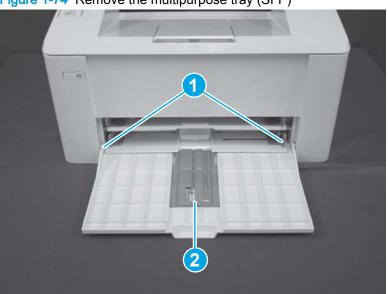
Figure 1-74 Remove the multipurpose tray (SFP)
