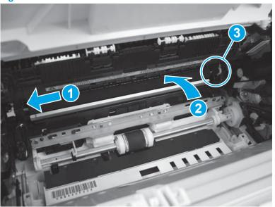
Figure 1-448 Install the roller
