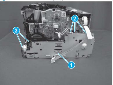
Figure 1-884 Install the LVPS (MFP)
