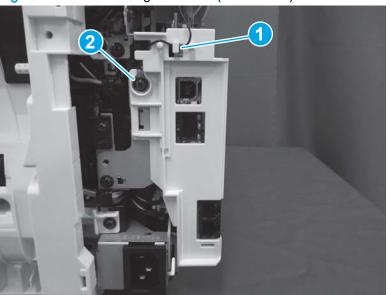
Figure 1-740 Install the ground wire (ISA models)
