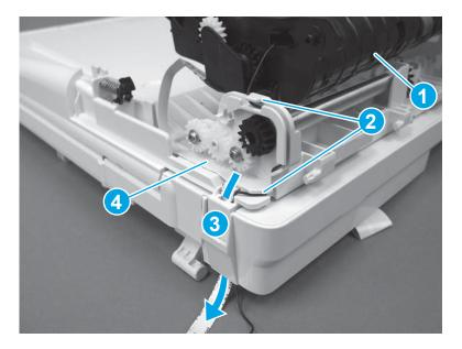
2. Seat the pin on the gear end of the core assembly in the holder (callout 1), carefully lower the assembly into place (callout 2), and then engage one tab (callout 3) to install the assembly.
