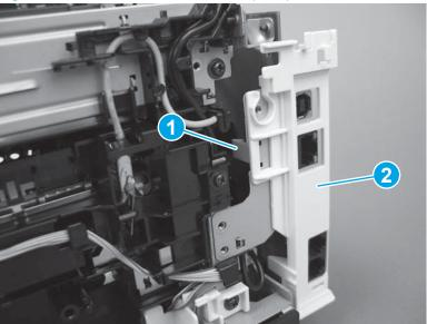
Figure 1-707 Remove the USB cover (MFP)
