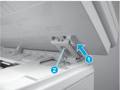
Figure 1-186 Engage the right hinge (M129/M134)
