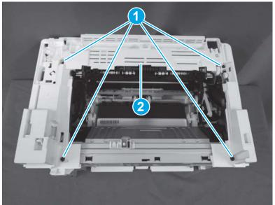
Step 10: Remove the formatter and sheet-metal bracket
