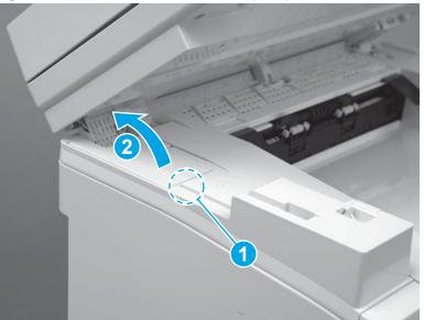
Figure 1-133 Remove the cable cover (MFP)
