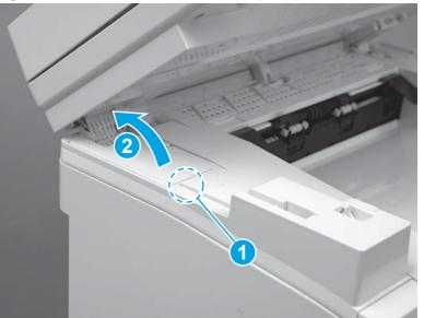
Figure 1-1037 Remove the cable cover (MFP)
