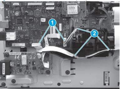
Figure 1-708 Disconnect the connectors (MFP)
