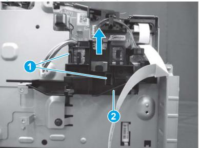
Figure 1-961 Remove the guide (MFP)
