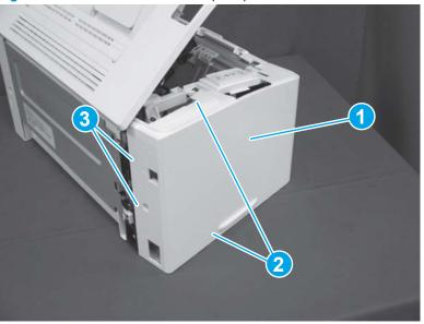
Figure 1-88 Install the left cover (SFP)
