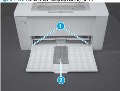
Figure 1-195 Remove the multipurpose tray (SFP)
