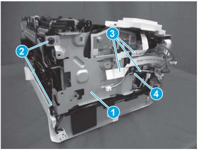
Figure 1-880 Install the support plate (M101/M106)
