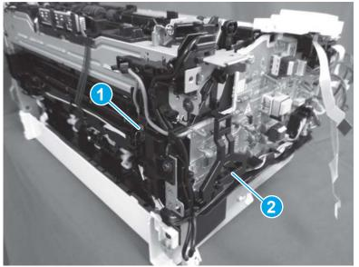
M101/M106 only: Position the support plate (callout 1) on the printer, install two screws (callout 2), and then install the flat cables and the wire harness (callout 3) in the guide (callout 4).
