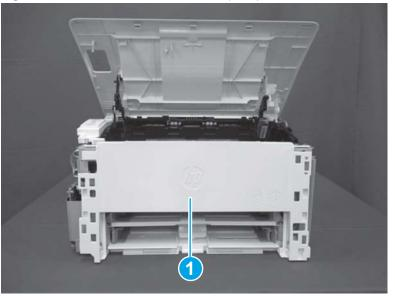
Figure 1-213 Remove the front cover (SFP)
