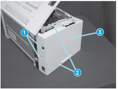
Figure 1-752 Remove the left cover (SFP)
