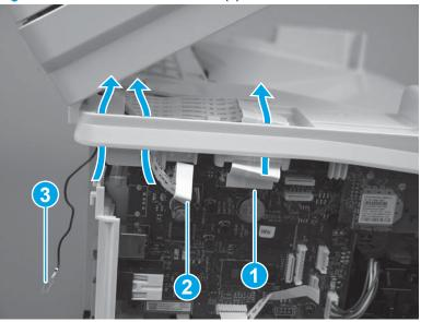
Figure 1-624 Disconnect flat cable(s)
