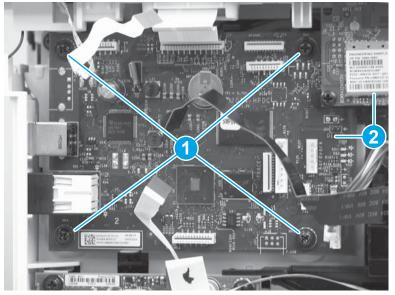
Figure 1-459 Remove the formatter PCA and wireless PCA (M129/M134)
