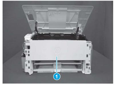
b. Turn the printer over to rest on the rear panel, and then engage two tabs (callout 1).Return the printer the normal position.
