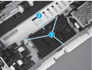
Figure 1-506 Release three springs
