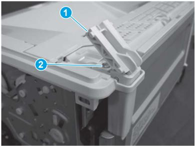
Figure 1-303 Install the hinge assembly (MFP)
