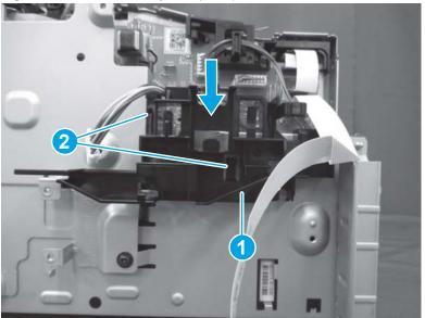
Figure 1-887 Install the guide (MFP)
