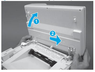
Figure 1-206 Release the left hinge (M129/M134)
