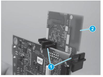
Figure 1-457 Remove the wireless PCA (wireless models only)
