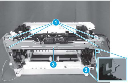
Figure 1-972 Remove the fuser
