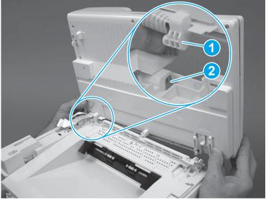
3. Push the right side of the ISA or IS toward the front of the printer to engage the right hinge (callout 1). Make sure that the tab (callout 2) snaps into place.
