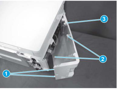
Figure 1-476 Remove the left cover (MFP)
