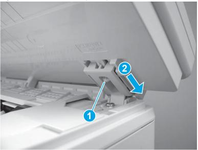
Figure 1-162 Release the right hinge (M129/M134)
