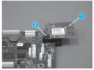
Figure 1-464 Install the wireless PCA (wireless models only)
