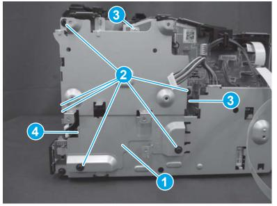
Figure 1-793 Install the support plate (MFP)
