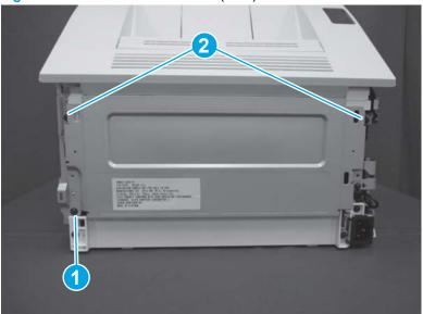
Figure 1-947 Remove one screw (SFP)
