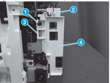
Figure 1-929 Remove the USB cover (MFP)
