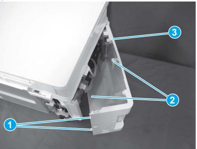
Figure 1-282 Remove the left cover (MFP)
