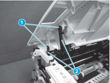
2. Before proceeding, note that the lower right-side link arm (callout 1) is connected with a small white-plastic clip (callout 2). Do not drop the clip into the printer when it is removed.
