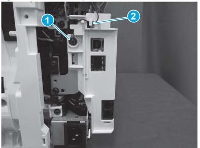
Figure 1-248 Release the ground wire (ISA models)
