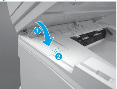
Figure 1-741 Install the cable cover (MFP)
