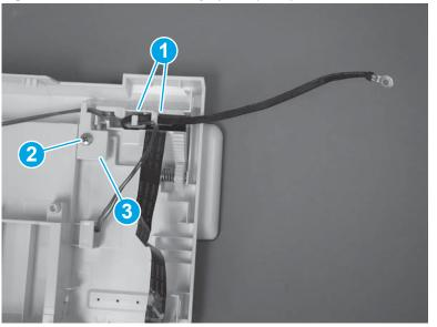
Figure 1-258 Remove the hinge plate (MFP)
