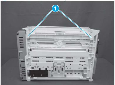
Figure 1-212 Release two tabs (SFP)
