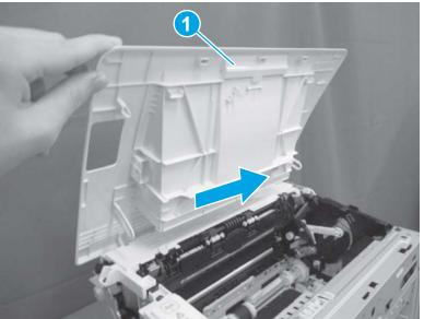
Figure 1-778 Remove the cartridge door
