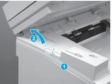
Figure 1-328 Remove the cable cover (MFP)
