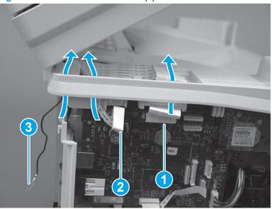
Figure 1-286 Disconnect flat cable(s)
