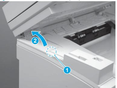
Figure 1-247 Remove the cable cover (MFP)
