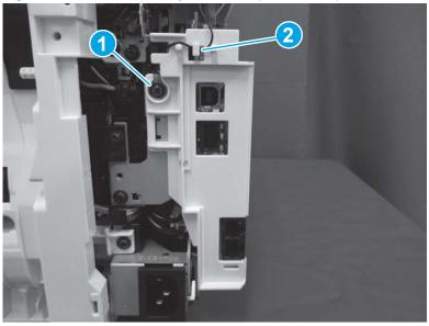
2. **ISA models only**: Disconnect two flat cables (callout 1/2), and then pass the flat cables and the ground wire (callout 3) through the opening in the chassis.
