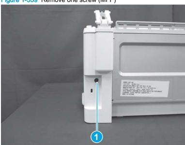
Figure 1-559 Remove one screw (MFP)
