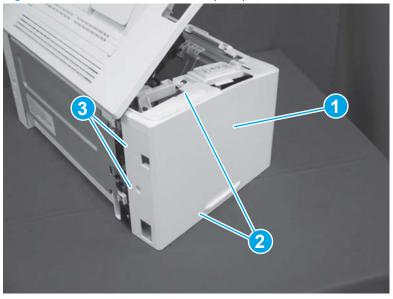
Figure 1-1023 Install the left cover (SFP)
