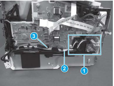
Figure 1-873 Disconnect five connectors
