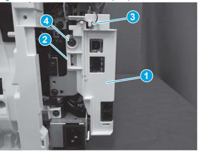
Figure 1-1125 Install the USB cover (MFP)
