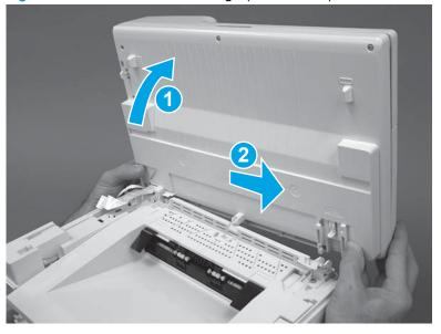
Figure 1-483 Release the left hinge (M129/M134)
