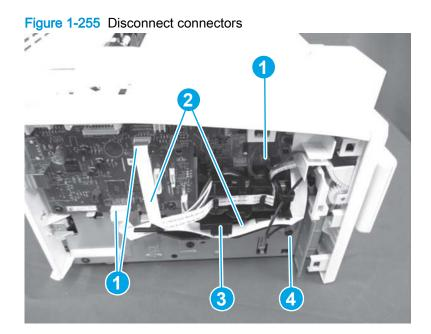
2. Turn the printer over to rest on the rear panel, and then release two tabs (callout 1).
