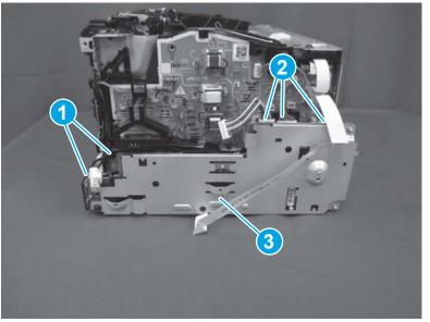
Figure 1-788 Remove the LVPS (MFP)
