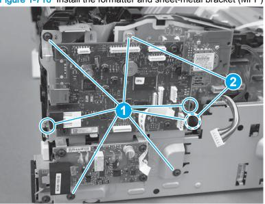
Figure 1-716 Install the formatter and sheet-metal bracket (MFP)
