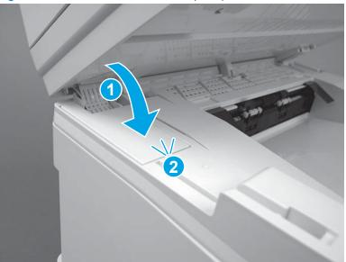
Figure 1-534 Install the cable cover (MFP)
