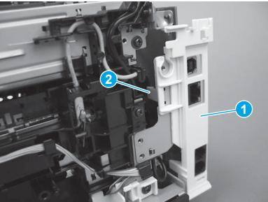
Figure 1-719 Install the USB cover (MFP)
