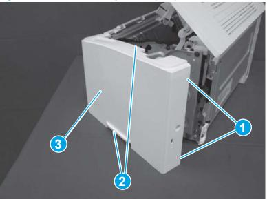
Figure 1-689 Remove the right cover (SFP)
