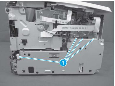
Figure 1-791 Connect four connectors (SFP)
