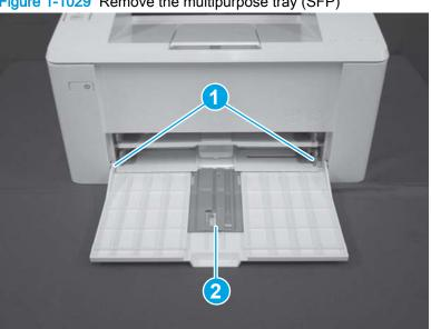
Figure 1-1029 Remove the multipurpose tray (SFP)
