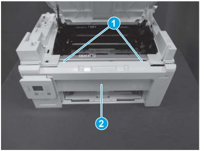
Figure 1-493 Remove the front cover (MFP)
