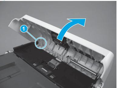
3. Slide the top cover as shown below to release three hinge pins (callout 1), and then remove the cover.
