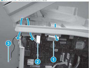
Figure 1-148 Connect flat cable(s)
