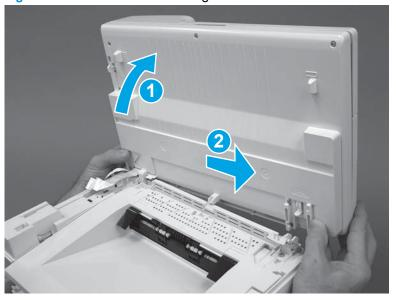
Figure 1-418 Release the left hinge
