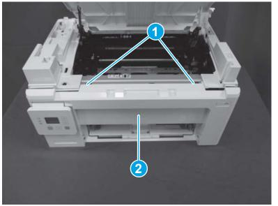
Figure 1-216 Remove the front cover (MFP)
