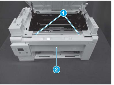
Figure 1-851 Remove the front cover (MFP)
