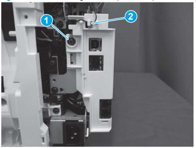
Figure 1-134 Release the ground wire (ISA models)
