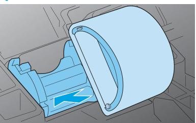
Figure 1-39 Install the roller
