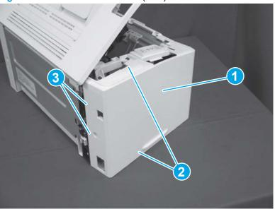
Figure 1-371 Install the left cover (SFP)
