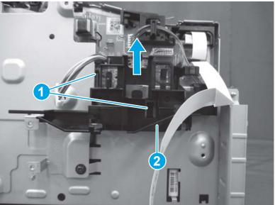
Figure 1-785 Remove the guide (MFP)
