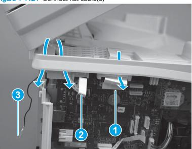
Figure 1-1121 Connect flat cable(s)
