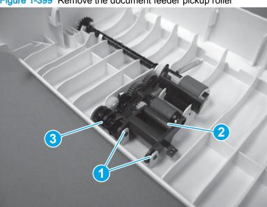
Figure 1-399 Remove the document feeder pickup roller
