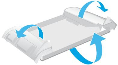
2. With the dust cover in the closed (down) position, insert the left-side hinge pin in the holder, and then install the right-side hinge pin the other holder.
