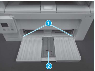
Figure 1-1030 Remove the multipurpose tray (MFP)
