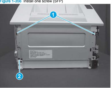
Figure 1-356 Install one screw (SFP)
