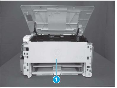
Turn the printer over to rest on the rear panel, and then engage two tabs (callout 1).
