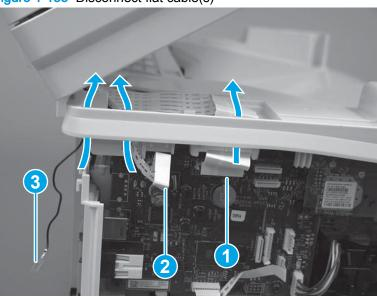
Figure 1-135 Disconnect flat cable(s)
