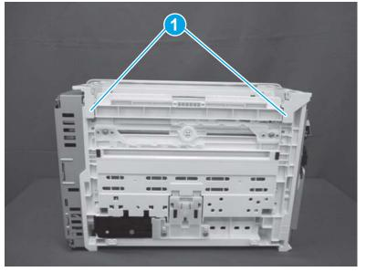
Figure 1-521 Engage two tabs (M101/M106)
