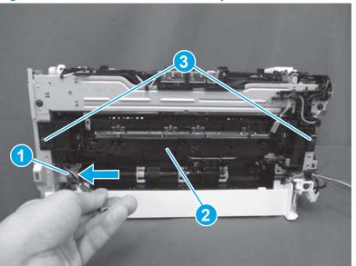
Figure 1-876 Install the transfer assembly
