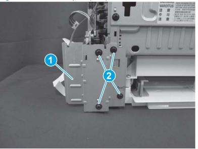
Figure 1-886 Install the plate (MFP)
