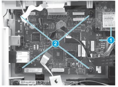
Figure 1-465 Install the formatter PCA and wireless PCA (M129/M134)
