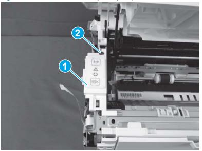
Figure 1-536 Install the control panel (SFP)
