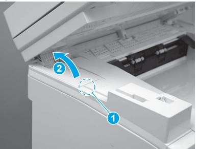
Figure 1-284 Remove the cable cover (MFP)
