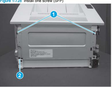
Figure 1-728 Install one screw (SFP)
