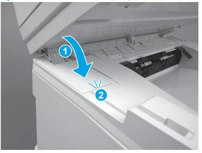
Figure 1-369 Install the cable cover (MFP)
