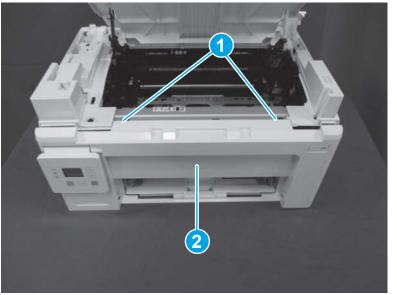
Figure 1-565 Remove the front cover (MFP)
