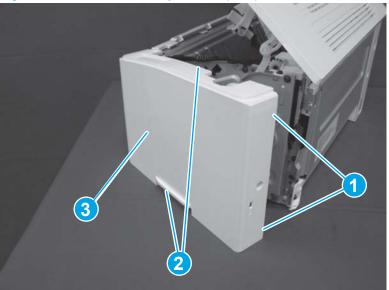
Figure 1-114 Remove the right cover (SFP)
