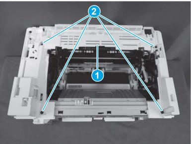
Figure 1-648 Install the top cover (MFP)
