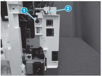
Figure 1-381 Release the ground wire (ISA models)
