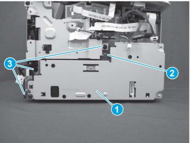
Figure 1-881 Install the LVPS (SFP)
