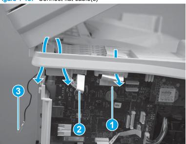
Figure 1-187 Connect flat cable(s)
