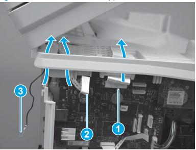
Figure 1-1039 Disconnect flat cable(s)
