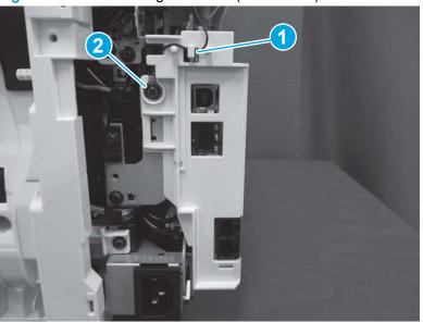
Figure 1-312 Install the ground wire (ISA models)
