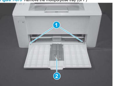
Figure 1-675 Remove the multipurpose tray (SFP)
