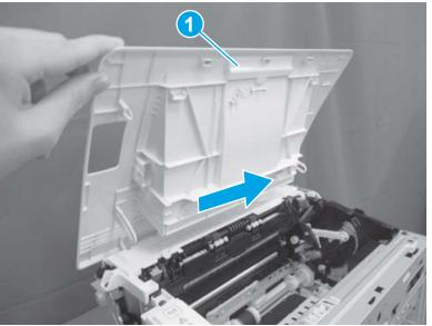
Figure 1-298 Remove the cartridge door
