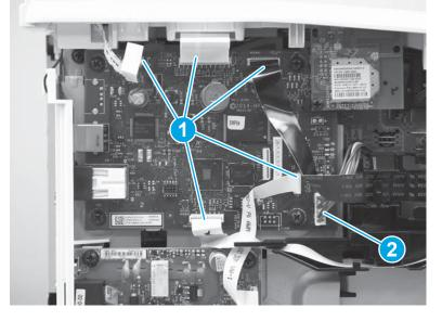
Figure 1-458 Disconnect five flat cables and one connector (M129/M134)
