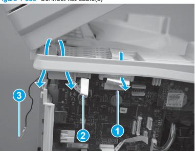
Figure 1-389 Connect flat cable(s)
