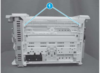
3. Return the printer the normal position, open the cartridge door, release two bosses (callout 1), and then remove the front cover (callout 2).
