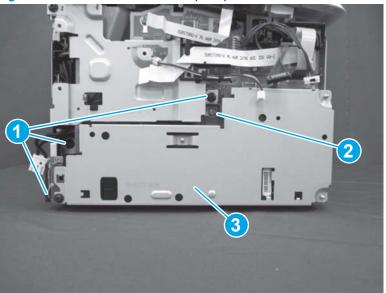
Figure 1-959 Remove the LVPS (SFP)
