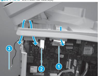
Figure 1-1018 Connect flat cable(s)
