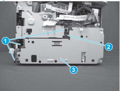
Figure 1-783 Remove the LVPS (SFP)
