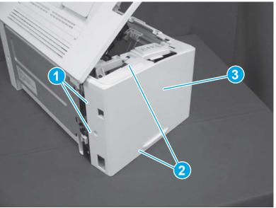
Figure 1-678 Remove the left cover (SFP)
