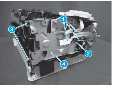
Figure 1-1085 Install the support plate (SFP)
