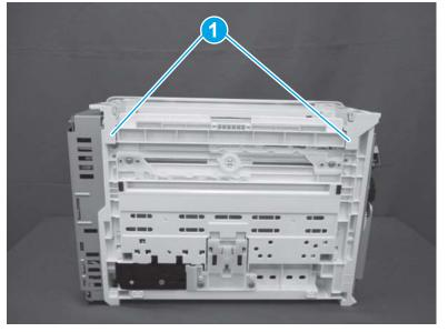
Figure 1-807 Engage two tabs (M101/M106)
