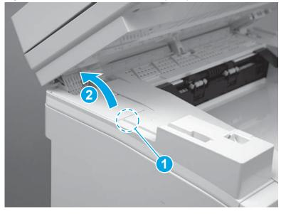
Figure 1-79 Remove the cable cover (MFP)
