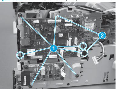
Figure 1-710 Remove seven screws (MFP)
