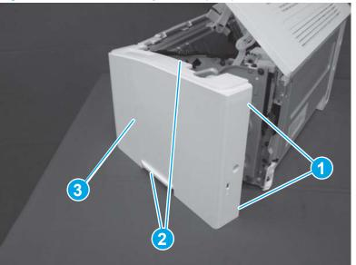
Figure 1-209 Remove the right cover (SFP)
