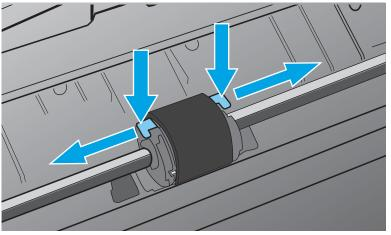
5. Rotate the top of the roller up and off the holder to remove the roller.
