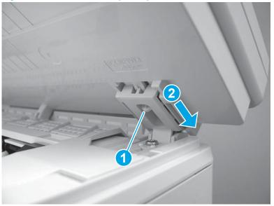
Figure 1-417 Release the right hinge
