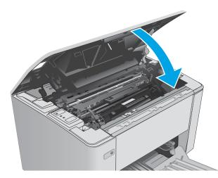
Remove and replacement: Toner cartridge and image drum (M129-M133)
