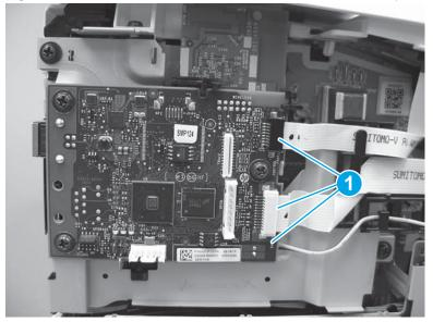
**b.** Remove three screws (callout 1), and then remove the formatter PCA and wireless PCA (callout 2).
