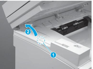
Figure 1-202 Remove the cable cover (MFP)
