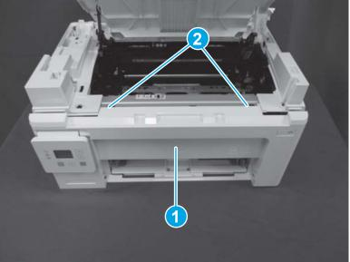
c. Turn the printer over to rest on the rear panel, and then engage two tabs (callout 1).Return the printer the normal position.
