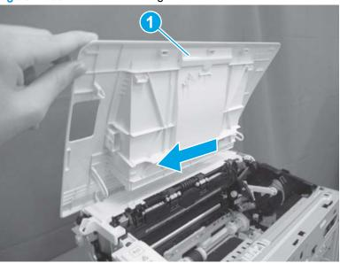
Figure 1-799 Install the cartridge door
