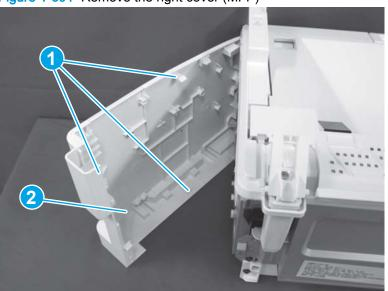
Figure 1-691 Remove the right cover (MFP)
