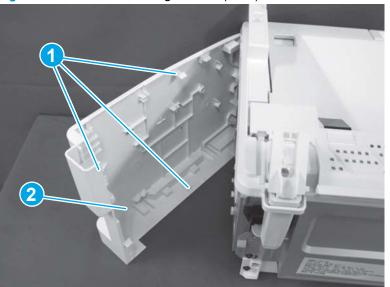
Figure 1-116 Remove the right cover (MFP)
