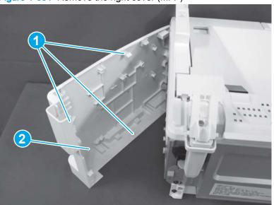
Figure 1-631 Remove the right cover (MFP)
