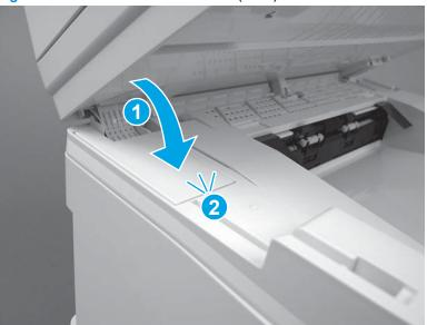
Figure 1-820 Install the cable cover (MFP)
