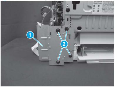
Figure 1-1097 Install the plate (MFP)
