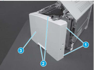
Figure 1-291 Remove the right cover (SFP)
