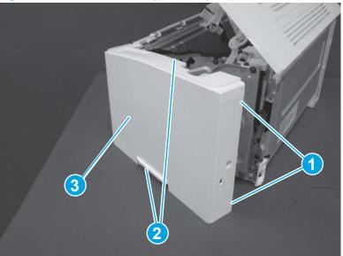
Figure 1-1044 Remove the right cover (SFP)
