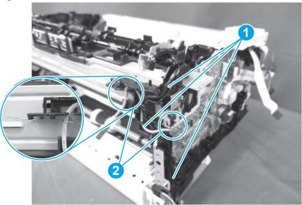
Figure 1-981 Install the wire harnesses
