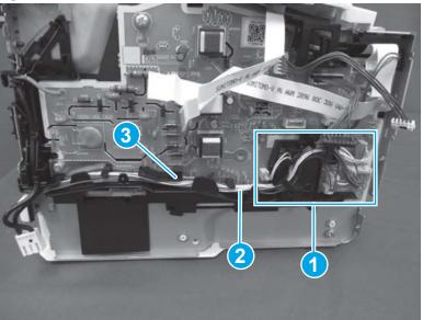
Figure 1-967 Disconnect five connectors
