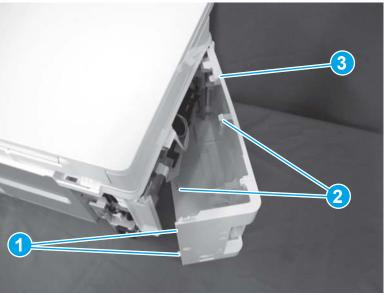
Figure 1-834 Remove the left cover (MFP)
