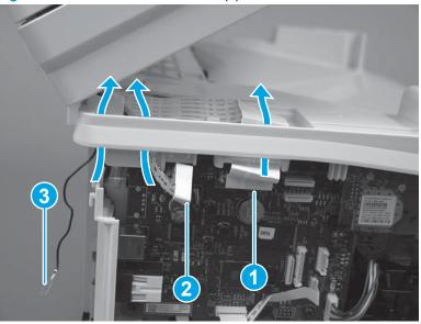
Figure 1-933 Disconnect flat cable(s)
