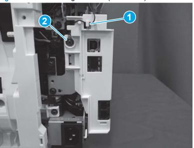
Figure 1-533 Install the ground wire (ISA models)
