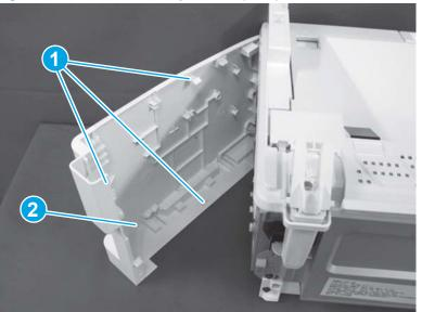
Figure 1-488 Remove the right cover (MFP)
