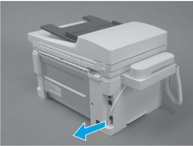
2. Open the integrated scanner assembly (ISA).
