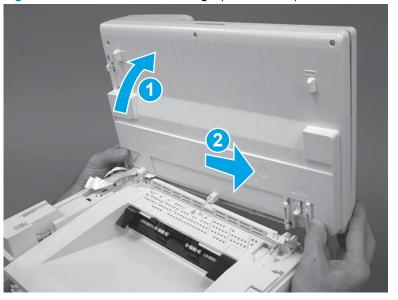
Figure 1-761 Release the left hinge (M129/M134)
