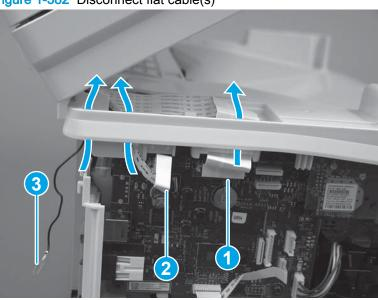
Figure 1-382 Disconnect flat cable(s)
