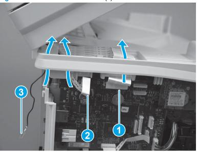
Figure 1-161 Disconnect flat cable(s)
