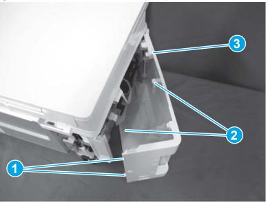
Figure 1-454 Remove the left cover (MFP)
