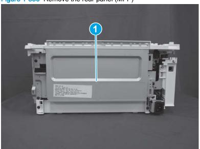
Figure 1-856 Remove the rear panel (MFP)
