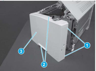
Figure 1-629 Remove the right cover (SFP)
