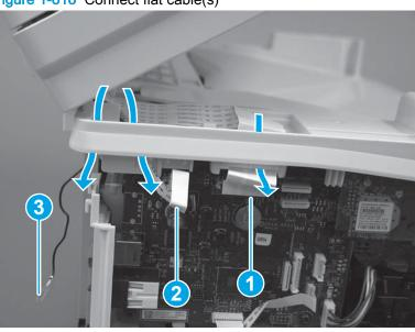
Figure 1-818 Connect flat cable(s)
