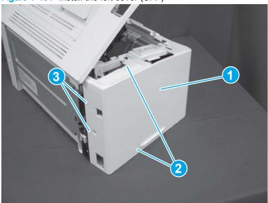
Figure 1-191 Install the left cover (SFP)
