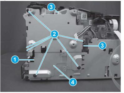
Figure 1-963 Remove the support plate (MFP)
