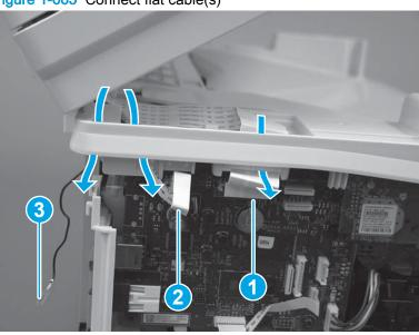
Figure 1-665 Connect flat cable(s)
