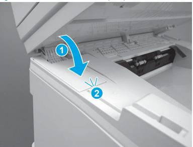
Figure 1-313 Install the cable cover (MFP)
