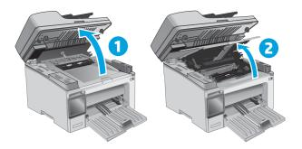
2. Remove the used toner cartridge from the printer.
