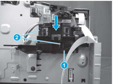
Figure 1-993 Install the guide (MFP)
