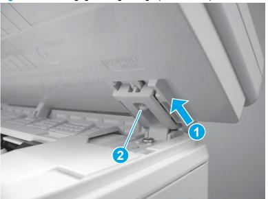
Figure 1-1017 Engage the right hinge (M129/M134)
