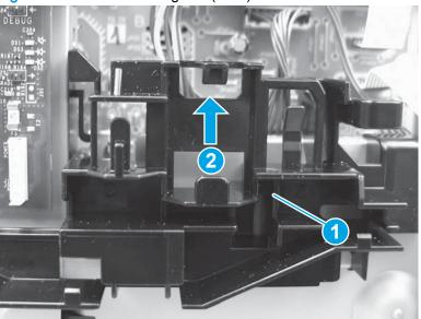
Figure 1-709 Remove the guide (MFP)
