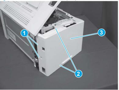
Figure 1-474 Remove the left cover (SFP)
