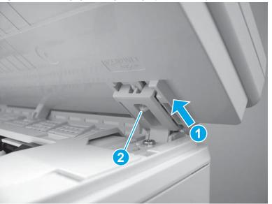
Figure 1-310 Engage the right hinge (M129/M134)
