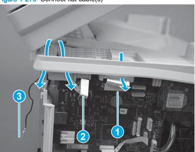
Figure 1-270 Connect flat cable(s)
