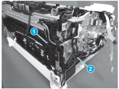
5. M101/M106 only: Position the support plate (callout 1) on the printer, install two screws (callout 2), and then install the flat cables and the wire harness (callout 3) in the guide (callout 4).
