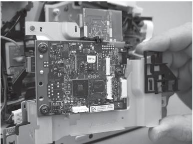
Figure 1-705 Remove the formatter and sheet-metal bracket (SFP)
