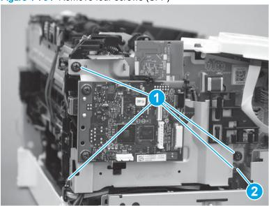
Figure 1-704 Remove four screws (SFP)
