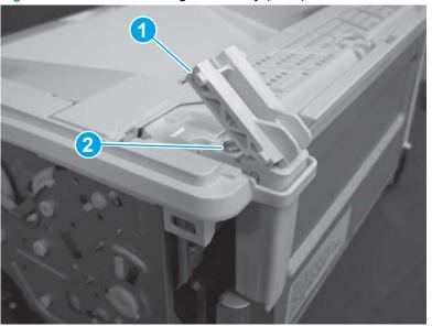
Figure 1-519 Install the hinge assembly (MFP)
