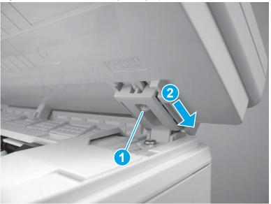
Figure 1-685 Release the right hinge (M129/M134)
