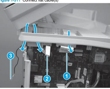
Figure 1-311 Connect flat cable(s)
