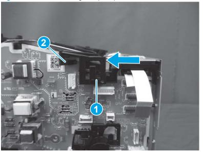
Figure 1-1088 Install the guide (MFP)
