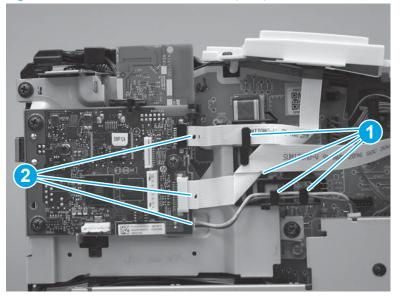
Figure 1-714 Connect the connectors (SFP)
