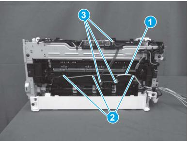
Figure 1-877 Connect three connectors
