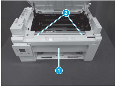
b. Turn the printer over to rest on the rear panel, and then engage two tabs (callout 1).
