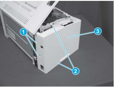
Figure 1-198 Remove the left cover (SFP)
