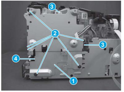
Figure 1-1096 Install the support plate (MFP)
