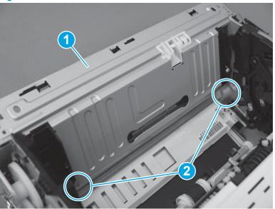
Figure 1-581 Install the laser scanner cover
