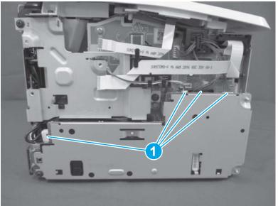
Figure 1-1061 Disconnect four connectors (SFP)
