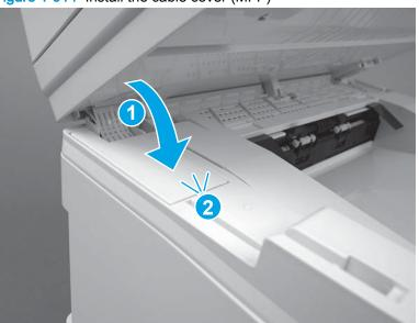
Figure 1-914 Install the cable cover (MFP)
