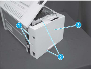
Figure 1-832 Remove the left cover (SFP)
