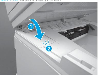
Figure 1-189 Install the cable cover (MFP)
