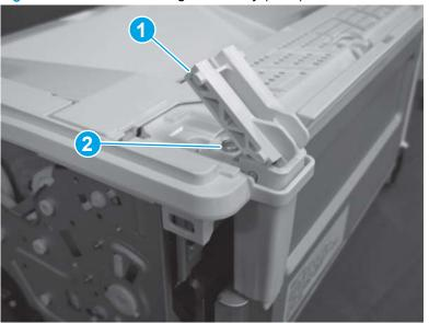
Figure 1-805 Install the hinge assembly (MFP)
