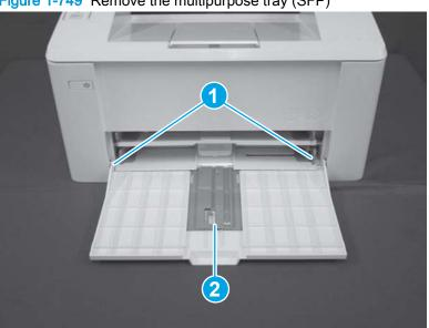
Figure 1-749 Remove the multipurpose tray (SFP)
