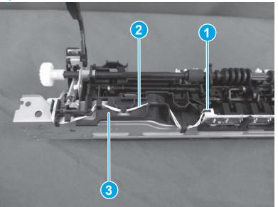
Figure 1-973 Disconnect one connector
