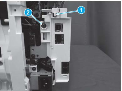
Figure 1-368 Install the ground wire (ISA models)
