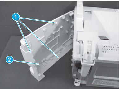
Figure 1-211 Remove the right cover (MFP)
