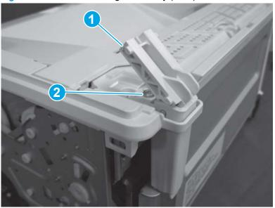
Figure 1-179 Install the hinge assembly (MFP)
