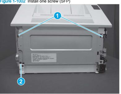
Figure 1-1002 Install one screw (SFP)
