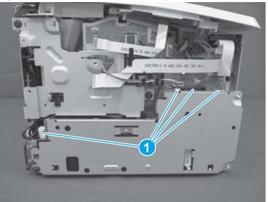
Figure 1-1094 Connect four connectors (SFP)
