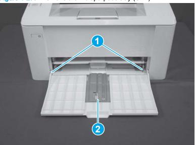
Figure 1-277 Remove the multipurpose tray (SFP)
