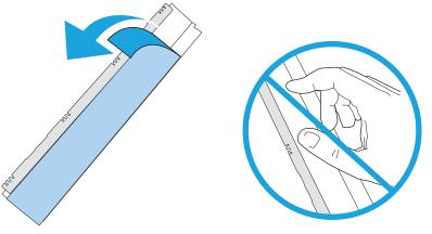
2. Position the mylar ramp on the image scanner.
