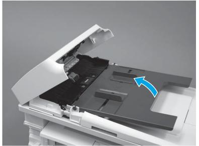
3. Pull the input tray straight up and off of the printer to remove it.
