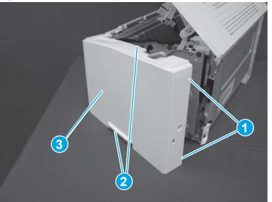
Figure 1-335 Remove the right cover (SFP)
