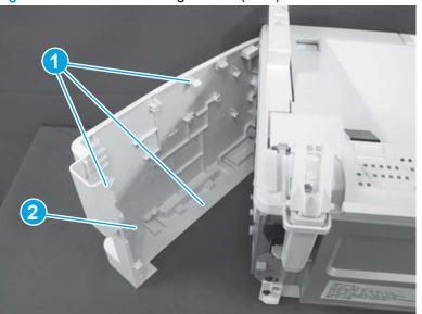
Figure 1-940 Remove the right cover (MFP)
