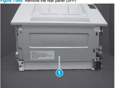
Figure 1-948 Remove the rear panel (SFP)
