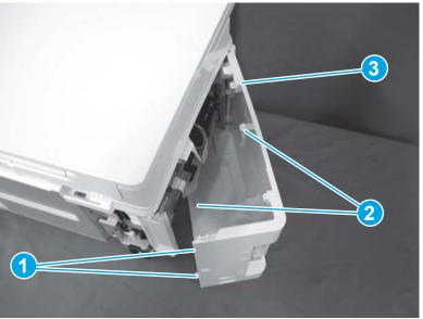
Figure 1-754 Remove the left cover (MFP)
