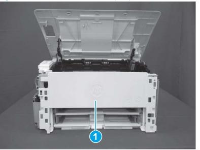
Figure 1-768 Remove the front cover (SFP)
