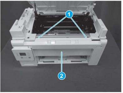
Figure 1-1051 Remove the front cover (MFP)
