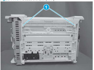
Figure 1-770 Release two tabs (MFP)
