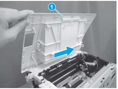
Figure 1-700 Remove the cartridge door
