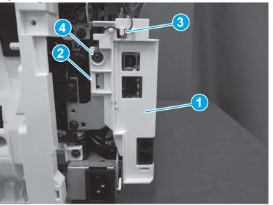
Figure 1-1022 Install the USB cover (MFP)
