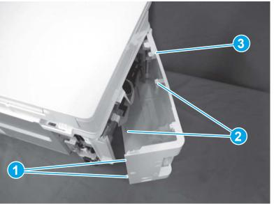
Figure 1-86 Remove the left cover (MFP)
