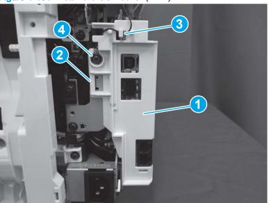
Figure 1-101 Install the USB cover (MFP)
