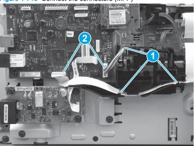
Figure 1-718 Connect the connectors (MFP)
