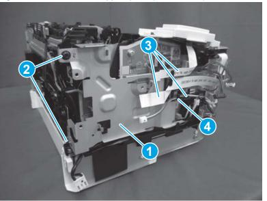
Figure 1-986 Install the support plate (M101/M106)
