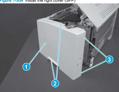
Figure 1-304 Install the right cover (SFP)
