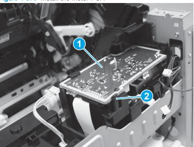
Figure 1-579 Install the motor PCA
