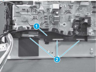
Figure 1-1082 Install the guide (SFP)
