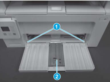
Figure 1-830 Remove the multipurpose tray (MFP)
