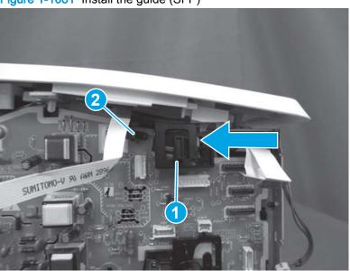
Figure 1-1081 Install the guide (SFP)
