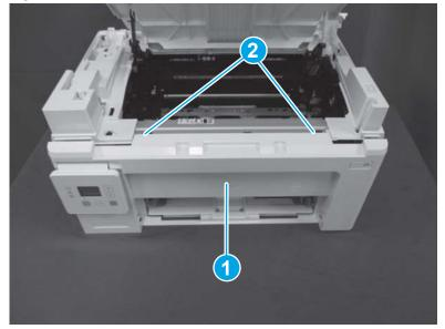
2. Turn the printer over to rest on the rear panel, and then engage two tabs (callout 1).
