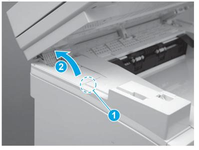
Figure 1-414 Remove the cable cover (MFP)
