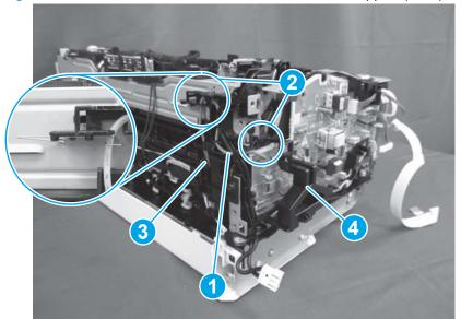
Figure 1-1091 Connect one connector and install the support (MFP)
