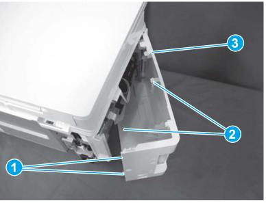
Figure 1-680 Remove the left cover (MFP)
