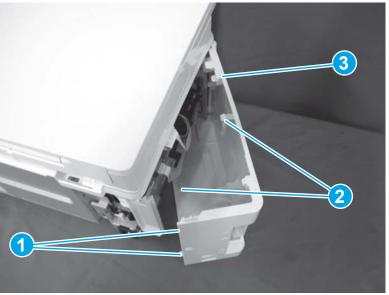
Figure 1-928 Remove the left cover (MFP)
