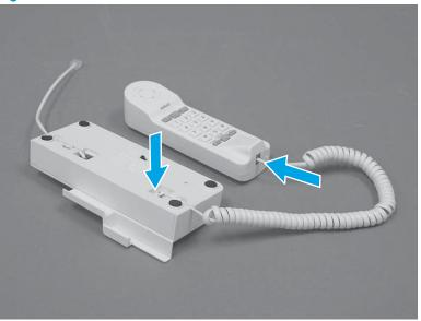
Figure 1-53 Connect the receiver cord
