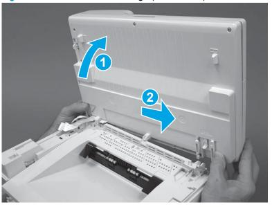
Figure 1-137 Release the left hinge (M129/M134)
