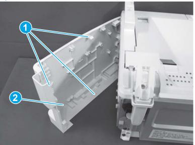
Figure 1-1046 Remove the right cover (MFP)
