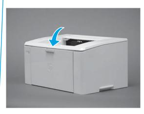
4. M129/M134 only: Close the integrated scanner assembly (ISA) or the image scanner (IS).
