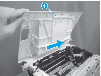
Figure 1-500 Remove the cartridge door
