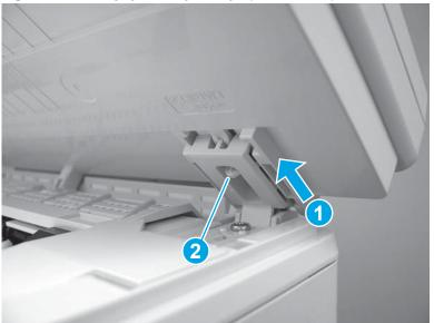
Figure 1-269 Engage the right hinge (M129/M134)
