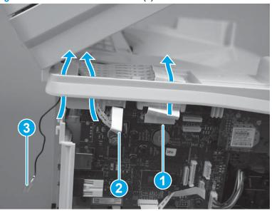
Figure 1-553 Disconnect flat cable(s)
