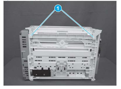
Figure 1-1110 Engage two tabs (M101/M106)
