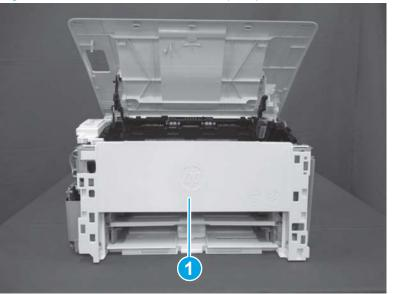
Figure 1-848 Remove the front cover (SFP)
