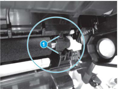
Figure 1-445 Transfer roller right collar tabs
