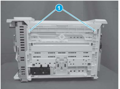
**c.** Return the printer the normal position, open the cartridge door, release two bosses (callout 1), and then remove the front cover (callout 2).
