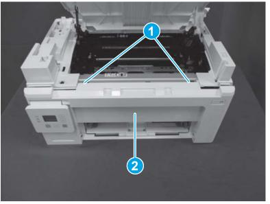
Figure 1-945 Remove the front cover (MFP)
