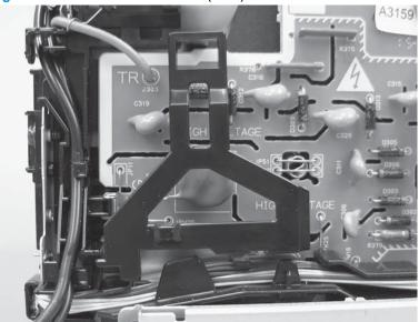
Figure 1-712 Install the standoff (SFP)
