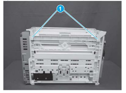
Figure 1-901 Engage two tabs (M101/M106)
