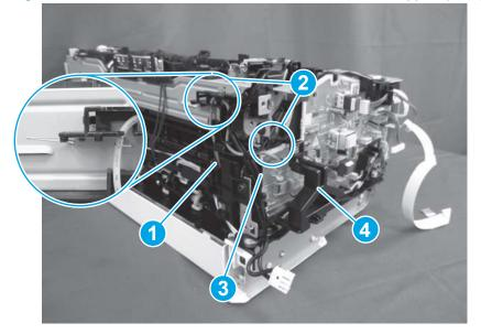
Figure 1-1075 Disconnect one connector and remove the support (MFP)
