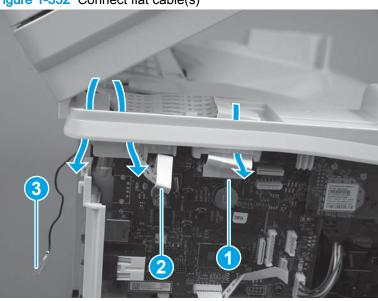
Figure 1-532 Connect flat cable(s)
