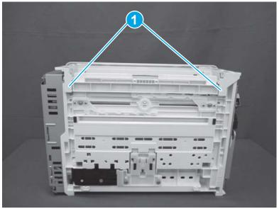
b. Return the printer the normal position, open the cartridge door, and then remove the front cover (callout 1).
