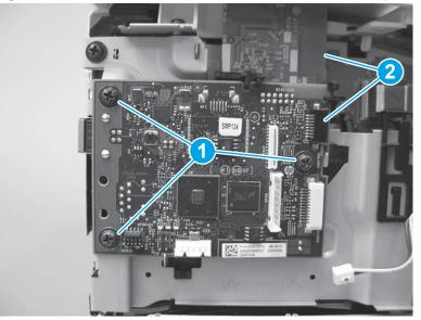
Figure 1-456 Remove the formatter PCA and wireless PCA (M101/M106)
