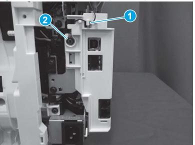
Figure 1-271 Install the ground wire (ISA models)
