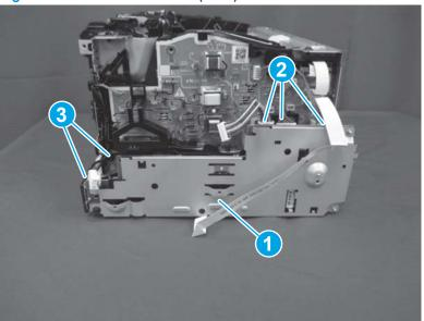
Figure 1-792 Install the LVPS (MFP)
