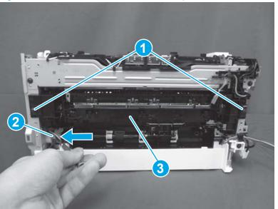
Figure 1-969 Remove the transfer assembly
