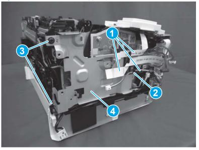
2. Disconnect one connector (callout 1), and then remove the black-plastic support bracket (callout 2).
