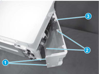
Figure 1-200 Remove the left cover (MFP)
