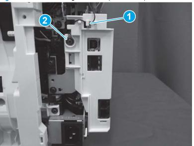
Figure 1-819 Install the ground wire (ISA models)
