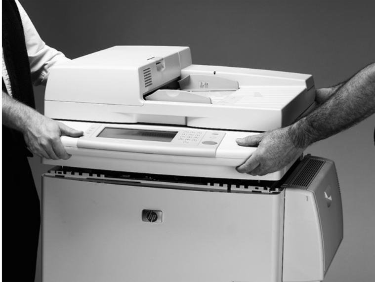
📝 **NOTE:** As you remove the scan engine assembly, two black plastic spacer rings (see figure) fall into the top of the print engine under the rear alignment holes. These rings cannot be reinstalled, but removing them is recommended to ensure that they do not interfere with printing operations.
