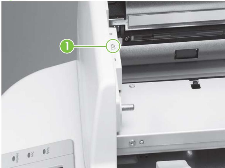
2. Slightly lift the ADF front cover, and slide the cover to the left to disengage two claws (not visible). Lift to remove the cover.
