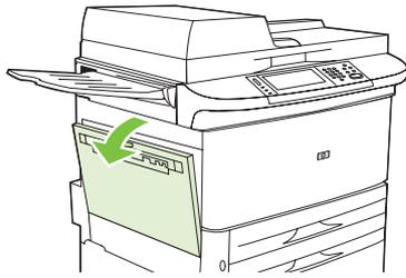
3. Remove any jammed or damaged media from this area by pulling it out of the product.
