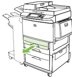
2. Press the tab on the front paper guide, and slide the guide all the way out.
