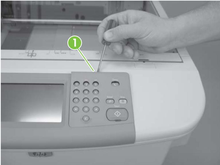
3. Insert a small flat blade screwdriver in the notch on the side of the control panel and press the tab (callout 2) while lifting the control panel. Repeat for the other side, and then disconnect the connector on the back of the control panel.
