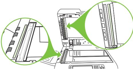
6. Clean the ADF backing and the calibration strips by wiping them with a clean, damp, lint-free cloth.
