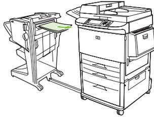
3. Open the back door on the finisher. If jammed paper inside the finisher has not entered the folding rollers, remove the paper and then skip to step 7. If the paper has entered the folding rollers, proceed to step 4.
