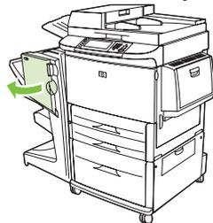
5. Turn the bottom green knob clockwise to advance the jammed paper through the folding rollers and into the booklet bin.
