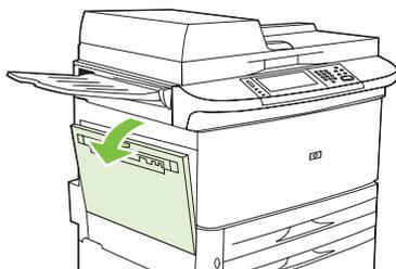
3. Remove the duplex printing accessory by pressing the green lever and pulling the unit out until it stops.
