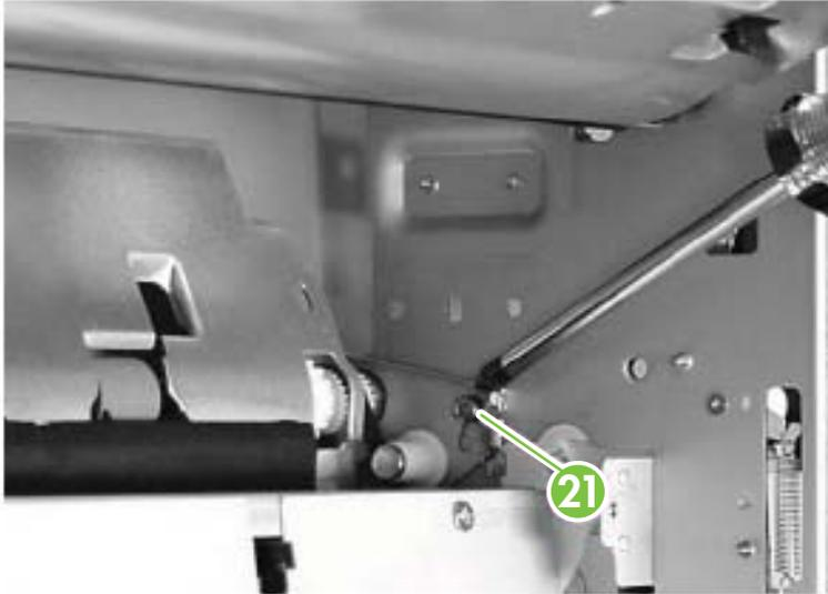
22. Rotate the plate to relieve tension on the registration belt, and then retighten the screw.
