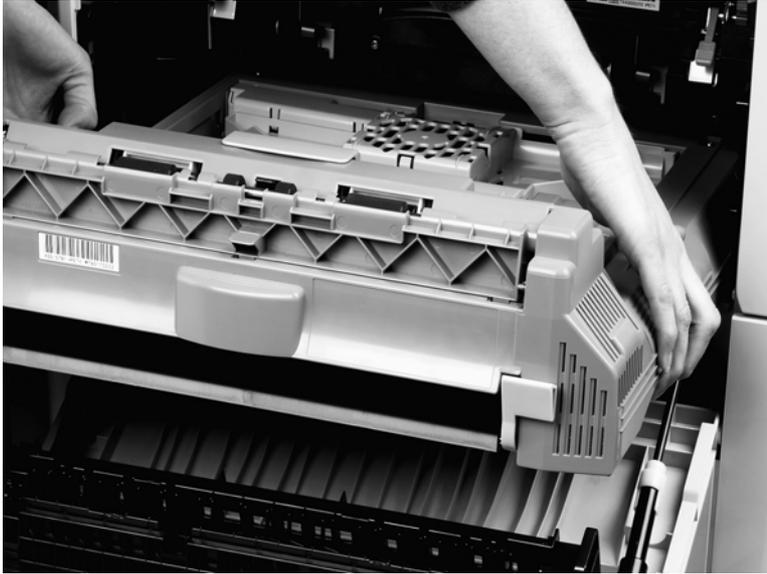
5. Lift the duplexer up to release two underside catches, and then remove it.
