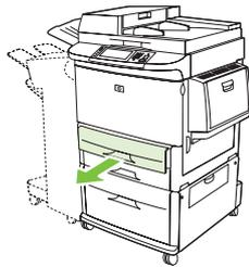
2. Check for media in the tray area, and remove any media from this area. Carefully check to be sure you have removed all pieces of torn media.
