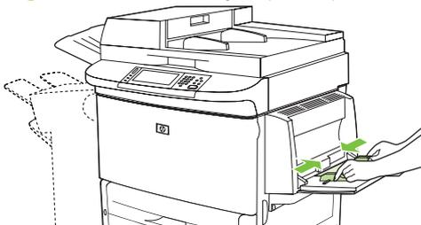
4. Make sure the paper fits under the tabs on the guides and not above the load level indicators.
