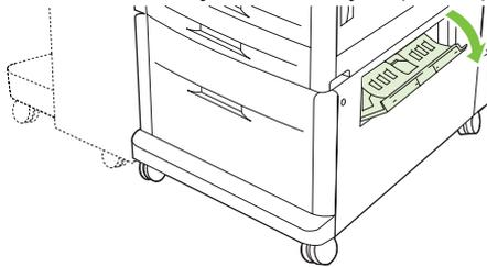
2. Check for paper in this area, and remove any paper from this area. Carefully check to be sure that you have removed all pieces of torn paper.
