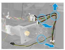
4. Remove 4 T-15 screws from both sides.
