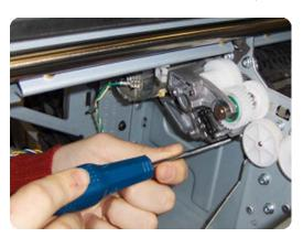
Loosen the encoder sensor adjustment screw.
