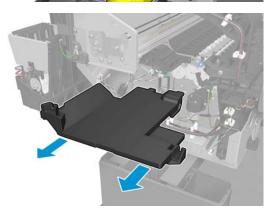
Remove the first starwheel rail. See <u>Customer Self Repair Flyers on page 353</u>.
