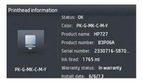
In the service plot (Go to Embedded Web Server: Support tab -> Service support -> Printer information.
