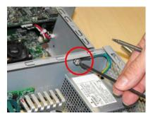
**6.** Remove the power supply unit.
