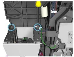
Remove the bracket and side plate.
