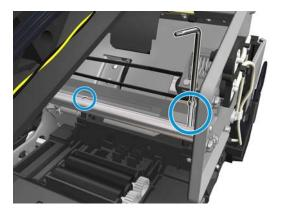
Remove the 2 T-15 screws and the left bracket.
