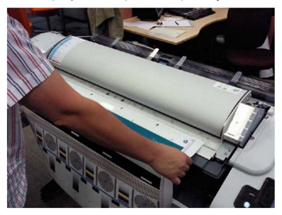
Follow the next steps to calculate the Y-Axis adjustment scale: Measure the total length of the two vertical rules at both sides of the copied plot (we call it M1 and M2).
