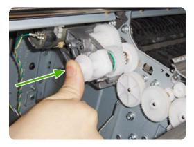
While maintaining pressure on the Media Advance Drive Adjustment Tool, fully tighten the three T-15 attachment screws in the order shown.
