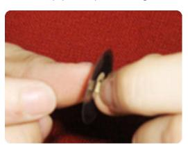
Pre-assemble the encoder on the roller without using pressure.
