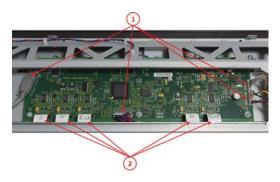
Remove the Screws (Torx 10), and remove the Scanner Controller Board.
