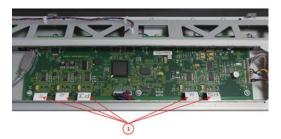
NOTE: For some of the cables it may be helpful to remove the Scanner Controller board. See Scanner Controller Unit (SUP) on page 328.
