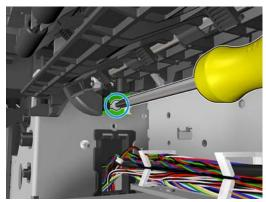
5. Remove the sensor valves.
