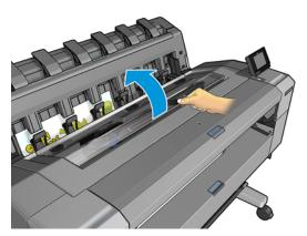
2. Move the carriage manually to the left side of the printer, if feasible.
