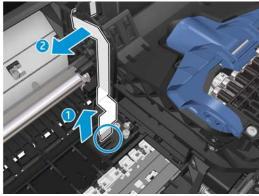
Unclip the mylar, and disconnect trailing cable.
