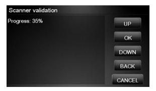
Wait until the scanner validation test has completed. The Touch Control Panel will then show the test results. Press OK to continue
