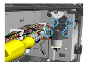
4. Remove the valves motor.
