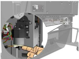
4. Disconnect the cable, and remove the T-10 screw.
