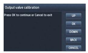
The screen will show the 'calibrating status' during some minutes, while the output valve is performing some movements.
