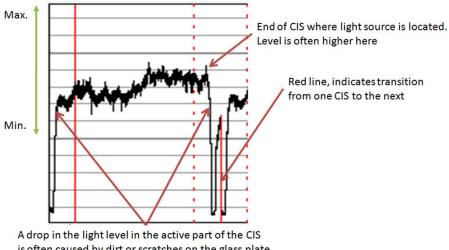
is often caused by dirt or scratches on the glass plate
