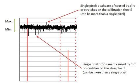
Peaks will show up in a scan as a lighter color and not necessarily in all colors, it depends on which color channels are being affected by the dirt/scratch.
