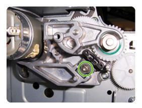
Insert the three T-15 attachment screws, but do not fully tighten them.
