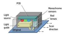
The purpose of the lens is to channel the light from the "pixels" on the image to the sensors. There is no magnification in the lens (1x1).
