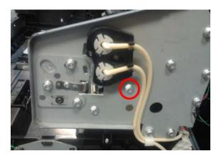
Remove the starwheel lifter cover and actuator.
