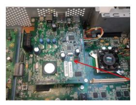
**4.** Disconnect the cables and remove the clamp.
