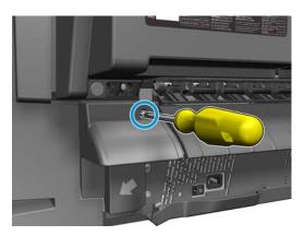
2. Remove the arch sidewall cover from the front panel side.
