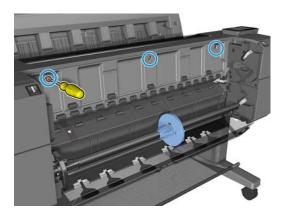
4. Remove the wheels, and then the 3 T-15 screws underneath.
