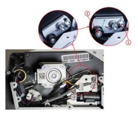
**7.** Remove the motor screws.
