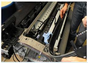
After installing the carriage, when closing the latch, make sure the carriage is placed in the printhead replacement position so the carriage doesn't interfere with the rear guide.
