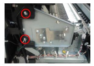
Remove the Scan Axis Motor. See Scan Axis Motor on page 244.
