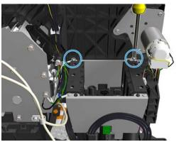
4. Remove the bracket and side plate.
