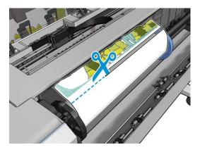
8. Remove the paper left in the printer.
