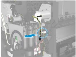
5. Remove 3 T-15 screws and the rewinder.
