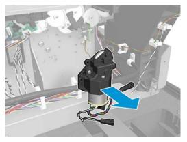
4. Disconnect the cable, remove the screw and the OPTO PCA.
