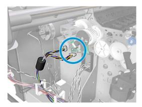
**5.** Remove the 2 screws and remove the connectors.
