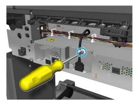
5. Disconnect and unclip the front panel cable.
