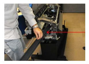
**11.** Remove 5 screws and the printheads.
