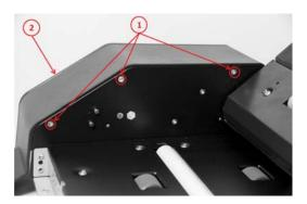
Remove the screws (1), and then the motor cover (2).
