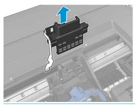
NOTE: After installing the carriage, when closing the latch, make sure the carriage is placed in the printhead replacement position so the carriage doesn't interfere with the rear guide.
