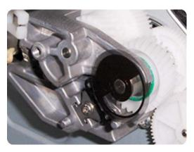
Press the encoder using the Media Advance Drive Adjustment Tool (reversed) so that it sticks to the
