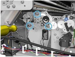
**7.** Remove the paper axis motor.
