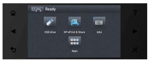
The front panel has a large central area to display dynamic information and icons. On the left and right sides you can see up to six fixed icons at different times. Normally they are not all displayed at the same time.
