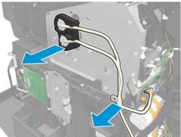
NOTE: On the first primer tubes holder make sure the holes are aligned with the holes of the carriage.
