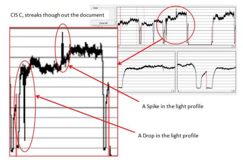
A light profile with an about 20 pixel drop can be a contaminated lens in the CIS module.
