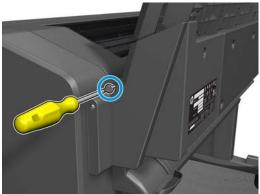
2. Remove the fixed tray cover from the front panel side.
