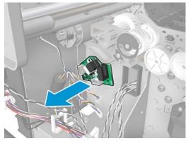
Disconnect the cable, and remove the 3 screws. 6.
