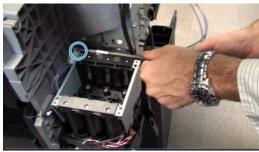
Remove the service station. See <u>Service Station with Drop Detector on page 248</u>.
