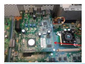
NOTE: When replacing the Jester PCA, also replace the small inter-connector provided with the kit.
