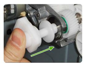
While maintaining pressure on the Media Advance Drive Adjustment Tool, fully tighten the three T-15 6. attachment screws in the order shown.
