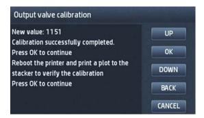
By pressing **OK** in the next screen, the printer will shut down automatically.
