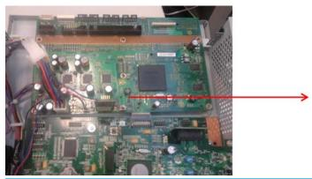
**WARNING!** If the engine PCA is not removed before the formatter, the bridge connections may be damaged.
