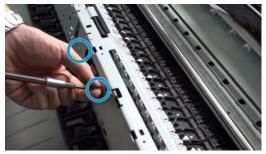
Remove the ISSWALL (removing 2 T-10 screws).
