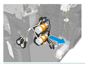
NOTE: The primer service kit includes the valves, the plastic, and the tubes.
