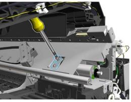
**10.** Slide out the auto pinch lifter, and disconnect the sensor.
