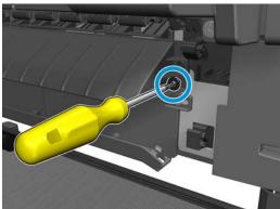
3. Remove the output platen.
