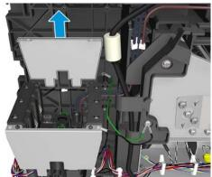
Remove 2 screws and the side plate. **5.**
