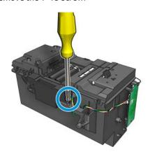
4. Remove the Drop Detector from the service station.
