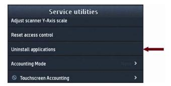
A message similar to the following will be displayed in the Front Panel. Press the OK button to remove the installed applications, or press Back or Cancel to exit.
