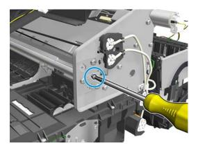
Press the bracket to release the encoder strip tension.
