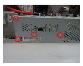
3. Disconnect the cable and remove the T-8 screw.
