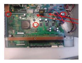
Slide out and remove the engine PCA (which is connected to the formatter PCA).
