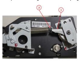
4. Remove the screw and carefully free the CIS bridge.
