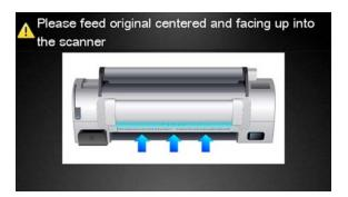
The Control Panel prompts you to feed the original. Load the Scanner IQ plot that you printed previously in the Scanner input tray. Wait then for the product to scan and print the image.
