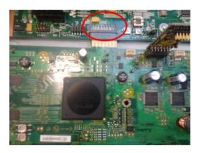
The red PCA must be installed in the new engine PCA.
