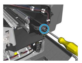
3. Remove the bump cutter actuator.
