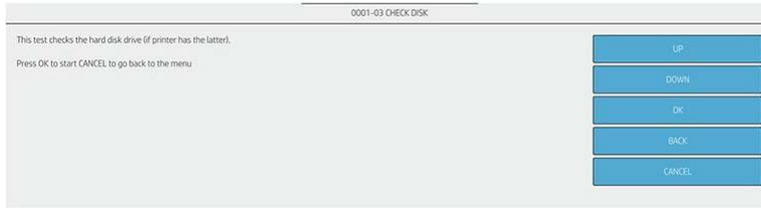
3. The screen below shows a message which explain that the printer is going to perform several checks in the hard disk. Only if it detects any fail, a System Error will prompt. Tapping the **OK** button will shut down the printer and reboot it. If you do not want to turn off, press **CANCEL**.
