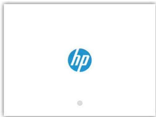
2. Tap at least three times to enable the boot mode selection. A new beep is emitted if the selection is enabled (the time for this activation depends on the boot of the operating system).
