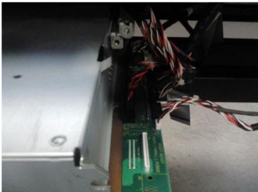
6. Remove the E-Box from the printer.
