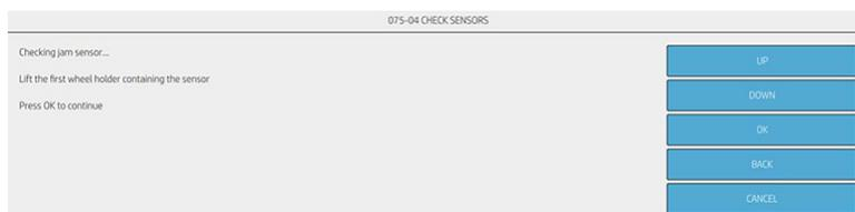
4. The screen below asks for lower the first wheel holder which activate the **jam sensor** to check if it works correctly. Lower the wheel and press **OK** in order to continue.
