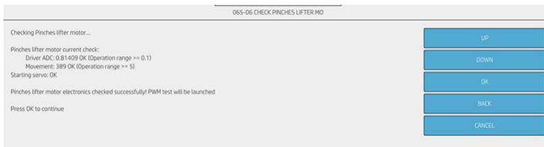
4. Screen below shows the initial preparation to perform the PWM test. Press **OK** button to start it.
