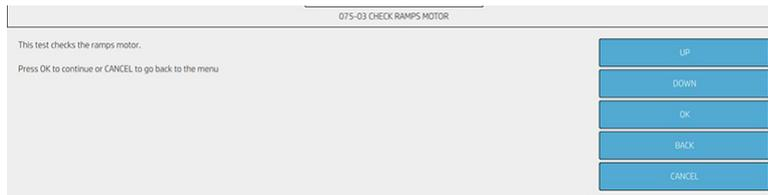
3. The screen below shows the diagnostic result of ramps motor. These are the results of motor current check, the setup of different positions (home, low and high). Also, diagnostic compares the distance path with the NVM manufacturing value. Press **OK** in order to continue with the service diagnostic.
