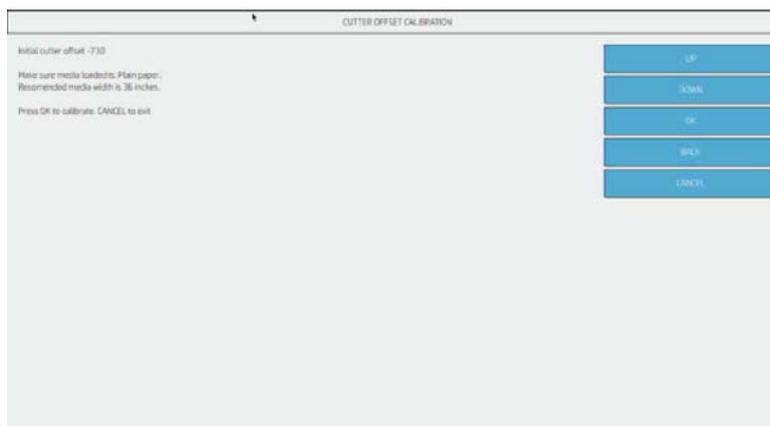
3. The front edge position along all the scan-axis will be measured (19 measures performed).
