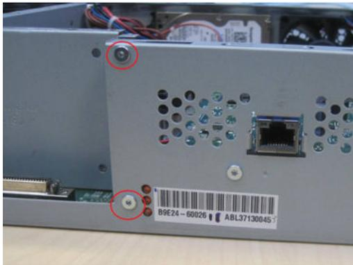
4. Disconnect the cables and remove the clamp.
