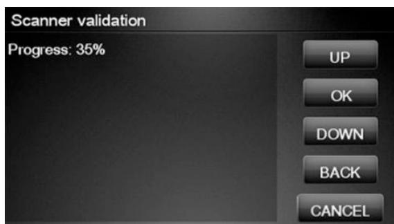
7. Wait until the scanner validation test has completed. The Front Panel will then show the test results. Press **OK** to continue
