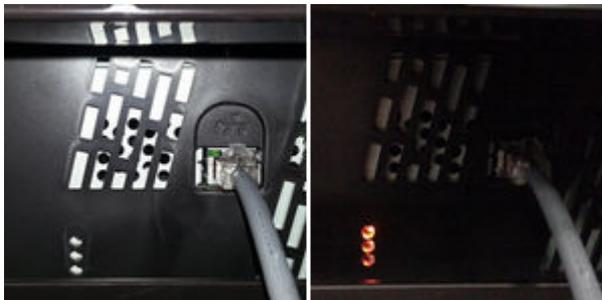
3. Use the information in the next section to interpret the LEDs and find the source of the problem. Remember that you should read these LEDs when you press the power button. Some combinations may require the replacement of more than one component. In this case, always replace one component at a time. Check the LEDs again to see whether the problem has disappeared. If the same LED sequence appears, replace the next component indicated in the table.
