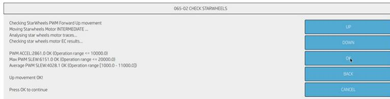
7. The screen below shows the diagnostic which performs a PWM backward check at star wheels motor in low position. The diagnostic picks up the traces and show the results. Press **OK** in order to continue with the service diagnostic.
