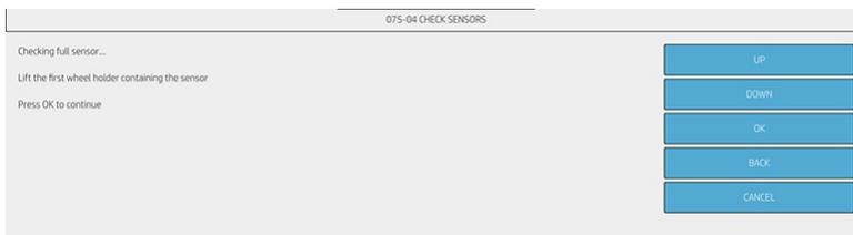
6. The screen below asks for lower the first wheel holder which activate the **full sensor** to check if it works correctly. Lower the wheel and press **OK** in order to continue.
