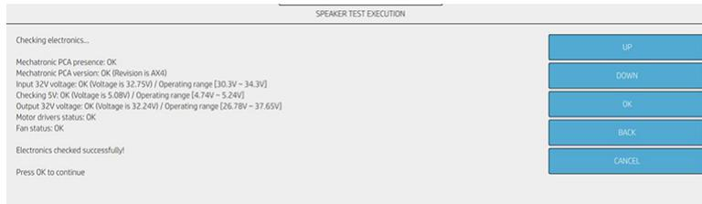
3. The screen below shows the status of the Engine PCA (Mechatronic PCA), for more info check [00102 Check Mainboard electronics on page 288](#).
