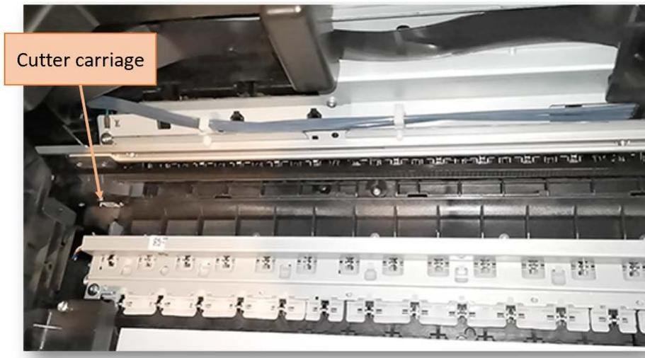
The auto cutter allows cutting all the supported media in both directions of movement with a self-orientated rotary blade. This cutter is completely independent from the printer carriage. Therefore, the printing process and the cutting process can be parallel, optimizing this way the printer's throughput.
