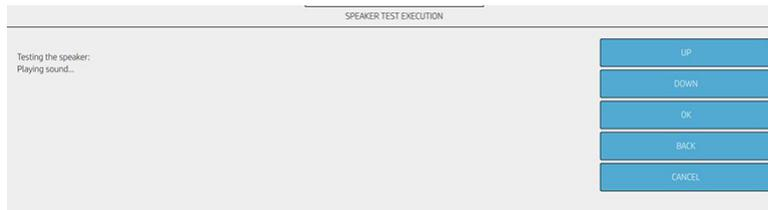
4. The diagnostic performs the test of the speaker by playing a sound.
