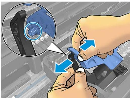
6. Remove the latch pin on the right side.
