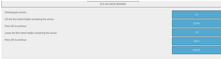
5. The screen below asks for lifting the first wheel holder which activate the **full sensor** to check if it works correctly. See the image attached below to know where is located the component. Lift the wheel and press **OK** in order to continue.
