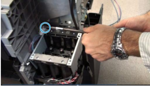
7. Remove the service station. See [Service Station with Drop Detector on page 532](#).
