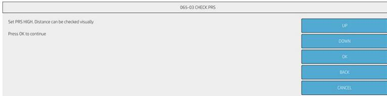
5. The diagnostic set the PRS at its maximum height to check the distance visually. Press **OK** button to continue when it will be checked.
