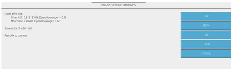
4. The diagnostic asks for opening the window cover in order to visually check the carriage movement through the scan axis. Then, tap the **OK** button in order to continue the checking process.
