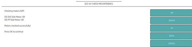
11. The diagnostic checks the optotrip sensors when the ISS motor is up. Then press **OK** button to continue.
