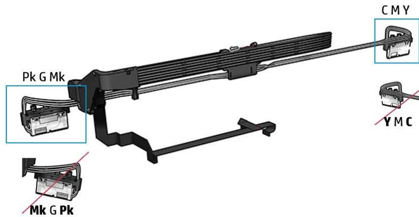
2. Power on the printer and enter the Service utilities menu (see [Entering the Service utilities menu on page 343](#)). In this menu, reset the Tubes and Trailing cable usage counter (see [Reset Life Counters on page 354](#)). Then, run the Purge Tubes utility, and follow the steps prompted by the printer (see [Purge tubes on page 354](#)).
