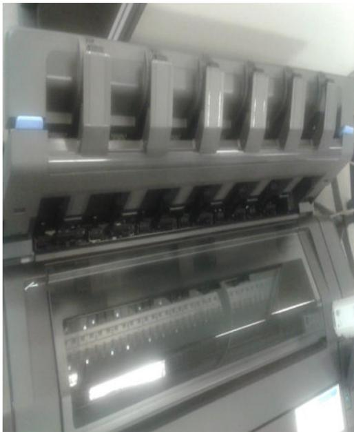
After printing with thin media, remember to return the blue lever so that the gap between the arms and the stacker tray is small again.
