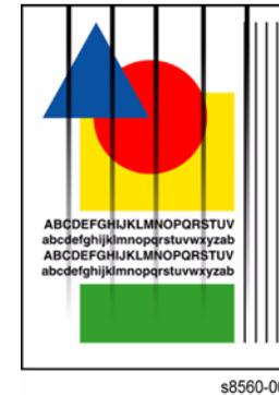
**Figure 1 Example of Streaks and Lines on Output**
