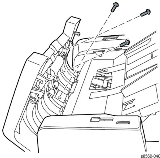
Figure 1 DADF Front Cover Fasteners
