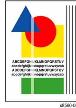
**Figure 1 Example of Scratches on Output**
