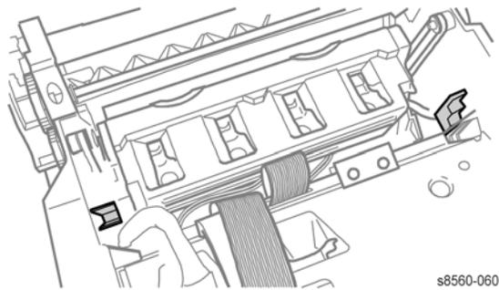
**Figure 9 Printhead Cradle Notch Location**
