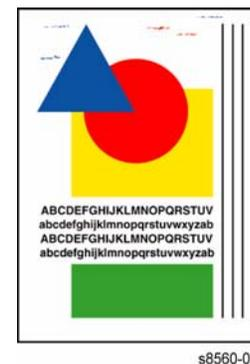
**Figure 1 Example of Latent Image on Output**
