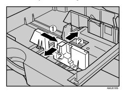
4. Pinch the clips on the end guide ( ), and match the guide to the paper size ( ).
