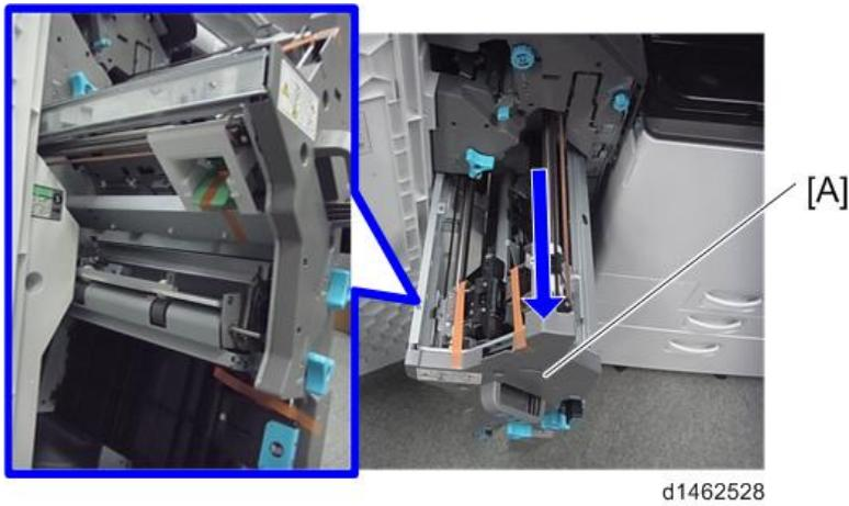
5. Remove the accessories in the package (fixing screws, etc.).
