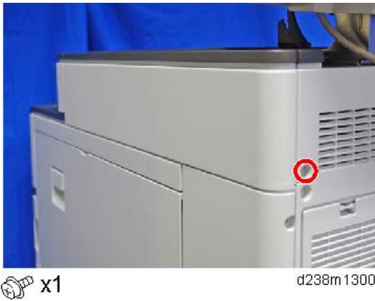
12. Remove the scanner right cover [A].
