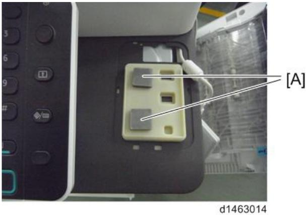
10. Connect the cable [B] to the IC reader [A] and attach the reader to the table.
