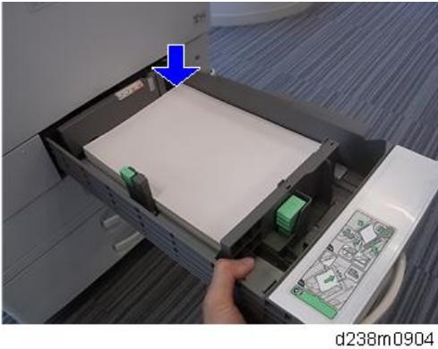
4. Reattach the tray. Lift the tray slightly when you attach it.
