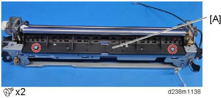
5. Fusing exit driven roller [A]
