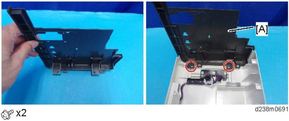
5. Remove the scanner front cover [A].
