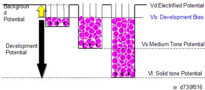
In addition to the development gamma and the potential, the toner density in the developer needs to be controlled. This is done to maintain the proper toner density (the amount of toner adhesion).
