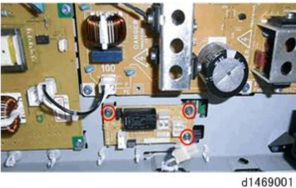
4. Connect the two harnesses between "PCB: DHB" and "PSU".
