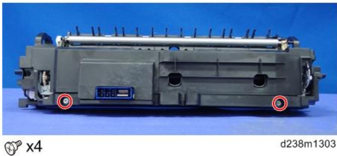
3. Lift the fusing unit to remove the fusing lower cover [A]
