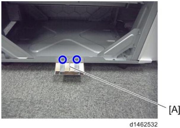
11. Attach the joint bracket [A] to the machine (🔩×4 : 4×12).
