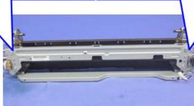
8. Release the boss caps on both sides, and then detach the heating sleeve unit [A].
