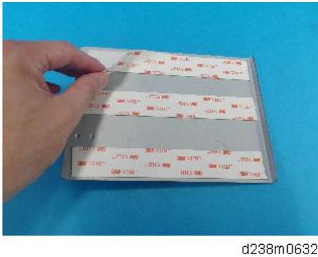
6. Stick the lock plate [B] with its center aligned with the indentation [A] on the right door.
