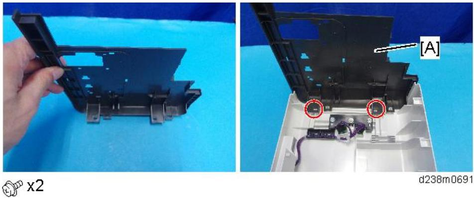
5. Remove the scanner right cover [A].
