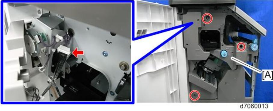
5. Remove the punch guide plate [A].
