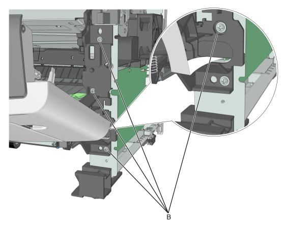
**6** Remove the right front mount, and then remove front door. Below are the front door and the right front mount.
