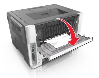
3 Firmly grasp the jammed paper on each side, and then gently pull it out.Note: Make sure all paper fragments are removed.
