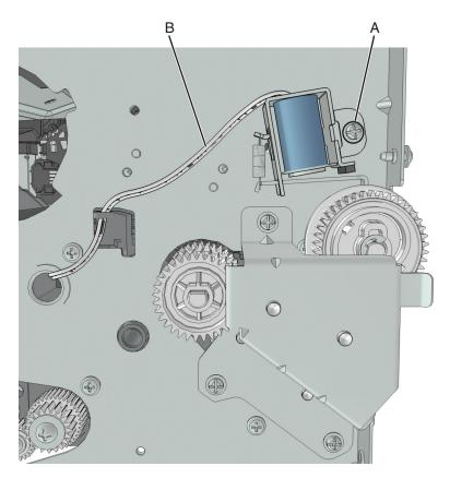
**11** Remove the other half of the cable from the printer.
