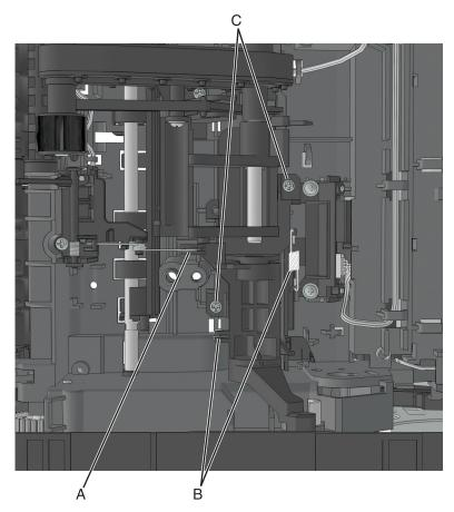
Below are the cam release and bracket.
