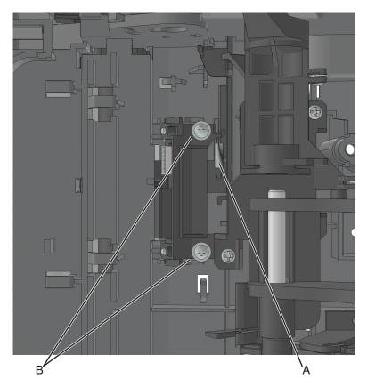
**9** Disconnect the cable from the sensor.
