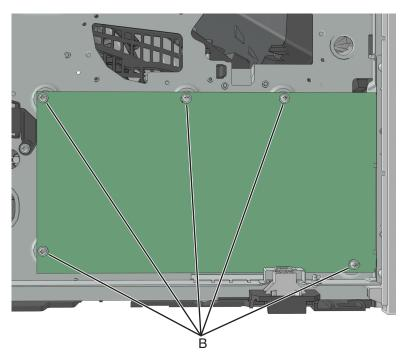
**Installation note:** After installing a new controller board, perform the printer configuration restoration. See **"Restoring the printer configuration after replacing the controller board" on page 205**.
