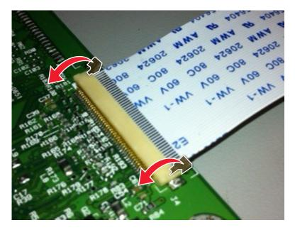
**2** Slide the cable out of the connector.
