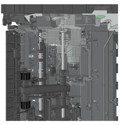
**c** Secure the cable at the pick/lift motor gearbox using cable ties. Cut off any excess cable tie.
