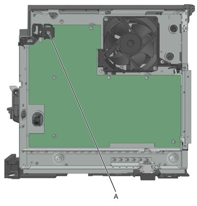
6 Disconnect the cables JUICC1 and J24 from the controller board.
