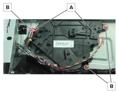
• For the Polygon LSU, disconnect the cable (A), remove the three screws (B), and then disconnect the cable JVIDEO or JLSU1 from the controller board.
