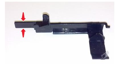
**b** Apply RheoGel 793 to the point of contact between the bracket (A) and cam.
