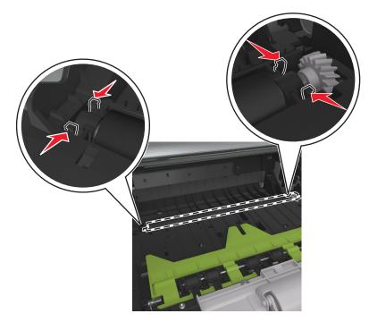
**2** Lift to remove the transfer roll.
