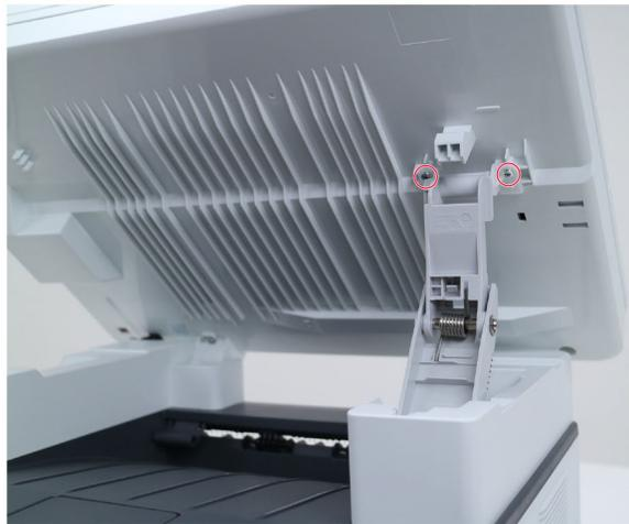
8 Remove the control panel.
