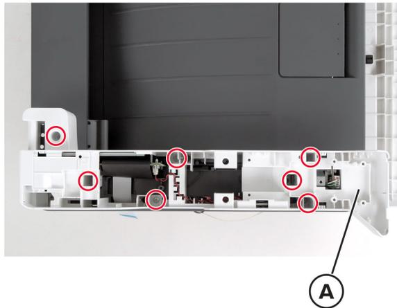
**13** Remove the screws, and then remove the USB cable (B) from the guides.
