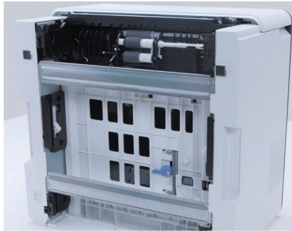
3 Remove the left and right pick roller retainers.
