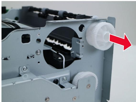
**Installation note:** Before installing the gear, make sure that it is properly greased.
