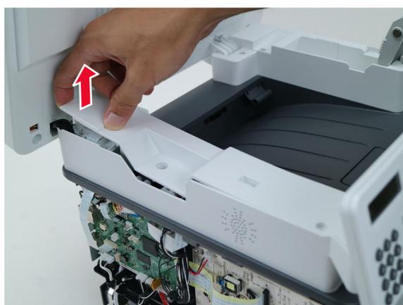
**7** Disconnect the FFC cable, and then remove it from the frame.
