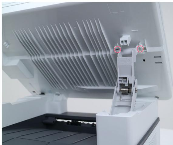
**8** Remove the control panel.
