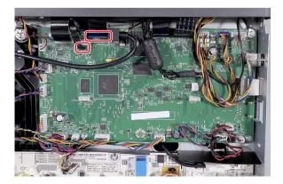
**5** Remove the three screws (A), remove the two cables (B) from the toroid (C), and then remove the printhead.
