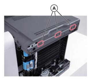
**4** Release the latch at the front, and then remove the cover.
