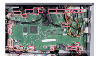
**3** Remove the five screws, and then remove the controller board.
