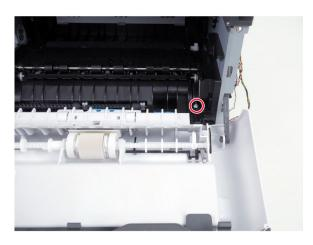
**3** Release the latches securing the sensor, and then disconnect the sensor cable.
