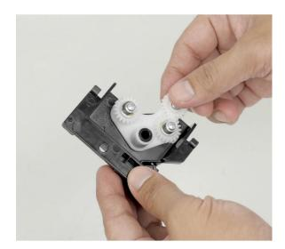
**b** Align the tab on the housing to the notch in the frame, and then install the duplex swing arm assembly.
