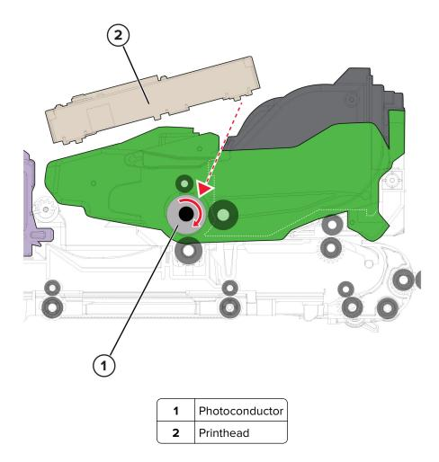
The printhead emits a laser that exposes the surface of the photoconductor. The laser pulses coincide with the digital latent image. The exposed areas of the photoconductor surface are discharged, resulting in a photoconductor surface potential that is less negative than the non-exposed areas.
