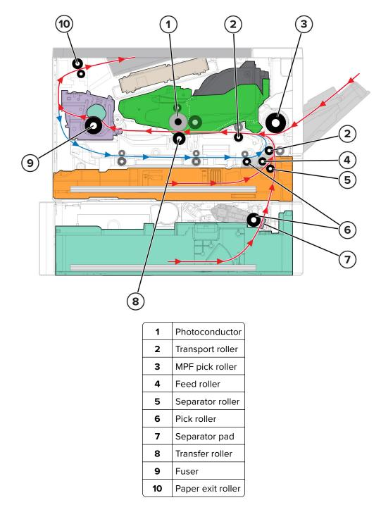
The pick roller picks and the feed roller feeds the paper to the separator roller or separator pad. The feed roller feeds the paper to the transport roller. For MPF print jobs, the MPF pick roller picks and feeds the paper to the transport roller.
