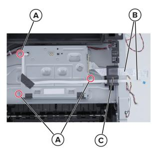
Installation note: When installing the printhead, tighten the screws in the following the order:
