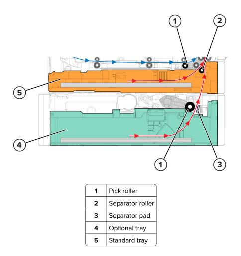
The motor (main drive) in the printer drives the standard tray. The lift plate in the tray is spring loaded and is not driven by a motor. The spring raises the lift plate until the paper is in contact with the pick roller.
