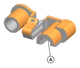
The grease may spread and contaminate other areas of the bushing. If this happens, the grease may transfer when paper is being picked from the tray.
