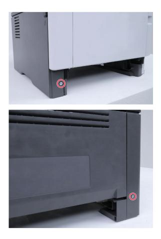
**2** Open the front door, and then release the left front door link.
