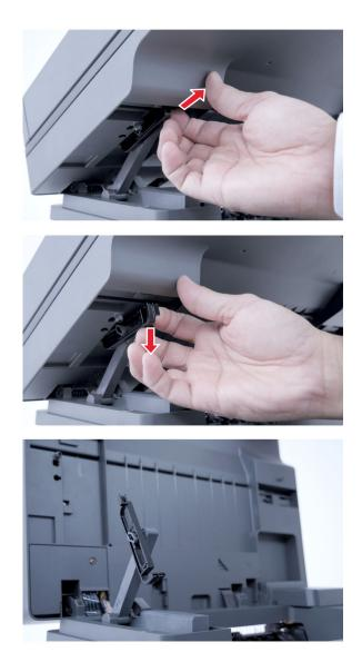
**3** Remove the two screws, and then remove the scanner pivot arm.
