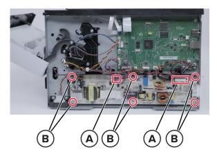
**CAUTION—SHOCK HAZARD:** To avoid the risk of electrical shock, do not remove the shield from the back of the LVPS.
