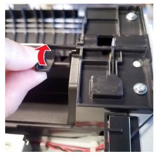
**c** Make sure that the actuator is properly installed and freely rotates without binding.
