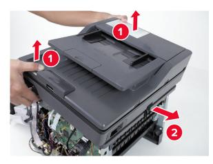
Installation note: Make sure to perform the ADF scanner calibration after replacing the ADF and scanner.
