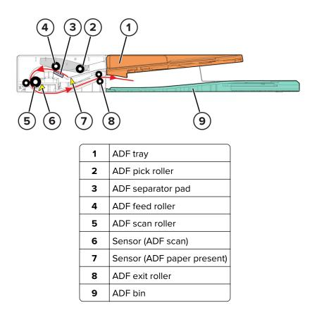
Paper from the ADF tray enters the ADF through the ADF pick roller, ADF feed roller, and ADF separator pad. On the ADF tray, the sensor (ADF paper present) detects if paper is loaded.
