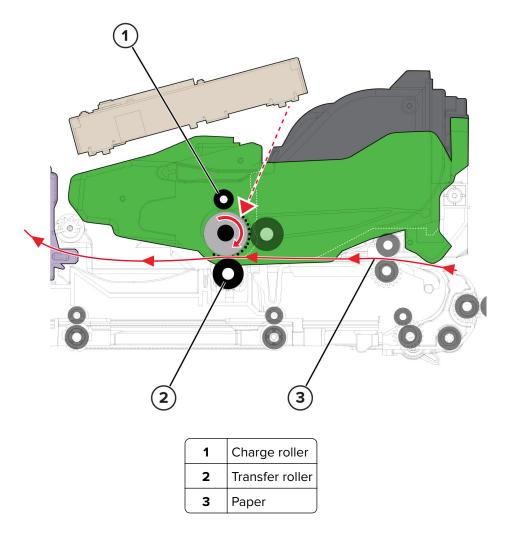
A positive potential relative to the toned image formed on the photoconductor is applied to the transfer roller. This allows the transfer roller to move the developed toner from the surface of the photoconductor to the paper as the paper is passed between the transfer roller and photoconductor.
