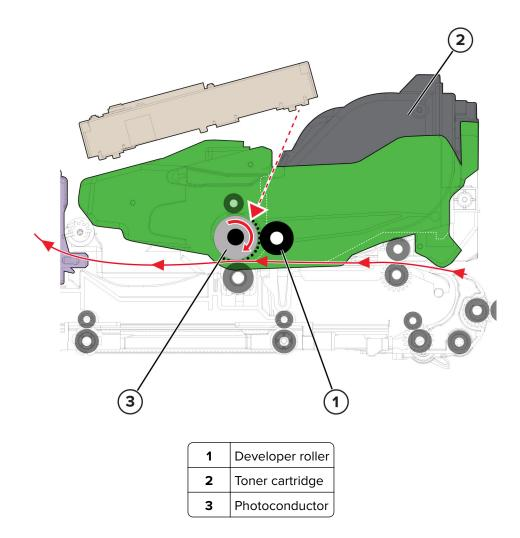
The developer roller applies the toner from the toner cartridge to the photoconductor during the development process. The difference in surface potential creates an electric field that causes the toner particles to move to the photoconductor according to the pattern of the latent image.
