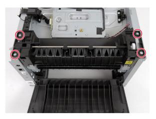
**5** Lift the redrive, and then disconnect the cable from the redrive.
