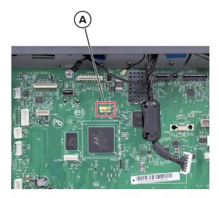
4 Move the jumper to cover the middle and exposed prongs.
