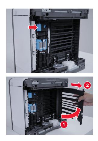
**Installation note:** Make sure that the duplex guide is properly inserted into the locating features inside the printer.
