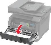
**2** Locate the printer serial number behind the front door.
