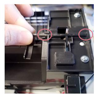
**b** Carefully rotate the actuator upward until it is engaged to the printer frame.
