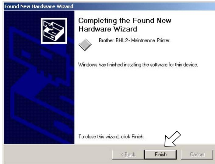
**NOTE:** After completion of the driver installation, if you press the **9** key on the FAX machine twice to exit the maintenance mode, the "Found New Hardware Wizard" screen in step (6) appears again. Click **Cancel**.
