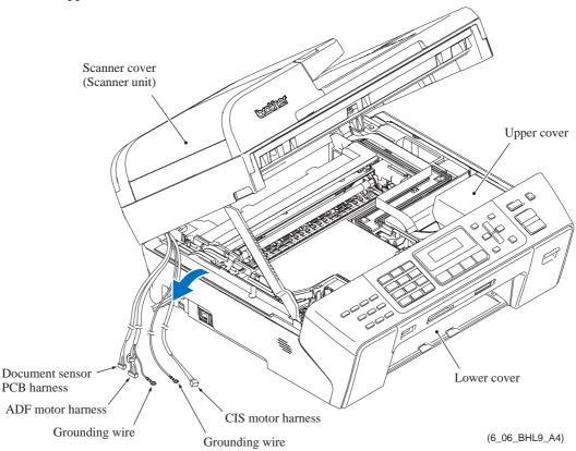
**Assembling Note:** Route the document sensor PCB harnesses, ADF motor harness, CIS motor harness, and grounding wires as shown below.
