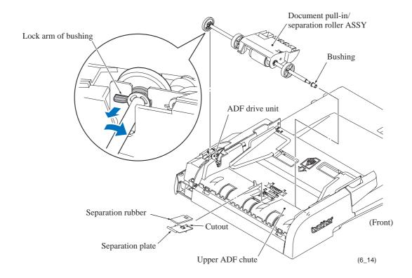
**Assembling Note:** When putting the separation plate and its rubber back into place, fully insert the plate until the cutout becomes fitted over the boss on the upper ADF chute.
