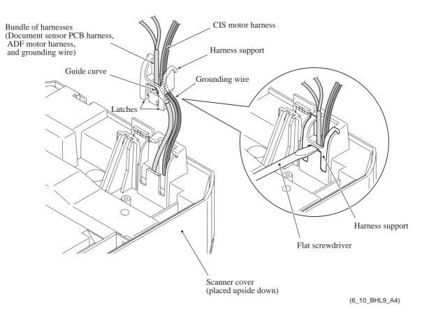
**Assembling Note:** Before fitting the harness support (shown above) into the scanner cover, route the document sensor PCB harnesses and the bundle of ADF motor harness and its grounding wire through the guide curve provided in the harness support. The CIS motor harness and the grounding wire should be placed at the rightmost position (viewed from the bottom) in the square opening in the scanner cover.
