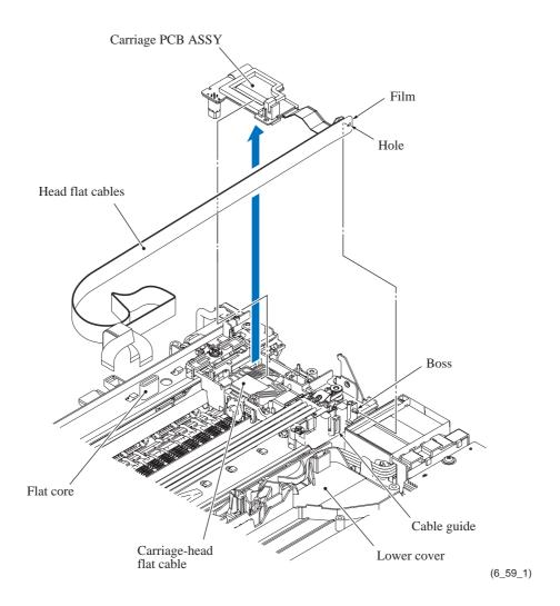
**Assembling Note:** When mounting the carriage PCB ASSY, route the head flat cables, observing instructions given on the next page.
