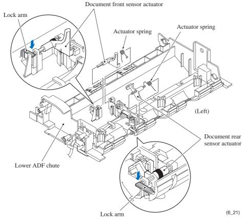
(22) Press the lock arm and pull the left edge of the document sensor PCB to the front and upwards to remove the PCB. Then disconnect the document sensor PCB harness from the PCB.
