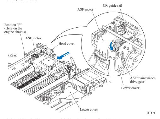
(7) Unlatch the head cover from the head/carriage unit and pull it up.
