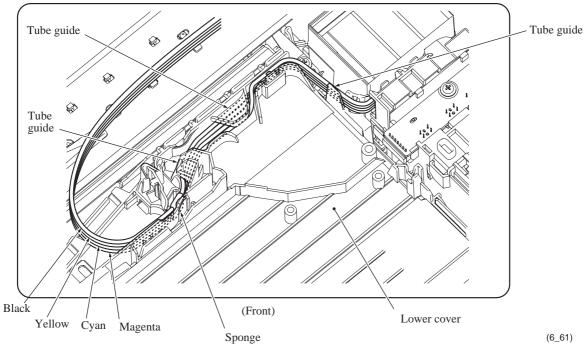
**Assembling Note:** After mounting the ink refill ASSY, route the ink supply tubes on the lower cover, aligning the four colors in the order as shown above.
