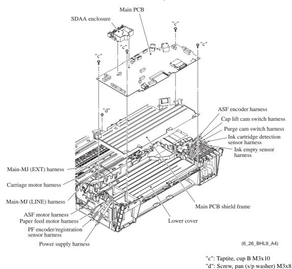
Assembling Note: If you replace the main PCB, you need to load programs onto the flash ROM, restore the machine information that has been backed up in an external memory (refer to Chapter 9, Section 9.4.10), and make specified adjustments of various settings (refer to Chapter 7, Section 7.3). Make sure beforehand that the head/carriage unit is mounted.
