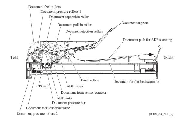
The scanner mechanism offers two types of scanning: ADF scanning and flat-bed scanning. It automatically switches to the former at the start of a scan operation if the document front sensor inside the ADF detects a document.
