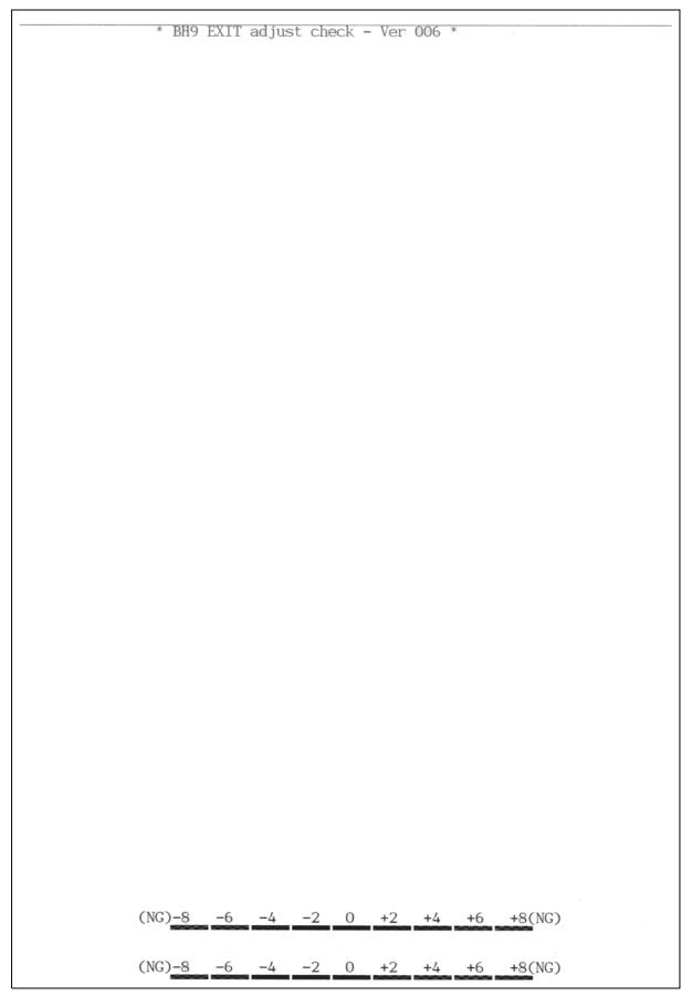
Paper Feeding Check Pattern for the Paper Ejection Roller
