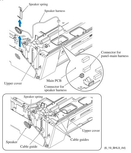
**Assembling Note:** After mounting the speaker and its spring into the pocket provided on the upper cover, route the speaker harness through the cable guides on the upper cover as shown below.
