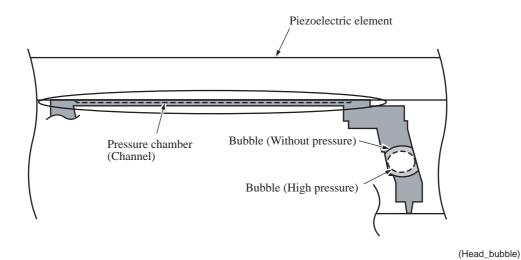
The above illustration shows an example of an extremely large air bubble reaching the head nozzle from the channel ink flow path; the dotted line, the changes resulting from applying a voltage to the laminated electrode, expanding the piezoelectric ceramic actuator. Note how contraction of the air bubble absorbs the pressure from the piezoelectric ceramic actuator, preventing ink ejection.
