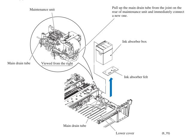
**Assembling Note:** If you replace the ink absorber box (without replacing the main PCB), you also need to replace the flushing box (see Section 6.1.13) and reset both the purge and flushing counters as specified in Chapter 7, Section 7.5.
