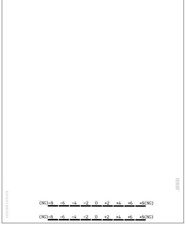
Paper Feeding Check Pattern for the Paper Ejection Roller
