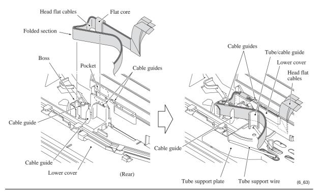
• After making sure that the ink supply tubes are routed between the tube/cable guide and the lower cover, pass the ink supply tubes through the bent section of the tube support wire as shown below.
