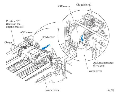
(7) Unlatch the head cover from the head/carriage unit and pull it up.
