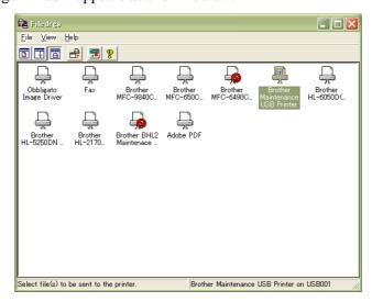
(2) Drag and drop the "chart.prn" onto the Brother Maintenance USB Printer driver icon in the Filedrgs window shown above.
