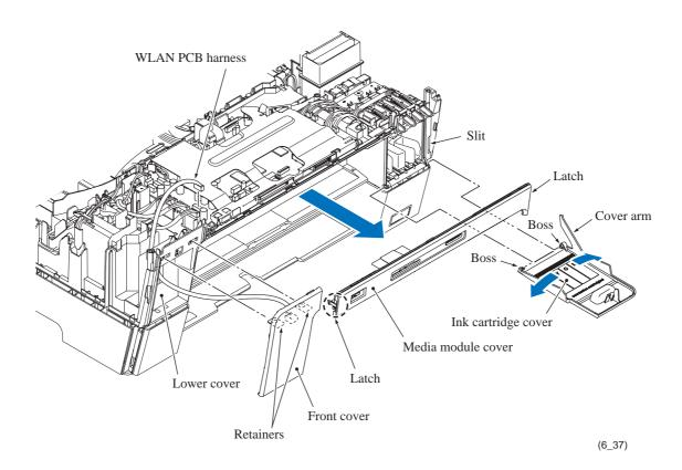
(5) Release the two latches on the front cover and take out the WLAN PCB.
