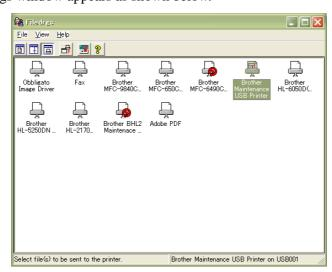
(2) Drag and drop the "qualbh9.prn" onto the Brother Maintenance USB Printer driver icon in the Filedrgs window shown above.
