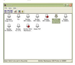
(2) Drag and drop the firmware (e.g., lz0023\_a.pmu) onto the Brother Maintenance USB Printer driver icon in the Filedrgs window shown above.
