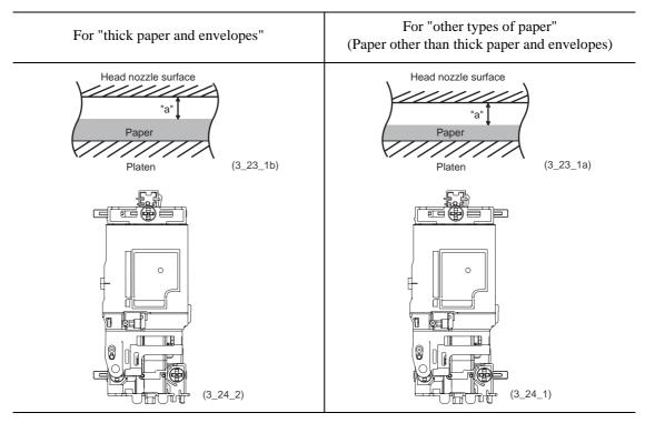
As listed below, the printer driver on the connected PC or the paper type setting on the machine controls the slider cams to determine the height of the head/carriage unit.
