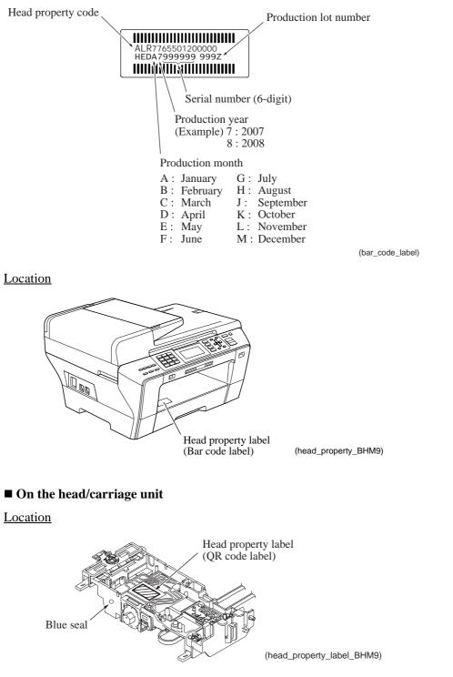
**Note:** Depending on whether the head/carriage unit has a round, blue seal on its left side, the purge type to be performed differs. Refer to Chapter 7, Section 7.2 [2].
