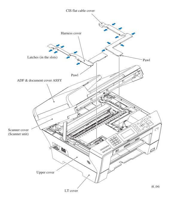
(3) Disconnect the CIS flat cable from the main PCB, pull it to the rear through the two flat cores, and then release it from the cable guides. Unlatch the flat cores and take them out of the upper cover.
