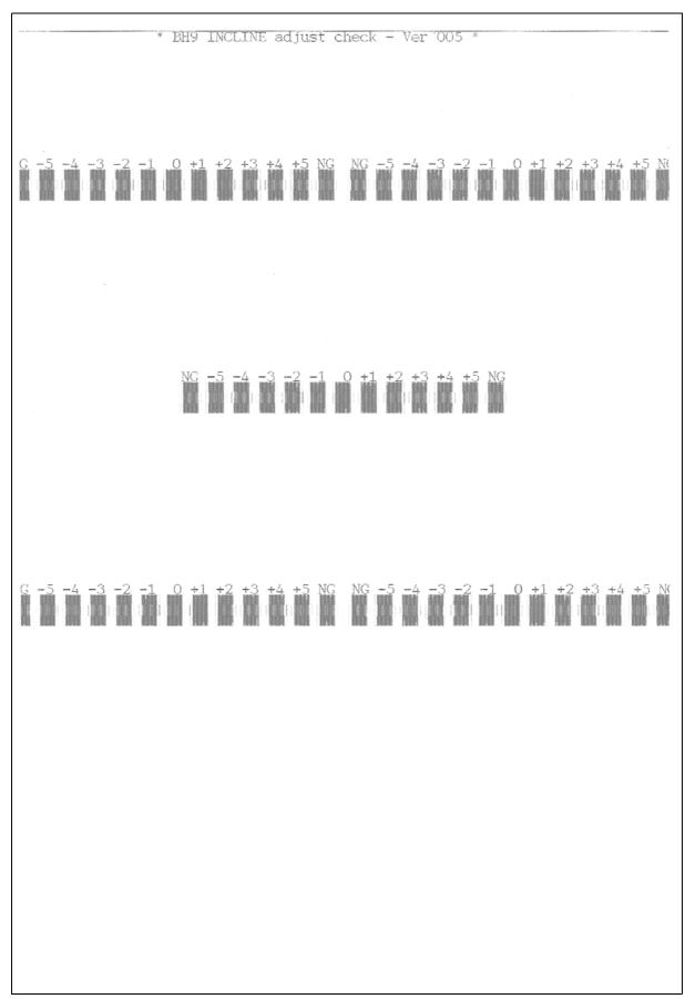
**Head Positioning Test Pattern**
