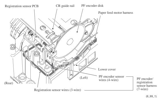
**<u>Routing L: ASF motor/encoder harness on the lower cover</u>**
