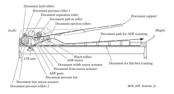
The scanner mechanism offers two types of scanning: ADF scanning and flat-bed scanning. It automatically switches to the former at the start of a scan operation if the document front sensor inside the ADF detects a document.
