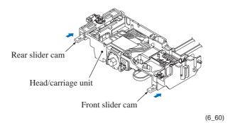
• When mounting the head/carriage unit on the left end of the engine unit, first fit the front end over the CR support chassis (shown on page 6-65) and then set the rear end onto the CR guide rail. Make sure that the two front bosses (see below) provided on the bottom of the head/ carriage unit catch the front edge of the CR support chassis and the two rear bosses are fitted in the two cutouts (on page 6-65) in the CR guide rail.
