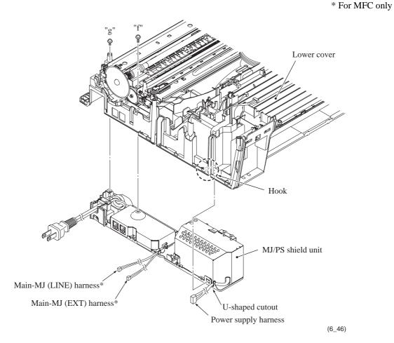
"f": Screw, pan (s/p washer) M3x8 "g": Taptite, cup S M3x6 (4) Unlatch the power cord bush and pull it up from the AC cord holder. Then release the power cord from the cable guides provided on the AC cord holder (shown on page 6-56).
