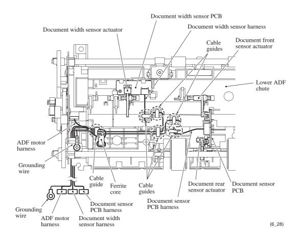
• After mounting the lower ADF chute on the document cover, be sure to route a bundle of harnesses (document width sensor harness, document sensor PCB harness, and ADF motor harness and its grounding wire) on the underside of the document cover and secure the bundle with a cable tie as shown below.
