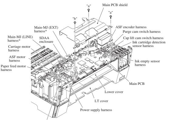
(2) Remove the three screws (two "a" and one "b" screws) from the main PCB shield and lift it up.
