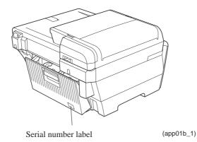
(7) In the **Head Info.** box, type the 16-digit property code (e.g., ALR7765501200000) which is printed on the bar code label attached to the lower cover. Click the **OK** button.
