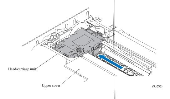
(7) Insert the tip of a flat screwdriver into the square hole provided in the head cover to release the latch in the direction of the arrow, then release other three latches and lift up the head cover.
