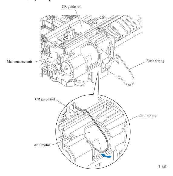
**Assembling Note:** When mounting the earth spring, take care not to contaminate it with grease.
