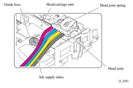
**Note:** Make sure that all of the four ink supply tubes are routed in front of the guide boss as shown above.
