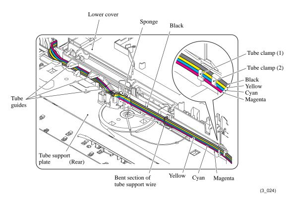
**Note:** Bind ink supply tubes with two tube clamps. As shown above, align four ink supply tubes in the order of Magenta, Cyan, Yellow, and Black from bottom to up. Set tube clamp (1) on magenta, cyan, and yellow ink tubes from the bottom, and tube clamp (2) on black, yellow, and cyan ink tubes from the top.
