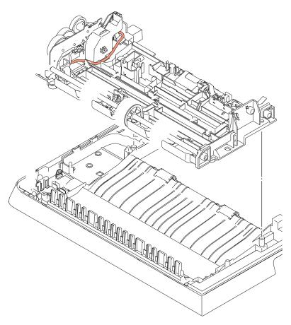
(27) At the rear end of the document feed roller ASSY, pull the lock arm of the bushing inwards to release the boss and turn it to the position shown below.
