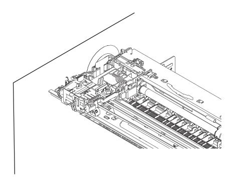
**Assembling Note:** Make sure that all of the four ink supply tubes are routed in front of the guide boss as shown above.
