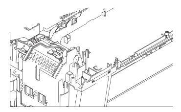
**Assembling Note:** After mounting the speaker and its spring into the pocket provided on the upper cover, route the speaker harness through the cable guides on the upper cover as shown above.
