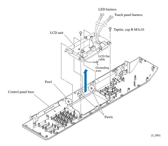
(7) Remove the LCD from the LCD lower cover.
