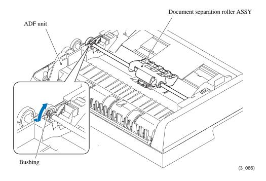
(14) Release the rear end of the document separation roller ASSY and take the ASSY out of the ADF unit.
