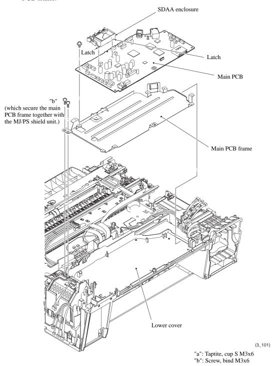
**Assembling Note:** If you replace the main PCB, you need to load programs onto the flash ROM, restore the machine information and head calibration data that have been backed up in an external memory, and make specified adjustments of various settings (refer to Chapter 4, Section 2 "IF YOU REPLACE THE MAIN PCB"). Before starting, make sure that the head/carriage unit is mounted.
