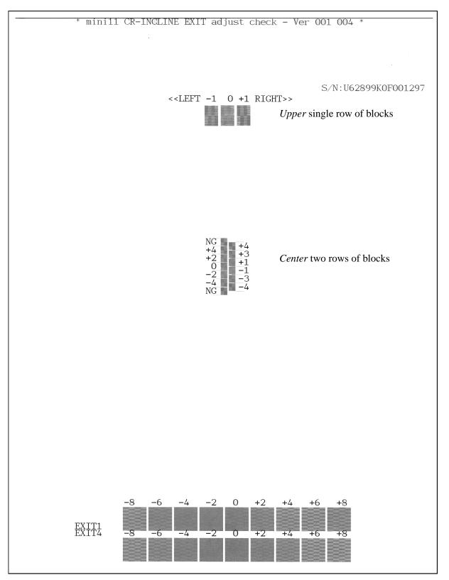
**Head Inclination Test Pattern**
