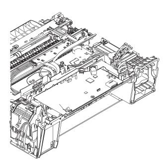
**Assembling Note:** Before securing the main PCB shield, route the harnesses on the top of the lower cover as shown below. Make sure that the MJ (EXT) harness and MJ (LINE) harness are routed through the SDAA enclosure. Gather the slack of the MJ (LINE) harness around section "X" shown below. (See the illustration given on page 3-84 for the routing of those harnesses on the left side of the lower cover.)
