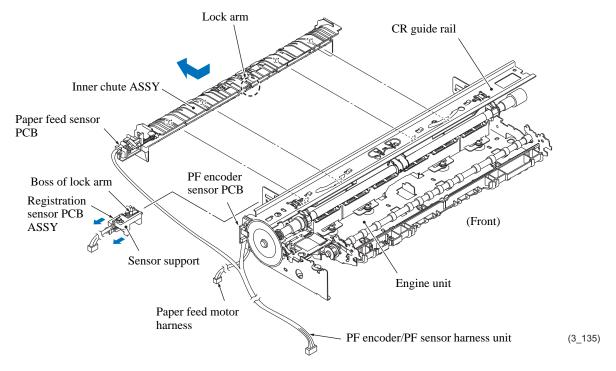
(20) Release the registration sensor PCB ASSY from the support arm and take it up and out of the sensor support.
