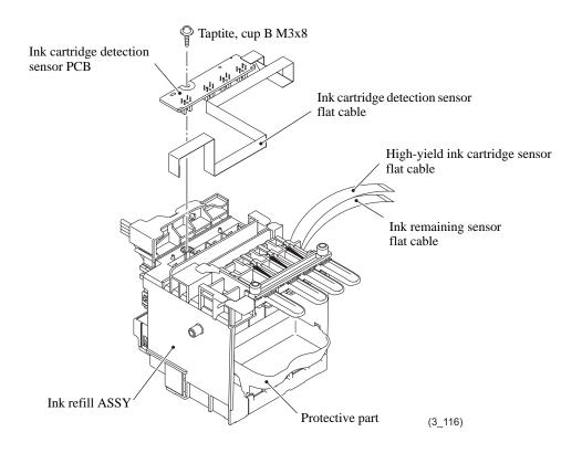
**Assembling Note:** When replacing the ink cartridge detection sensor PCB ASSY, fold its flat cable as specified below.
