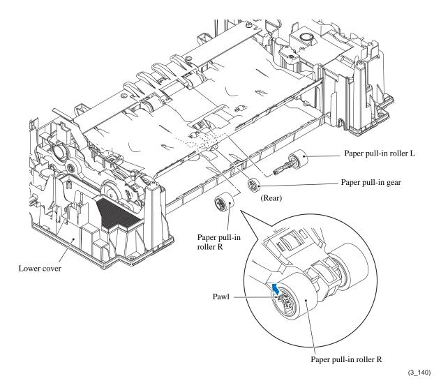
**Assembling Note:** Before mounting the paper pull-in roller L, apply the specified lubricant to the specified points on its shaft, referring to Section 5.
