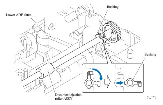
(24) At the rear end of the document ejection roller ASSY, slide the bushing to the right to remove it from the chassis of the ADF drive unit and then remove the front end of the ASSY from the lower ADF chute.
