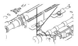
**Assembling Note:** When attaching the PF encoder disk to the PF roller gear L, using a spatular tool makes the job easier. Put on clean gloves to protect the disk surface from dust or fingerprints.
