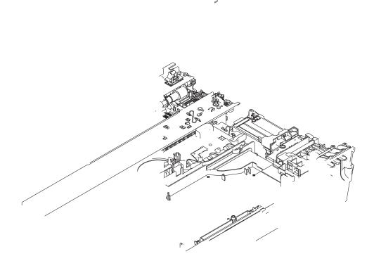
**Assembling Note:** Set the CR encoder strip so that the -marked end is to the right (carriage motor side) and the mark points upwards as shown above.
