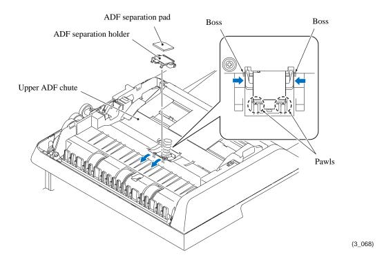
(16) Remove the ADF separation spring from the upper ADF chute.
