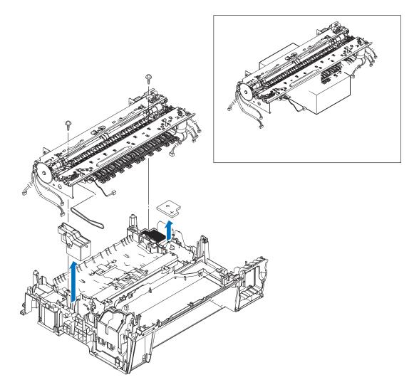
(8) Remove the ink cartridge cover switch from the front right side of the lower cover.
