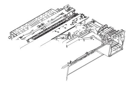
(2) To remove the parts of the T2 paper pull-in roller ASSY, first pull the pawl on the T2 paper pull-in roller R outwards and remove the roller R, then pull out the T2 paper pull-in roller L while rotating it. The T2 paper pull-in gear also comes off.
