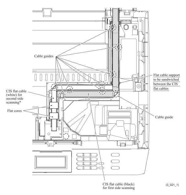
Underside of the scanner cover (scanner unit): ADF motor harness, CIS motor harness, Document detection/width & scanning position (first side) sensors harness, Document scanning position sensor harness (second side)\* and ADF cover switch harness
