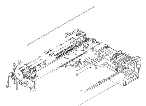
Assembling Note: Set the CR encoder strip so that the -marked end is to the right (carriage motor side) and the mark points upwards as shown above.
