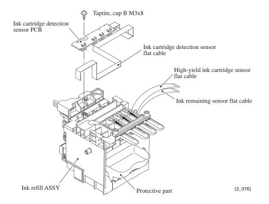
Assembling Note: When replacing the ink cartridge detection sensor PCB ASSY, bend its flat cable as specified below.
