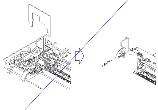
6) Slide the head/carriage unit by hand to check that it moves smoothly. If it does not move smoothly, the leveler roller (LR) ASSY is not in place. Go back to step 5).
