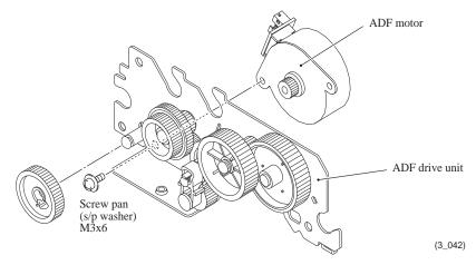
Assembling Note: When mounting the ADF motor on the ADF drive unit, connect the ADF motor harness to the motor beforehand.
