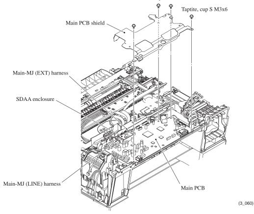
**Assembling Note:** Before securing the main PCB shield, route the harnesses on the top of the lower cover as shown below. Make sure that the main-MJ (EXT) harness and main-MJ (LINE) harness are routed through the SDAA enclosure. Gather the slack of the main-MJ (LINE) harness around section "X" shown below. (See the illustration given on page 3-101 for the routing of those harnesses on the left side of the lower cover.)
