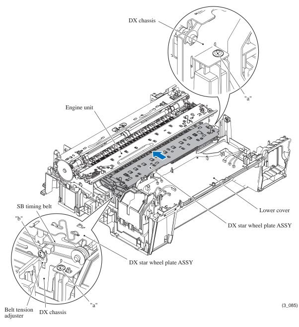
"a": Taptite, cup B M3x10 "b": Screw, pan (s/p washer) M3x5DB
