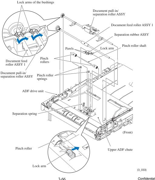
Assembling Note: When mounting the document feed roller ASSY 1, make sure that it presses down the document guides of the document pull-in/separation roller ASSY as shown below.
