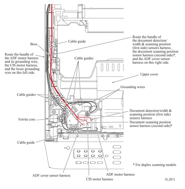
Assembling Note: Route the harnesses and grounding wires as shown below.
