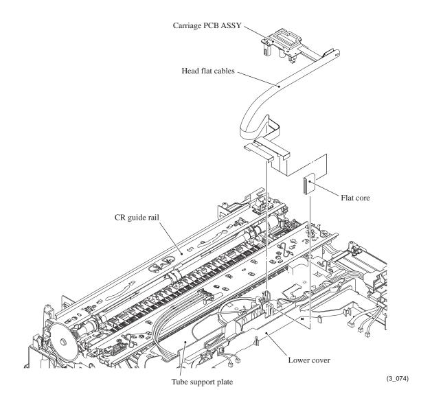
Assembling Note: When mounting the carriage PCB ASSY, route the head flat cables as shown below.
