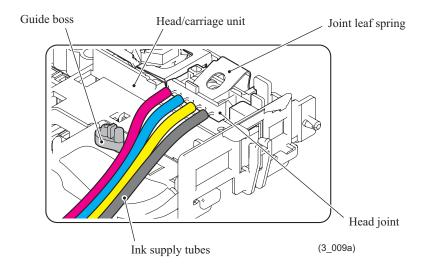
**Note:** Make sure that all of the four ink supply tubes are routed in front of the guide boss as shown above.
