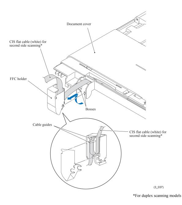
**Assembling Note:** When mounting the FFC holder, make sure that the white CIS flat cable (for second side scanning)\* is routed through the cable guides in the FFC holder as shown above.
