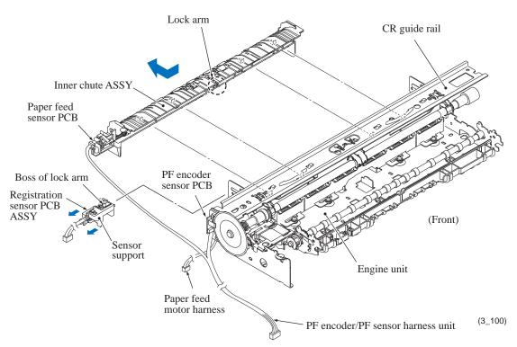
(19) Release the registration sensor PCB ASSY from the support arm and take it up and out of the sensor support.
