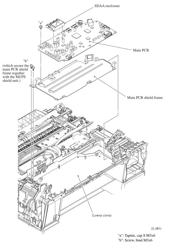
**Assembling Note:** If you replace the main PCB, you need to load programs onto the flash ROM, restore the machine information and head calibration data that have been backed up in an external memory, and make specified adjustments of various settings (refer to Chapter 4, Section 4.2). Before starting, make sure that the head/carriage unit is mounted.
