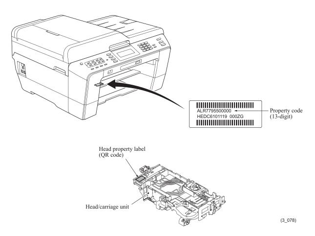
**Note:** When storing the removed head/carriage unit for a long period, put it in the head casing correctly using the following steps. Leaving it out of the casing causes the head nozzles and ink supply ports to dry up so that the head/carriage unit can no longer provide the original performance.
