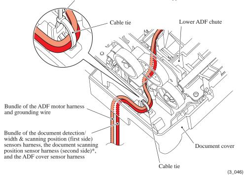
Cut off the excess of the cable tie with nippers.
