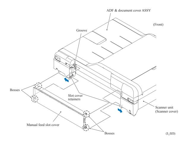
Assembling Note: Mount the manual feed slot cover, using the following steps.
