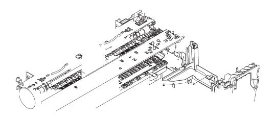
**Assembling Note:** The DX chassis is positioned with reference to the engine unit. If the engine unit is removed and mounted (Section 3.9.17), therefore, it is necessary to position the DX chassis again, using the following steps.
