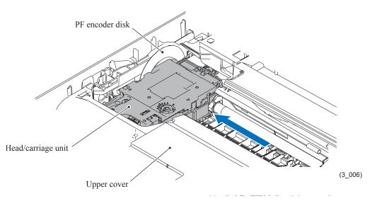
(8) Insert the tip of a flat screwdriver into the square hole provided in the head cover to release the latch in the direction of the arrow, then release other three latches and lift up the head cover.
