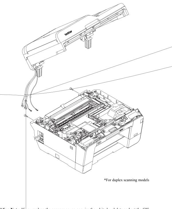
**Assembling Note:** If you replace the scanner cover, acquire the white level data and set the CIS scanner area (Function code 55), referring to Chapter 5, Section 5.1.4.15.
