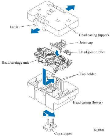
Assembling Note: Mount the head/carriage unit, using the following steps.
