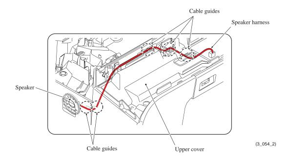
**Assembling Note:** After mounting the speaker and its spring into the pocket provided on the upper cover, route the speaker harness through the cable guides on the upper cover as shown above. (See also the figure on the previous page.)
