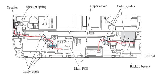
Assembling Note: When setting the backup battery, route the battery harness through the cable guides on the upper cover as shown above.
