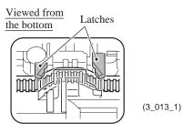
4) First fit the front end of the head/carriage unit over the CR support chassis and then set the rear end onto the CR guide rail.
