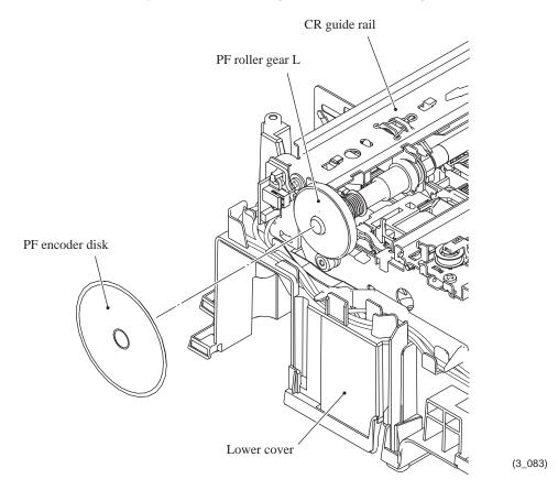
Assembling Note: When attaching the PF encoder disk to the PF roller gear L, using a spatular tool makes the job easier. Put on clean gloves to protect the disk surface from dust or fingerprints.
