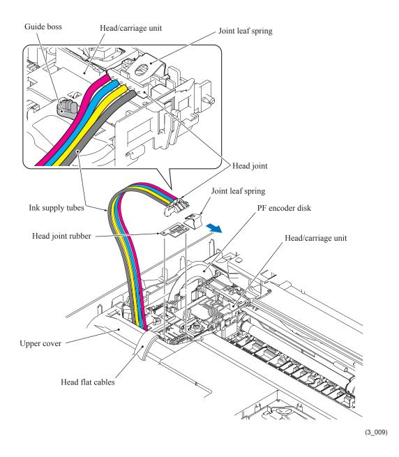
Assembling Note: Make sure that all of the four ink supply tubes are routed in front of the tube guide as shown above.
