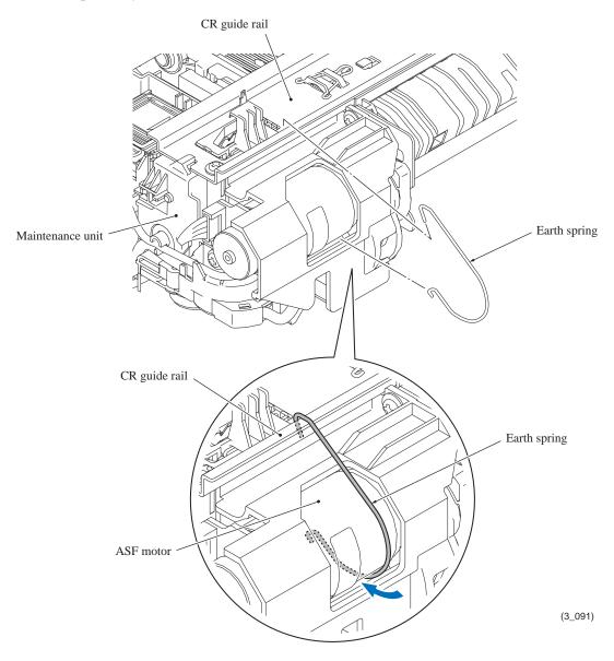
**Assembling Note:** When mounting the earth spring, take care not to contaminate it with grease. First hook the upper end on the CR guide rail and insert the lower end under the ASF motor. The earth spring twines around the ASF motor by itself with the spring force. After mounting it, check that the earth spring is in contact with the metal part of the ASF motor.
