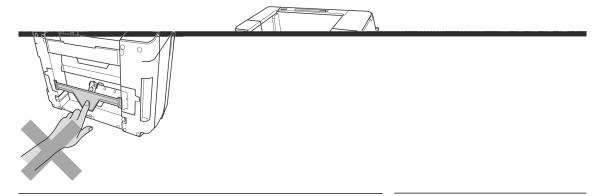
Iding the scanner cover or the Jam Clear Cover. Doing this may DO NOT carry the machine by ho
