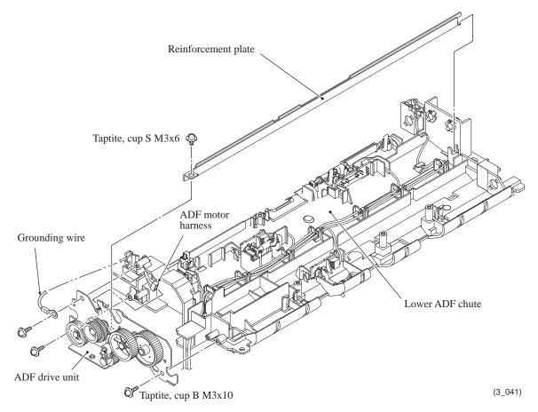
(38) Remove the gear and the screw as shown below, and take the motor off the ADF drive unit.
