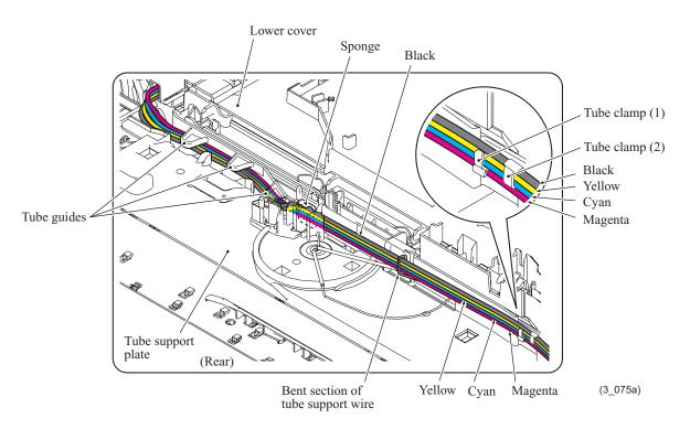
**Note:** Bind ink supply tubes with two tube clamps. As shown above, align four ink supply tubes in the order of Magenta, Cyan, Yellow, and Black from bottom to up. Set tube clamp (1) on magenta, cyan, and yellow ink tubes from the bottom, and tube clamp (2) on black, yellow, and cyan ink tubes from the top.
