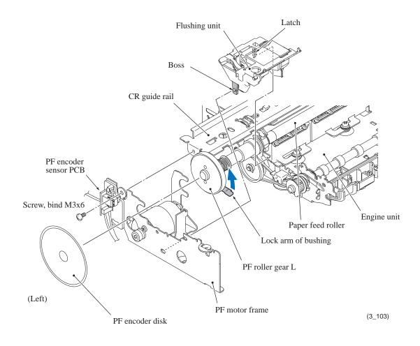
Assembling Note: When attaching the PF encoder disk to the PF roller gear L, using a spatular tool makes the job easier. Put on clean gloves to protect the disk surface from dust or fingerprints.
