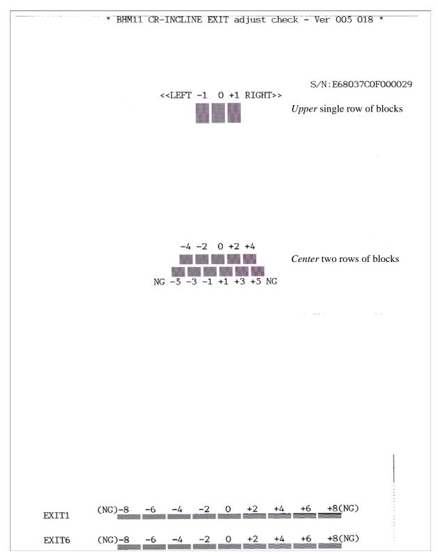
**Head Inclination Test Pattern**
