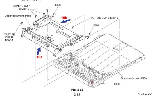
(12)Pull out the Second side CIS flat cable from the Hole of the Upper document chute.
