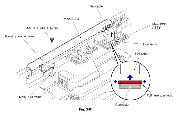
(3) Release the four Bosses and remove the Panel ASSY.
