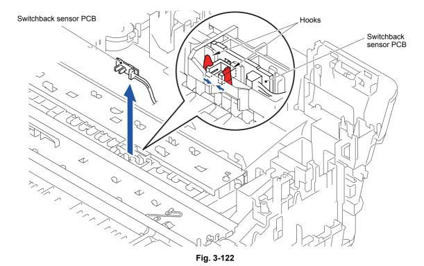
Harness routing: Refer to " Main PCB ASSY and MJ PCB ASSY", " Switchback sensor PCB"
