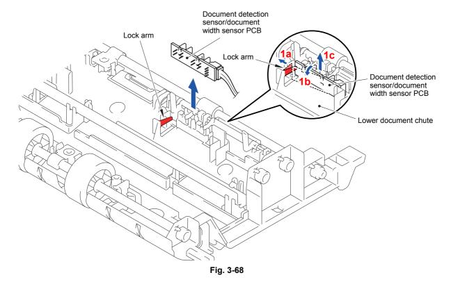
(2) Disconnect the Connector from the Document detection sensor/document width sensor PCB.
