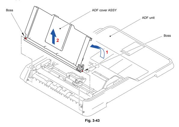
(3) Release the nine Hooks and remove the ADF cover side cover from the ADF cover ASSY.
