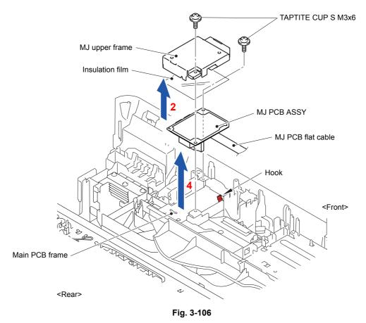
Harness routing: Refer to " Main PCB ASSY and MJ PCB ASSY"
