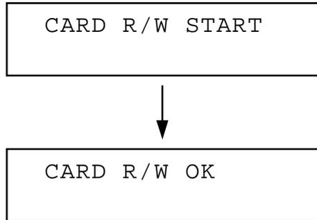
CARD R/W OK: The compact flash card works correctly.
