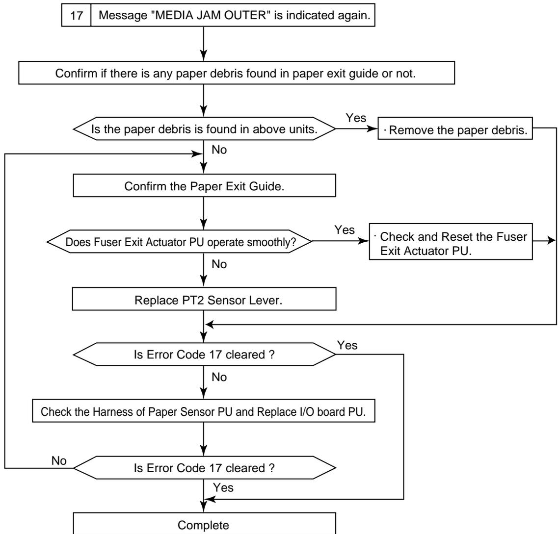
PT2 Sensor : Fuser Exit Sensor
