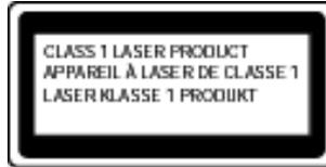
This printer has a laser diode which emits invisible laser radiation in the Laser Unit. The Laser Unit should not be opened without disconnecting the two connectors connected with the AC power supply and laser unit. Since the variable resistor in the laser unit is adjusted in accordance with the standards, never touch it.
