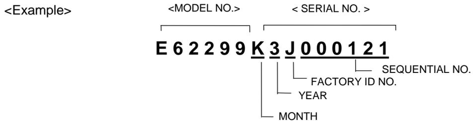
(2) Process unit: Imprinted on the aluminum bag
