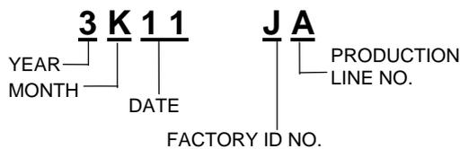
(3) Drum unit: Printed on the bar code label attached inside the drum unit
