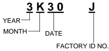
Printed on the bar code label attached on the toner cartridge
