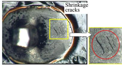
Figure 1 Shrinkage Cracks
