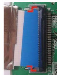
NG: The FFC is not connected straight.
