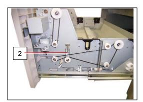
3. Pressing down the Pulley 3 (3), remove the **Timing Belt 753** (4). Replace the **Timing Belt 753** (4) with the new one.
