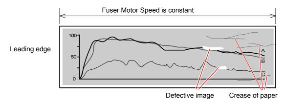
It is effective to fix these problems if we change the Fuser Motor Speed step by step during 1 sheet of print.
