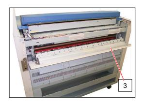
3. Moving the stopper levers (4) to the inside, remove each Duct 5 (5) with Filter 2.
