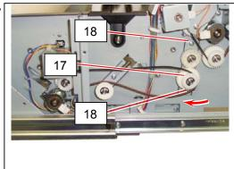
(2) You do not have to adjust the belt tension especially.As the Spring 7 (21) gives enough tension to the Timing Belt 480, just tighten the
