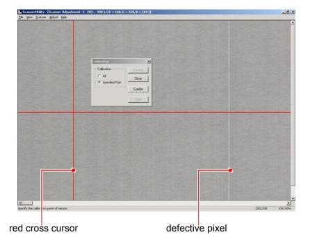
12. Move the red cursor so that its vertical line matches the defective pixel and click it. The defective pixel is selected by this operation.
