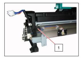
3. Remove 4 pieces of 4x6 screws (2) which fix the Hopper Assembly.
