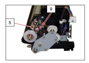
6. Reinstall the Gear Helical 20T (6) and the Retaining Ring-E (8).
