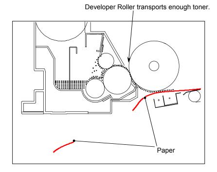
2. It is preferable for avoiding the deterioration of toner not to transport so much toner when the situation is "interval of print" (paper does not exist under the Drum).
