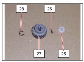
19. Set the Collar (25) onto the shaft of Regulation Roller. Install the Parallel Pin (26) to the shaft.
