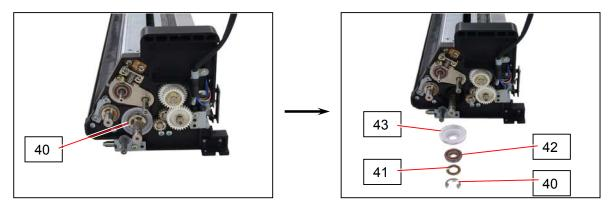
17. Remove the Retaining Ring-E (44 : E10) to remove Thrust Washer (45 : 12.2x20x0.5), Bearing (46) on the Electrode Plate side.
