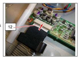
(2) Each Flexible Cable is fixed with the tapes (13). Strip off the tape (13) to make the Flexible Cable free.
