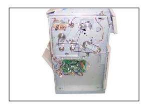
6. Loosen the 4x6 screw (8), move the Pulley 3 (9) toward the arrow mark, and then remove the Belt 1 (10).
