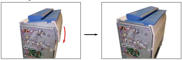
34. Both the LED Head and the Image Corona are locked with the screws (41) being separated from the Drum, not to be damaged during the transportation. Loosen the screws (41) to unlock the Fixing Brackets (42) at both sides. Pressing down the Fixing Brackets (42) firmly, tighten the screws (41).
