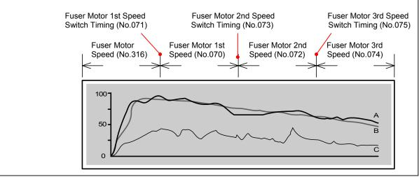
You can specify the Fuser Motor 1st Speed, 2nd one and 3rd one in each Item No.070, 072 and 074.
