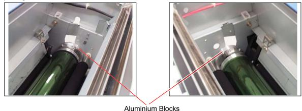
Print out the Test Pattern No.3 to check if the Aluminium Blocks are fixed at the correct position. The density of halftone is uniform as the following left image if the Aluminium Blocks are fixed at the correct positions (focus is good).
