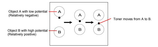
On the contrary, suppose that the toner exists on the object B of which electric potential is higher than the object A.
