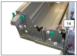
12. Mount the Roll Deck 2 Drive Assembly (15) onto the Roll Deck.
