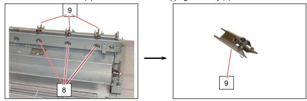
9. Disassemble the Nail Stripping Assembly as the following photo. Replace the Nail Stripping (10) with the new one.
