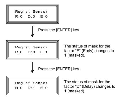
6. In case you will mask any error, press the [ENTER] Key several times to indicate the necessary mask item.
