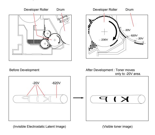
Even if some toner has not been removed by the Cleaning Roller but remained on the -620V area of Drum (It corresponds to the white area of the print) in the later [3.1.2.7 Drum Cleaning], this toner is removed at the time of Development because it moves to the Developer Roller of which potential (-230V) is higher than that of Drum (-620V).
