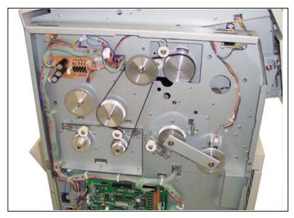
Loosen the 4x6 screw (17), move the Pulley 3 (18) toward the arrow mark, and then remove one more piece of Belt 1 (19).
