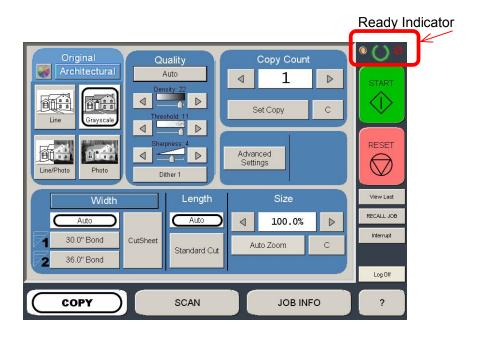
4. The Ready Indicator lights green when the KIP 3000 is ready. Set media type / width and then make a test copy.
