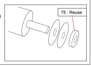
31. Remove both the **Seal L Assembly** (74) and **Seal R Assembly** (75), and replace them with the new one.
