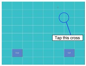
The cursor will appear just underneath the tapped point in a correct condition (calibration is not necessary).
