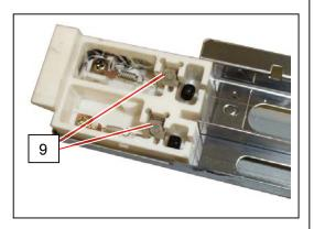
(2) Fit the Corona Wire into the groove of Height Adjuster (10).
