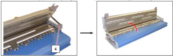
4. Loosen 2 pieces of screw (5), and then bring down the Tension Pulleys (6) to unfasten the Belt.
