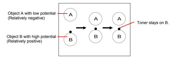
Thus, the toner has a characteristic to move from one place with a lower potential to another place with a higher potential.
