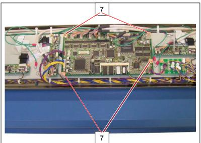
Disconnect all of the Flexible Cables (8) from each CIS Controller Board. (Handle with great care not to break the Flexible Cable at this time!)
