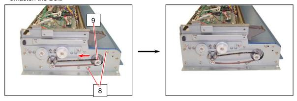
5. Remove the Belt 60S2M284 (10), and replace it with the new one.
