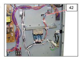
34. Connect the above mentioned Relay Cables (42) to the Relay (43).
