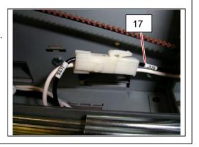
10. Connect "J114" side (18) of the AC Paper Harness 2 to the Dehumidify Heater.
