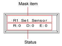
Pressing [←] key or [→] key, indicate the necessary mask item on the LCD.
