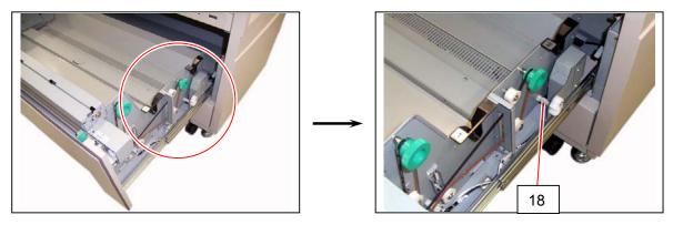
11. Install the Cover 2 (19) with 2 pieces of 4x6 Bind Screw (20) to hide the harness.
