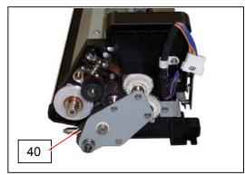
To make sure, rotate the Gear Helical 34T (39) by hand from under the Engine Unit. Both gears will be in gear by this treatment.
