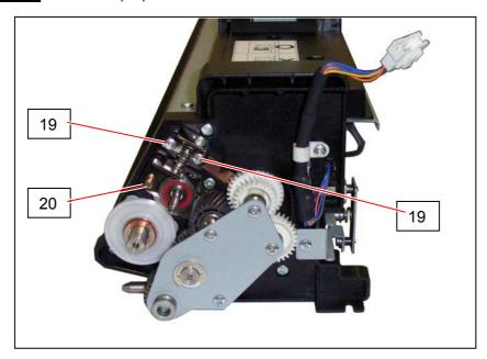
16. Completely press down and hold the Bracket 4 (21), tighten the screws (19).
