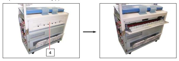
5. Remove the 4x6 screw (5) to remove the Plate 2 (6) on the right of machine.
