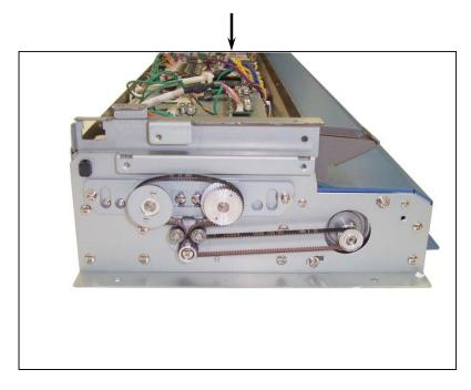
3. Remove the Belt 60S2N250 (4), and replace it with the new one.
