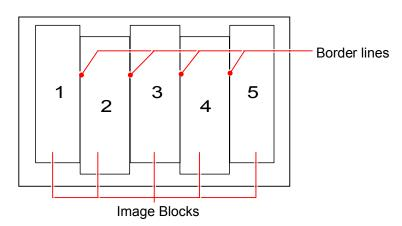
You can integrate these Image Blocks correctly by specifying the same image included in both Image Blocks. (By selecting the same image, the program automatically calculates how much the image Block should be shifted vertically and horizontally.)
