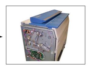
7. Rotate 4 Levelling Bolts (7) on the bottom of the KIP 3000 with a wrench to bring up the KIP 3000 from the floor.
