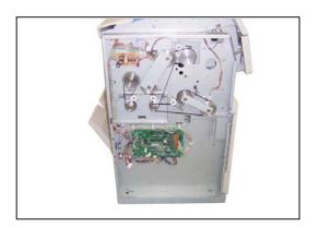
Loosen the 4x6 screw (4), move the Pulley 3 (5) toward the arrow mark, and then remove the Belt 1 (6).
