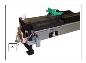
4. Remove 4 pieces of 4x6 screws (5) which fix the Hopper Assembly.
