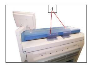
2. Remove 8 screws (2) on both front and rear side of the machine.
