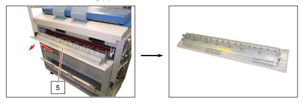
8. Remove the 4x6 screw (8) to remove each Nail Stripping Assembly (9).
