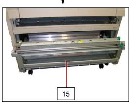
13. Fix the Roll Deck 2 Drive Assembly (15) with 2 pieces of 4x6 screw (16),
