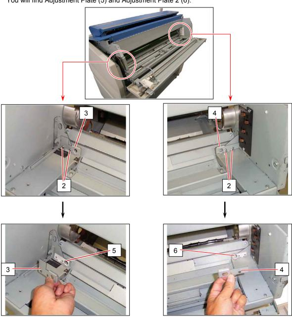
3. On the left side, add (or remove) as many Adjustment Plate (5) as required, cover them with the Bracket 32 (3), and then fix with 2 screws (2).
