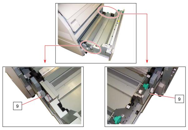
9. Loosen 4 pieces of 4x6 screw (10), and then remove the Cover 1 (11).
