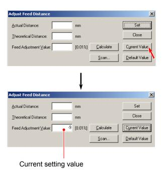
5. At first, input the actual distance between "a point" and "c point" in [Actual Distance], which you have measured at the former step "1".
