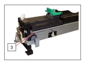
4. Remove 4 pieces of 4x6 screws (4) which fix the Hopper Assembly.
