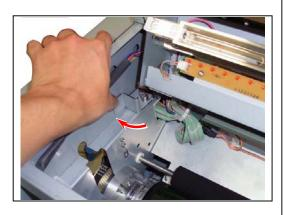
15. Remove the 4x6 screw (20) to remove the Fixing Bracket (21) on the right.
