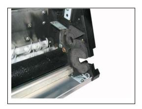
30. Remove the Retaining Ring-E (70 : E10) to remove Thrust Washer (71 : 12.2x20x0.5) and Bearing (72) on the driving side.
