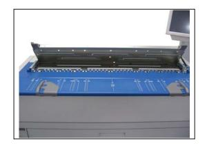
18. Put 3 pieces (for the front) or 2 pieces (for the rear) of Adjustment Plastic Sheet (30: 0.3mm thick) between Feed Roller and Scan Glass.
