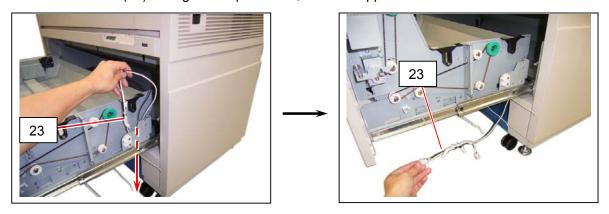
16. Put the harness (23) through the square hole, from the bottom side to the upper side.
