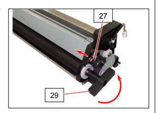
(2) Do not rotate the Developer Roller when the Gear Helical 20T (27) is not installed to the shaft of Regulation Roller!
