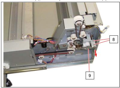
6. Remove 3 pieces of 4x6 screw (10) to remove the Bracket 9 (11).
