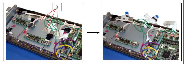
(3) The central one of Flexible Cable is running under the Data Controller PCB and the CIS Controller PCB. Remove the Ring (10), strip off the tape (11) under the Data Controller PCB, and then put the Flexible Cable aside.
