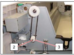
3. Remove the **Timing Belt 330** (4), and replace it with the new one.
