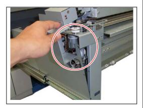
(2) Make sure that the step part (9) on the lower side of each Cover 3 (7) and Cover 7 (8) is inside of the plate (10).
