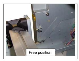
6. Fix the Brackets 26 (6) at the "free position" with the 4x6 screws (4) and (5) you have removed or loosened at the former step 3.
