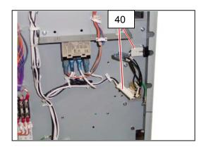
30. Fix the Ground Wires with 2 pieces of Tooth Washer Screw (41)
