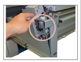
(2) Make sure that the step part (8) on the lower side of each Cover 3 (6) and Cover 7 (7) is inside of the plate (9).
