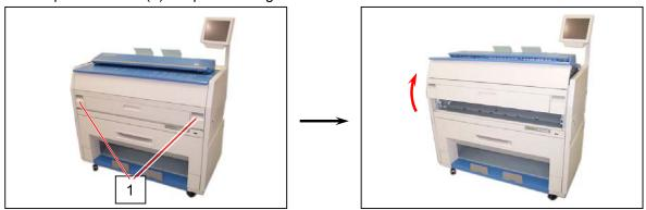
2. Remove 5 pieces of screw (2) which fix the Cover 3.
