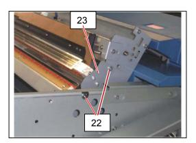
17. Move the Plate (23) to the right to release the pin (24) of Corona Block. Then remove the Image Corona Unit (25).
