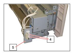
4. Remove 3 pieces of Wire Stopper Brackets (6) removing 1 piece of 4x6 screw for each.
