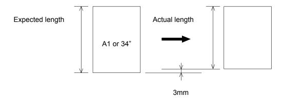
3. Necessary value for the compensation is 10 times as long as the difference between actual length and expected length.
