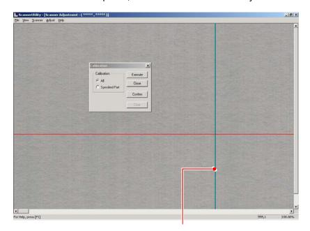
Match the vertical line to a defective pixel.
