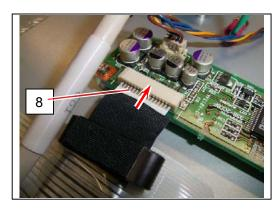
(2) Each Flexible Cable is fixed with the tapes (9). Strip off the tape (9) to make the Flexible Cable free.
