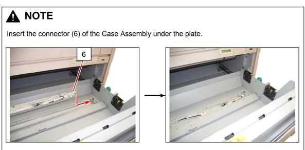
5. Fix the Case Assembly (6) with 2 pieces of 4x6 Tooth Washer Screw (7) and 8 pieces of 4x6 Bind Screw (8).
