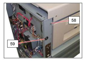
41. Hold the harness with the Bushing (59), and fit it to the Side Plate.
