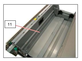
11. Remove 2 pieces of 3x6 Bind Screw (16), and remove the Cover 9 (17).
