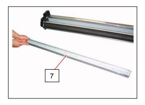
7. Remove 10 pieces of screw (8), and then disassemble the Scraper Assembly. Replace Scraper (9) with a new one.
