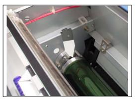
20. Remove the **Photoconductive Drum** (30), and replace it with the new one.
