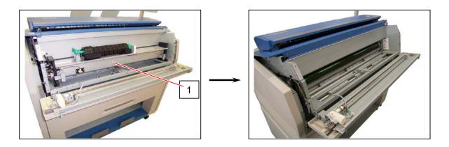
2. Remove 2 pieces of 3x6 screw (2), and then turn over the Bracket 11 (3).
