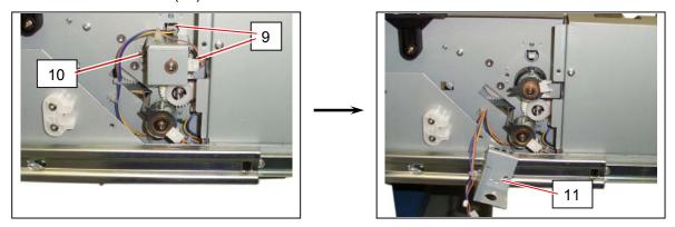
6. Pull out both the Bush (12) and the **Clutch** (13 : CL7). Replace the **Clutch** (13 : CL7) with the new one.
