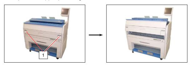
2. Remove 6 pieces of 4x6 screw (2) which fix the Cover2.
