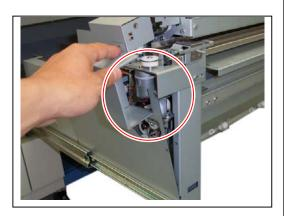
(2) Make sure that the step part (7) on the lower side of the Cover 3 (6) is inside of the plate (8).
