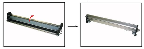
33. Remove 2 pieces of 4x6 screws (76) to remove the Bracket Assembly (77).
