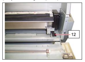
11. Holding both side plates firmly, slide the Developer Unit (13) out of the machine.
