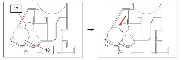
(2) Make sure to fix the right side (electrode plate side) of the Regulation Roller first then the left side (gear side).
