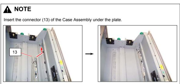
9. Fix the Case Assembly (12) with 2 pieces of 4x6 Tooth Washer Screw (14) and 8 pieces of 4x6 Bind Screw (15).
