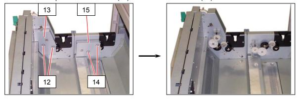
9. Remove the 4x6 screw (16) to remove each Bracket 12 (17).
