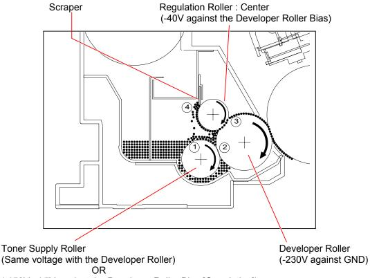
(-150V +/-5V against the Developer Roller Bias [On printing]) (Or -50V +/-5V against the Developer Roller Bias [Interval of print]) 5. The voltage of both sides of Regulation Roller is 0V as these parts are connected to the ground.
