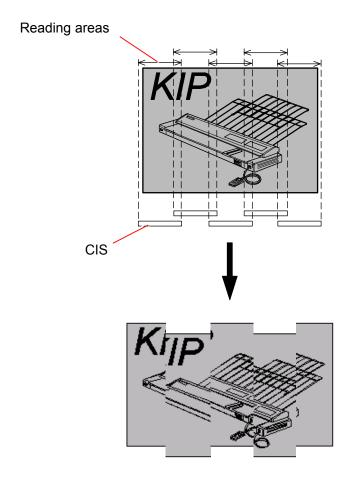
The image data before the positioning process
