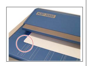
6. Click [OK] after setting Shading Sheet, and the scanner reads it. It takes about 5 minutes to complete Shading adjustment.
