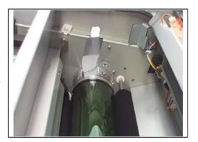
19. Similarly loosen 2 pieces of screw (28) on the right and rotate the Block 2 (29) as the arrow marks.
