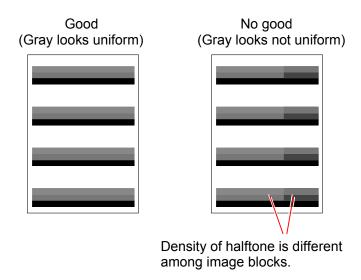
If the focus of LED Head is not good, fix the Aluminium Blocks properly making reference to the next page.
