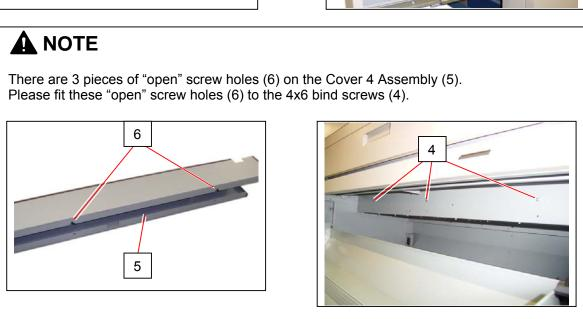
5. Put 3 more pieces of 4x6 screws (4) to the lower 3 pieces of screw holes. Then tighten 6 pieces of 4x6 screws (4) to fix the Cover 4 Assembly (5).
