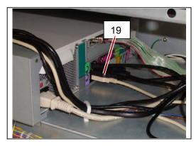
15. Open the Wire Saddles (20) to release the USB Cable (19).
