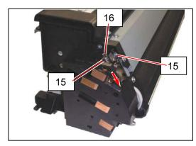
(2) On the left side of the unit (gear side), confirm that the Bracket 4 (21) is fixed with the screws (19) being completely pressed to the arrow direction.
