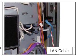
45. Connect the Power Supply Cable (47) to the connector (64) of the DC Power Supply. Hold the Power Supply Cable (47) with the Wire Saddles (65) at this time.
