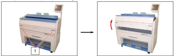
2. Remove 5 pieces of screw (2) which fix the Cover 3.
