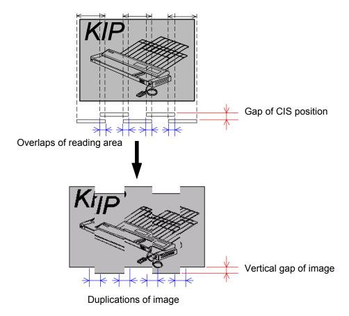
"Position" is the solution for these kinds of phenomenon. It is possible remove the vertical gap of image by vertical positioning process (Y offset). And it is also possible to remove the duplication of image by horizontal positioning process (X overlap).
