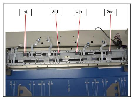
20. Open the scanner upper unit and remove Adjustment Plastic Sheets (30). Close the scanner upper unit.
