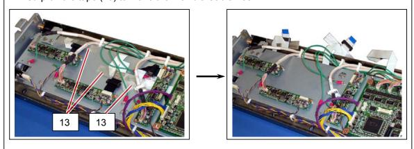
(3) The central one of Flexible Cable is running under the Data Controller PCB and the CIS Controller PCB. Remove the Ring (14), strip off the tape (15) under the Data Controller PCB, and then put the Flexible Cable aside.
