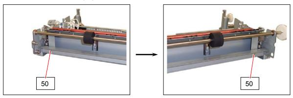
29. Remove the Guide Plate 2 Assembly (51).
