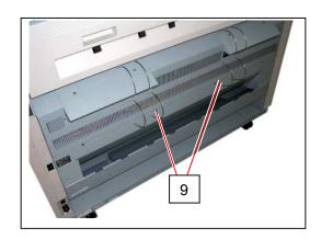
7. Attach 2 Plate 5 Assembly (10) with 4x6 Bind Screws (9) you have removed at step 6.
