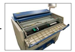
7. There are 2 pieces of Stopper (10) at both sides, which lock the LED Head Frame. Loosen the screw (11) and then slide the Stoppers (10) outside to unlock the LED Head Frame.
