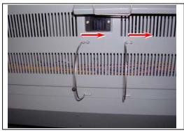
(2) Direct the flat end of each Arm 3 (7) and Arm 4 (8) to the bottom.
