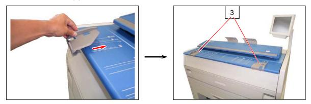
3. Loosen 4 screws (4), fit the Plate 2 (5) to the screws (4), and tighten the screws (4).
