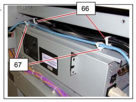
(2) Between the Wire Saddle (66) and the terminal of each cable, bundle each VGA Cable, Power Supply Cable and external cable together with the same Wire Saddle (68). But do not bundle the USB Cables (69: for both scanner and UI) together at this time, because the USB Cable is the great cause for a noise issue.
