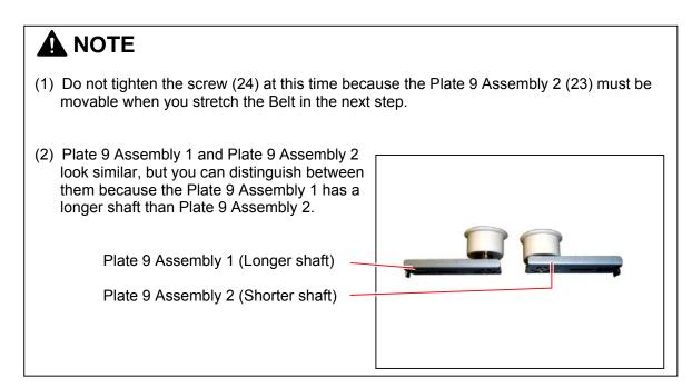
18. Stretch the Timing Belt 753 (26) among gears and pulleys. Then, tighten the screw (24) to fix the Plate 9 Assembly 2.
