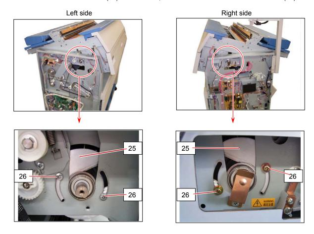
Do as follows to fix the Aluminium Blocks correctly.
