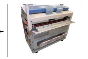
6. Remove the 4x6 screw (6) to remove the Plate 2 (7) on the right of machine.
