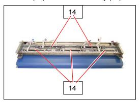
9. Remove 4 screws (16) and remove CIS Assembly (14). Replace CIS Assembly (14) with a new one.
