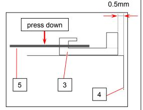
(2) Carry Image Corona Unit (1) by both corona blocks so that Grid Plate (5) faces the floor. Make sure that Grid Plate (5) has no excess slack (in less than 1mm) on the middle of the housing.
