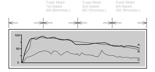
You can specify the switch timing to each Fuser Motor 1st Speed, 2nd one and 3rd one in each Item No.071, 073 and 075.
