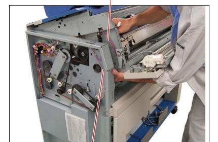
Hold the Gear Helical 28T with one hand.
