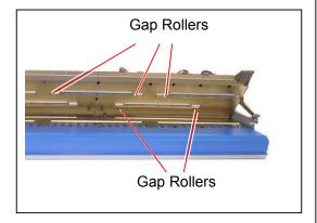
(2) 2 of all the 8 Gap Rollers are slightly wider, 2 types of Gap Roller replacement kits are provided.
