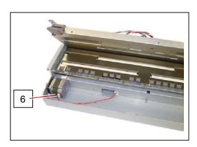
6. Remove 2 pieces of 4x6 screw (7) to remove the Motor Assembly (8). Replace the Motor Assembly (8) with the new one.
