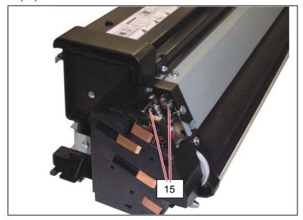
14. Completely press down and hold the Bracket 5 (16), and tighten the screws (15). (The Regulation Roller is pressed onto the Developer Roller.)
