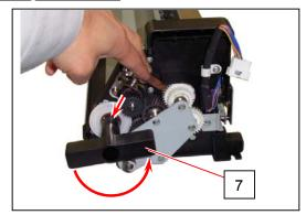
4. Remove both the Retaining Ring-E (8) and the Gear Helical 20T (6).
