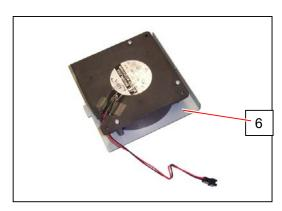
3. Remove 3 pieces of 4x35 screw (8) to remove the **Blower** (9). Replace the **Blower** (9) with the new one.
