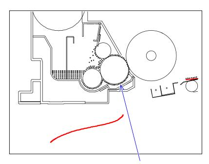
This toner is returned to the Developer Unit as it was not transferred onto the Drum.
