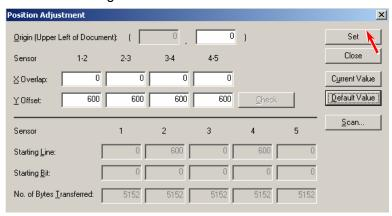
6. Set the Target Sheet to the scanner unit, and then click [Scan].
