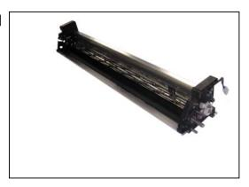
2. Remove Retaining Ring-E (1: E10) to remove Bearing (2).
