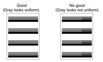
If it is still not uniform although you have fixed the Aluminium Blocks correctly, it is necessary to make focus adjustment with Spacers.
