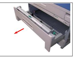
9. Remove 1 screw (7) and loosen 1 screw (8) on each side.
