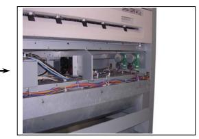
3. Disconnect the connector (6), remove 1 screw (7), and then remove the Bracket Blower (8). Remove 3 screws (9) to replace Blower (10) with the new one.
