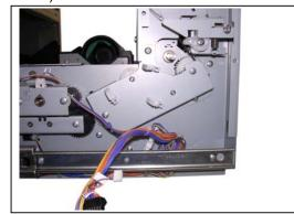
8. Remove 4 screws (17) to remove Bracket 33 (18).
