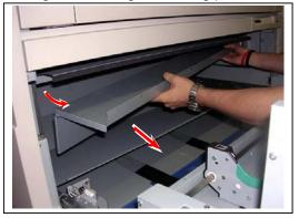
17. Remove 2 screws (21) to remove Bracket (22). (One of the screws (21) will be reused.)
