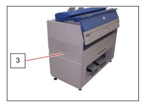
3. Remove 4 pieces of 4x6 screw (4), loosen 4 pieces of 4x6 screw (5), and then remove the Cover 15 (6).
