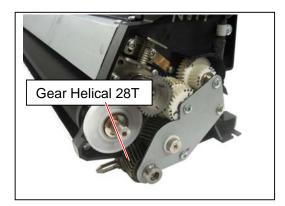
If there is no space between these gears, **the gear may be broken**. In this case it is necessary to add Adjustment Plates to keep a space.
