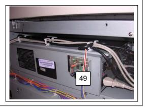
38. Secure Power Supply Cable (43) with wire saddles (50) and connect it to the connector on DC Power Supply (51).
