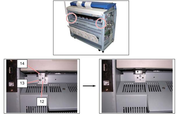
11. With Engine Unit <u>open</u>, remove **Fuser Unit** (15).
