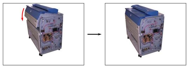
8. Rotate 4 Leveling Bolts (7) on the bottom of the KIP 3100 with a wrench to bring up the KIP 3100 from the floor.
