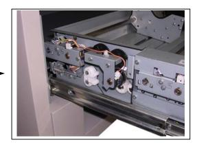
3. Remove 1 Bind Head Screw (4) and 1 Pan Head Screw (5), disconnect the harness (6) to remove Clutch (7: CL6). Replace **Clutch** with a new one.
