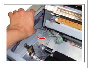
15. Pull up the Lever 2 (20) to open the Engine Unit.
