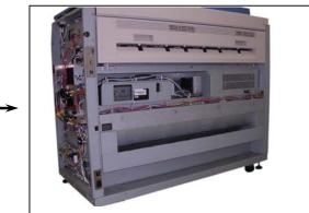
2. Disconnect the connector (4), remove 1 screw (5), and then remove the Fan Bracket (6). Remove 4 screws (7) and 1 connector (8) to replace Fan (9) with a new one.
