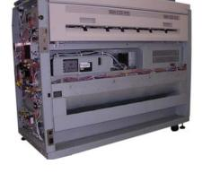
27. Remove 5 screws (30) to remove Case 5 (31).
