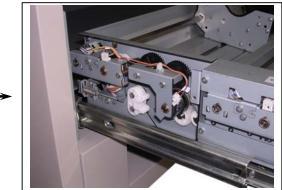
14. Remove 1 Bind Head Screw (16) and 1 Pan Head Screw (17) to remove Gear Bracket 2 Assy (18).
