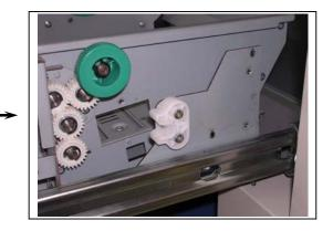
18. Loosen 1 screw (26) to release Pulley 3 (27). Move Pulley 3 (27) upward and fix it with the screw (26) to release Timing Belt 453.
