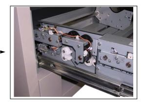
3. Remove 1 screw (4) to release the sensor bracket (5). Remove 1 connector (6) to replace Sensor (7: PH10) with a new one.
