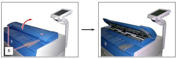
4. Remove 1 screw (7) to remove Stay (8) Open Upper Unit fully.
