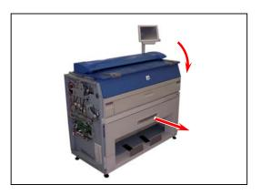
12. Remove 7 screws (12) to remove Cover 14 (13).
