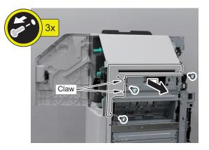
4. Remove the Hinge Unit (rear) from the Upper Cover.
