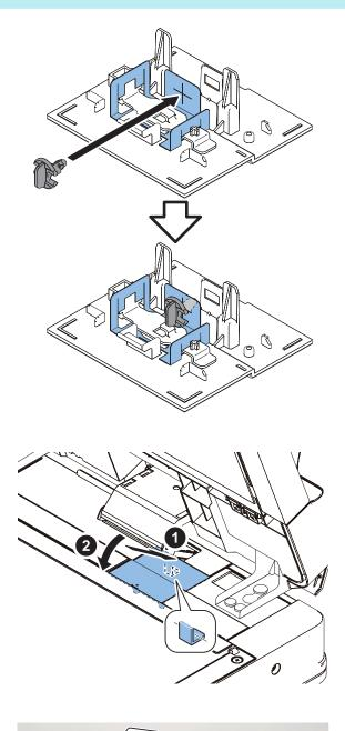
10. If the Cassette Pedestal is installed, turn the 3 adjusters of the Cassette Pedestal and fix.
