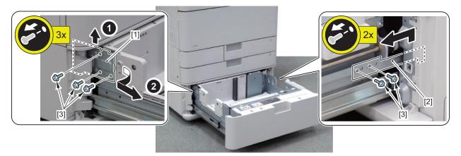
3. While pressing the 2 Leaf Springs [1] on the right and left of the rail, further pull out the High Capacity Cassette [2].
