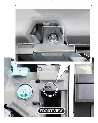
4. Loosen the screw fixing the Punch Unit positioning Guide, and then move the guide to adjust by referring the line marked in step 3. After adjusting, tighten the screw.
