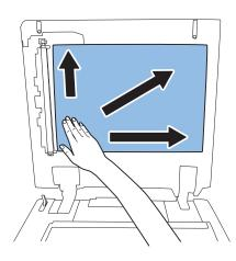
9. With the ADF closed, check that the White Plate is not placed on the Index Sheet as shown in the figures.
