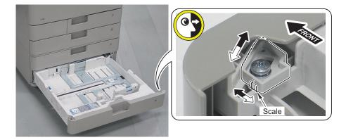
3. Loosen the 1 Fixation Screw.
