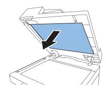
6. Place the White Plate on the Copyboard Glass by aligning it with the Index Sheet.
