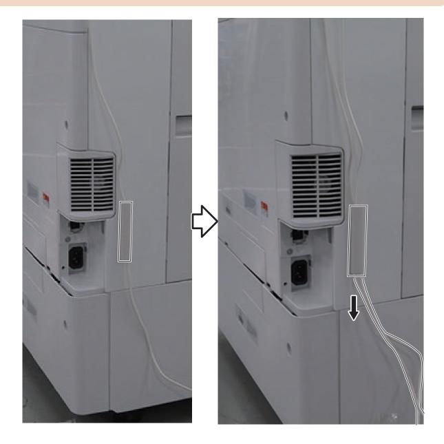
**11** Connect the power plug to the outlet. **12.** Turn ON the main power switch.
