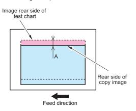
4. If it is not within the standard range, adjust the image position in the following service mode. COPIER > ADJUST > ADJ-XY > ADJY-DF2
