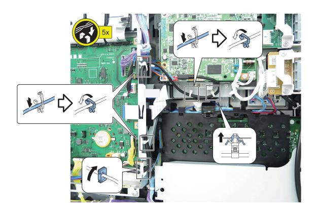
**7** Install the removed cover and the telephone code.
