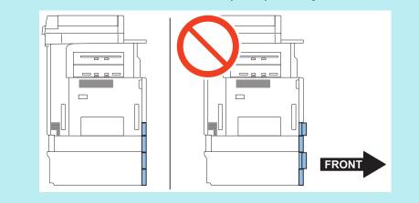
6. Pull out the next upper cassette, and check if the Adjustment Plate is correctly pushed against the frame.
