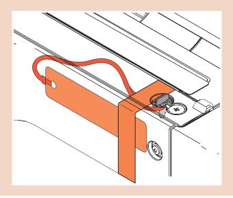
4. Open the right door of the host mashine and remove the two pins of the Secondary Transfer Outer Roller.
