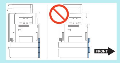
**6** Pull out the next upper cassette, and check if the Adjustment Plate is correctly pushed against the frame.
