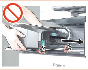
• Do not put the Harness of the Inner Finisher and Sensor Flag between the Inner Finisher and Host Machine.
