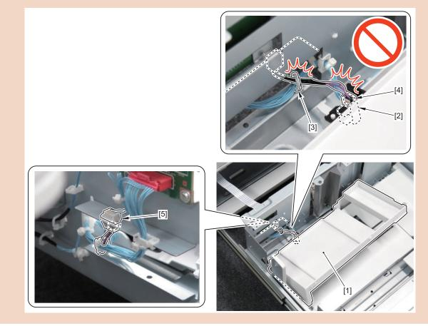
5. Switch the position of the boss [2] on top of each Paper Guide [1] from A4 to LTR.
