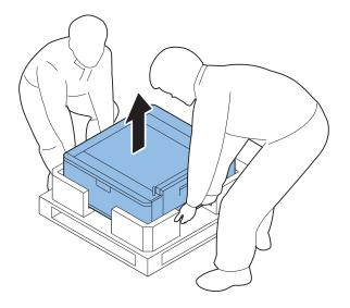
**3.** Remove the tapes attached to the packaged parts, the outside and inside areas of this host machine.
