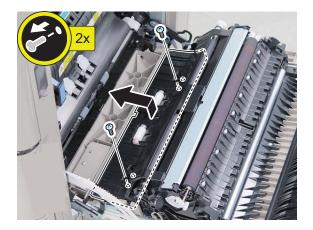
4. Remove the 3 springs from the guide removed in step 3, and install the 3 springs included in the package.
