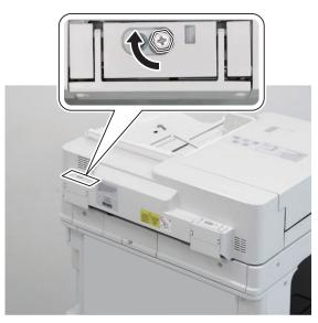
• If the rear side is not installed properly: Turn the Left Hinge Fixation Screw counterclockwise (white arrow).
