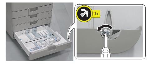
4. Move the Adjustment Plate left or right based on the scale value checked in step 2. (As the Adjustment Plate is moved toward the left of the machine by 1 tooth, the left edge margin is increased by 0.5 mm.)
