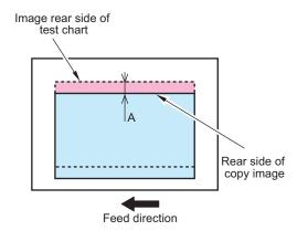
If it is not within the standard range, adjust the image position in the following service mode. COPIER > ADJUST > ADJ-XY > ADJ-Y-DF
