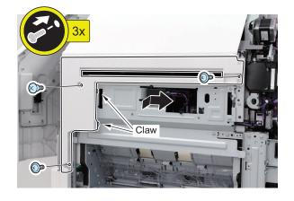
23. Insert the Punch Waste Tray in the direction of the arrow from the front.
