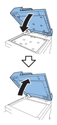
8. Press the White Plate upward as shown in the figure below.
