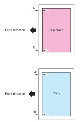
3. Loosen the screw securing the right hinge, and slide the hinge to the front or rear with reference to the marking-off line to adjust the perpendicularity.
