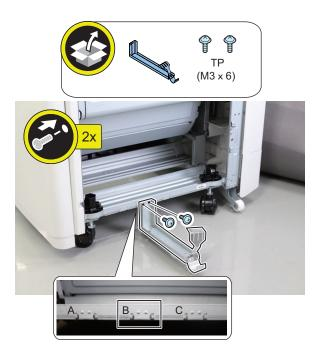
**NOTE:** Install the Ground rail to the position [B]. **2** When the Service Book Holder has already been installed in the host machine, relocate it to the Finisher.
