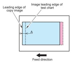
6. If it is not within the standard range, adjust the image position in the following service mode.
